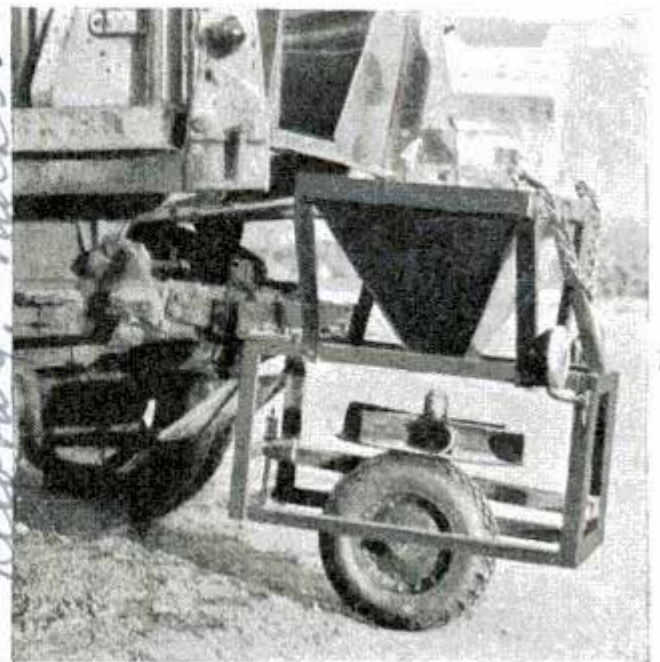
Sand-spreading trailer showing disk resting on rubber-tired wheel, and the hopper above
