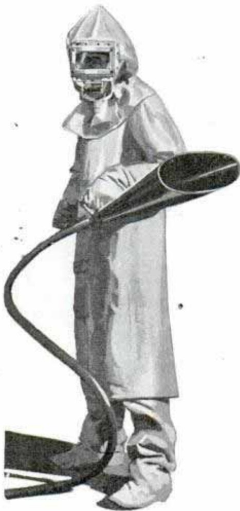
Left, "hot papa" holding carbon-dioxide thrower for quenching flames. Below, attaching disabled plane to truck before hauling the ship off the field
