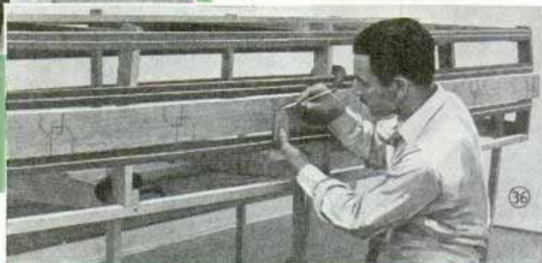
PLANKS ARE FITTED FROM BATTEN CENTERLINE TO BATTEN CENTERLINE, THE SHAPE BEING DETERMINED BY SPILING
