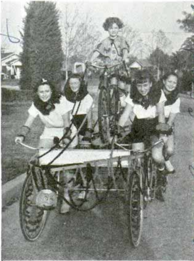
Four of the riders supply all the power needed to propel this float made by combining two tandems
