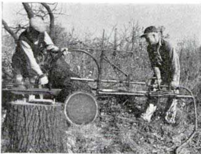
Two men grip the saw frame as the blade, reciprocated by an air compressor, cuts through a big log
