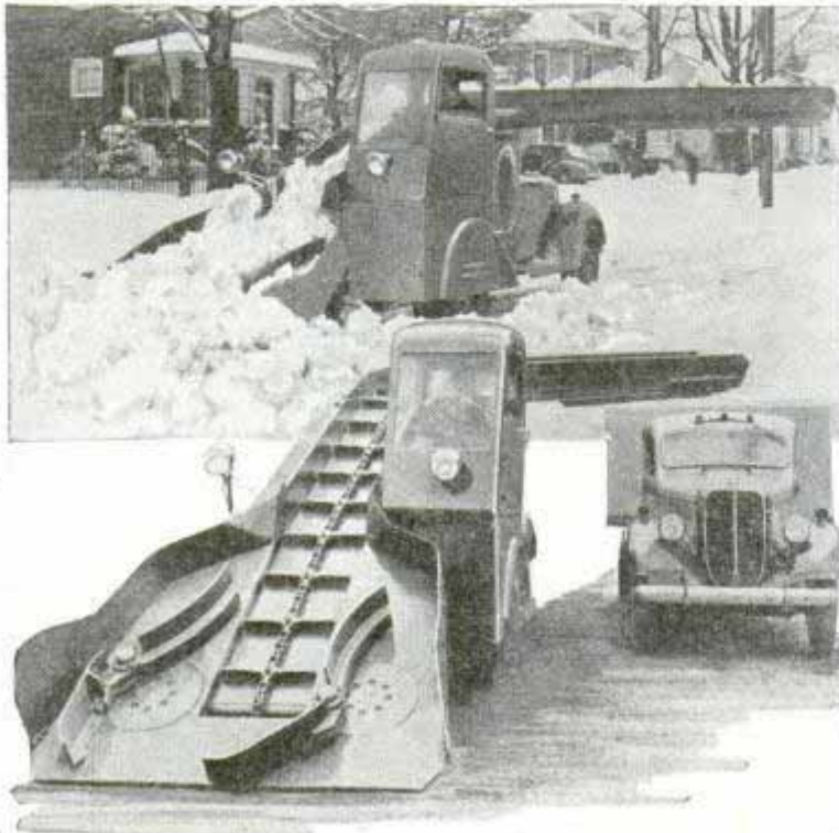
Truck follows alongside or behind to receive snow and ice picked up by scraper and elevated to long conveyor on top
