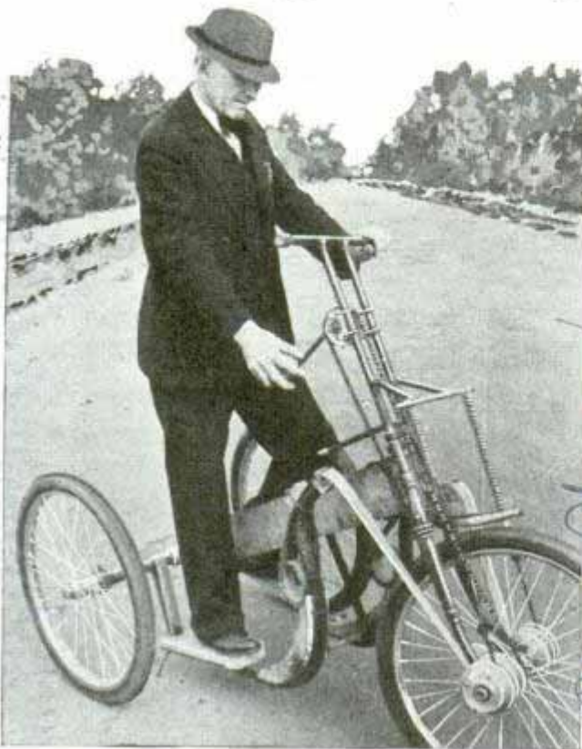
Treading on pedal boards drives this unique tricycle, and there is an extra pull in hand-turned crank
