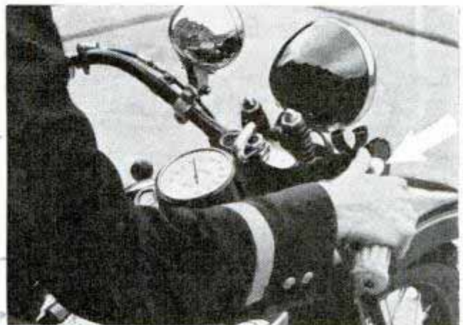
Pressing button with thumb "freezes" speedometer needle to keep record of traffic violator's speed
