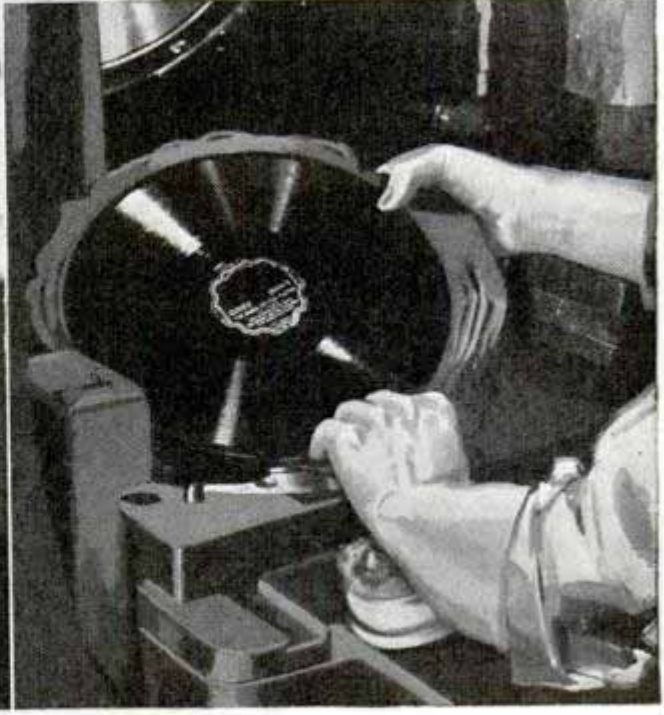
In taking off "lost voice" from fragile original record with aid of delicately cut sapphire, cylinder is played through amplifier to modern master disk, top. Center, record taken to R.C.A. laboratory is recorded on wax disk. Bottom, modern record on which voice is reproduced for posterity, and, right, Victor record just pressed and still retaining excess "dough" on edges
