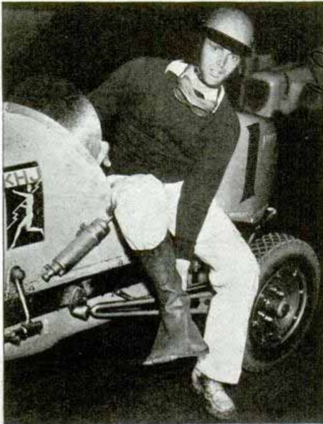
Inner tube protects driver's throttle foot in car that has developed an oil leak
