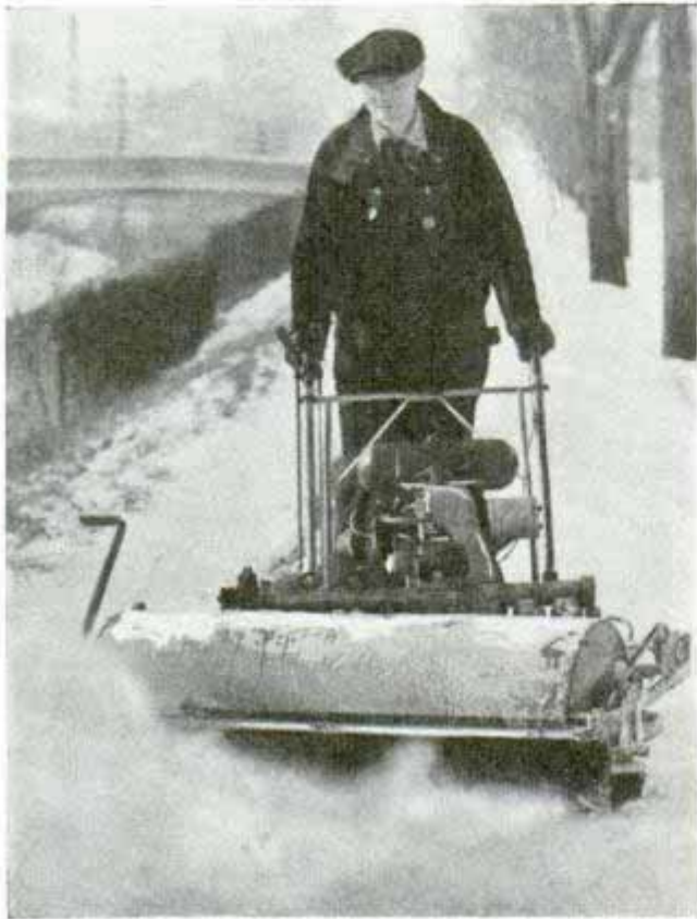
Snow removal is easy with this gasoline-driven plow which will go back to cutting grass next summer
