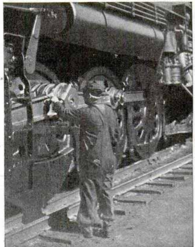
Measuring slack in driving rods with caliper while hostler sends "thump" of steam against set brakes
