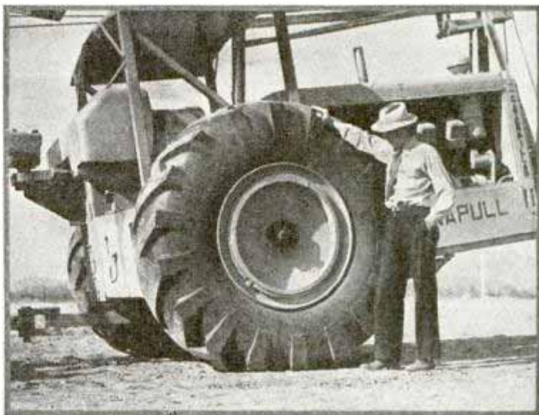
Above, the two-wheeled power unit. Note that the tires are man-size. Left, tractor hooked to a two-wheeled scraper, forming a forty-foot earth-working unit. The scraper has a capacity of thirty-eight cubic yards of dirt and it is useful in flood-control and dam-building operations. A Diesel engine develops 160 horsepower to drive the unit
