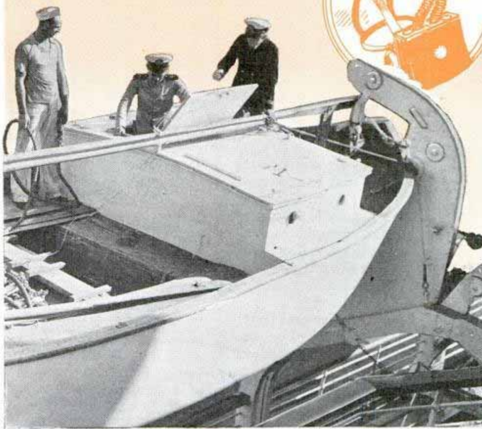
Left, ship's engine controls. Right, rescue-squad man. Bottom, inspecting motor lifeboat. Radio and engine are carried in watertight compartment
