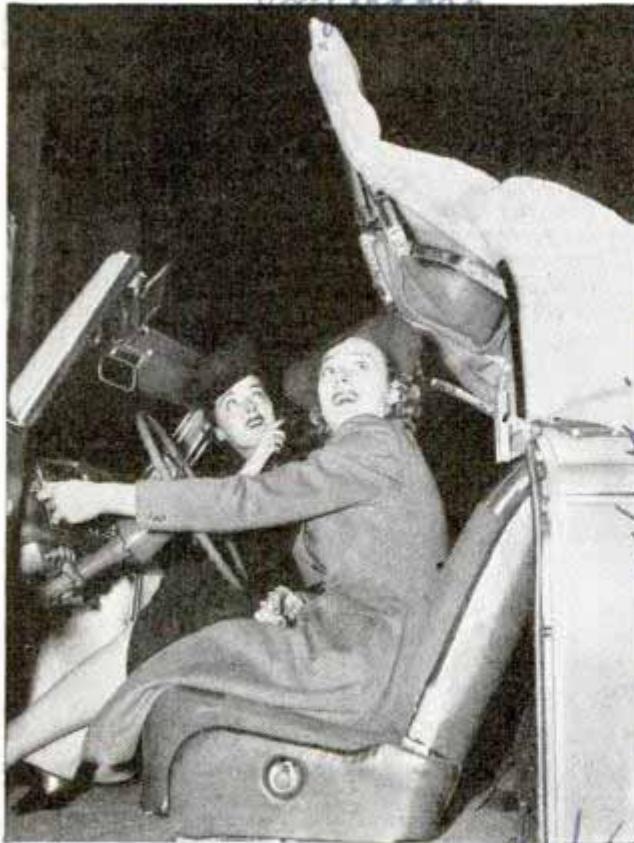
Cameraman catches top folding as driver operates control on the instrument panel
