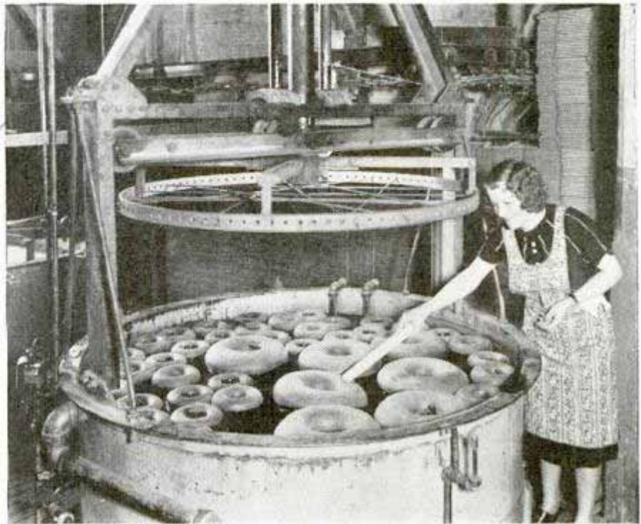
Like so many giant doughnuts, tubes for airplane tires are tested for leakage in water vat, thus assuring passengers of more safety
