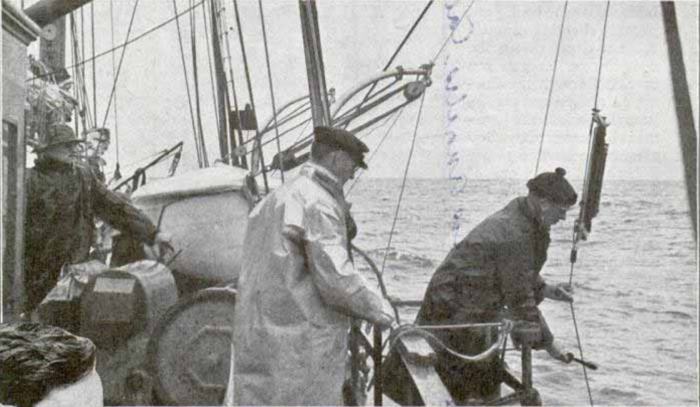
Lowering bottle for taking samples of deep-sea water. Left, "snapper" sampler with jaws which close automatically and bite out sample when bottom is touched
