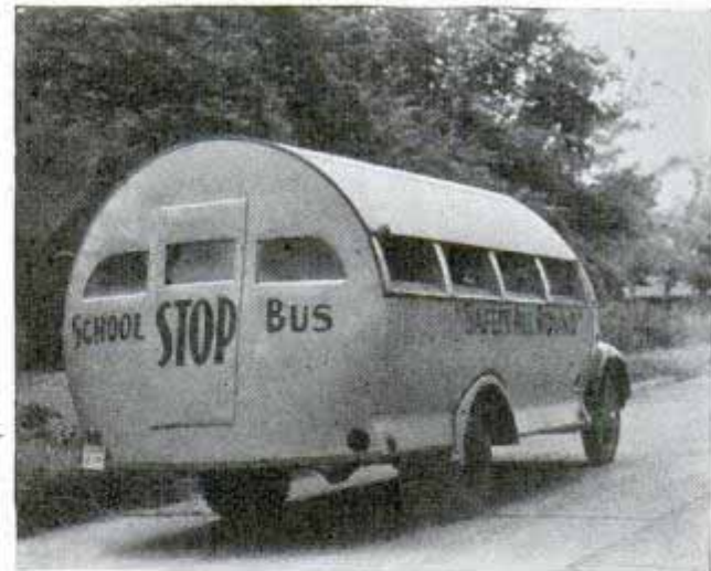
Youngsters riding in this school bus are safer, since it would roll over instead of taking flat crash
