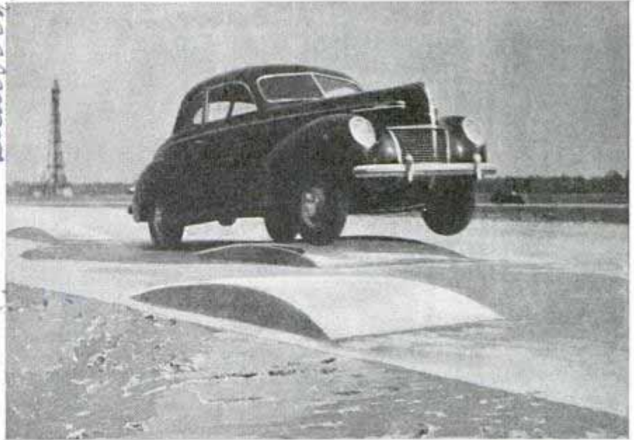
Auto "hitting the high spots" while being given a body-twisting test on new track. Note humps in the pavement
