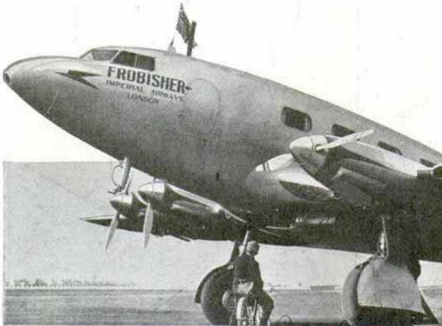
Nose of the new British streamline ship. Note flowing lines of engine nacelles and the front of passenger compartment
