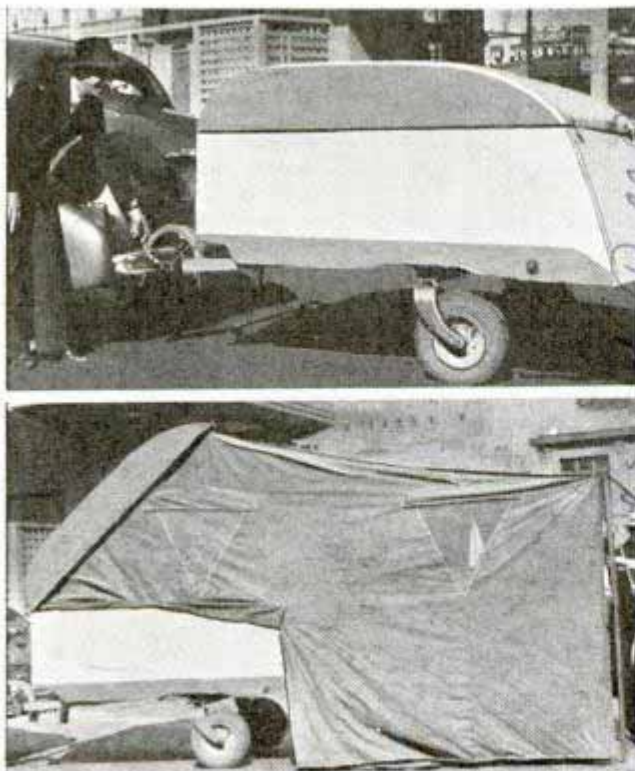
Double-arm coupler on this trailer, shown packed and with tent raised, is easily attached to any car
