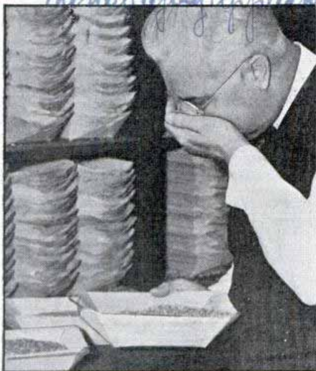
Smelling sample of grain to detect odor of weevil, smut or other defects
