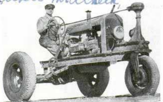
Farmer driving the three-wheeled tractor built from discarded automotive vehicles
