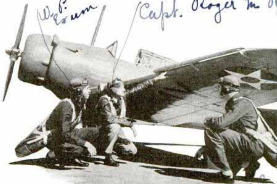
Pilot pointing to "eyebrow slot," a new safety device used on training plane to speed up recovery from stalling and spinning
