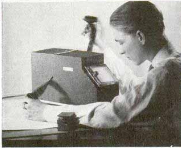
Top, inserting paper for enlarging; below, using ground-glass window for viewing strip of film
