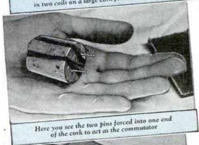
Twenty feet of No.-30 enameled wire wound in two coils on a large cork forms the armature
