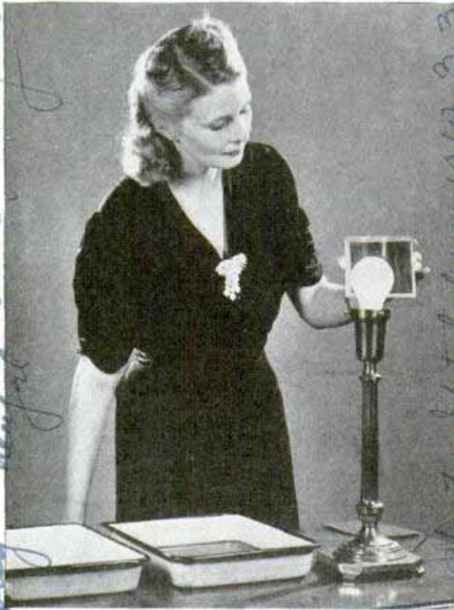
"Safelight paper" containing orange dye is placed with negative in flexible frame and exposed to light
