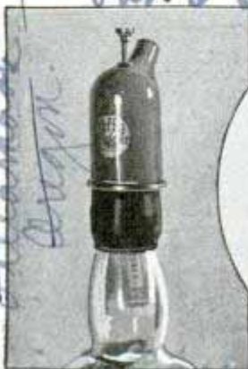
Pressing the plunger of dispensing cap measures out exactly one ounce of fluid from bottle
