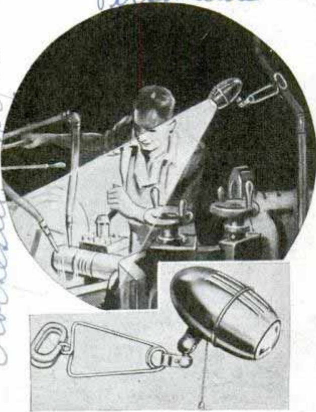
At top, spotlight is clamped to pipe in workshop and focused on center of operations
