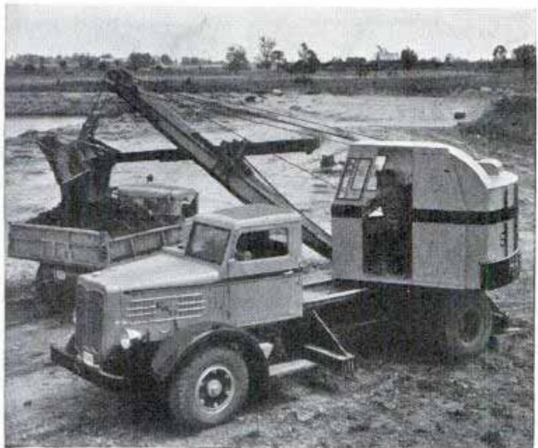
Notice the single-seat cab on this truck. It is made narrow so that the shovel boom can swing without interference
