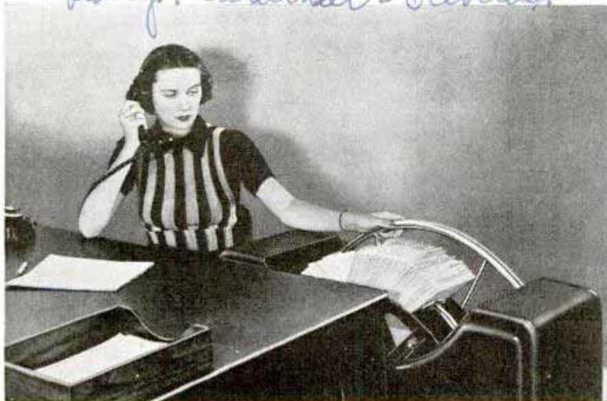
As many as 7,000 reference cards can be kept on this rotating-wheel file. A quick spin brings the desired card to the top
