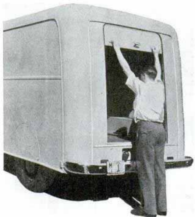
Opening like a roll-top desk, this flexible steel door makes it easy to load and unload truck
