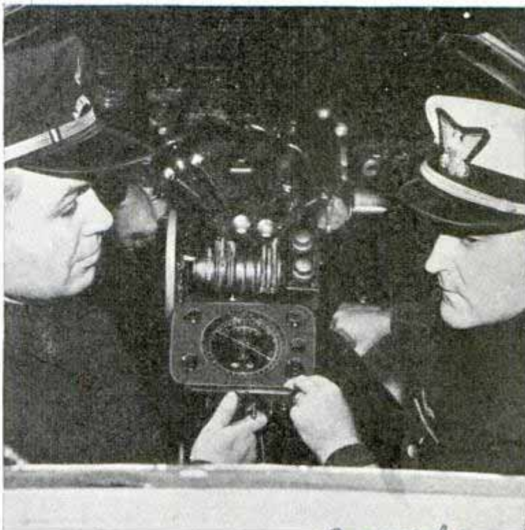
Acme. Automatic direction finder in cockpit of plane. Here the instrument is being set to tune in radio station
