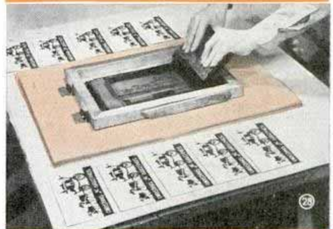
AFTER PRINTING, THE SCREEN IS HELD UNDER HOT WATER TO BRING OUT THE PICTURE-LEFT
