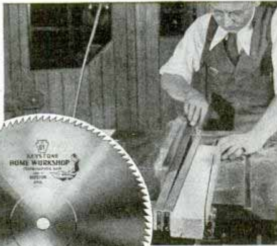
CUTTING TAPERS A hinged jig, with means for securely holding one end of work away from fence, makes cutting of tapers easy
