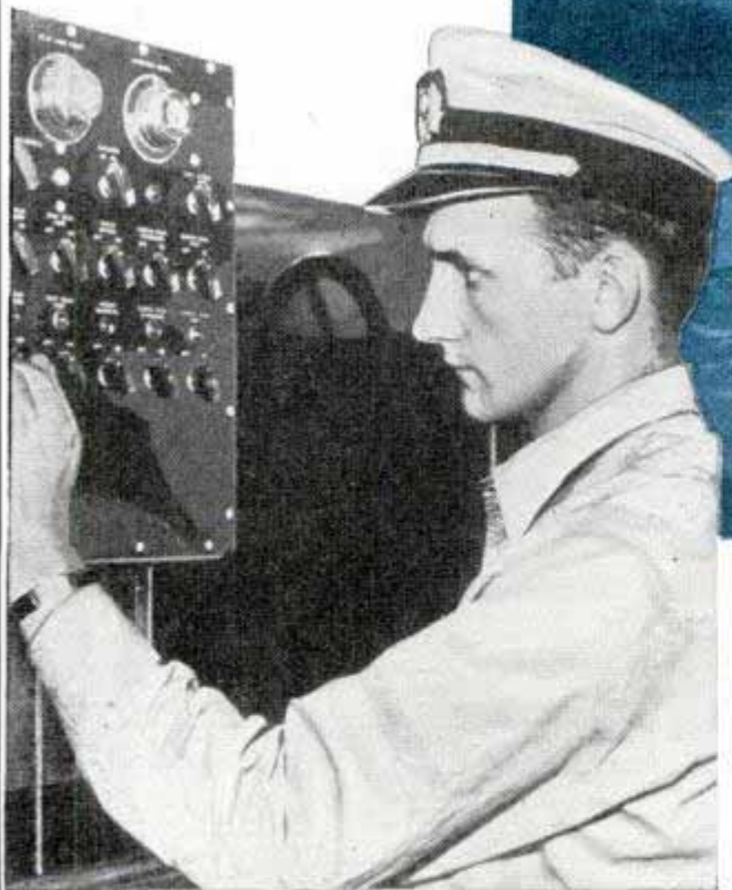
Cadet on passenger liner testing public-address system by which passengers and crew can be commanded during emergencies. Top, the "Tusitala," full-rigged sailing ship just after she had arrived in Honolulu from New York. She made the trip in eighty-four days
