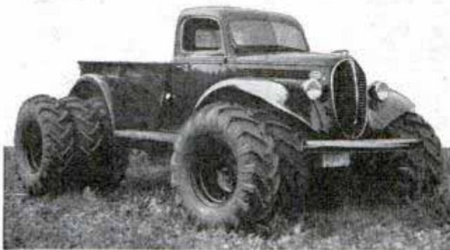
Ten huge tires on its ten driving wheels help this "marsh buggy" navigate almost impassable bog
