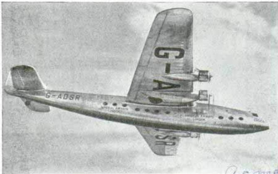
Twenty-one ton passenger-carrying landplane in flight. Note that undercarriage has been retracted into the engine nacelles
