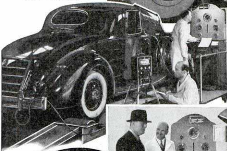
These instruments that reveal hidden troubles in the auto are part of a motor-measuring unit introduced recently
