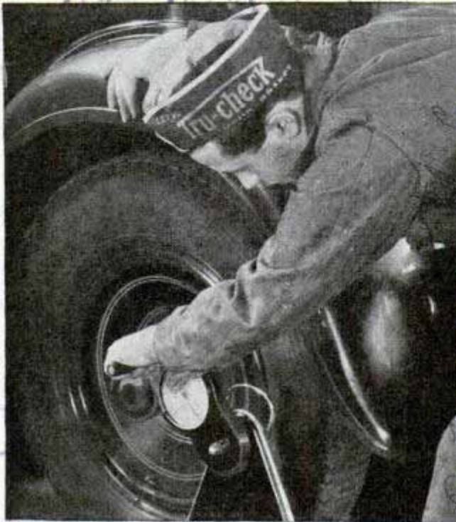
Taking a reading of the braking power of one automobile wheel with the portable tester
