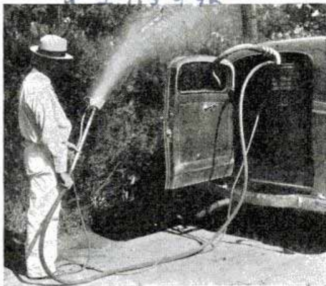
Exhaust gas in large hose blows insecticide in mist
