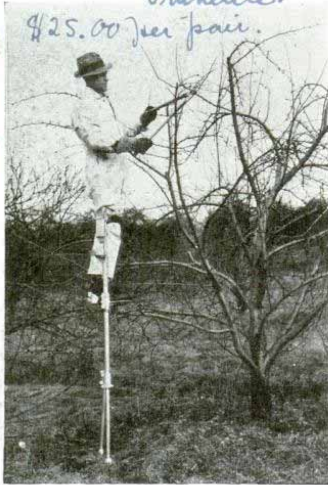
Orchard worker speeds his work by walking on aluminum stilts which are adjustable to various heights
