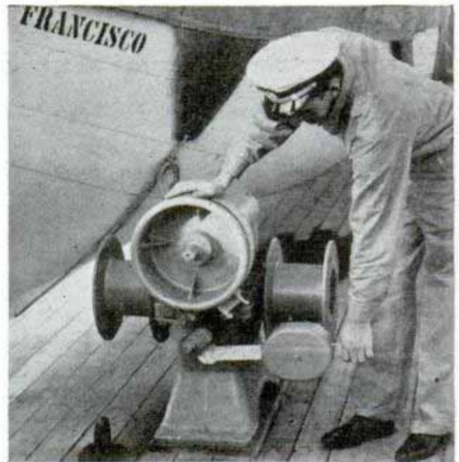
Gear and brake used for snubbing lifeboat as it is swung away from ship and lowered
