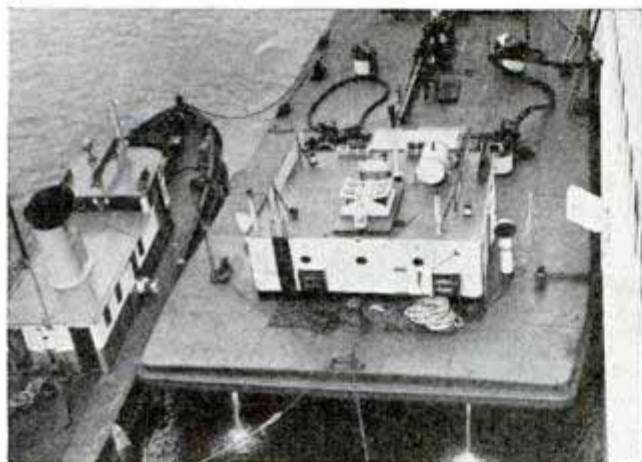
Servicing a liner. Water and half a dozen different oils and fuels are taken aboard as soon as liner docks
