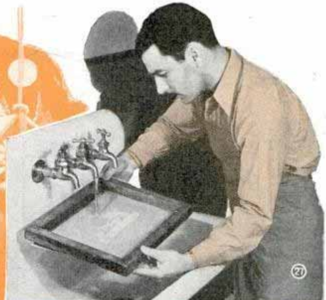
AFTER PRINTING, THE SCREEN IS HELD UNDER HOT WATER TO BRING OUT THE PICTURE-LEFT
