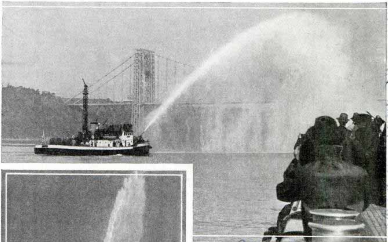
Two views of New York's newest fireboat undergoing trial tests. It can pump 20,000 gallons per minute
