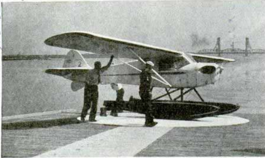
Seaplane on turntable after being lifted from water by the ramp. The plane can be taken from the water in thirty seconds
