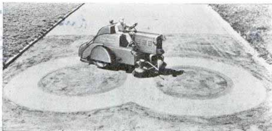
Sweeping a "figure eight" on a thirty-six foot pavement. A sprinkler and horizontal and vertical brushes do a thorough job of street cleaning
