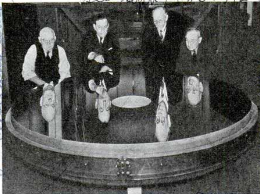
Here is the big mirror for the telescope after its bath in chromium and aluminum. The glass is twelve inches thick
