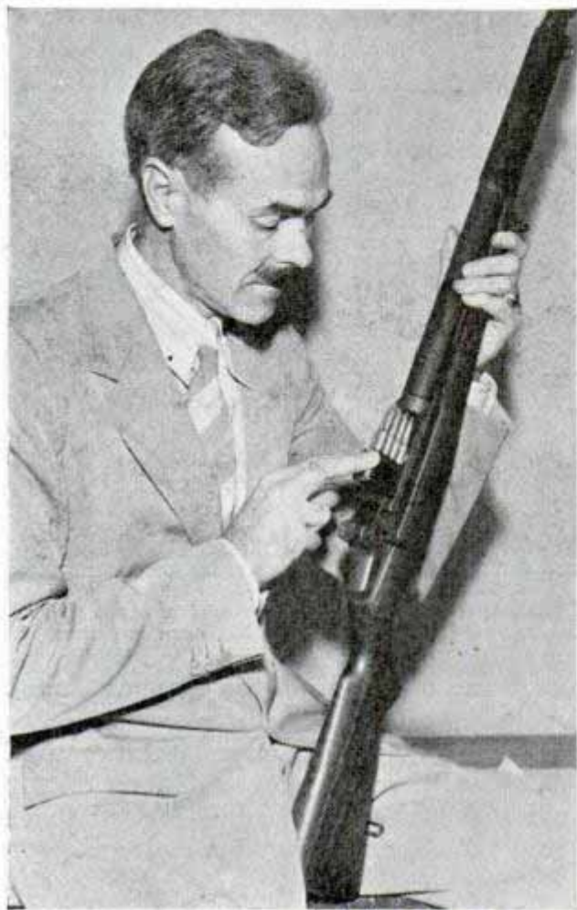
New army rifle holds eight cartridges, gas from explosion automatically throwing out empty shell
