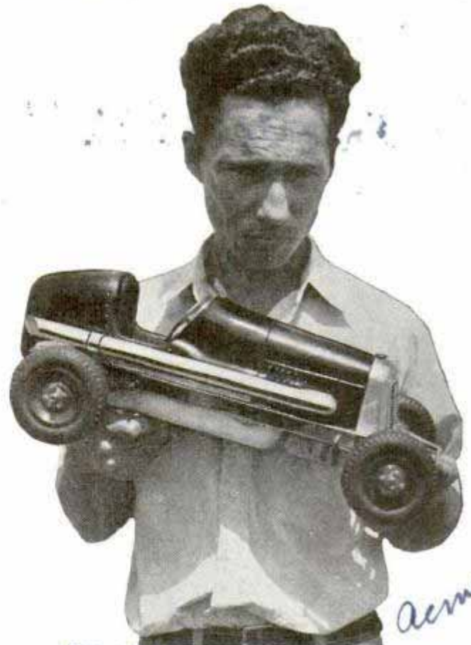
One-fifth horsepower motor gives this model racing car plenty of speed. Its tires came from ash trays
