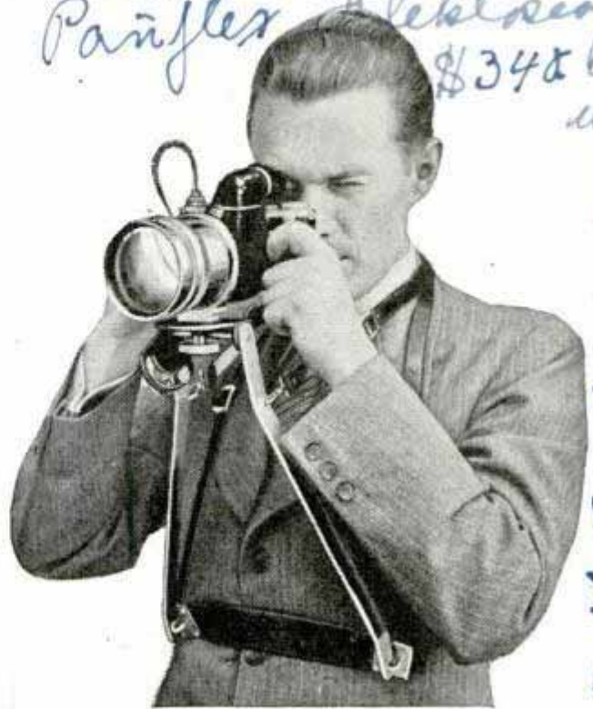
Using focuser-view finder on camera equipped with harness and metal supports
