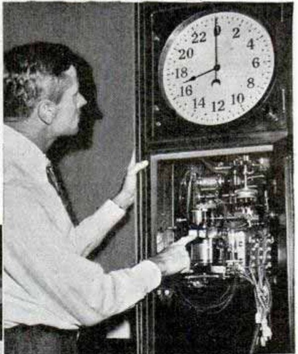
Left, astronomer at naval observatory operating "Zenith tube," which checks master clocks. It photographs stars crossing the zenith. Chronograph records time of stars' crossing. Above, master clock at observatory at exact noon, eastern standard time, but its face shows seventeen o'clock, which is Greenwich time. P. H. Tobleman points to mechanism that flashes long dash over radio to give correct time
