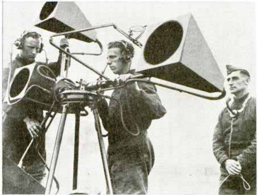
These are sentinels who will spread alarm if warplanes approach England. Sensitive "ears" amplify sound of motors and tell path of approach
