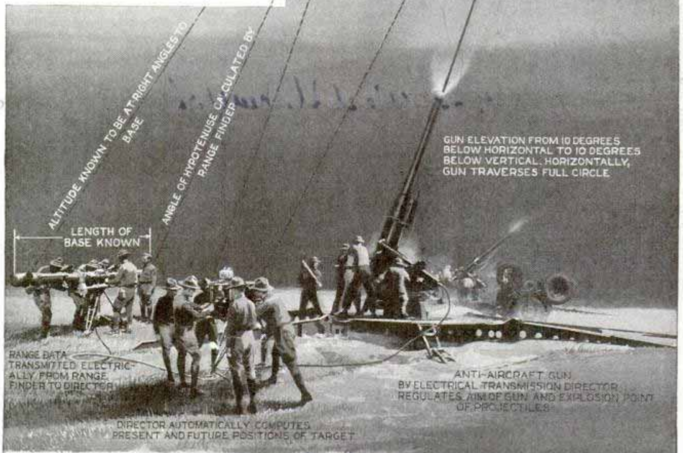
Camp Logan Here is how anti-aircraft guns are trained on an enemy bombing plane by range finder and director. Note circle showing effective shell pattern around the plane, at upper right
