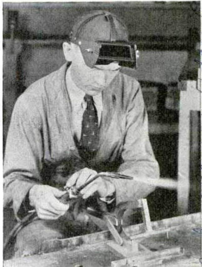
Eyeshield for the welder is designed to prevent fogging. Here it is in raised position
