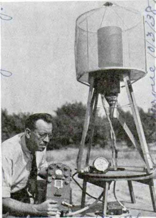
Compass needle of this direction-finder points "home" to radio station regardless of static
