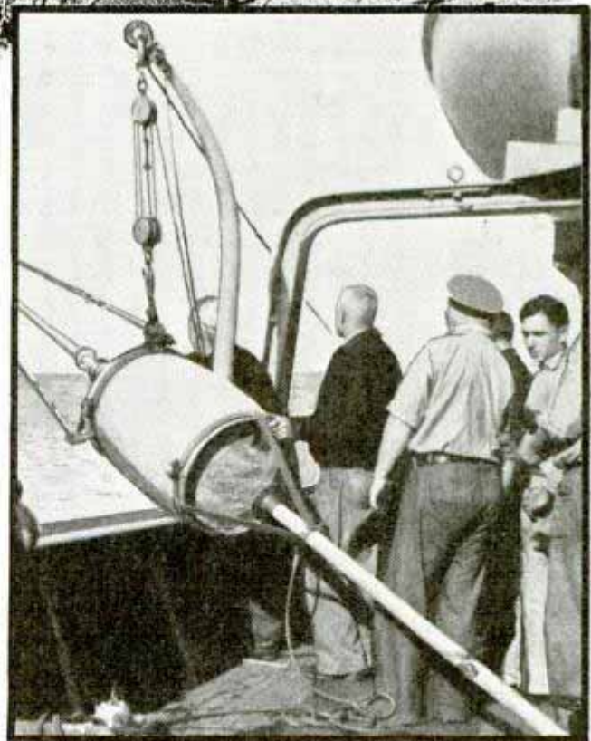
Here the crew is lowering a radio buoy into the ocean. It takes only a few minutes to drop the buoy or to remove it from the water, thus speeding up the survey work
