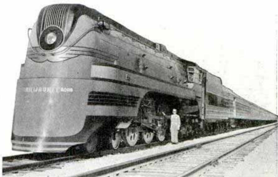
Eighty-four inch driving wheels of this powerful steam streamliner pull nine cars at 120 miles an hour. Notice longitudinal steel ribs of train
