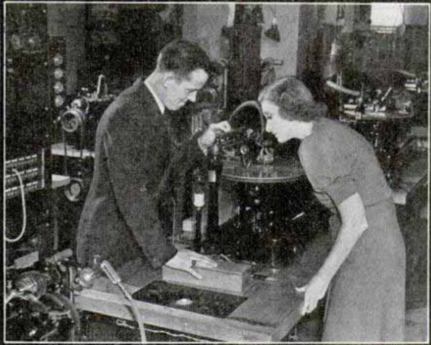
Top, control room where engineer manipulates "mixing panel" which blends volume and intensity of sound. Bottom, examining wax record under microscope
