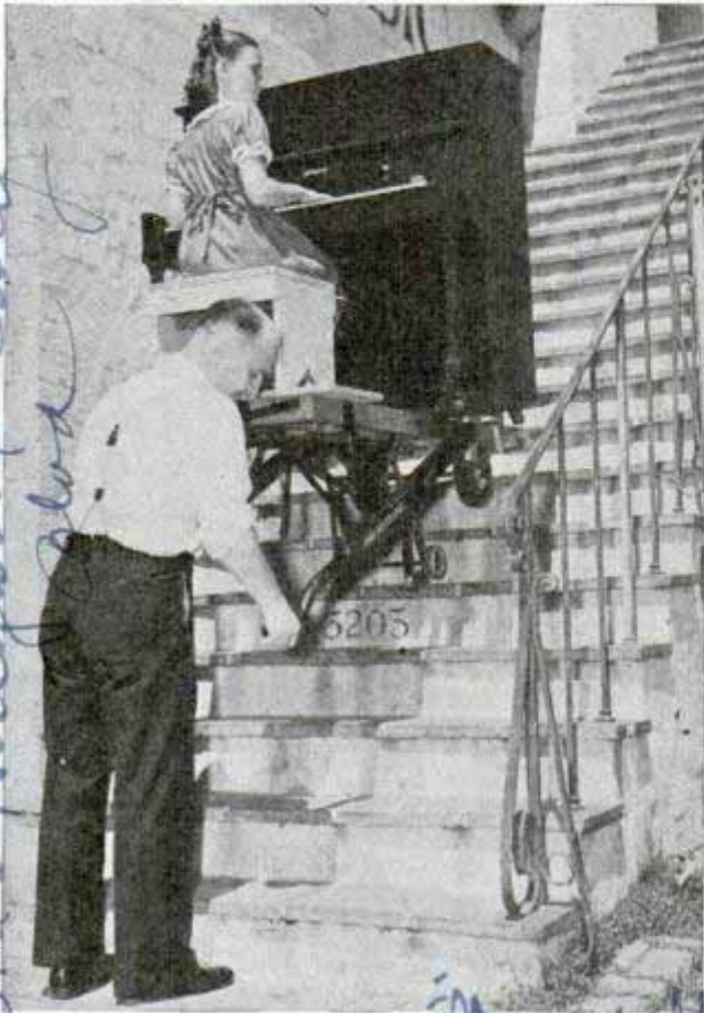
One man demonstrates how easy it is to move piano, bench and girl up stairs with "walking" truck
