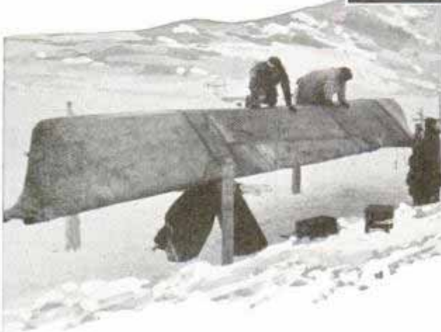
Right, oomiaks turned upside down to dry on racks made of whale ribs and driftwood. Bottom, sheathing oomiak with walrus hide
