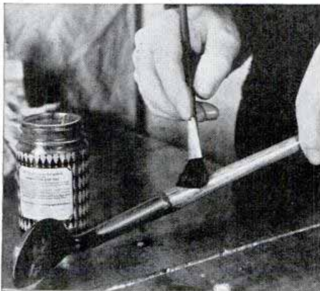
Sand and shellac wood shafts of your golf clubs each fall to prevent moisture from warping them
