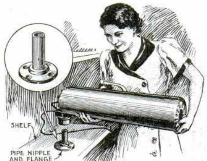
This holder supports the mangle securely at the same height as the washing machine
