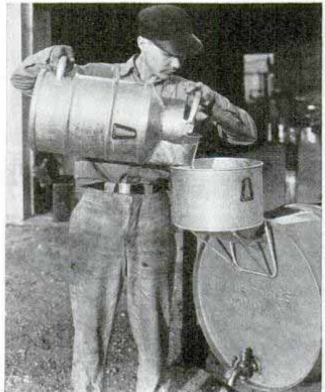
Its spout extending horizontally into end of barrel, this funnel is propped up by a special bracket
