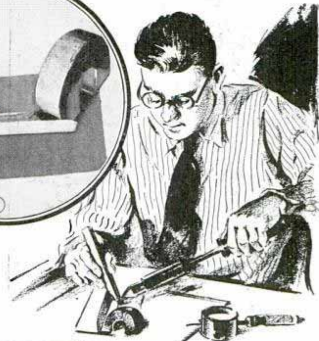
Clamping work when soldering
