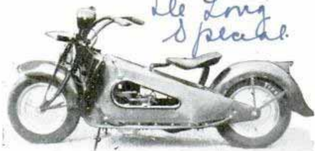
Frame, fenders and footboards of this motorcycle are of pressed metal, and wheels are aluminum disks
