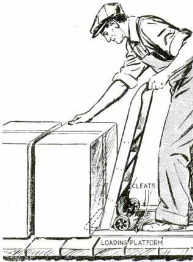
Hand-truck operators will welcome the installation of these cleats on the loading platform
