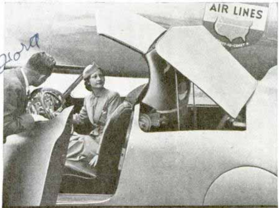
At touch of button on dashboard, the folding top disappears much as retractable landing gear of a plane vanishes into wing. At left may be seen the rudderlike tail, and below, the "pants" which turn with the front wheels
