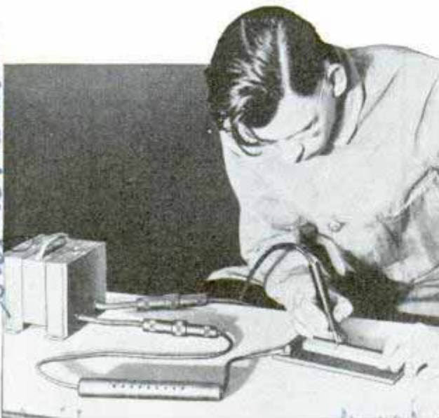
Etching a permanent identification mark on hard metal with the electric stylus
