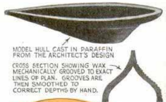
IMPROVING DESIGN BY USE OF MODELS AND TANK TESTS
