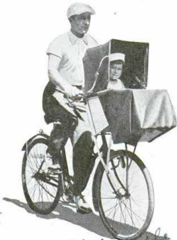
Seat built on handle bars has top for protection of the baby in bad weather
