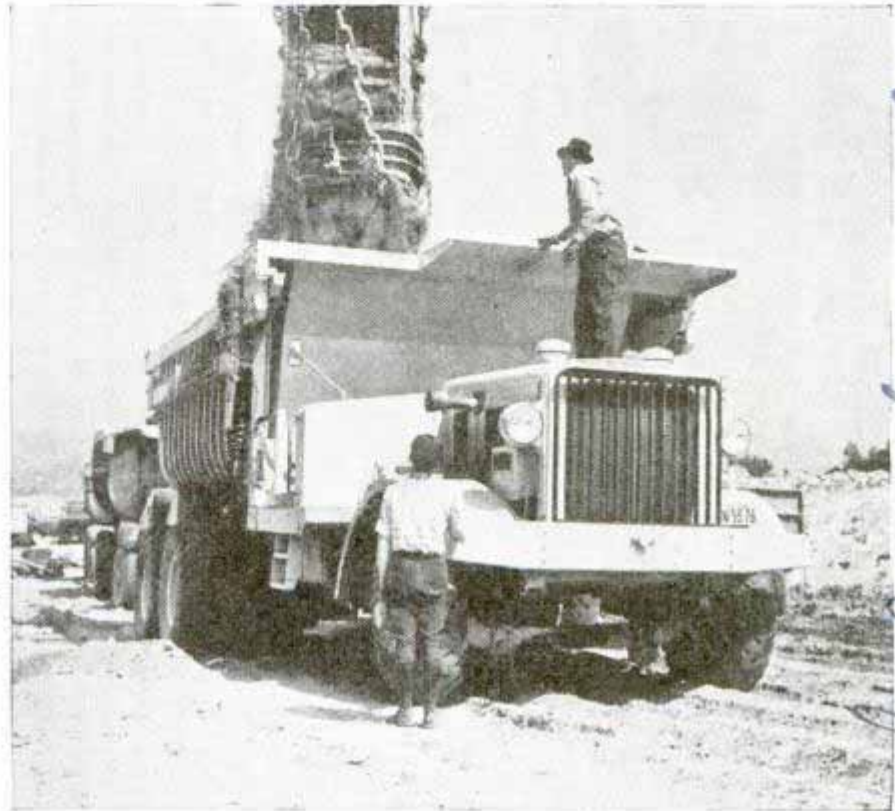
This tremendous materials truck has a capacity of forty-three yards and its Diesel engine is geared to four sets of triple drive wheels
