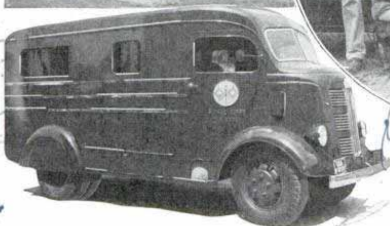
One window in side of army sound truck is high-fidelity loudspeaker. When officer addresses troops over mile range, towers with big loudspeaker horns are erected. Notice power outlets in truck wall, above
