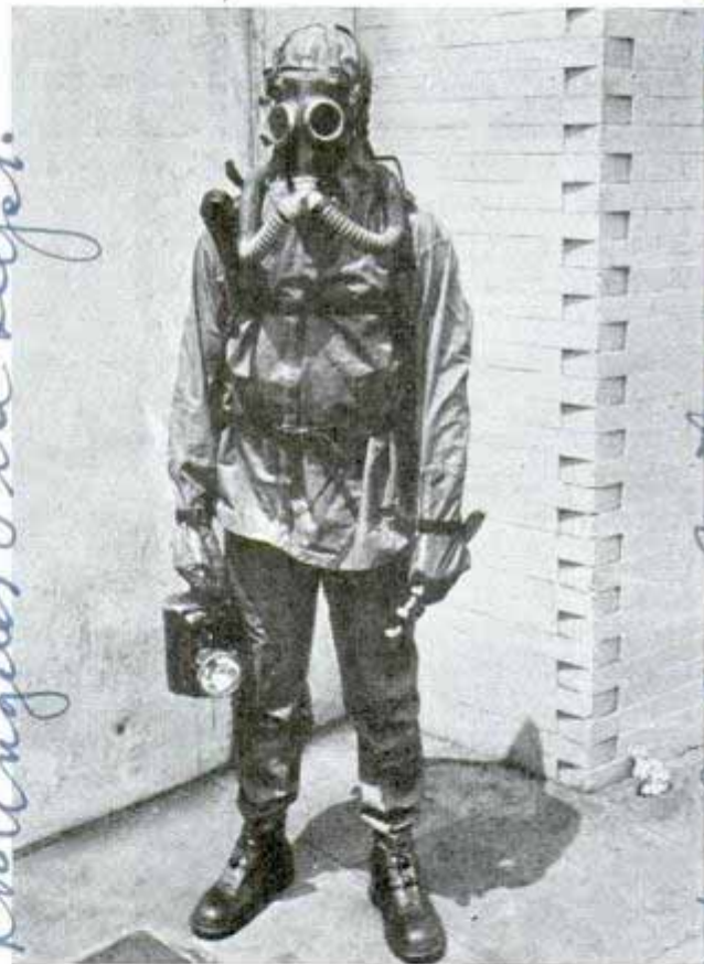
This suit not only protects face and lungs but keeps irritating gas from reaching any part of body
