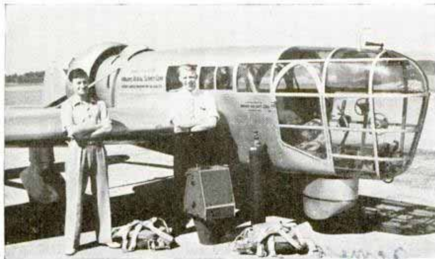
Latest aerial camera is shown on ground beside fast plane for which it was designed. Note plane's visibility
