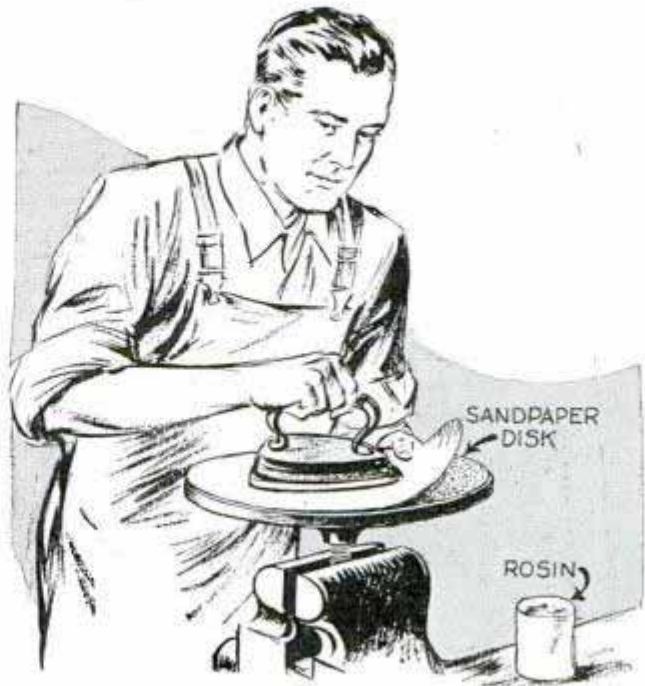
Hot iron applied to abrasive paper melts rosin, which sticks paper to sanding disk
