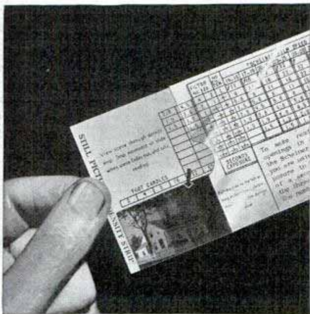
Sighting object through density strip at lower left, photographer takes reading when view is obscured
