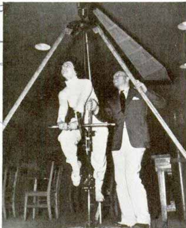
Rider pedals to drive the big airscrew, then pulls lever which the man is shown operating. This changes airscrew's pitch and the machine "flies"
