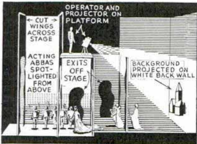
Above, building models to be photographed; below, method of projecting scene on backdrop of stage
