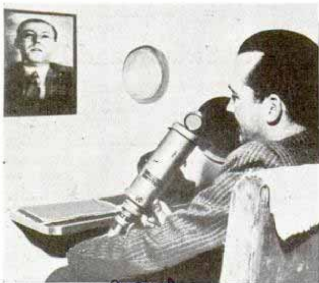
Distant speaker is seen in window on wall; round television "eye" sends picture of local operator
