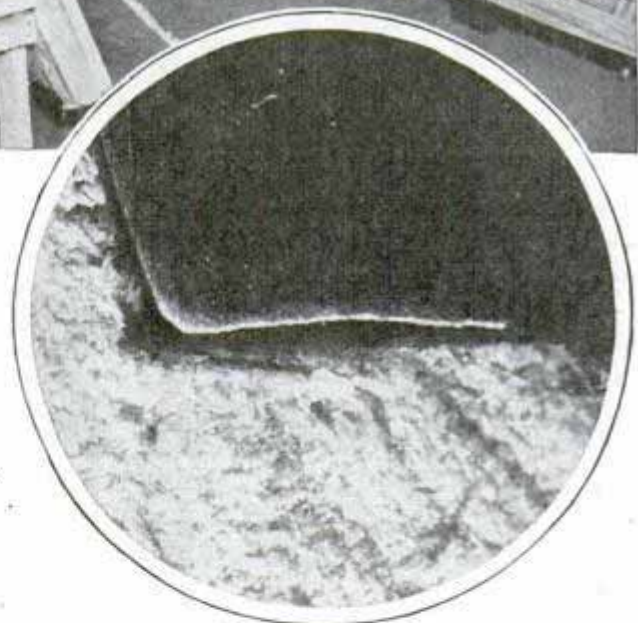
These pictures helped convict fire bugs. Top, papers attached to roof inside attic to help spread fire. Center, fire trail consisting of gasoline-soaked cotton. Bottom, photomicrograph showing how broken knife blade fits cuts in lath made by fire bug to provide ventilation
