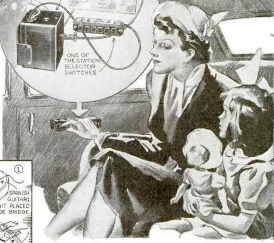
Above, motor-driven tuning unit, easily connected to any auto radio, provides 6-station push-button tuning from both front and rear seats. No tools are required to set push buttons for a new group of stations. Left, Fig. 1, suggested methods for using a contact-type microphone to reproduce vibrations of various musical instruments for amplification. Operating on the magnetic induction principle, it can be attached to all stringed instruments including a piano. Fig. 2 shows connection to volume control of a radio receiver, the set taking the place of special amplifier and speaker equipment. Below, compact cathode-ray oscilloscope in steel cabinet 4½ by 6½ by 8 in.; employs a 1-in. screen RCA 913 tube with 6X5 rectifier. Right, multi-tap plug-in switch made with tube socket
