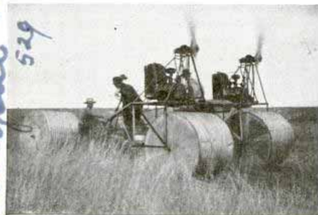
Twin propellers turned by automobile engines drive this "drum-wheeled buggy" over southern marshes
