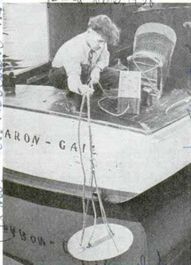
Dropping the metal locator from stern of power boat, the operator watches record made on meter box
