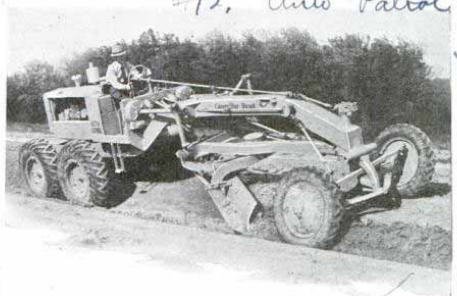
Here is the big road grader, at work on a typical job. The blade can be turned completely around for working in reverse gear
