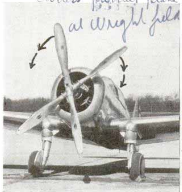
More power and less torque is result of single engine driving twin propellers in opposite directions
