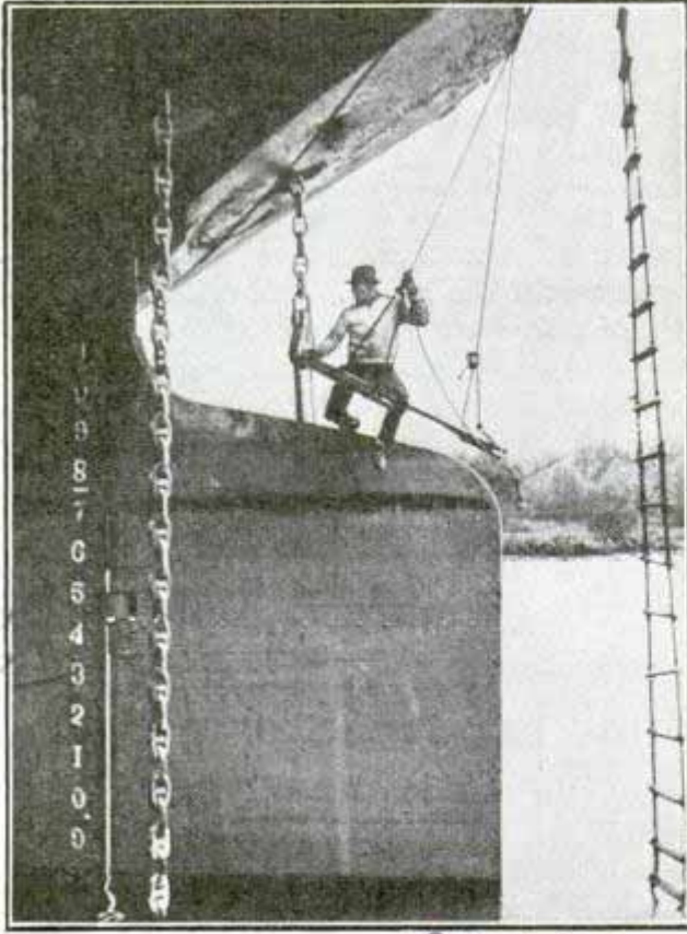
The rudder of this lake freighter is twenty feet high and ten feet wide. Top tug assisting a lake freighter up the Cuyahoga river at Cleveland.
