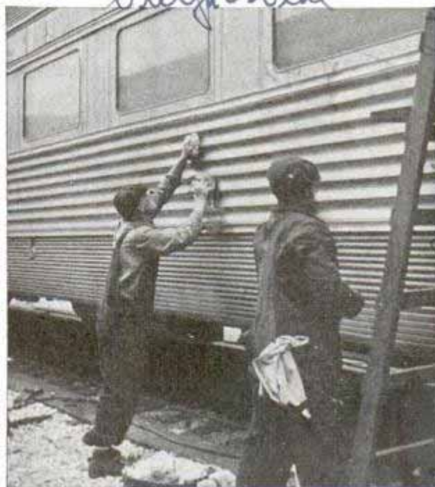
Dressing a streamliner in transparent film which preserves shiny appearance of metal
