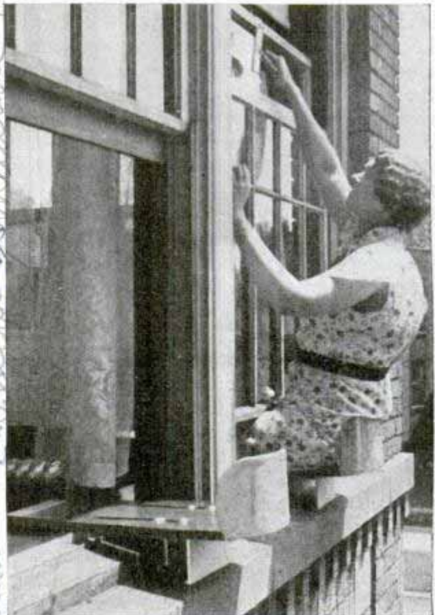
Two views of the window washer's safety seat for use in home or office building
