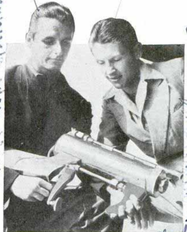
Compressed-air submarine gun shoots a brass dart and can kill a fish at fifty feet on the ocean bottom
