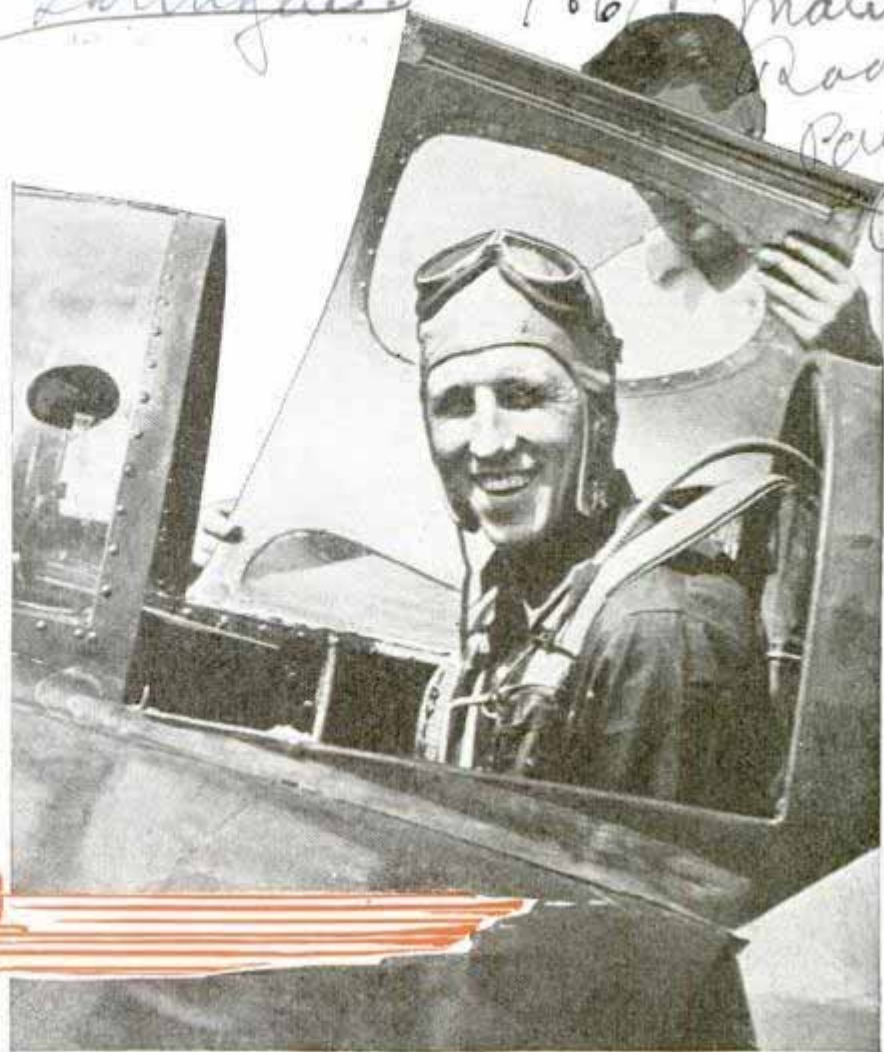
Top, closing cockpit hatch which completes streamlining of racing plane. Hole in transparent cowling enables pilot to signal the starter. Bottom, putting on parachute before testing new speed plane
