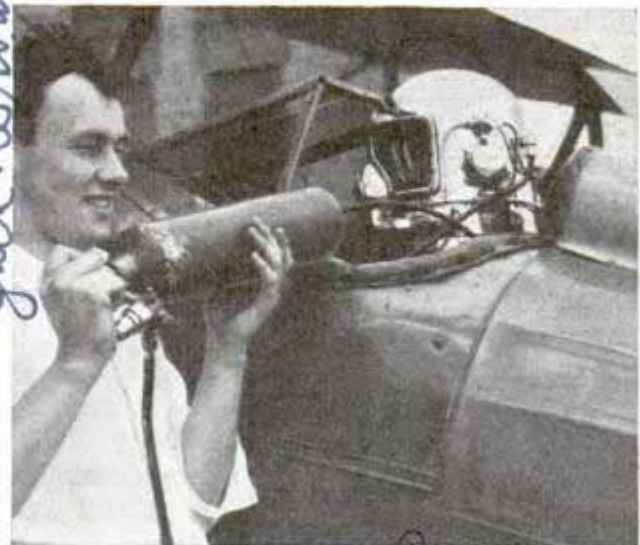
Putting oxygen bottle into cockpit of plane before altitude flight. Pilot is wearing a diver's helmet
