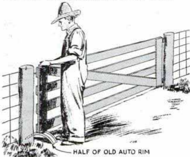
HALF OF OLD AUTO RIM Weight at free end of gate supported on wheel rim when closed
