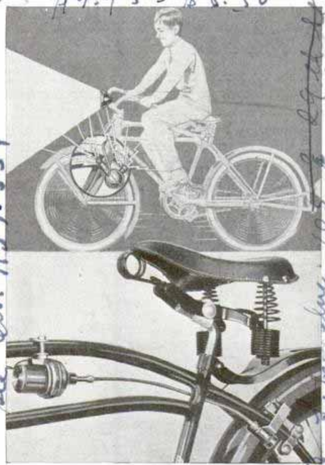
Bicycle lamp generator with remote drive can be mounted to take power from front or rear wheel
