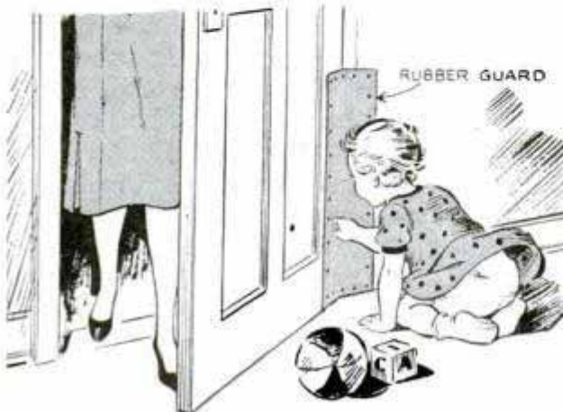
A small child cannot stick its finger in crack between door and casing if this guard is used
