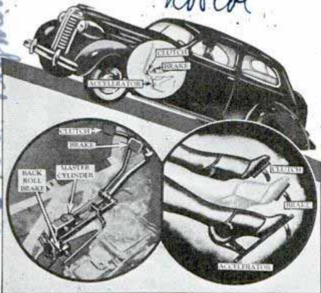
Drawings show location of backroll brake mechanism; it operates so long as clutch is depressed
