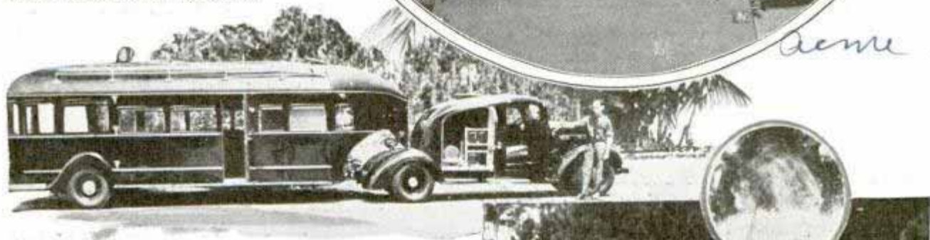
Top, patient in his "iron lung" smiles into mirror in which he sees view through rear observation window of trailer. Left, the air-conditioned trailer which has kitchen equipment. Right, periscope mirror on top
