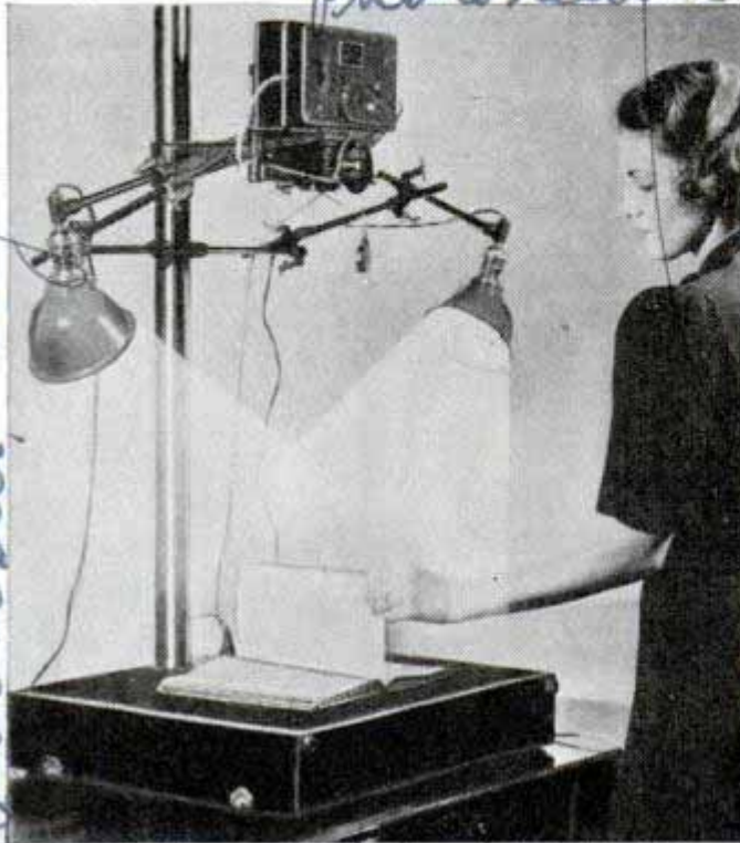
Simple photo-recording machine in operation, putting book pages on tiny film
