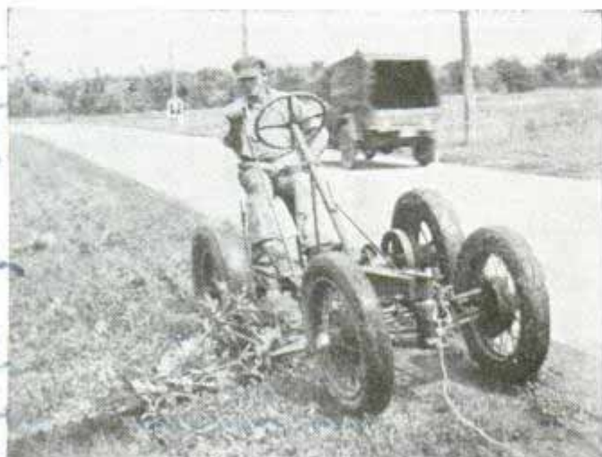
Hauled by truck which stays on pavement, driver of this roadside mower can steer around obstacles
