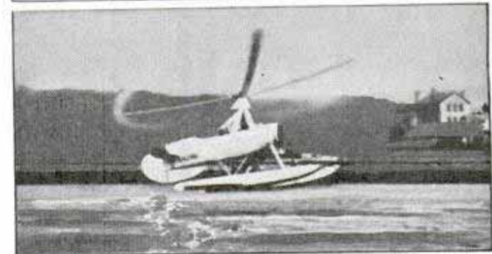
German helicopter, above, propelled by engine-driven rotors. Below, autogiro equipped with floats
