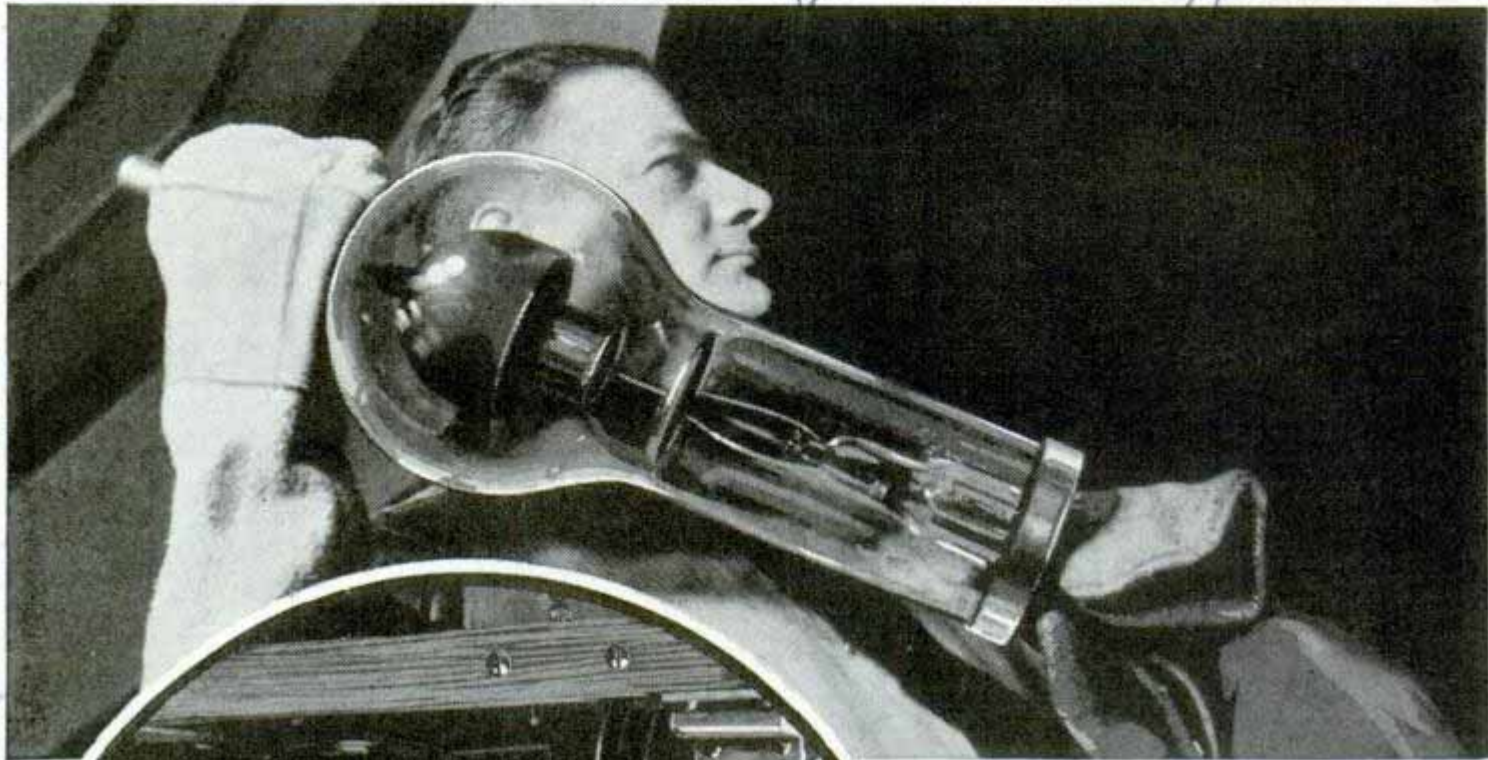
Top, handling big rectifier tube with asbestos gloves. Bottom, station engineer placing emergency clip lead on control apparatus at WEAF
