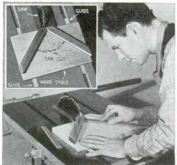
This jig will save considerable time when mitering moldings and other small work
