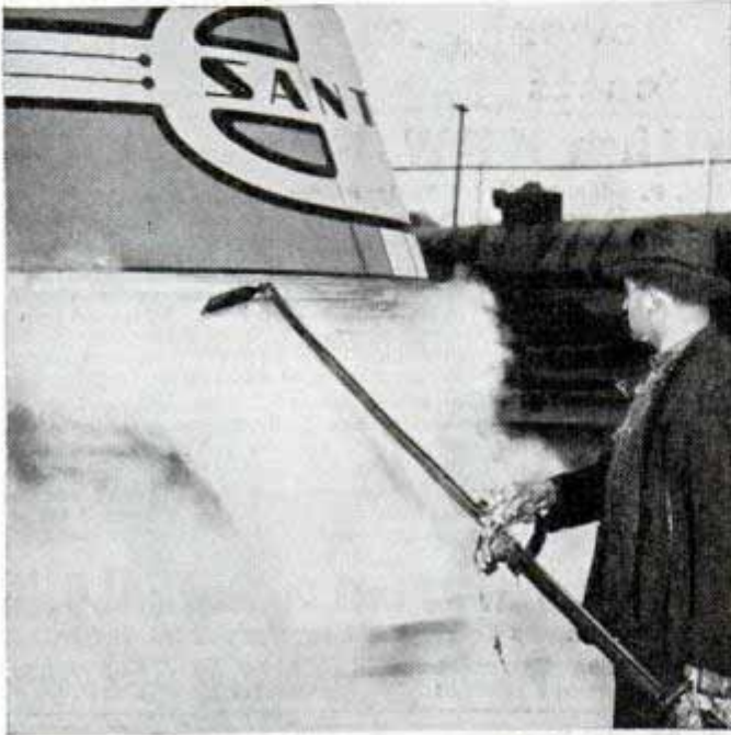
Scrubbing front of streamliner with a mixture of steam and soap solution
