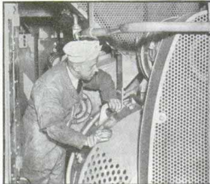
Fuel-hose connection and gauge on power unit. Right, inspecting 750-volt generator coupled to one of Diesels. Top, unloading Diesel piston and connecting rod for overhaul
