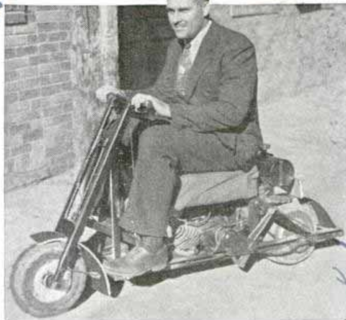
Half-horsepower motor that drives this homemade bicycle used to run a washing machine
