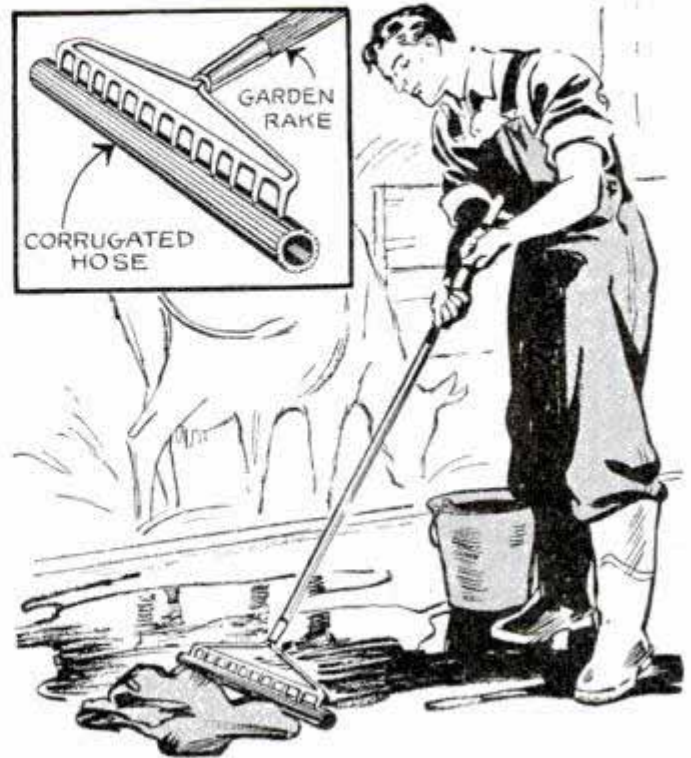
Squeegee to clean floor of dairy barn made by impaling garden hose on rake teeth
