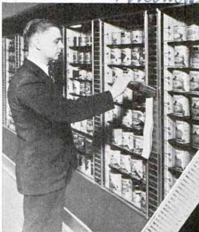
Pressing arm of magazine into various slots, as at left, customer obtains printed shopping list, below. Cashier totals bill and clerk fills order
