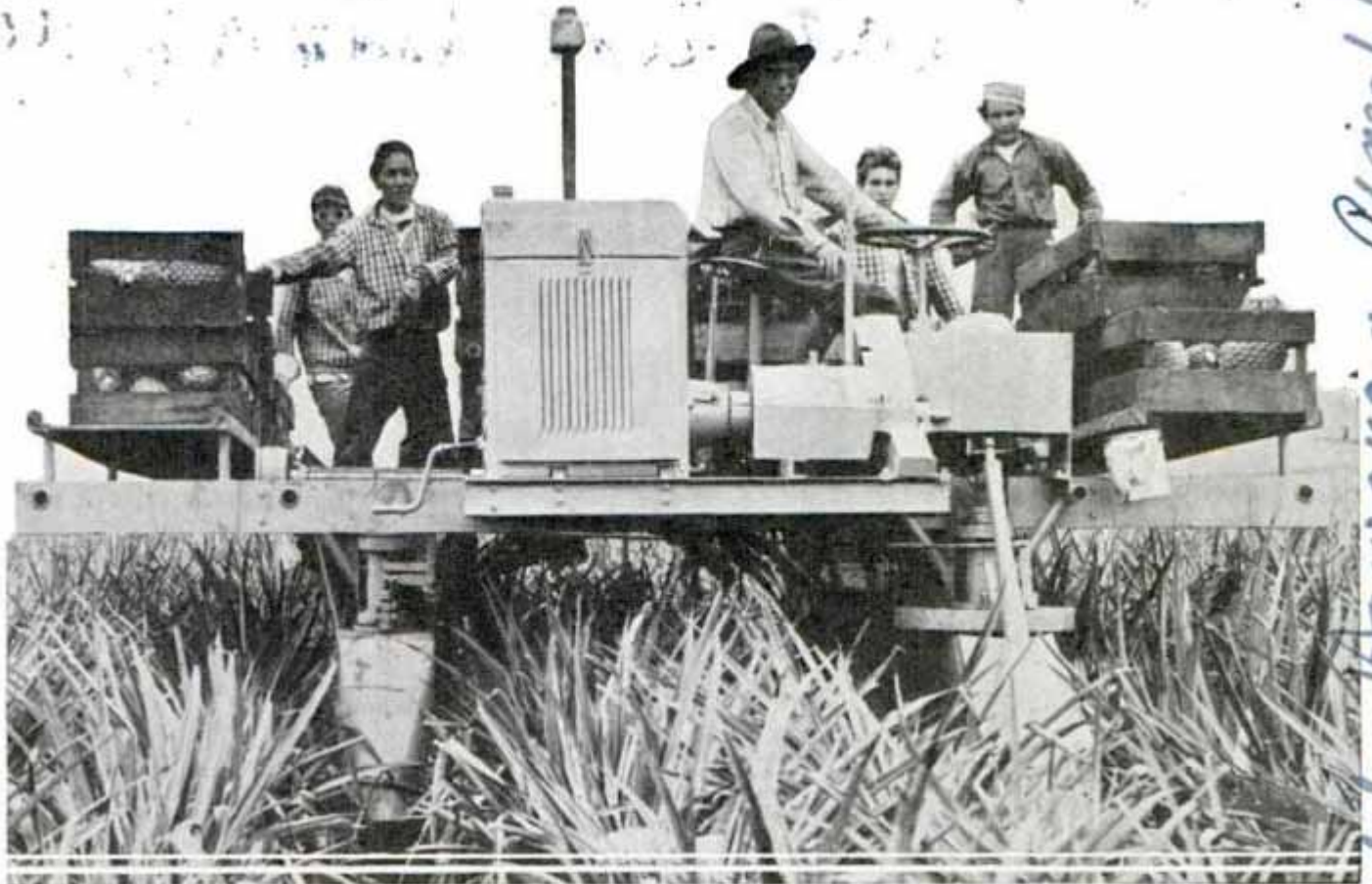
Strange-looking vehicle in pineapple field straddles the plants. As shown, the driver sits sidewise to watch loading and the path his machine is to follow. The vehicle speeds harvesting
