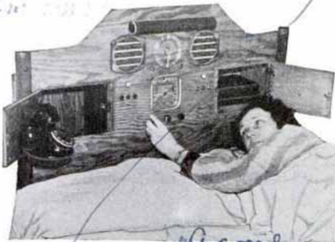
Radio, alarm clock, telephone, loudspeaker communication system and heat controls are wired to bed
