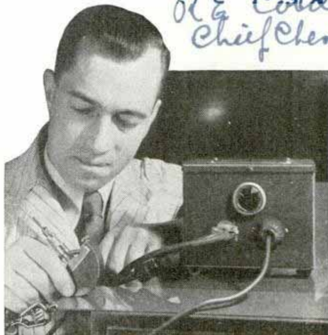
Demonstrating how the paint-testing instrument is applied to metal surfaces
