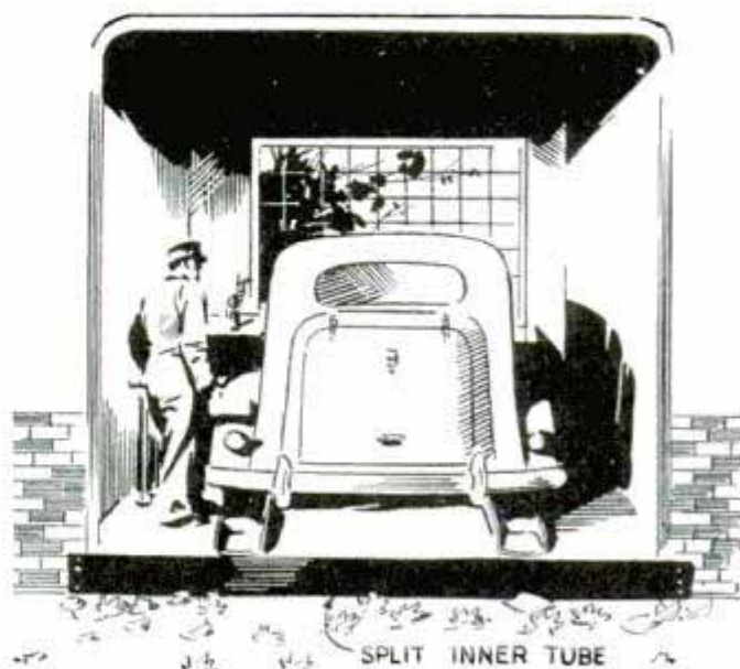
Split inner tube stretched across doorway of grease pit checks debris blowing along on ground
