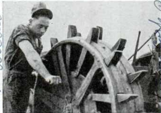
Top, cranking the retractable lugs out of sight within rim; below, the lugs fully extended
