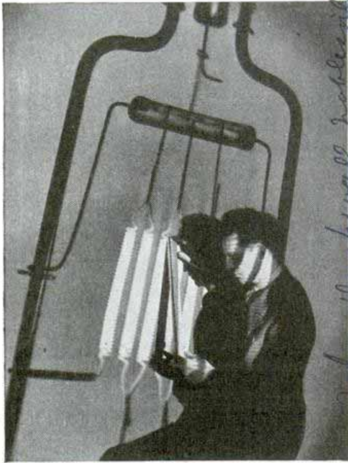
Measuring expansion of lighted filament with ruler as enlarged image is projected in laboratory
