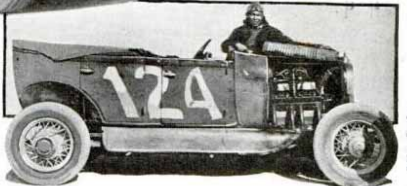
Driver at top is tightening water hose on his "flat-head" high-compression engine. Center, modified roadster with special racing engine. Bottom, touring car, dilapidated in appearance, but equipped with a racing engine which gives it a speed of 100 miles an hour
