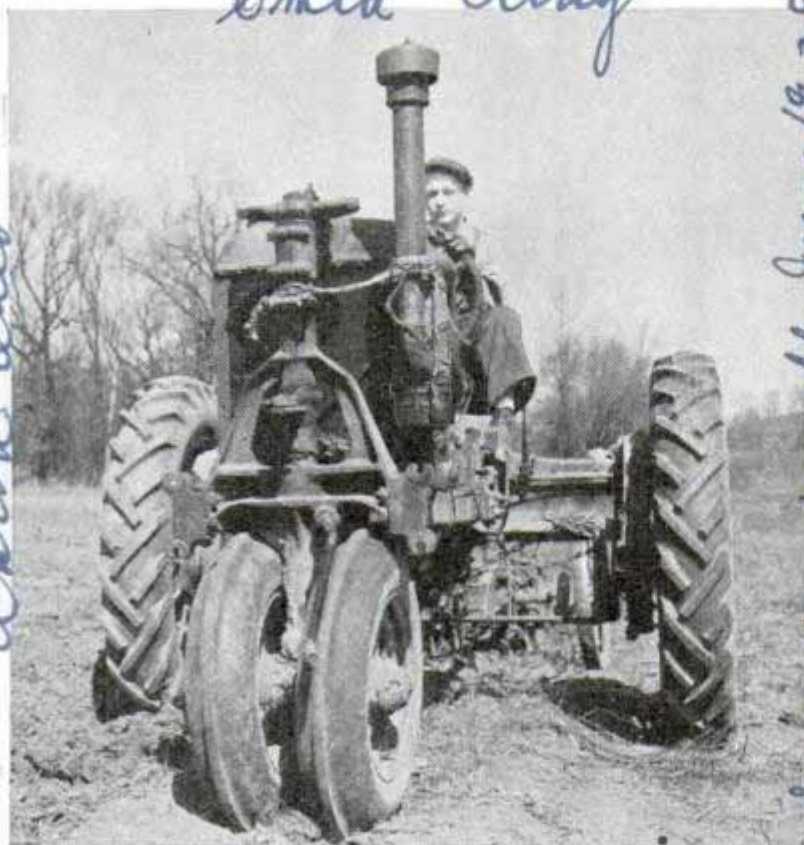
Inch-deep rubber flange on front tires of tractor prevents side-slipping and improves steering. Tires do not pick up mud
