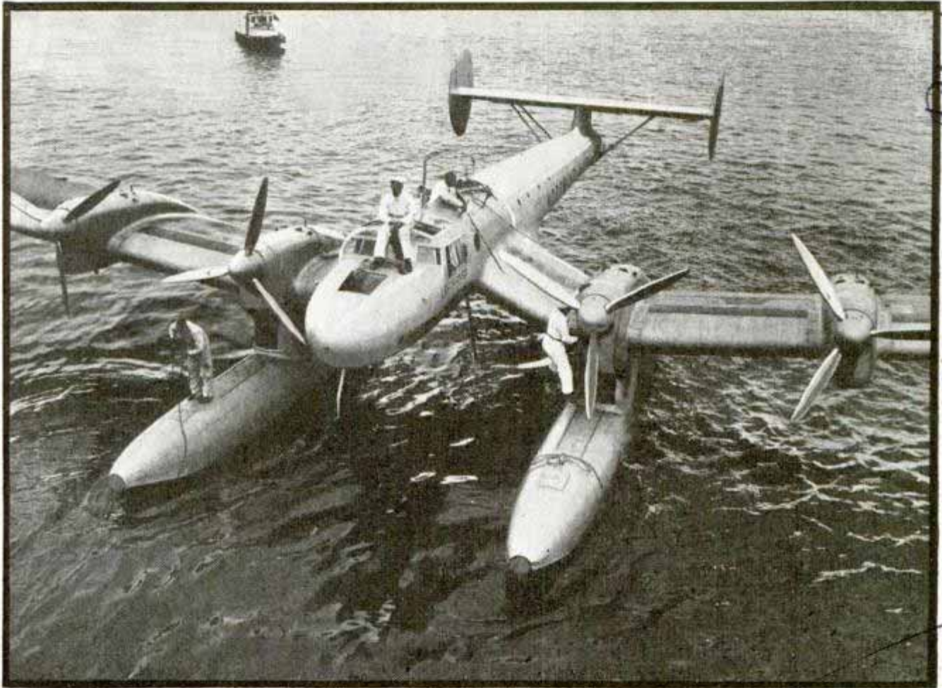
The "Nordmeer" waiting to be hoisted on board catapult ship after transatlantic crossing. This seaplane is equipped with four 600-horsepower Diesel engines
