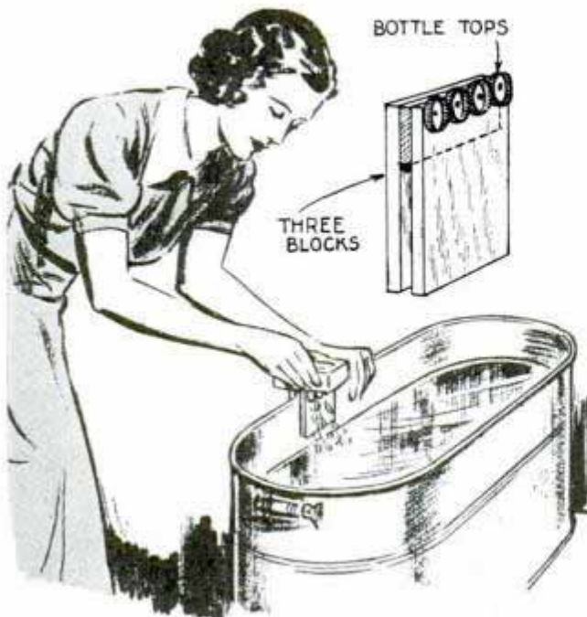
Pulling a bar of laundry soap over the edges of the bottle caps shaves off small pieces
