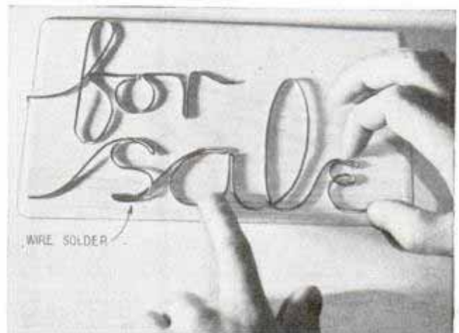
Using wire solder to form lettering or writing is especially handy in photographic work
