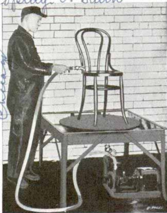
Excess stain drains from chair to perforated circular drip pan and flows back to tank for use again
