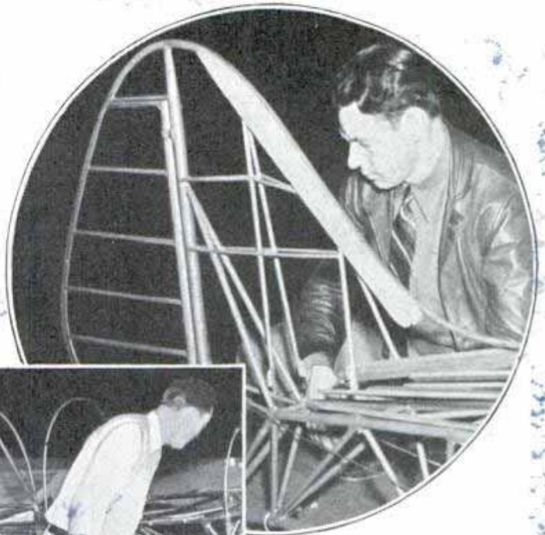
Top, tail assembly; bottom, the supercharged 400-horsepower motor of the "SK-4." Left, skeleton of the racer, showing round oil reservoir in tail and gasoline tank amidships
