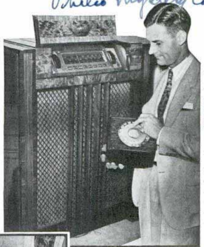
The radio receiver, above, can be operated from any room in the home with the aid of the remote-control box which is not connected by wires or in any other physical way with the receiver
