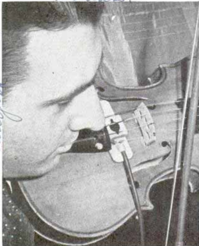
Wire from contact microphone on violin carries sound through amplifier to deaf person's earphones
