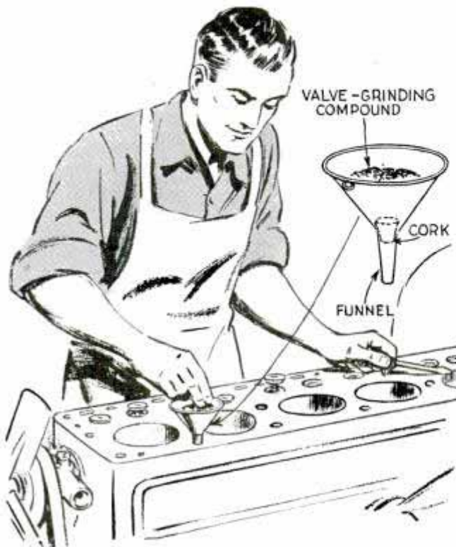
A small funnel with a cork in the spout keeps valve-grinding compound conveniently at hand
