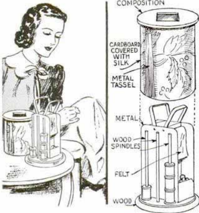
Lifting off the cover of this ornamental lantern exposes a convenient sewing basket
