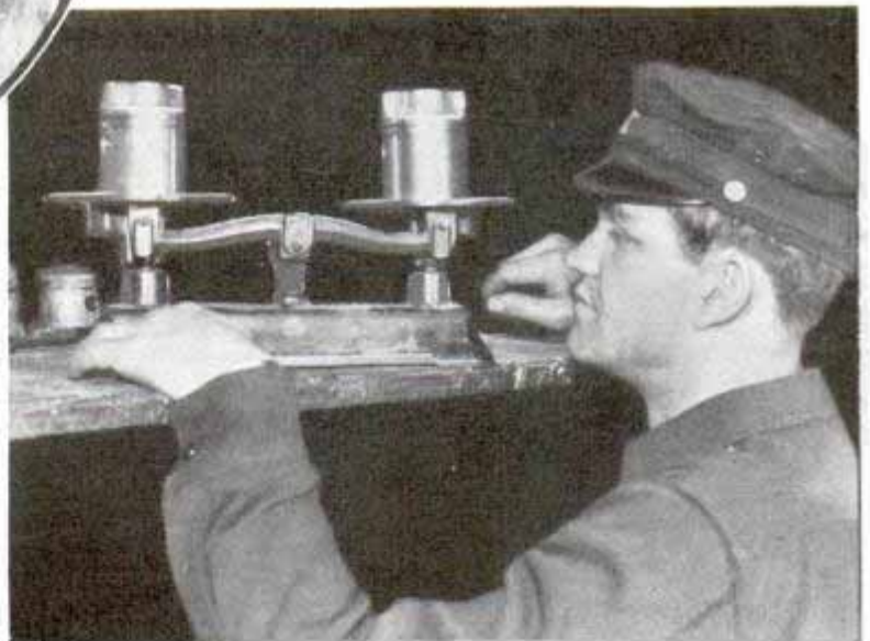
Top, various propellers used during season of racing. Circle, inspecting hydroplane bottom. Below, balancing pistons on scales
