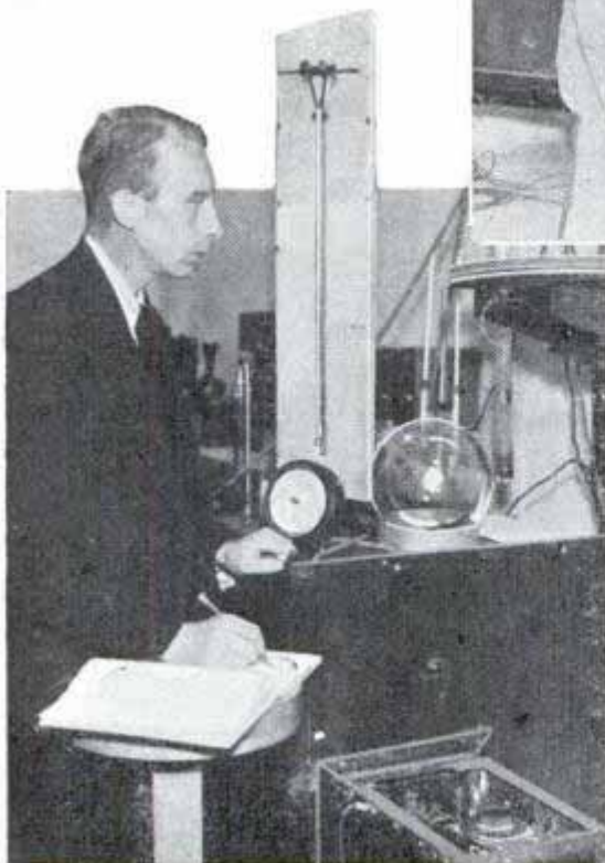
Above, taking readings of ultrasonic waves projected into chamber filled with nitrogen
