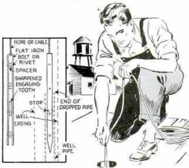
Long length of pipe dropped into deep well quickly removed with this "fishing" tool
