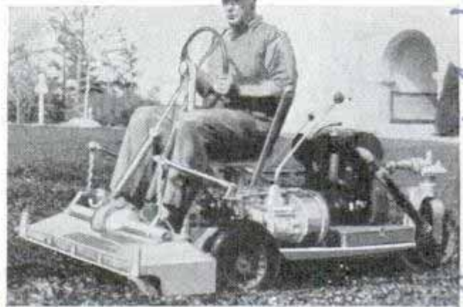
Cutter at front of power mower is lifted by pedal controls to avoid rocks and obstacles in grass
