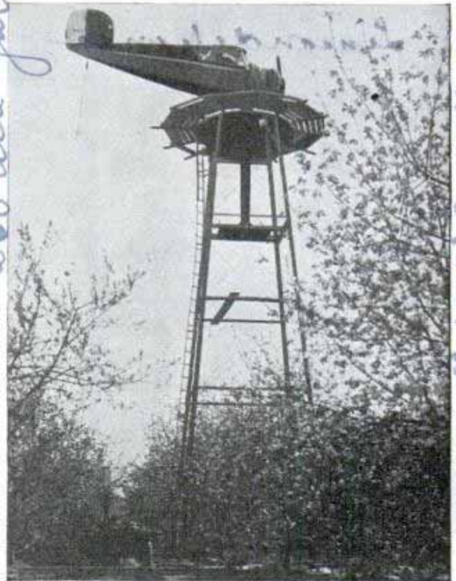
Rotating slowly on top of tower, this plane—once worth $50,000—fans air to prevent frost in orchard
