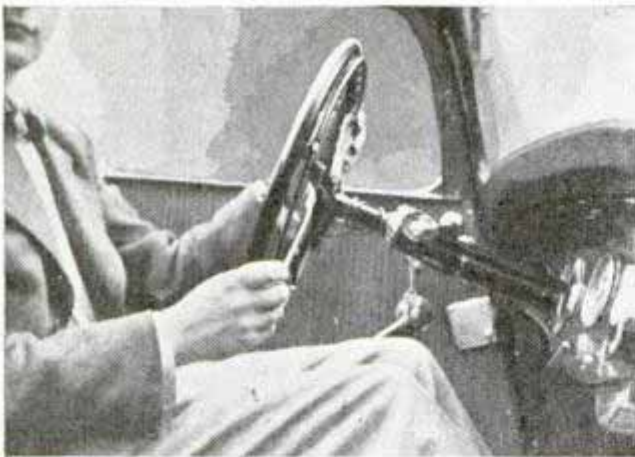
Small ring is held away from steering wheel by springs, and sounds horn if driver's grip relaxes
