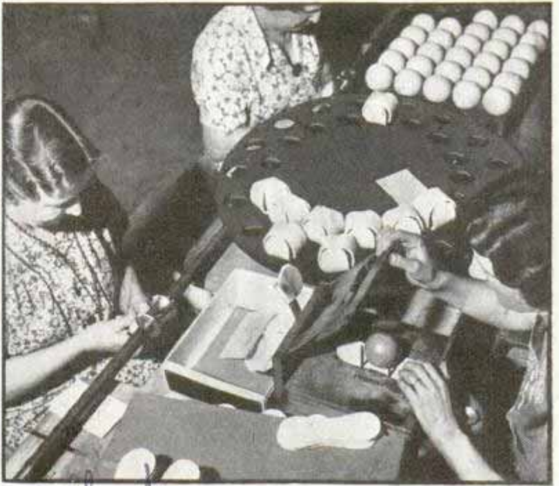
Above, a final stage in manufacture of tennis balls; putting on outer covering, sewing and "spooling"—ironing the seams down. Below, at right, the beginning of a tennis racket. Here a factory worker is bending strips of ash into shape. Rackets must conform to high standards as to weight, balance and stress
