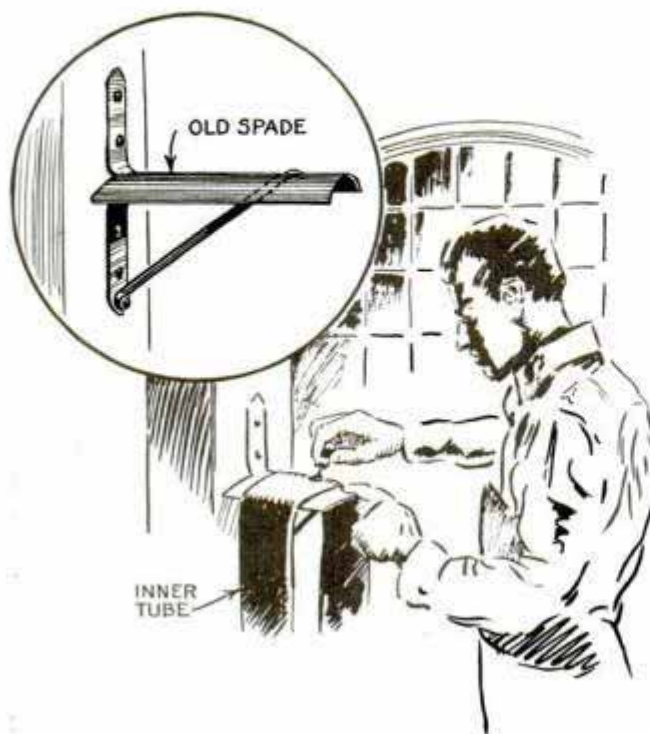
Old spade screwed to wall or bench provides handy support for inner tube while patching it
