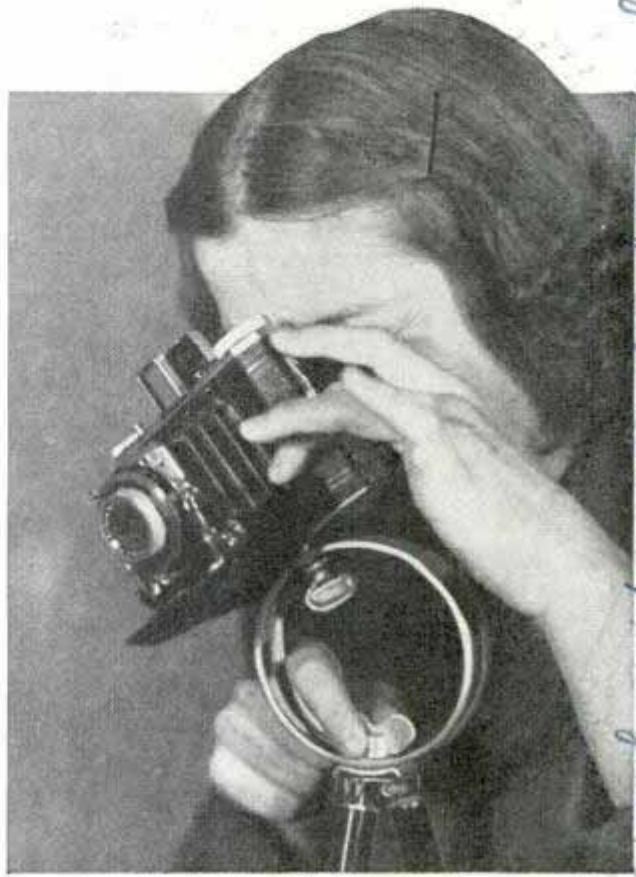
Adjustment of two thumbscrews on slotted ring allows camera to be mounted on tripod at any angle
