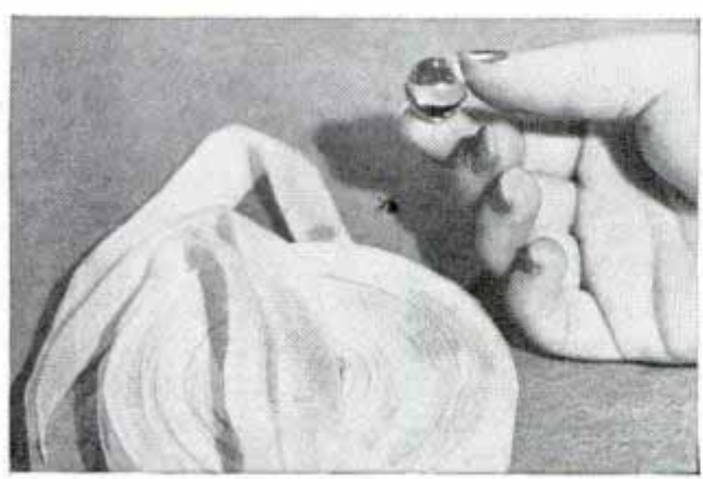
Insulating tape is woven of glass thread so fine a strand 150 miles long is drawn from small marble
