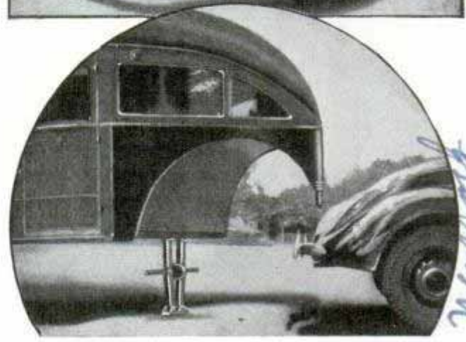
Two views of electric jack in use. Top, raising auto. Bottom, supporting trailer
