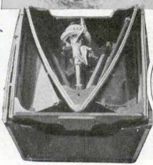
Top, two fishermen take separate sections and fish by themselves, then bring the boat together again. Below, the three-piece boat "nested" for transportation by auto or plane and afloat with outboard motor
