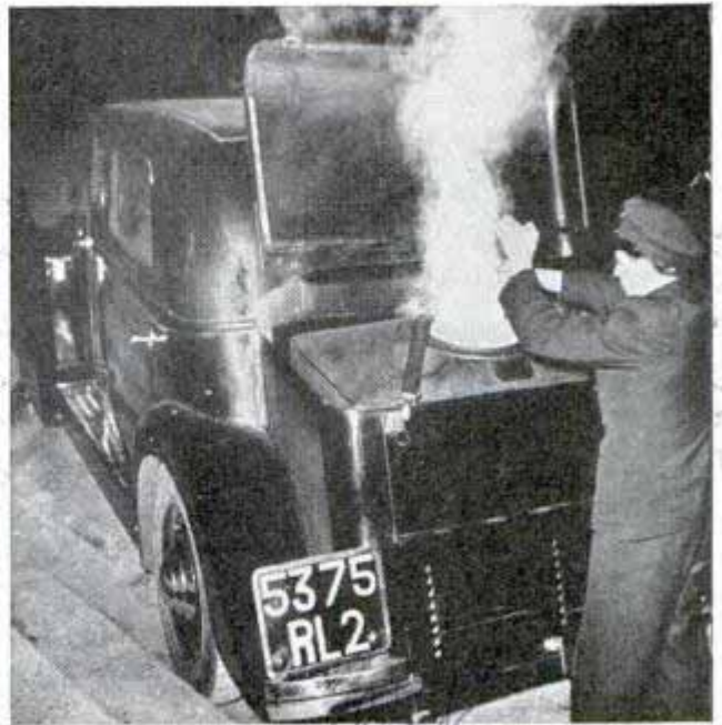
Boiler rack is mounted in place of trunk on rear of this economical wood-burning French automobile
