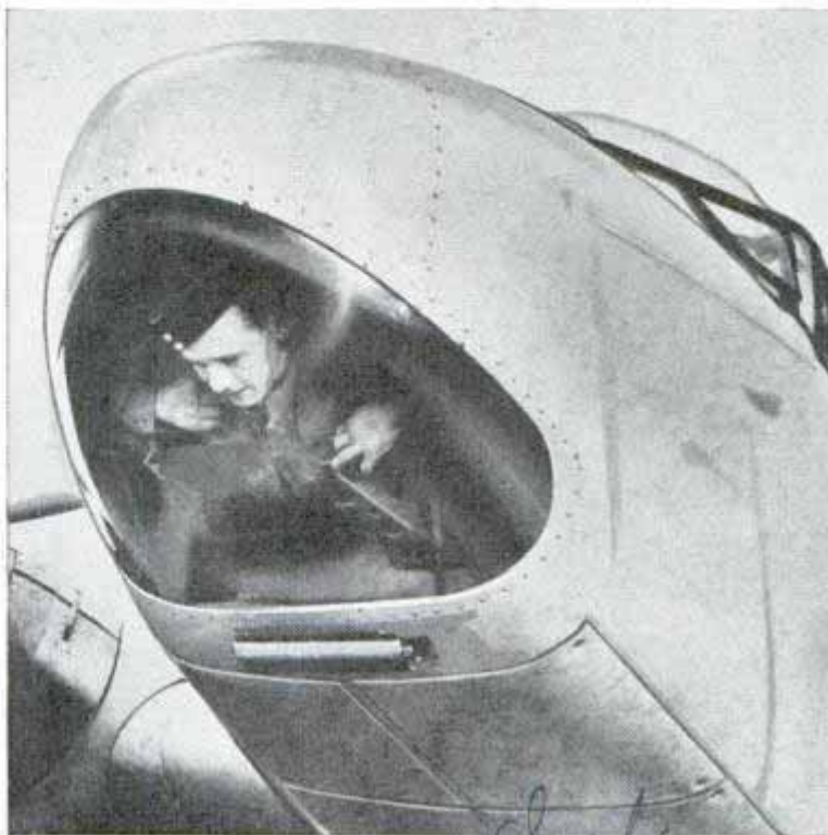
Lying prone in nose of British training craft, bomb operator sights his target through a window in the floor
