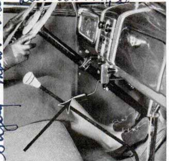
Arrow points to accelerator which leaves right foot free to operate brake pedal
