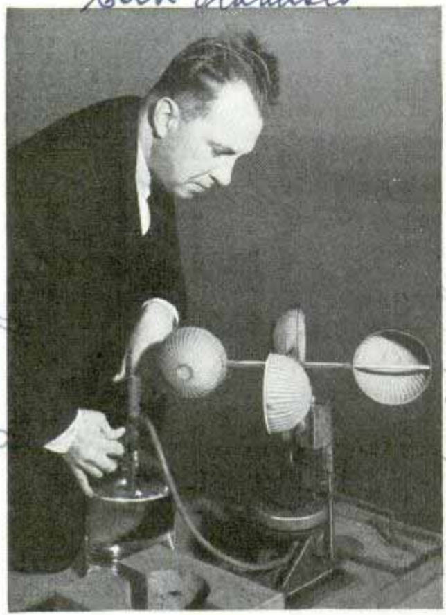
Four-cup fan pumps sample of air into bottle of distilled water for analysis of elements
