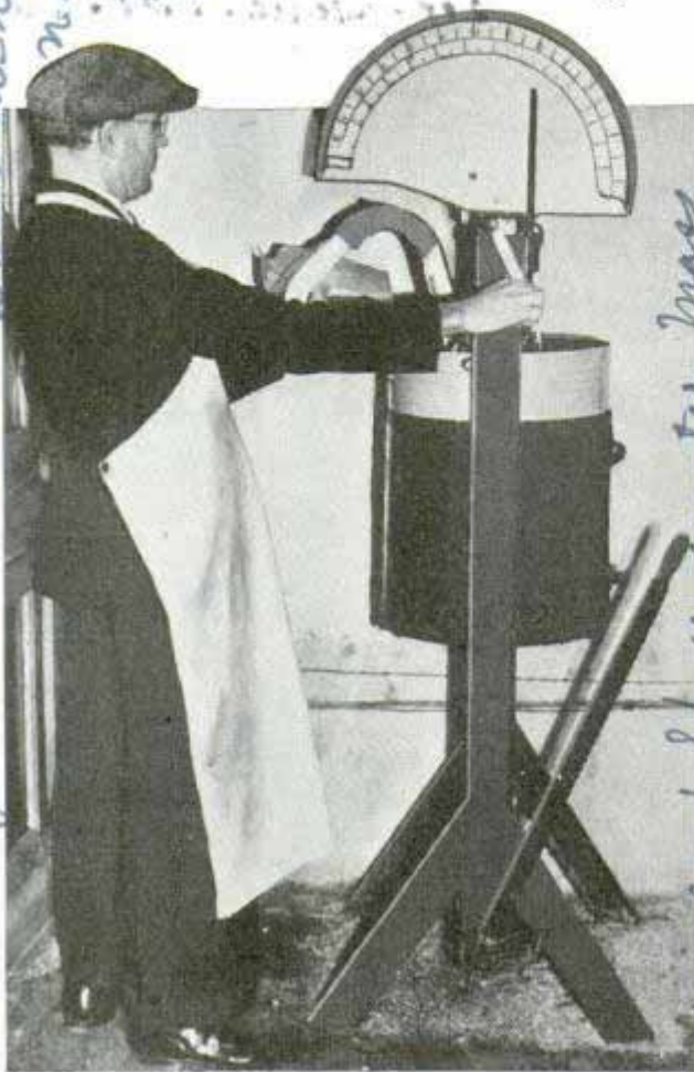
Cranking out lard to the penny's worth with dispenser which replaces old scoop-and-weigh method
