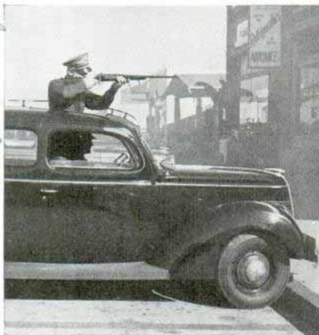
Police officer illustrates how sliding roof panel permits him to stand up and take aim at fugitive
