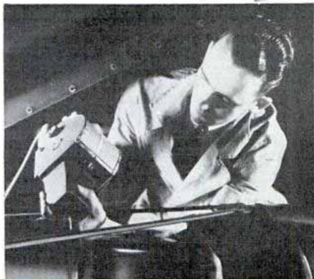
Tracing vibrations in automobile by means of small deflection indicator
