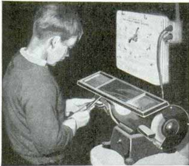
Providing eye safety against flying particles, this shield also illuminates the work
