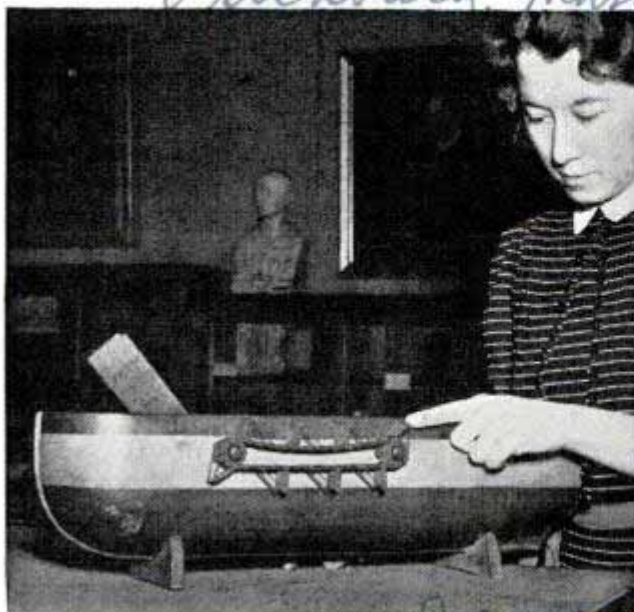
Original model of the first steamship, built in 1785 by John Fitch. Notice side paddles on belt
