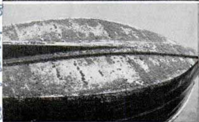
Two photographs compare boat bottoms; one at top is painted with resistant liquid
