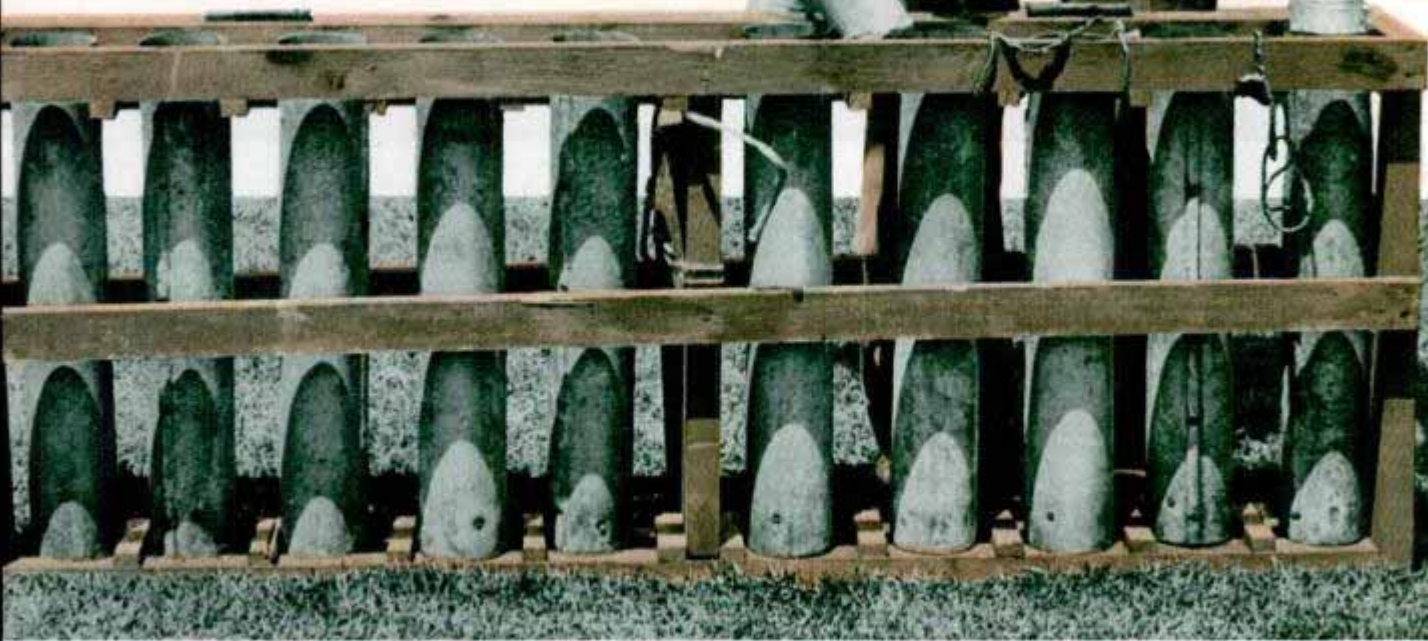
BOTH candles and bombs are fired from mortars. The candles shown here are propelled from the mortars by three ounces of powder and, when set off, create showers of fire.
