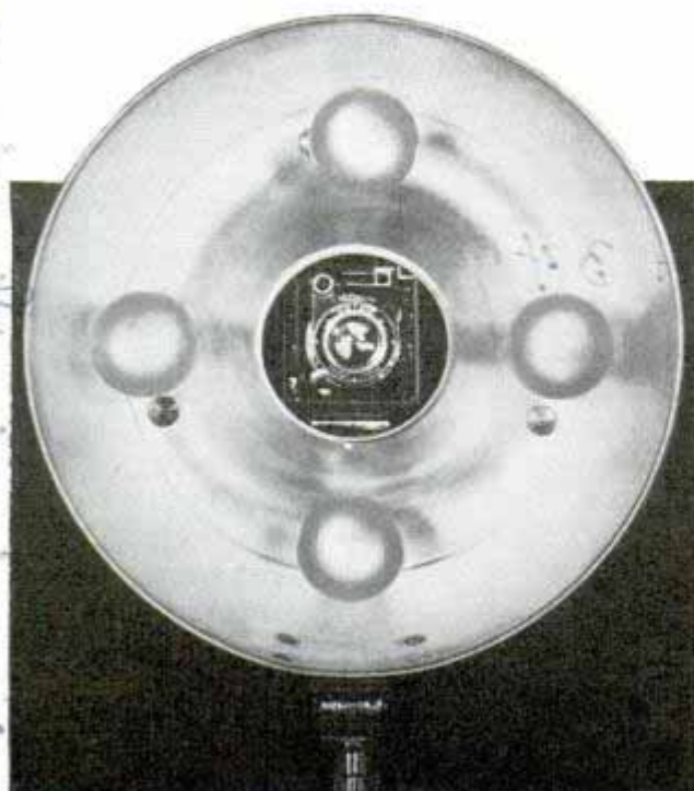
Camera shoots through window of four-bulb reflector
