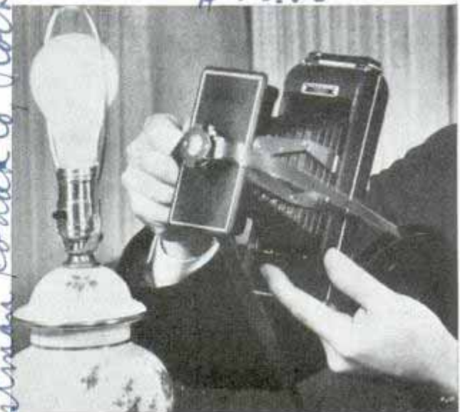
Movie film is locked in gate at front of enlarging camera and photo flood projects image on roll film
