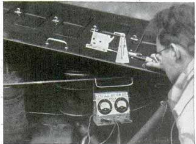
Testing ignition wiring and parts with newly developed analyzing device
