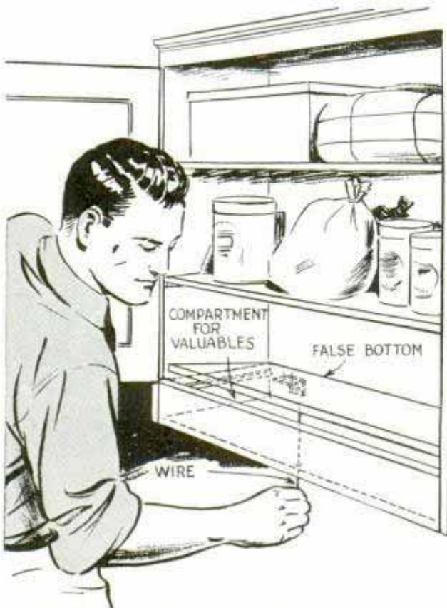
Compartment is opened by raising false bottom with wire inserted through tiny hole in real bottom
