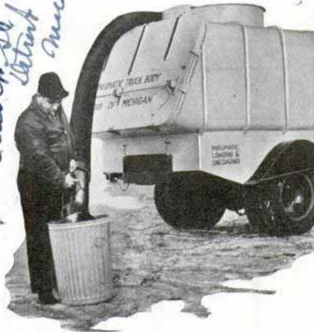
Driver dips lightweight hose into refuse can and vacuum sucks garbage into airtight container on truck
