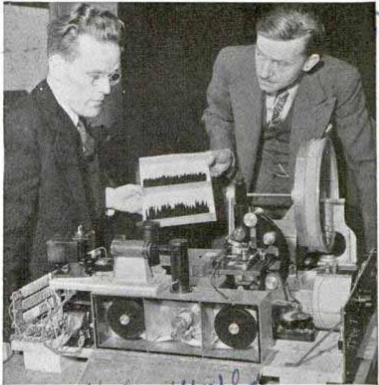
Photoelectric device with which two California scientists are trying to discover means of reducing graininess of film
