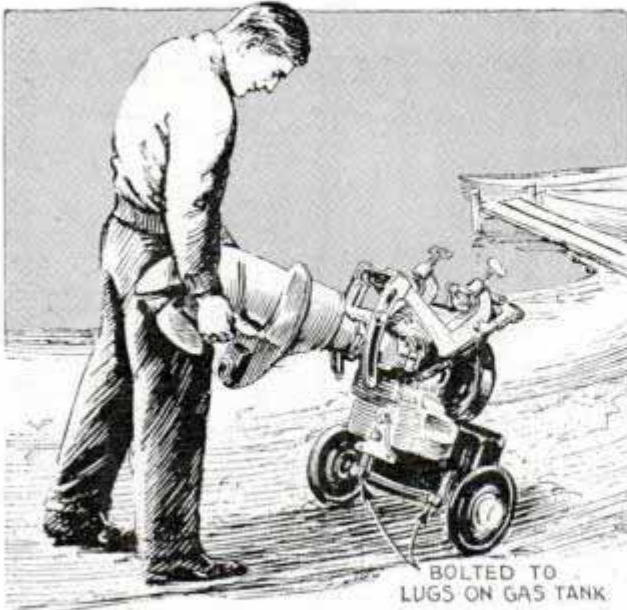
Wheels and axle from boy's wagon quickly attached to outboard motor to move it wheelbarrow fashion
