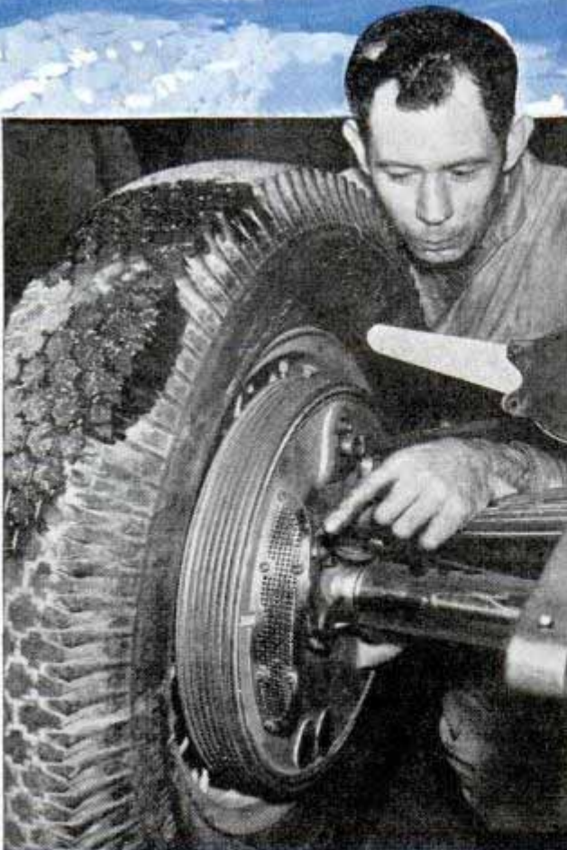
Top, race cars bunched at turn. Bottom, breather screen helps cool the brakes
