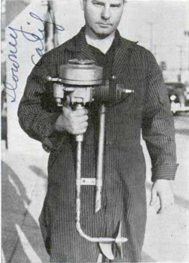
With no interference in front of it, propeller driven by flexible shaft obtains full thrust in water
