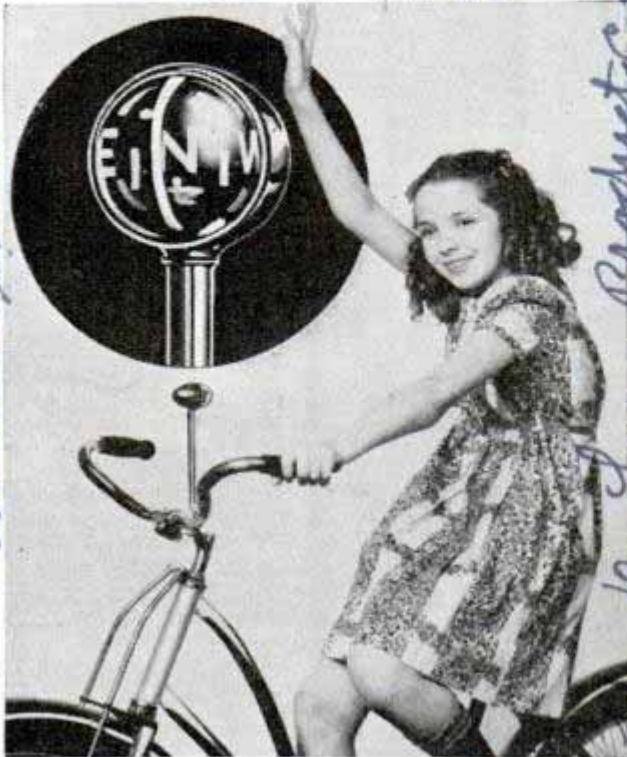
Compass, shown in circle, is mounted in streamline housing on post attached to bicycle handlebars
