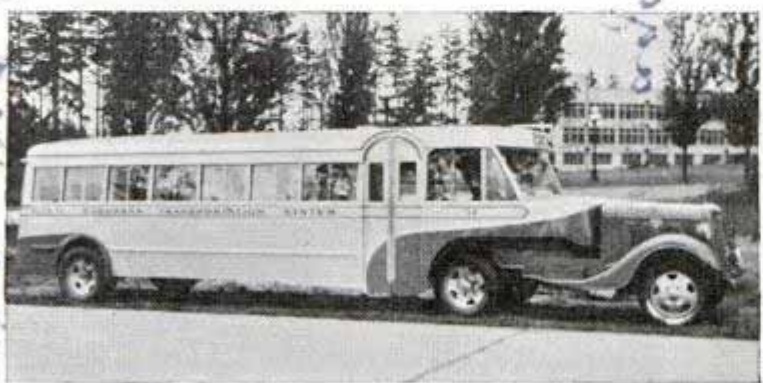
Bus driver's cab is at forward end of trailer, the controls passing through a circular turntable at rear of tractor
