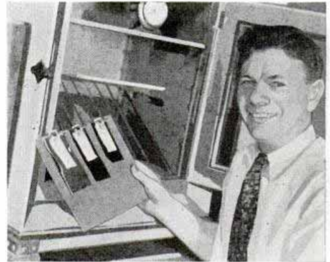
Cigarette papers clipped to leather samples test color-fastness of dyes in upholstery
