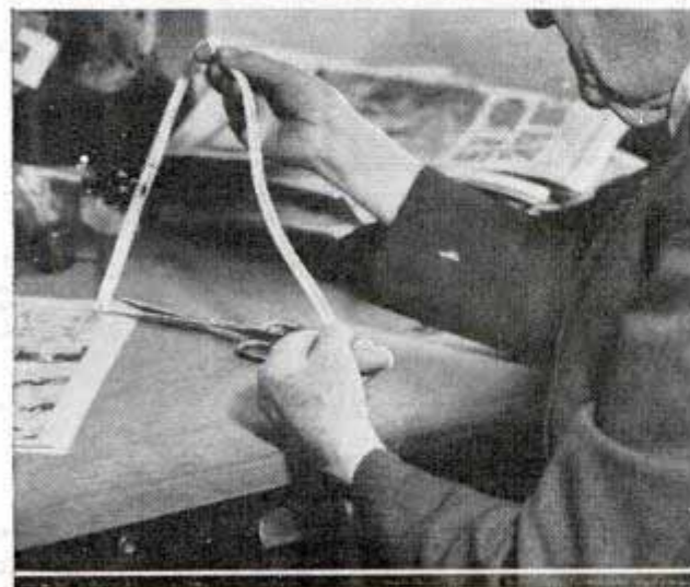
Top and bottom, cutting out sound track and pasting it into strip for reproducer. Center, typical sound feature page from which sound track would be taken
