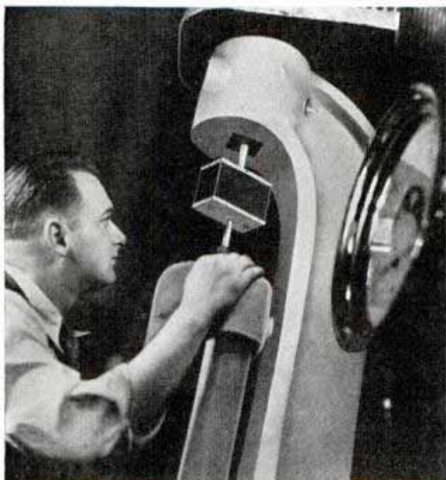
Applying 2,000 pounds tension in testing the steel-and-rubber bond of an engine mounting
