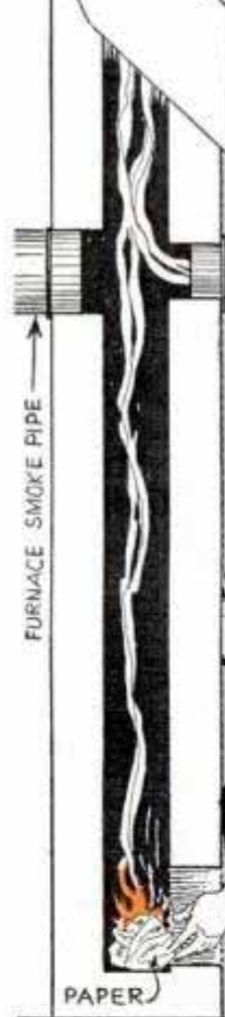
If your basement laundry stove smokes in the summer, open the cleanout door at the base of the chimney, place a roll of newspaper inside and ignite it. The heat drives the damp air from the chimney and restores the natural draft. Right, the next time you clean your library books try wallpaper cleaner to remove dust from both the pages and covers
