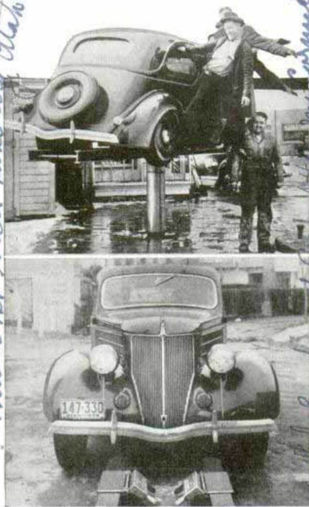
Top, showing how firmly auto is held. Bottom, preparing to hoist the car
