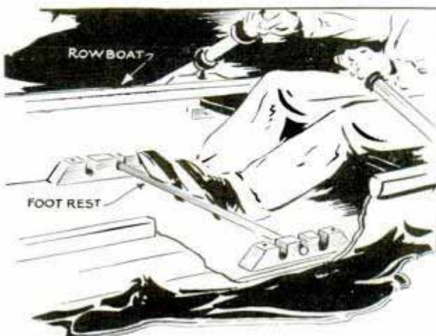
This footrest is instantly adjusted to suit rowers with either long or short legs
