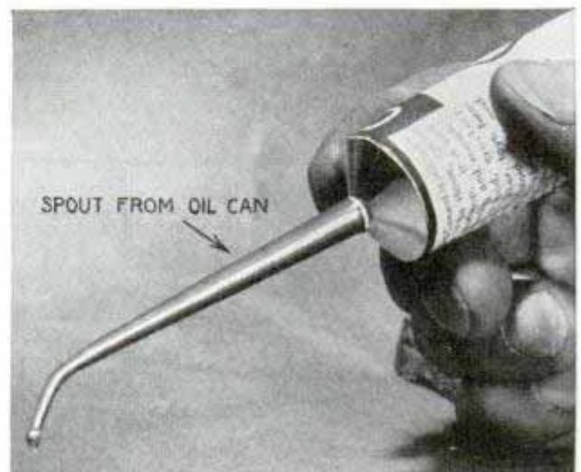
Long spout soldered to tube of cement to get at hard-to-reach places around the home
