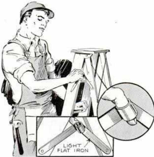
Loop on hinge of stepladder to insert finger for opening without danger of pinching the hand
