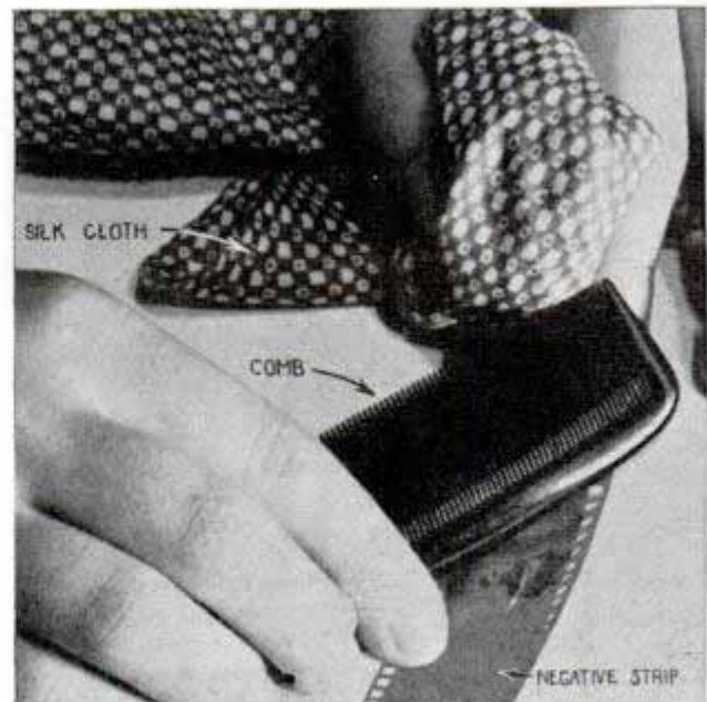
Rubber comb charged with static electricity removes invisible dust specks from miniature-camera film
