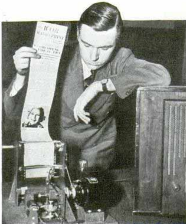
Removing sheet from receiver after test of facsimile transmission system
