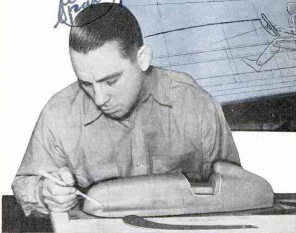
Top, celluloid model of driver's body on drawing board shows proportions for cockpit. Center, shaping racing model. Bottom, marking openings in body for radiators
