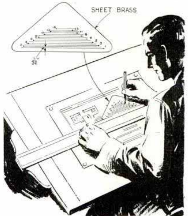
Correct spacing of lettering guide lines is assured when this simple gauge is used
