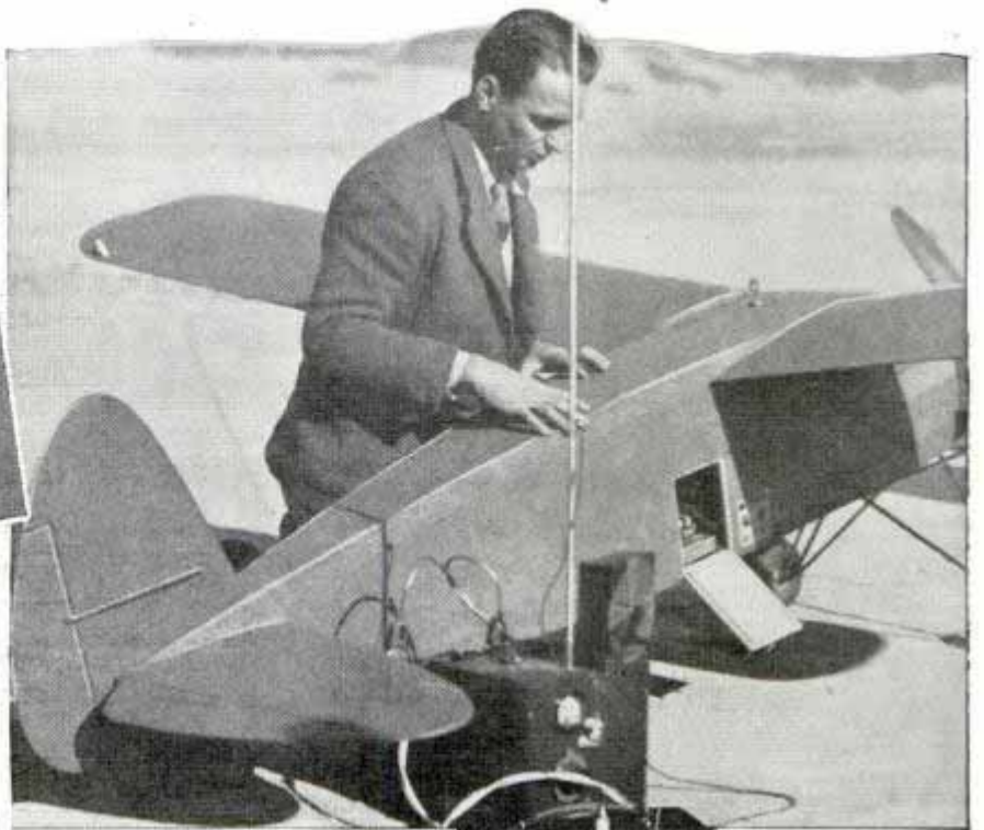
Midget planes controlled by radio are being used in army target practice. Movie cameras mounted on guns automatically register hits and misses as dummy shells pour through the anti-aircraft weapons
