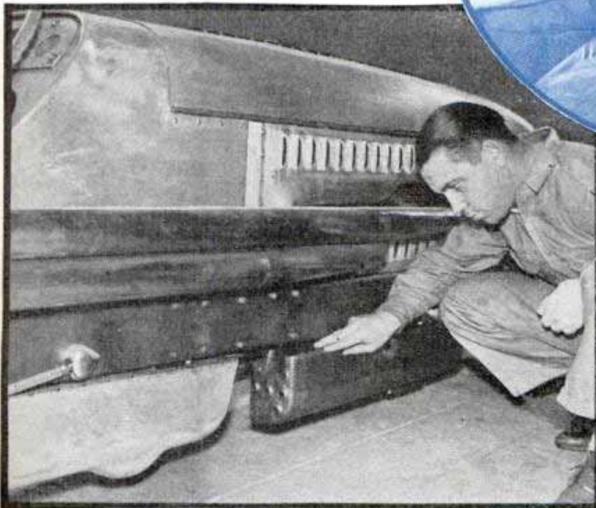
Top, streamline body of racing car. Center, smoothing off cooling fins projecting from oil tank. Bottom, oil tank slung under car
