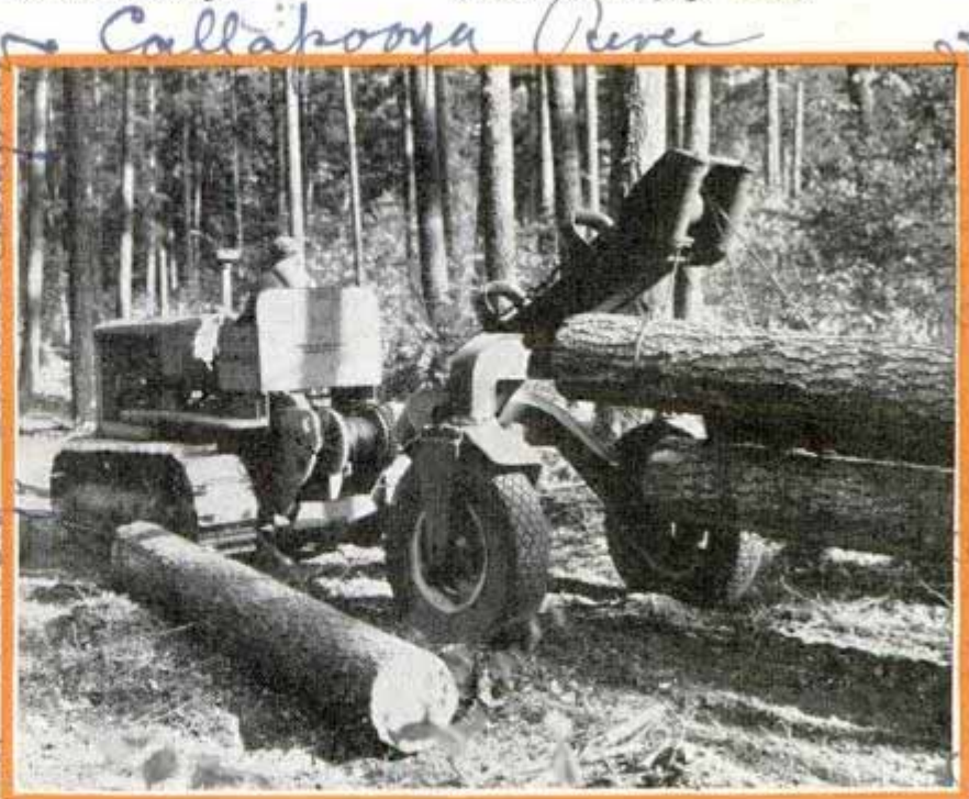
Top, load of huge fir logs on flatcar ready for shipment. Bottom, tractor with equipment powerful enough to lift fifty-ton load of logs off ground
