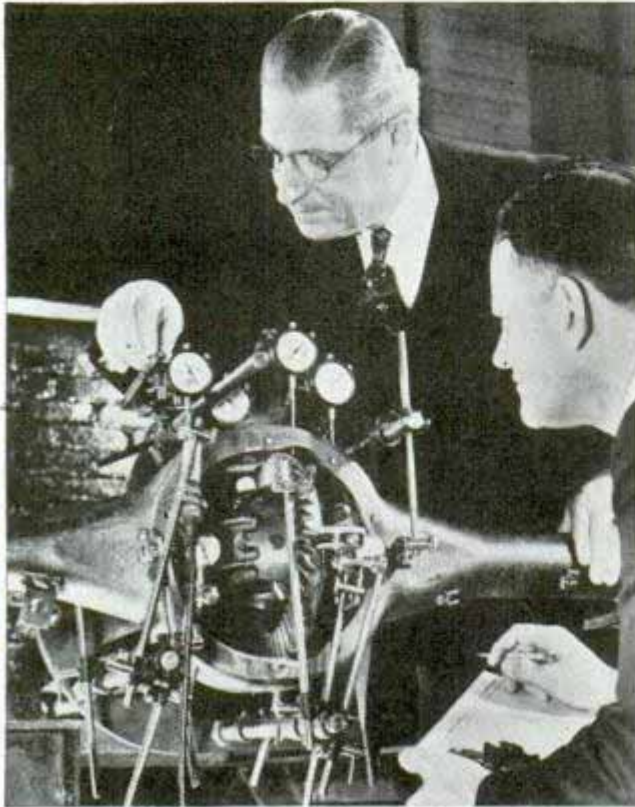
Apparatus in place to test rear axle's operation under driving condition loads
