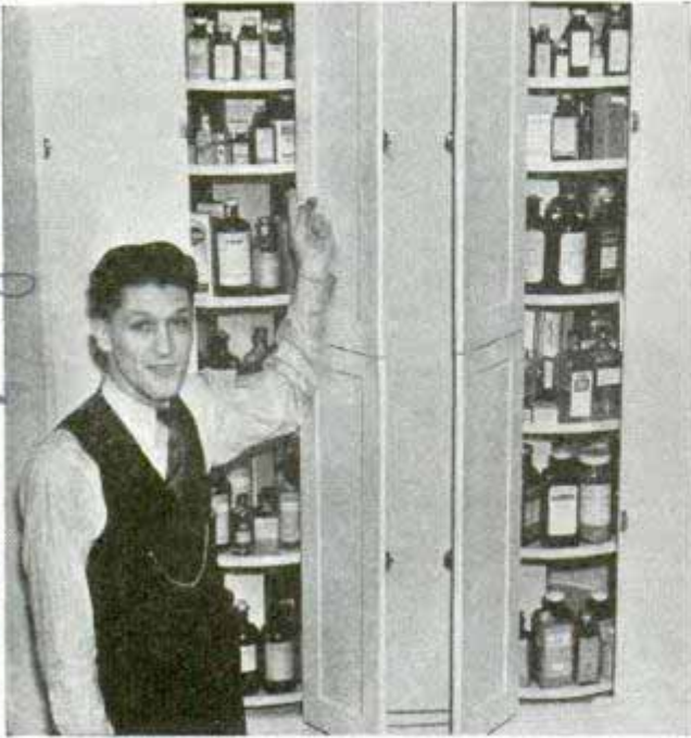
By twirling the shelf, the druggist brings to the front any bottle or package he is hunting
