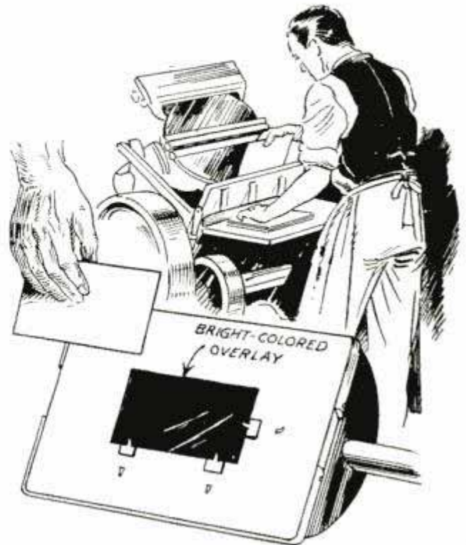
Printer's eyes follow colored area on tympan, and hand accordingly directs paper to guides
