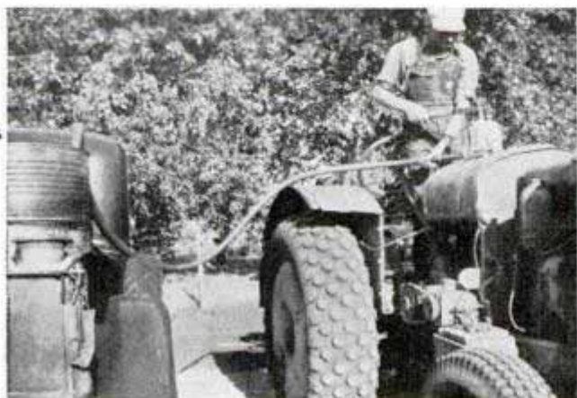
Refueling a farm tractor with hand pump controlled at spout end, reducing danger of overflow
