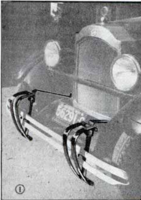
1. Bumperettes bolted over front bumper of tow truck aid in pushing cars. 2. Inverting battery-box clamps makes it easier to remove battery from dash
