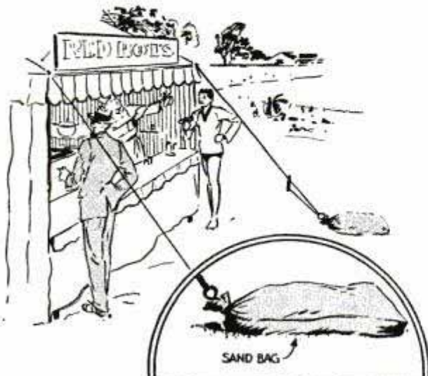
When soil is too loose to hold tent stakes, substitute large sacks filled with sand
