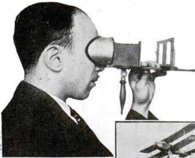
Top, old-fashioned stereoscope's optical illusion of a third dimension is the basis of the photogrammetrist's art. He catches it on his complicated machine and transfers it to paper in the form of topographic or contour map
