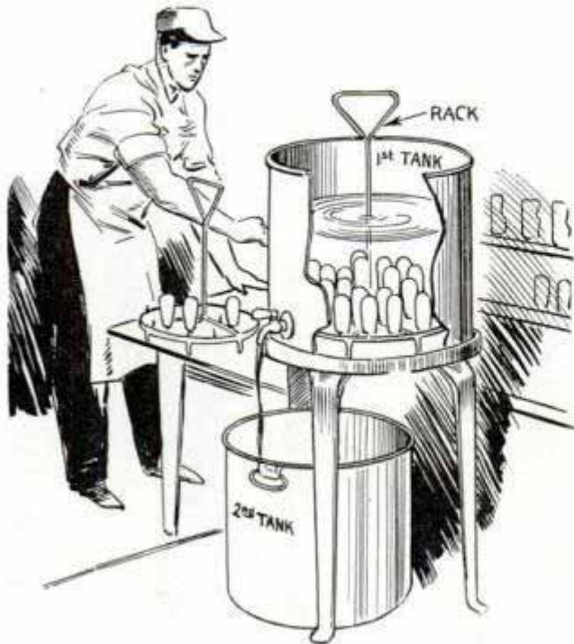
"Drain finishing" of small duplicate parts leaves a uniform paint film on flat and irregular surfaces
