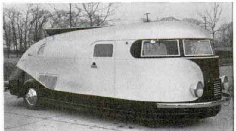
Specially built automobile provides for driver to sit close to the front, giving a wider range of vision
