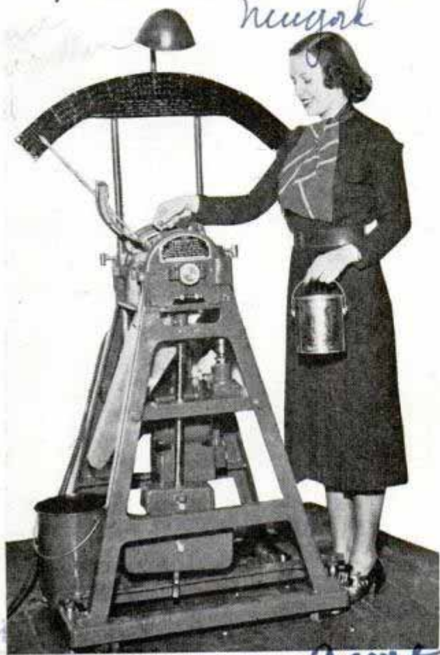
Testing peas for tenderness. Dial measures force required for knife to cut through sample of peas
