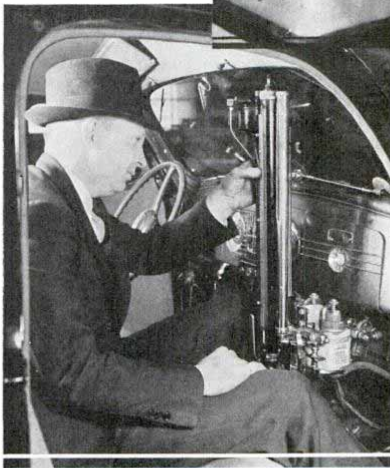
Adding sludge, above, to clean oil during a test of oil filters. Left, engineer reading "flowmeter" on Chrysler test car
