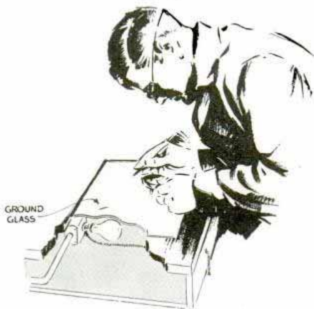
Intricate parts of models or watches are easily assembled on this lighted ground glass
