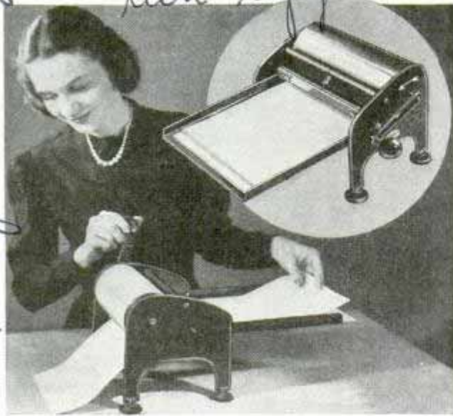
As many as sixty smudgeless copies a minute are turned out by this rotary duplicator
