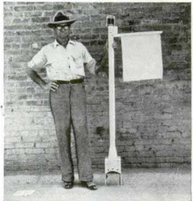
Signal arm drops into horizontal position and flag unfurls when irrigation water raises its float
