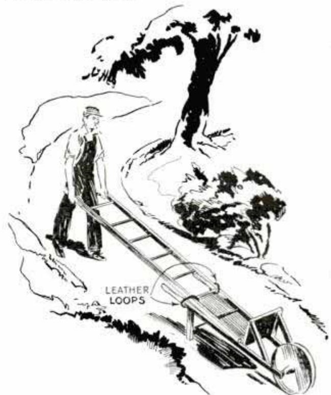
Attached to the handles of a wheelbarrow by means of straps, a heavy ladder is transported easily
