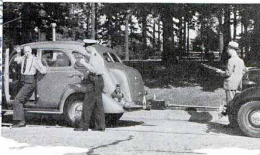
Demonstration of how fugitive car is halted by claw-and-cable on police car and how suspect may be captured easily
