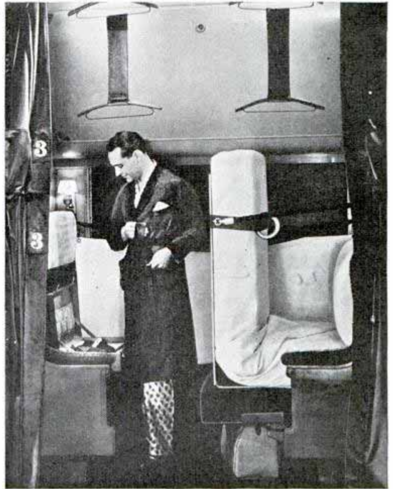
Sleeping car bed folds up on hinged metal sheet, allowing passenger standing room and a seat while dressing or undressing
