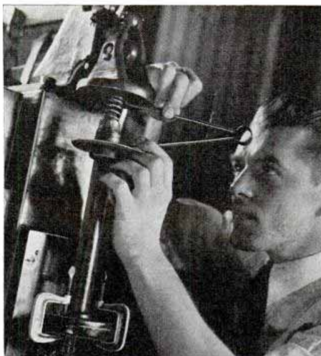
Setting limit of compression for small spring about to undergo fatigue test
