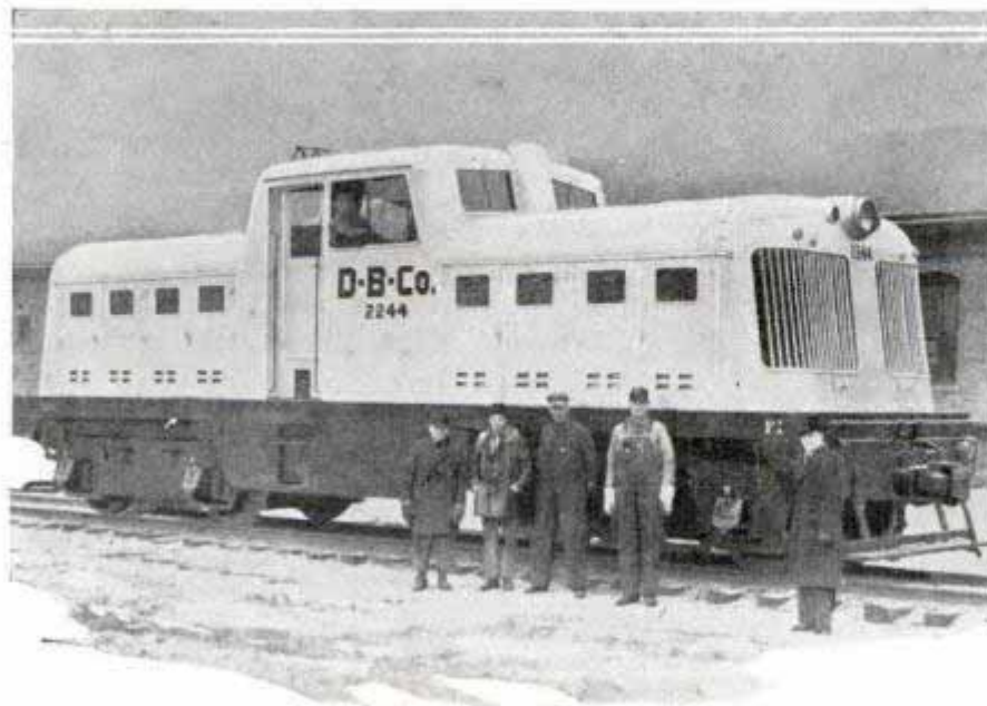
Designed for flexible, economical operation in switchyard, this Diesel locomotive has four eight-cylinder engines which work singly or teamed
