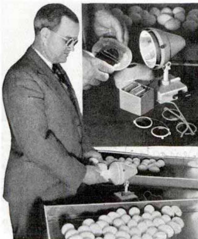
Inset, equipment for detection of infertile eggs. Below, candling the eggs
