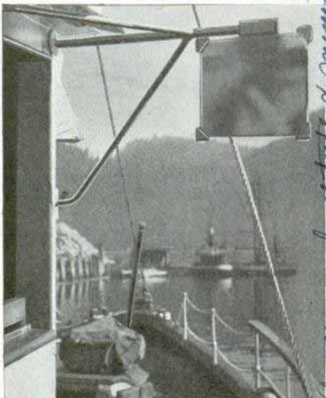
Looking in this mirror from wheelhouse, tug skipper can see beyond his own decks to the tow astern
