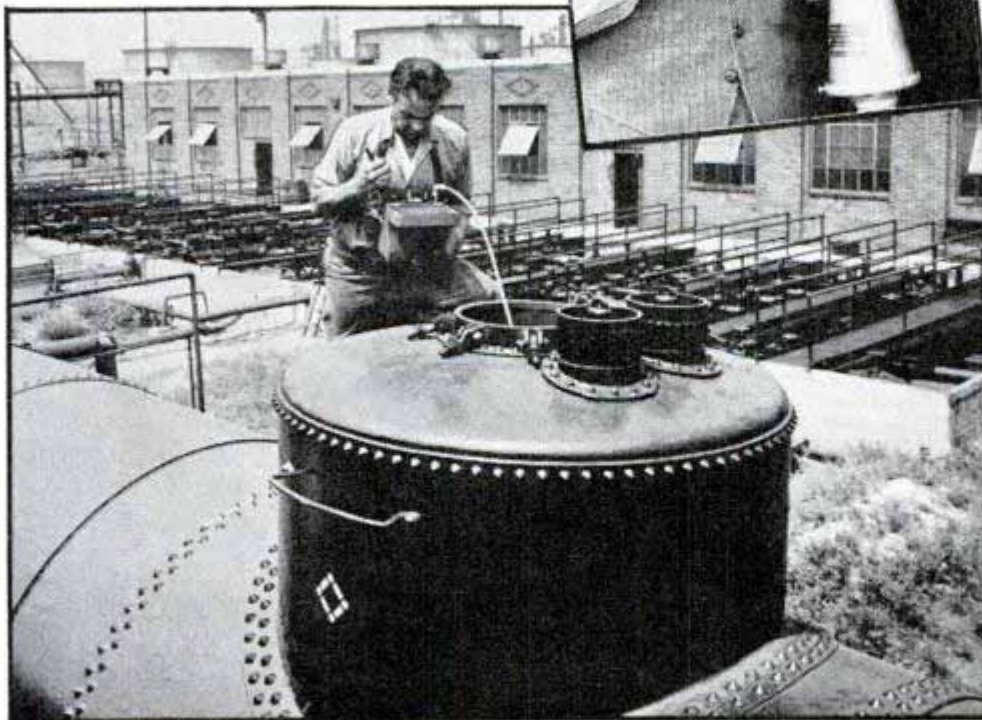
Top, eyes are saved in this manner. Center, sensitized paper being placed in mercury vapor detector. Bottom, testing tank car for combustible vapors
