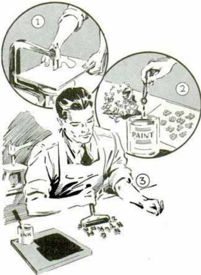
First dip letters in the color to show on the edges, then apply printers' ink to the upper surfaces
