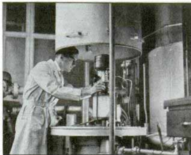
Testing carburetor and air cleaner to determine most economical fuel mixture
