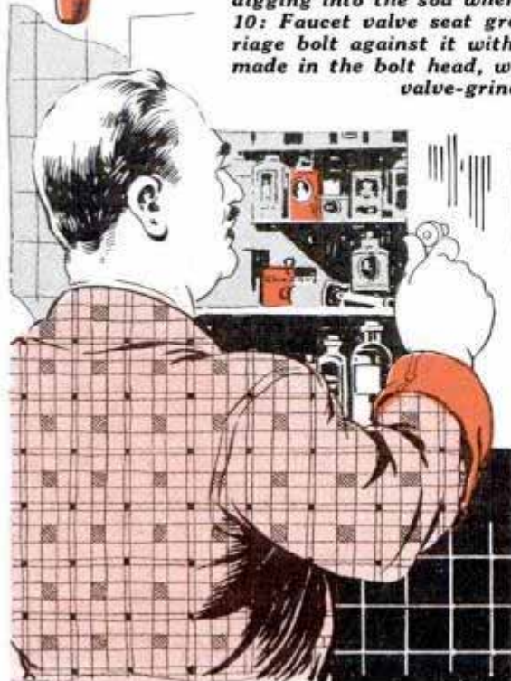
11: To avoid repeatedly opening the mirrored door of his bathroom medicine cabinet while shaving, one home owner pivoted the door on metal arms so that it could be moved forward and then swung to one side with the mirror facing him. A rod is run vertically through the cabinet at one side near the front to take a brass tube snugly. The arms are soldered to the ends of the tube and pivoted to the door
