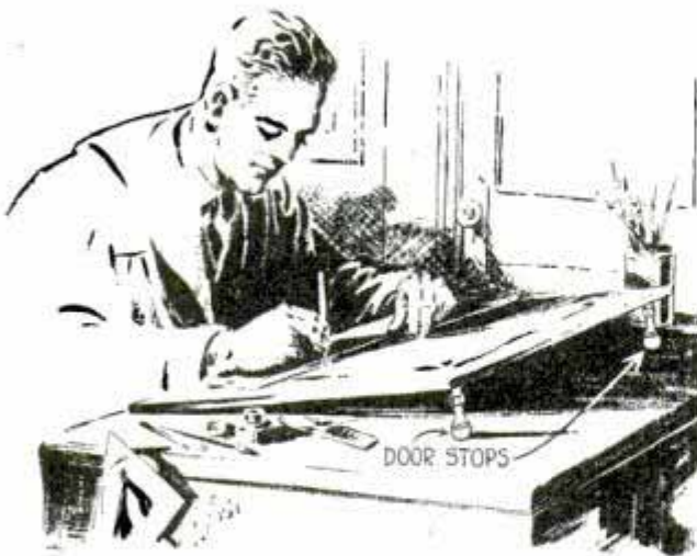
Two rubber-tipped doorstops driven into drawing board near rear edge tilt it at easy-working angle
