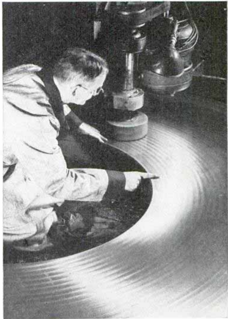
Polishing one of two 105-inch thrust bearings for Pickwick Landing Dam power plant. They will carry 2,500,000-pound load
