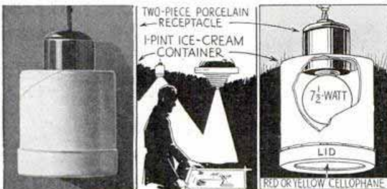
These photo safelights are so easy to make that you'll want several of them for your darkroom
