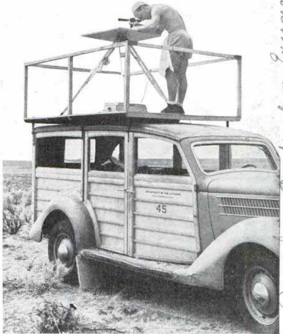
With instruments on top of truck, surveyors are ready for quick moves across desert and sighting is unaffected by "heat waves" near ground
