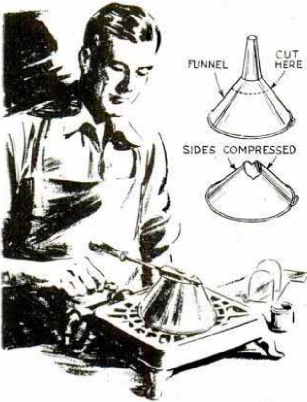
Top of tin funnel altered to hold soldering iron over gas burner and conserve flame for quick heating
