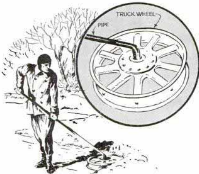
Paths can be cleared for skating by pushing truck wheel over snow-covered ice
