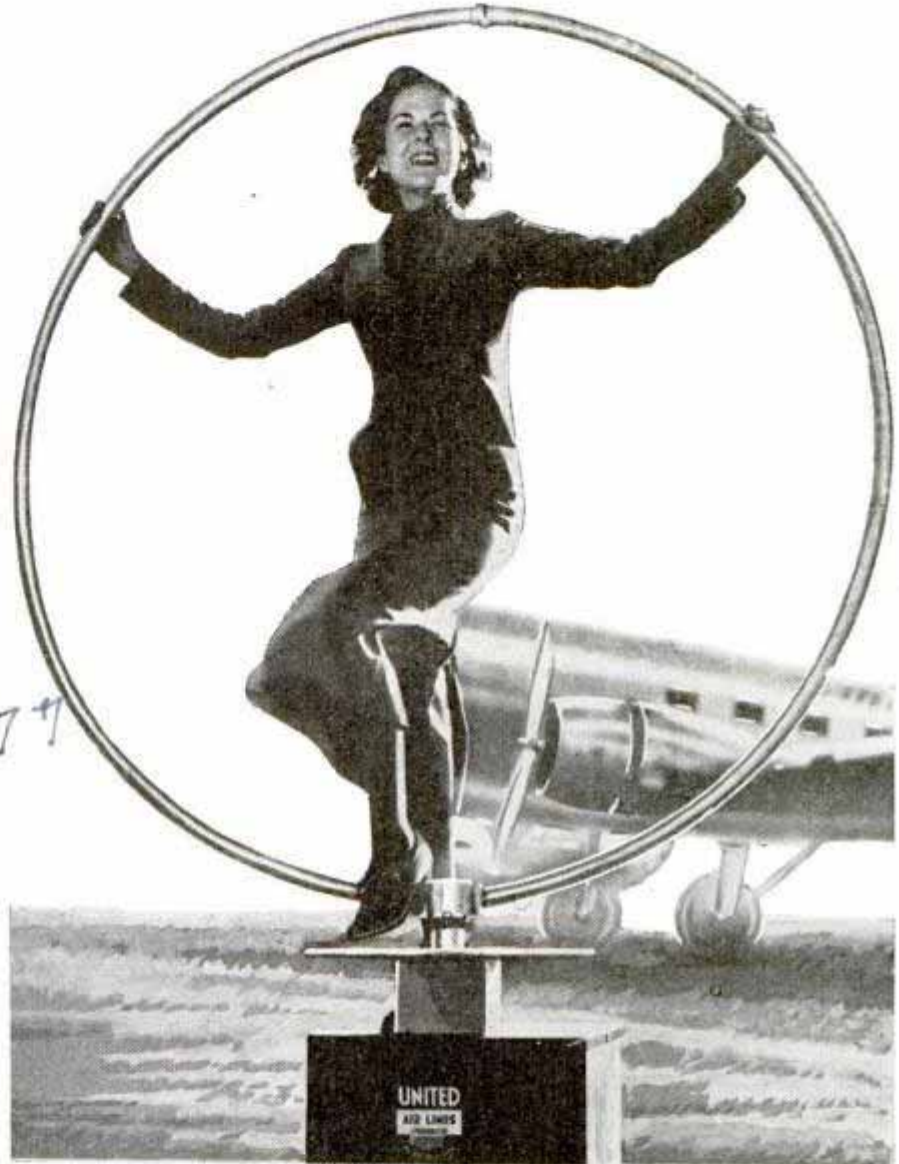
Demonstrating the size of anti-static loop for ground stations. The loop is intended to reduce interference in plane-ground communication
