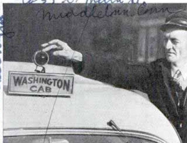
When cab driver switches on this blinking light, it is a signal to police that he is being robbed
