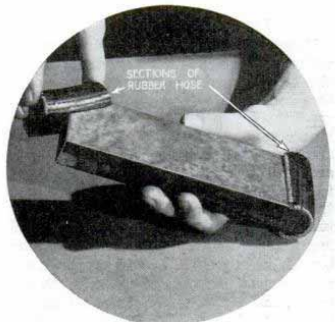
Slit pieces of garden hose over ends of oilstone provide friction against bench top
