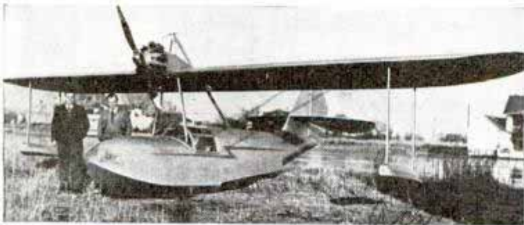
Here is the clipper ship, powered with a single motor, after a test. Its motor develops forty horsepower
