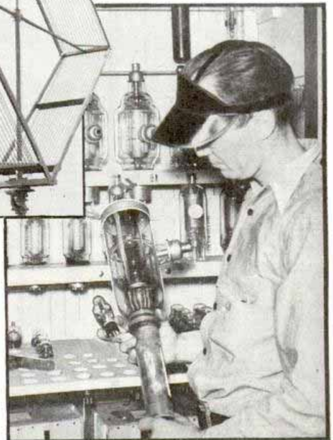
Center, fixed loop antenna used for reception of point-to-point radio messages. Bottom, water-cooled tube used in 5,000-watt transmitter
