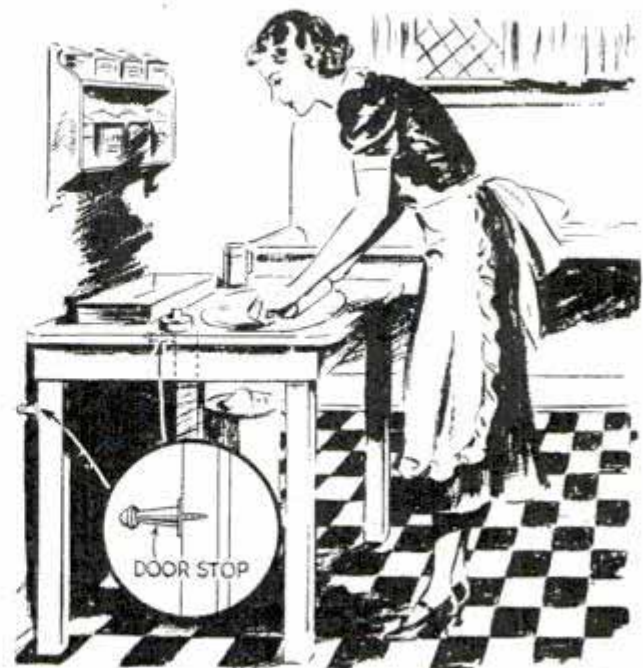
These stops prevent edge of table from bumping wall when kneading dough or doing other work
