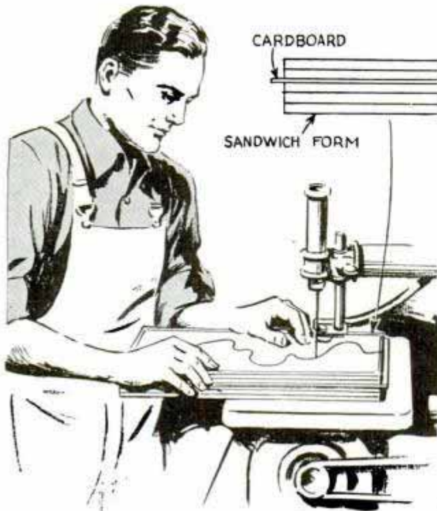
Cardboard placed between stacked work before sawing produces extra pattern without effort
