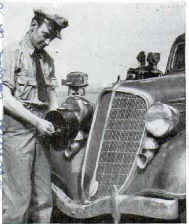
Here the mechanic is testing horn for volume by means of a handy meter
