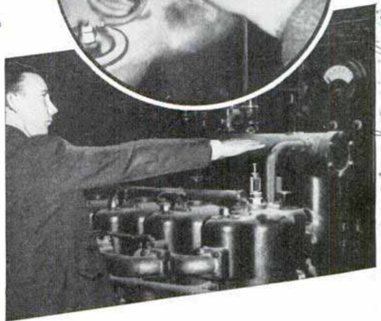
Inserting shotgun shell into special firing chamber in cylinder and touching it off with plunger to start gasoline engine
