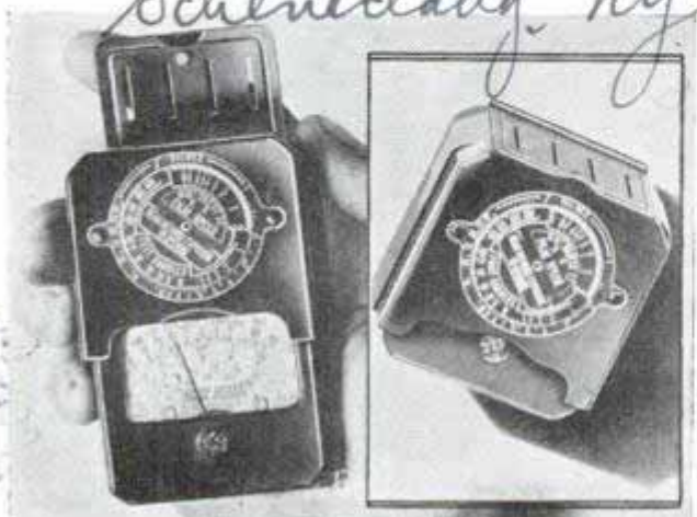
Two views of handy light meter devised for amateur or professional photographer
