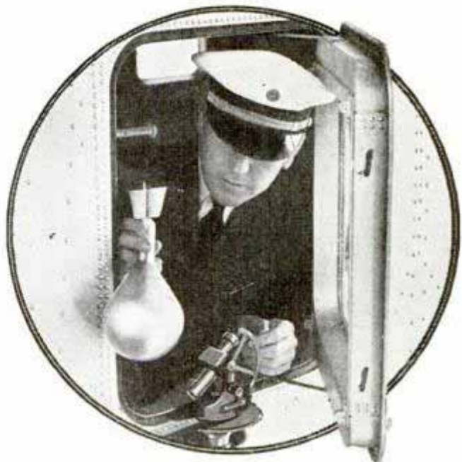
Top, testing engine. Bottom, releasing aluminum powder bomb. Drift indicator on window is used to sight the bright spot the powder makes on water
