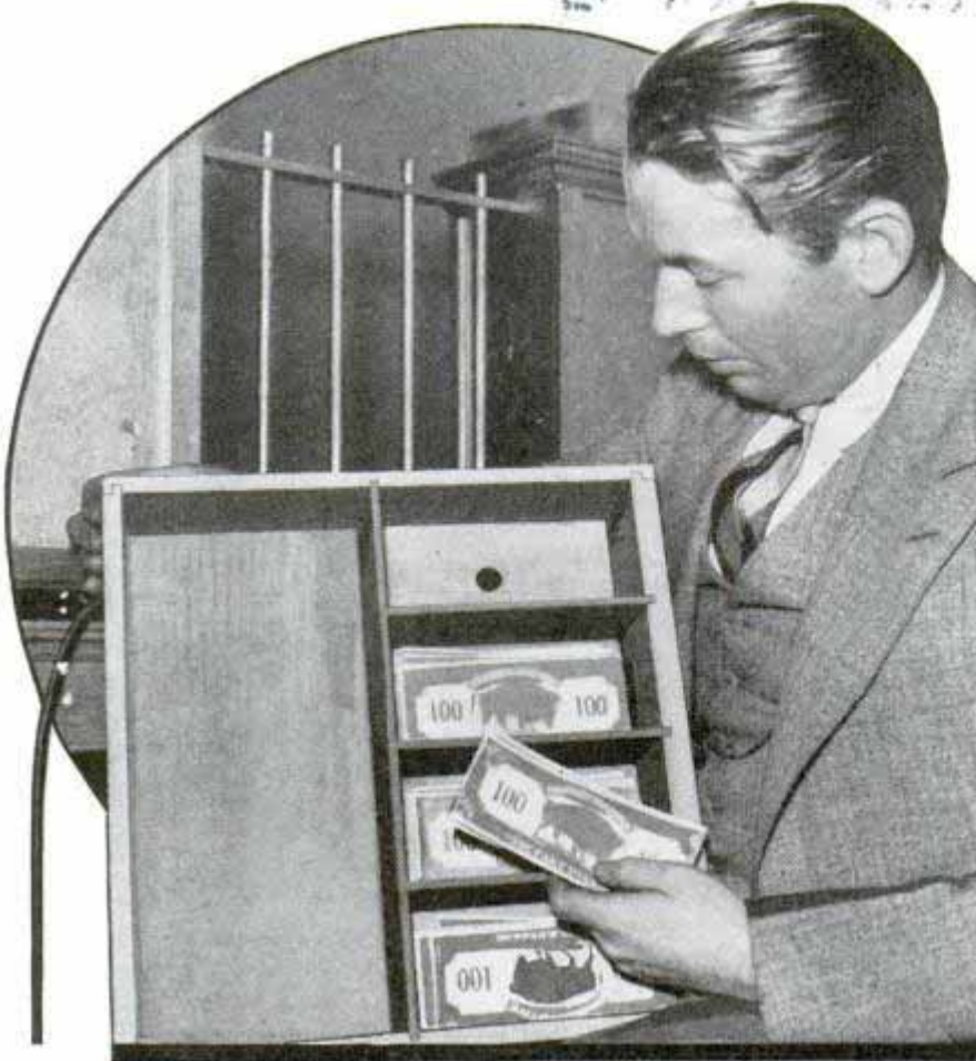
Photocell in currency drawer gives alarm when certain sheaf of bills is removed
