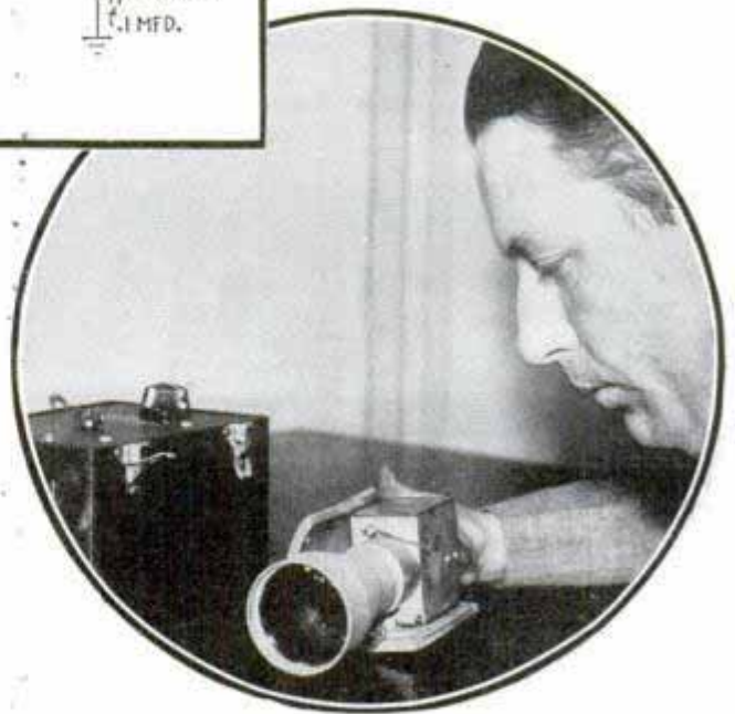
Center, typical hookup of projector and detector. Bottom, projector consists of tiny light, diaphragm, lens and infrared filter. It may be mounted in steel or concrete post
