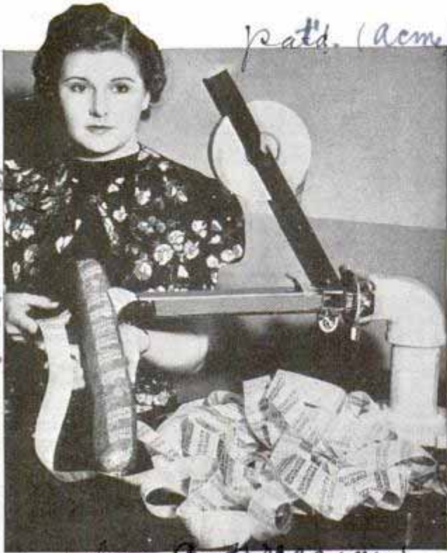
Small machine which places the non-removable labels in each sausage
