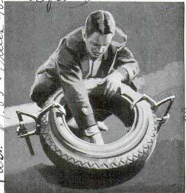
Handles of these twin tire spreaders support tire in easy position for inspection and repair
