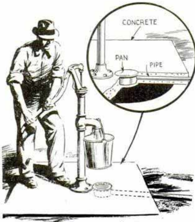
Drain pipe leading into depression in curb under pump spout carries away water
