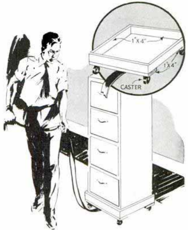
File cabinets mounted on dollies save many steps as they can be moved to the worker's desk when needed
