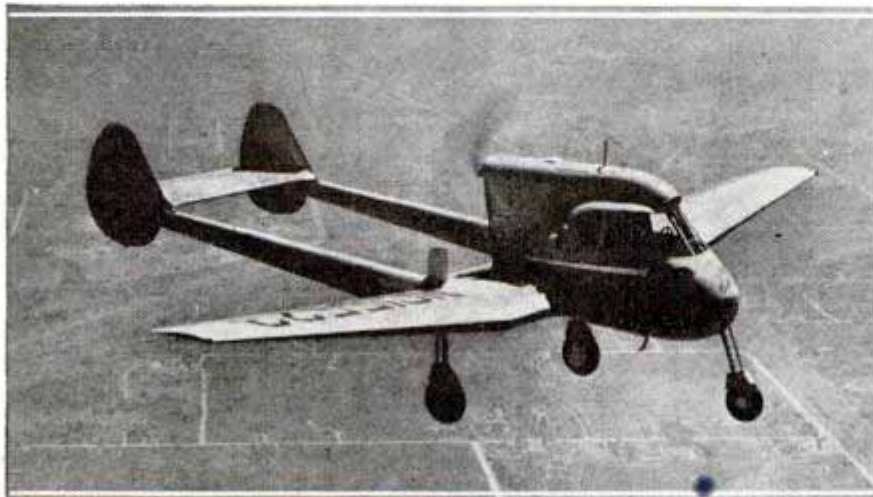
Twin-tailed plane in the air. Note the nose-wheel landing-gear
