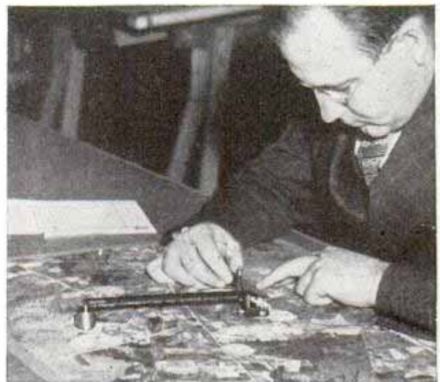
Applying planimeter to aerial map to measure acreages in checkup of crop-reduction contracts
