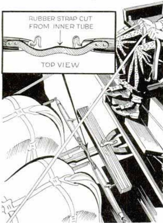
Bridging the space between the singletrees keeps lines from getting under them
