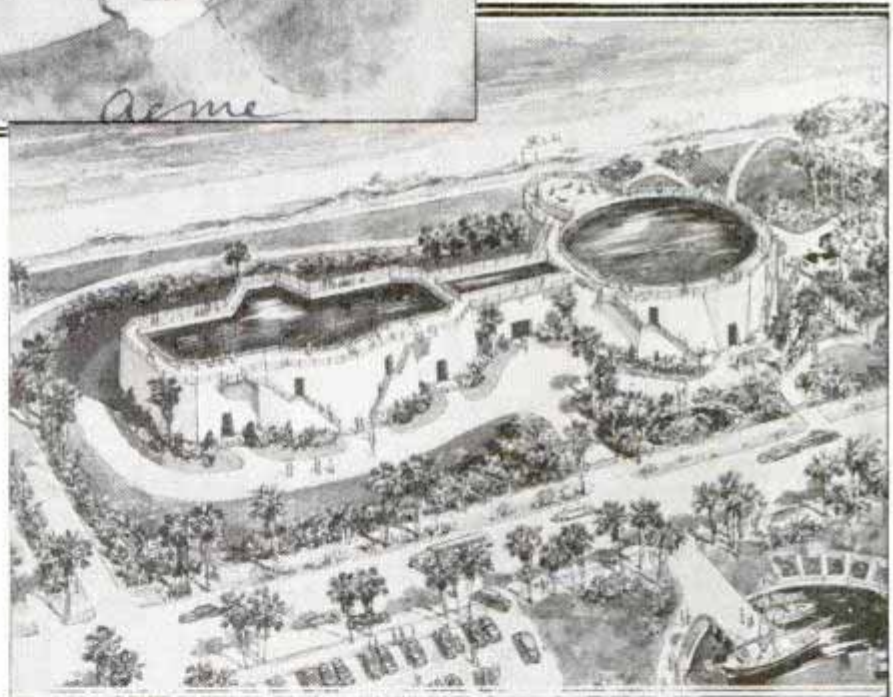
Top, sketch showing construction of tank with its inclosed galleries and windows at various submerged levels, permitting the visitor to watch life on the "ocean floor." Below, a general view of the seaside tanks
