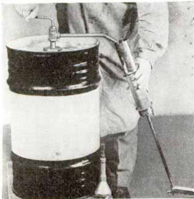
Filling grease gun by means of pump which fits bung of lubricant barrels
