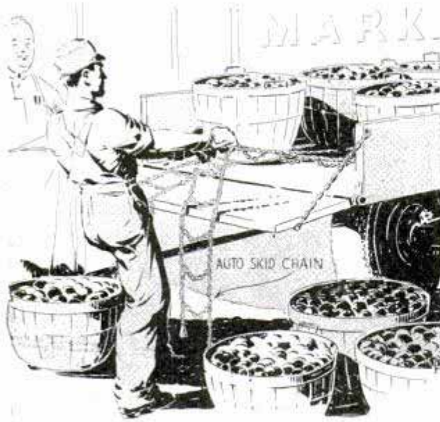
Baskets of fruit set on skid chains laid in truck bed easily moved to rear by pulling on chains
