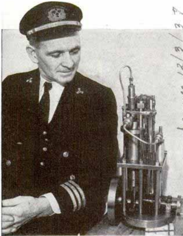
One-half horsepower Diesel engine designed to furnish power for small lighting plant
