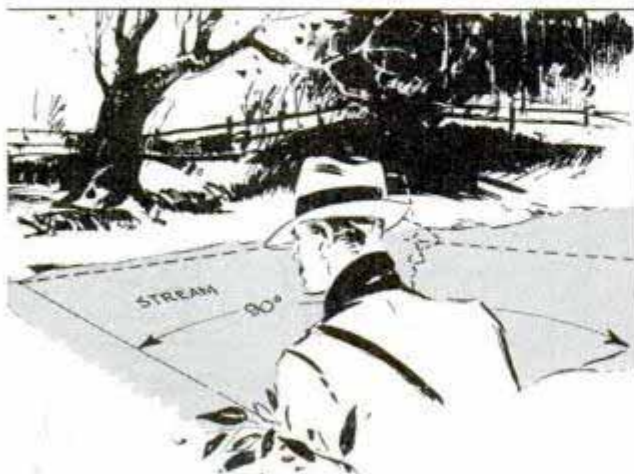
Line up brim with opposite bank, then turn and line up object on shore and step off this distance
