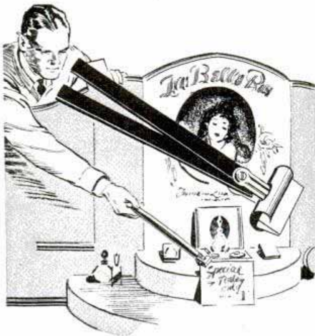
Small items in a crowded show window removed with these pincers without disturbing other articles
