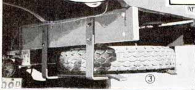
3: Truck spare tire carried on a flat-iron rack bolted to chassis frame. 4: Red lanterns are kept from swinging if wires are fitted to them to slip over hooks on boards
