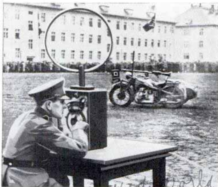
Army motorcycle without a rider maneuvers under radio control
