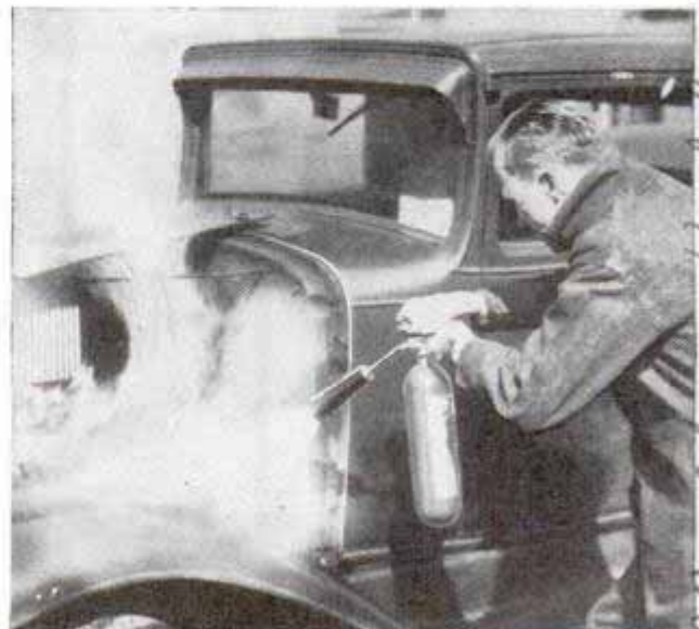
Smothering fire under hood with aid of extinguisher which fits beneath cowl
