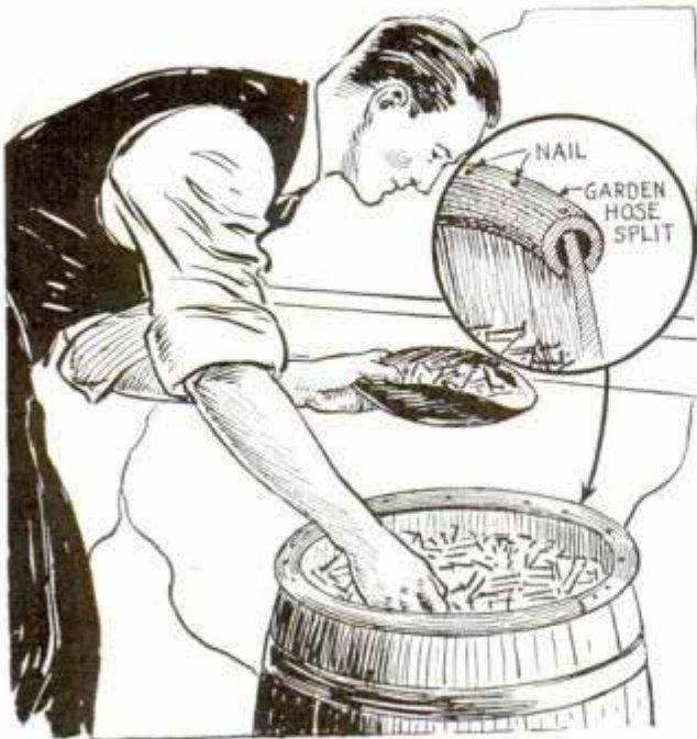
Rubber-hose shield around top edge of opened nail keg prevents injury to arms and hands
