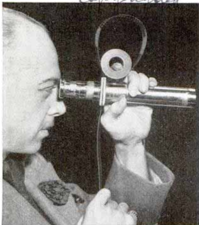
Examining film for light density with the aid of handy testing instrument
