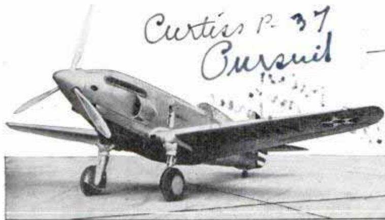
Latest army pursuit plane which has a speed above 300 miles per hour. The landing gear is retractable
