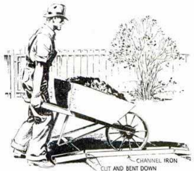
Loaded wheelbarrow pushed across sidewalk easily on bridge consisting of a length of channel iron
