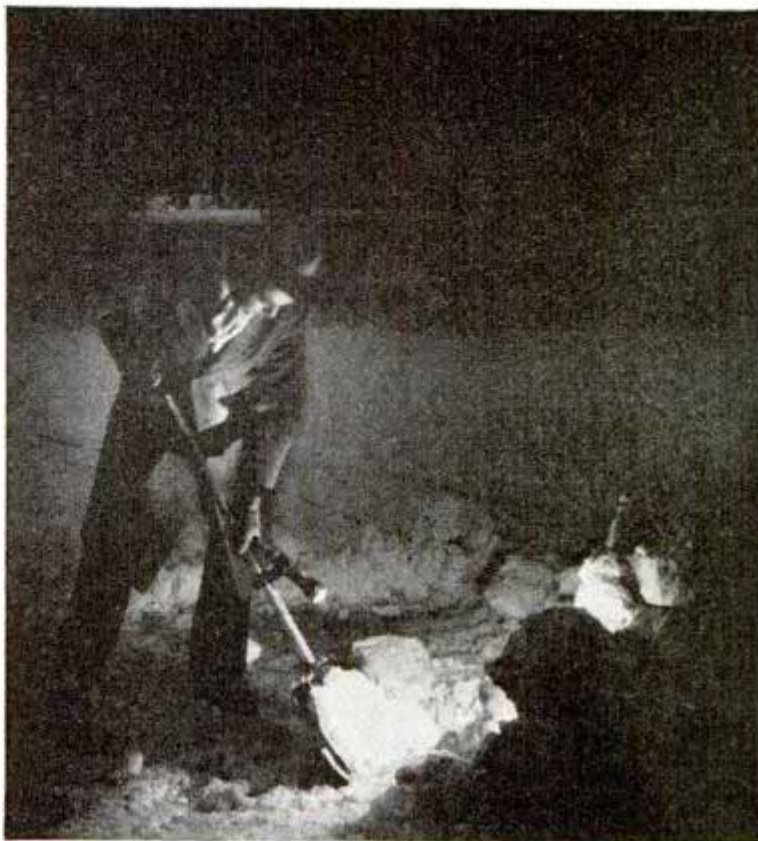
Flashlight mounted on handle of snow shovel makes it easy to guide when scooping the drifts off the sidewalk at night
