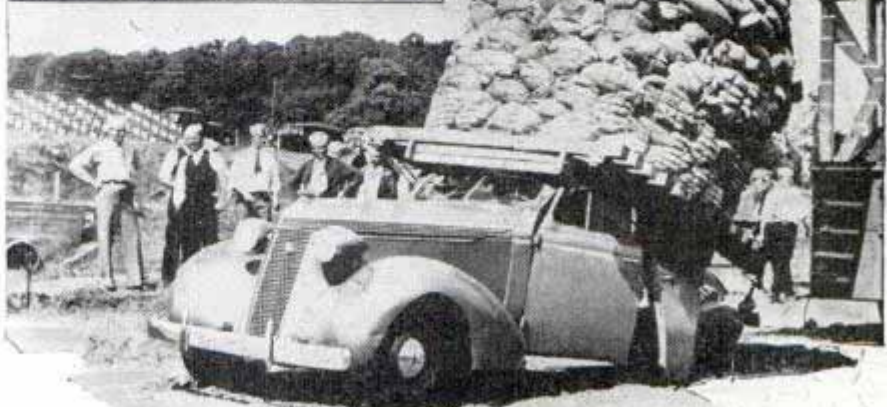
Here we see the automobile after it collapsed under a load of 24,750 pounds, seven times the weight of the sedan
