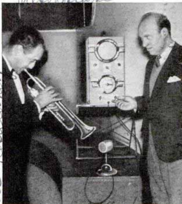
Finding proper pitch for instrument with the aid of cathode-ray tuning device
