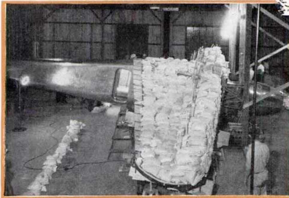
Top, drawing of the "flying wing" envisioned by the author. Left, static load test of a new Lockheed. Plane is inverted and sandbags weighing far in excess of any weight the plane will carry are placed on the wings
