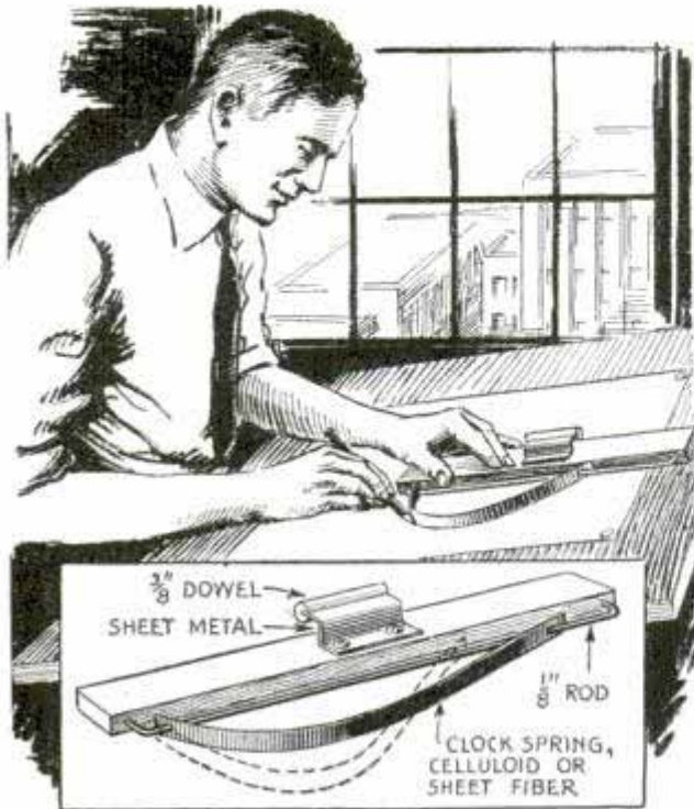
Adjustable drawing curve made from wood block fitted with a handle and a length of clock spring
