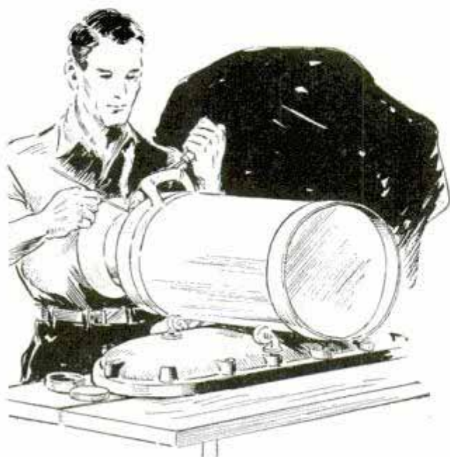
Large cylindrical objects, such as milk cans, that are to be soldered are readily rotated in this holder
