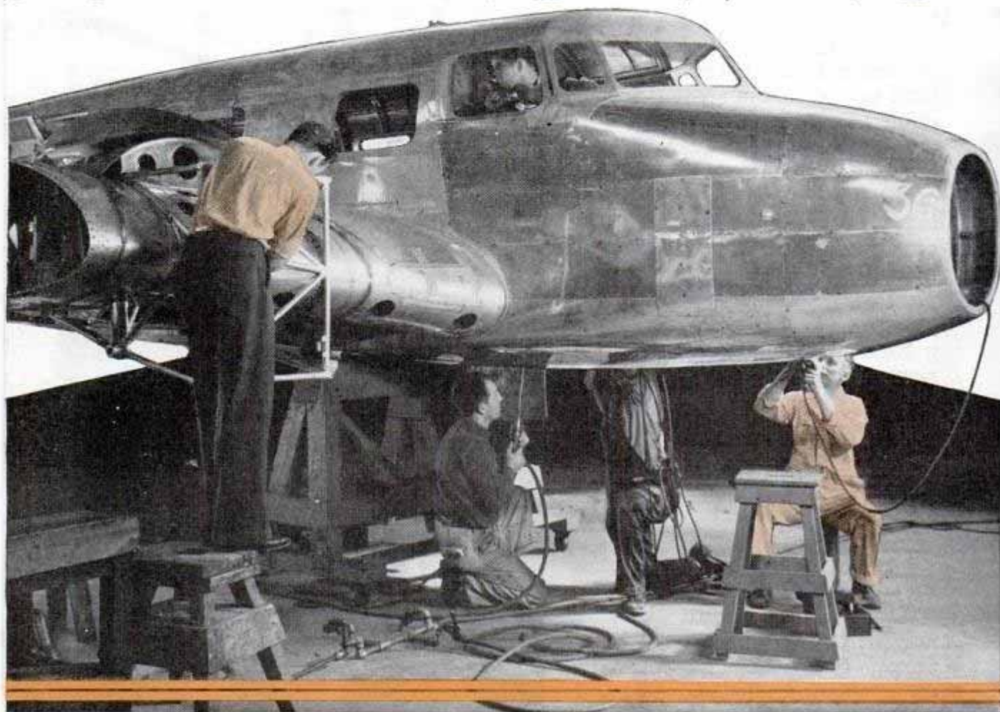
Building the first all-metal transport designed by the author. This is the Lockheed Electra, famed for its speed. Here we see workmen busy on wing and nose
