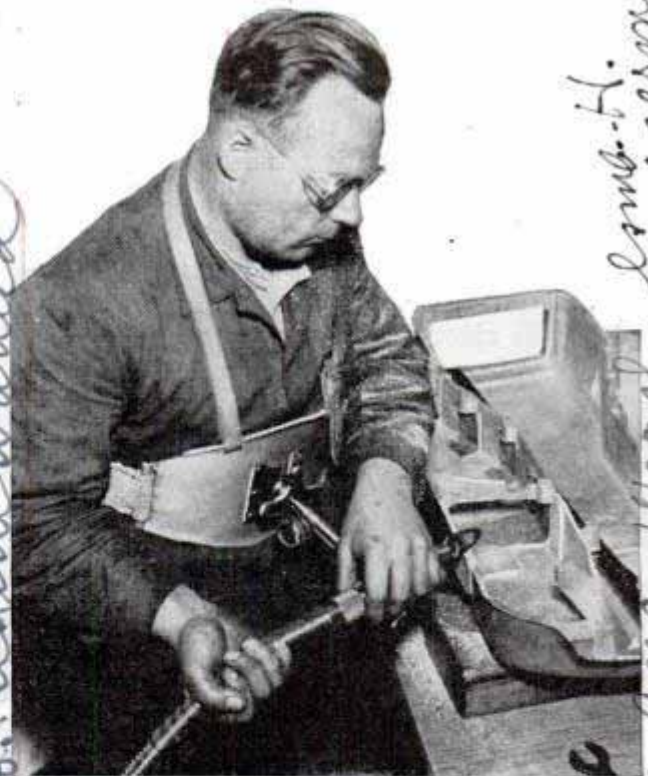
Operator applying pressure on tool by means of belt. His hands guide the tool
