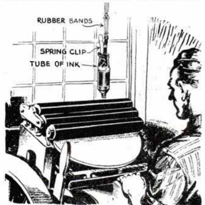
Ink tube suspended from ceiling above job press by rubber bands is always at hand for inking the plate
