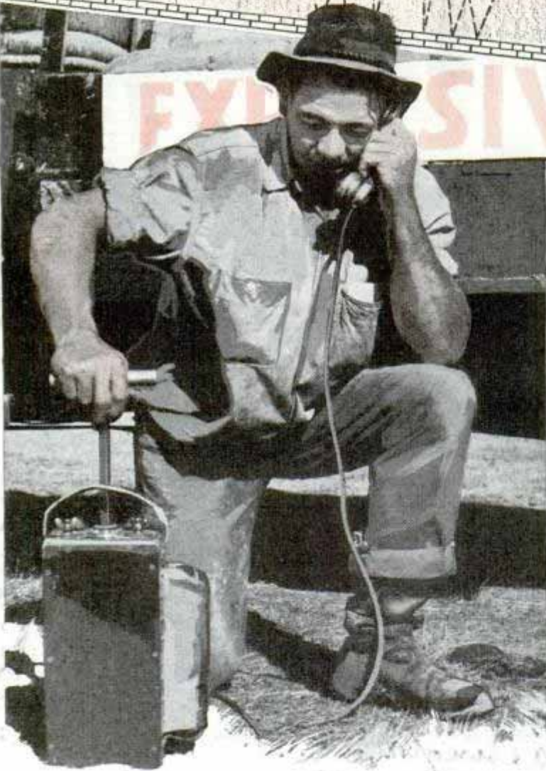
Top, diagram showing how earthquake waves are reflected by strata. Bottom, preparing to explode buried charge by pushing handle of blasting dynamo upon telephone order
