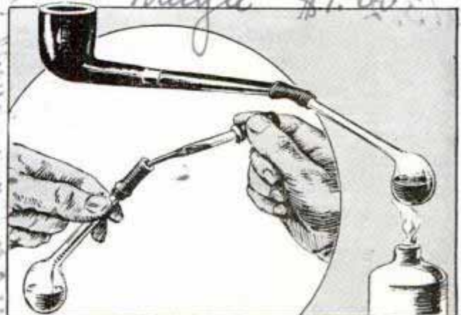
Cleaning fluid inserted in retort with medicine dropper boils up into pipe when heated
