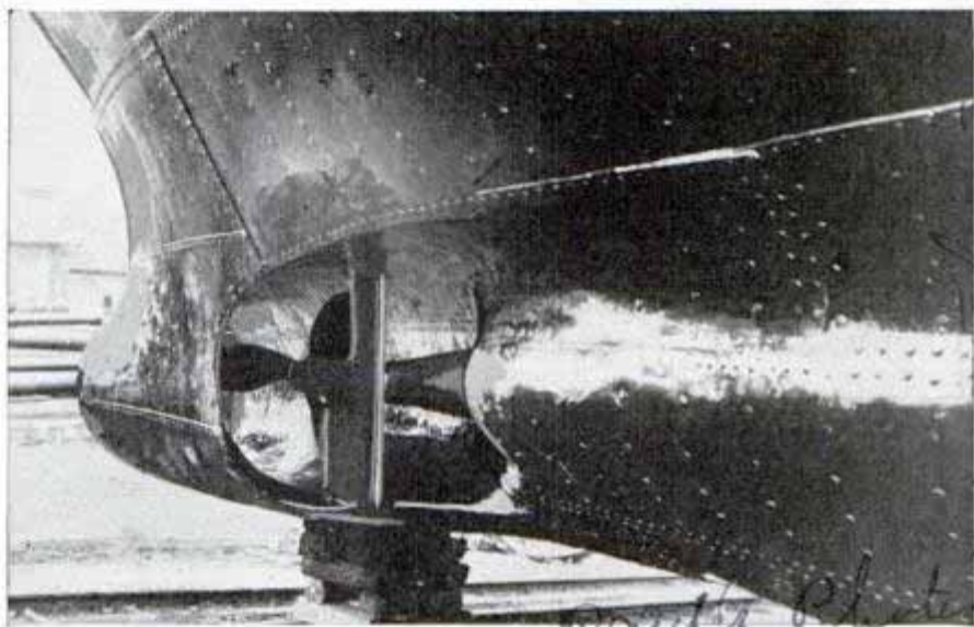
Top, latest watercraft designed for canals and small rivers. Bottom, front drive causes less disturbance of water than stern drive
