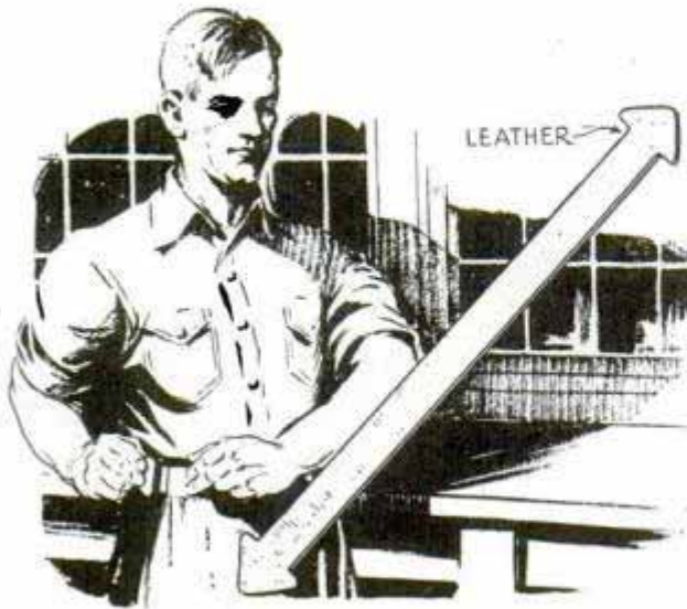
Workman's apron held by arrow-pointed strap is quickly put on or taken off
