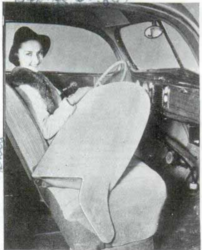
Back of divided front seat swings forward and inward in latest coach
