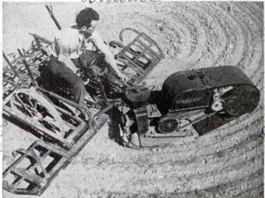
Demonstrating how the small tractor can turn sharply while pulling farm implement. Note that the tractor has only one track
