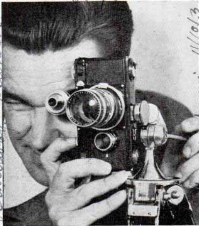
If camera has threads on only one side, swinging head on tripod permits mounting camera at any angle
