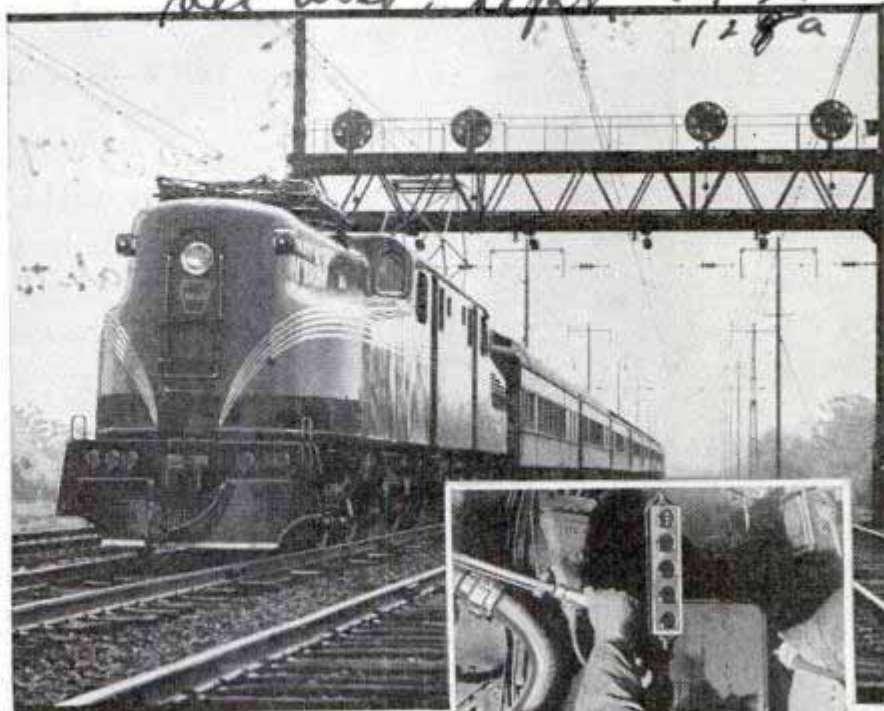
Coil in front of locomotive's pony wheels picks up varying frequency current from track and operates signal lights in cab
