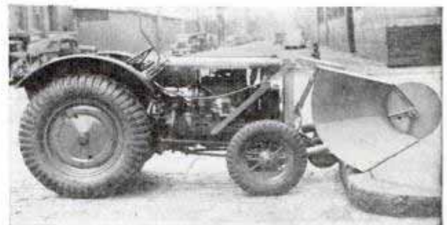
Curved scoop mounted on tractor cleans street up to curb and then climbs sidewalk to finish job
