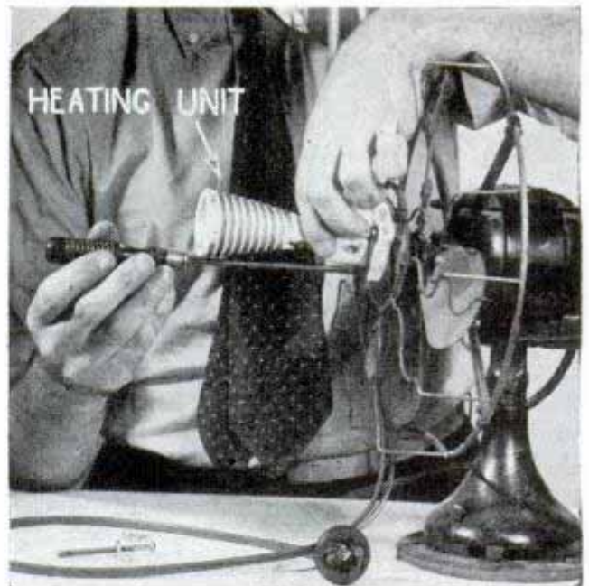
Electric heating unit attached to guard of electric fan heats air to dry photo prints quickly
