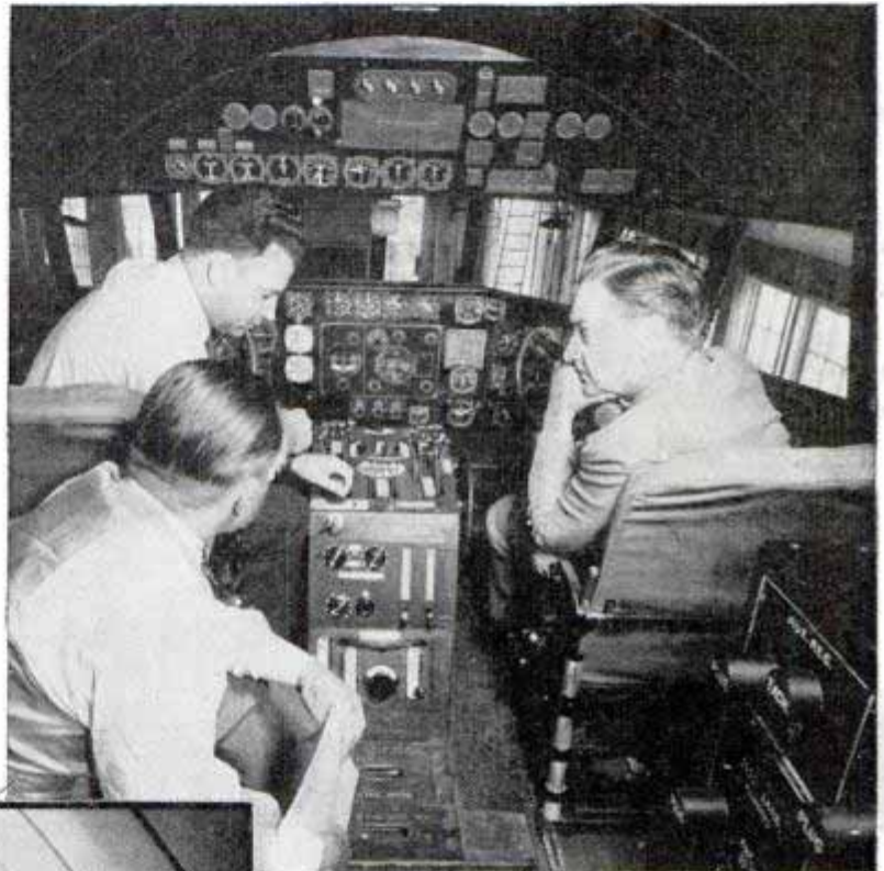
Boeing Clipper Wide World Top, pilots and engineers studying mock-up of cockpit instruments and controls of the giant four-engined transport. Bottom, part of ladies' dressing room on planes being built for TWA
