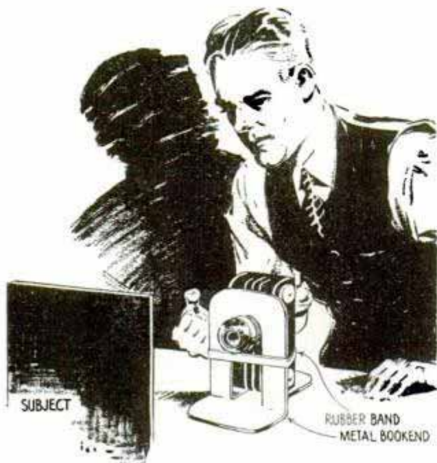
Stamped-metal book end supports miniature camera steady for copying or taking portraits
