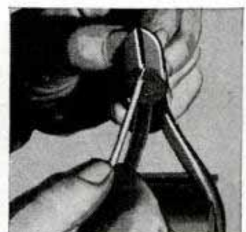
Below, cutting pliers clamped in vise provide a simple means for quickly stripping insulation from the ends of wire when numerous pieces are required for circuit connections. Separate the jaws a little more than the thickness of the wire at the hinge, pull wire down and outward to remove insulation
