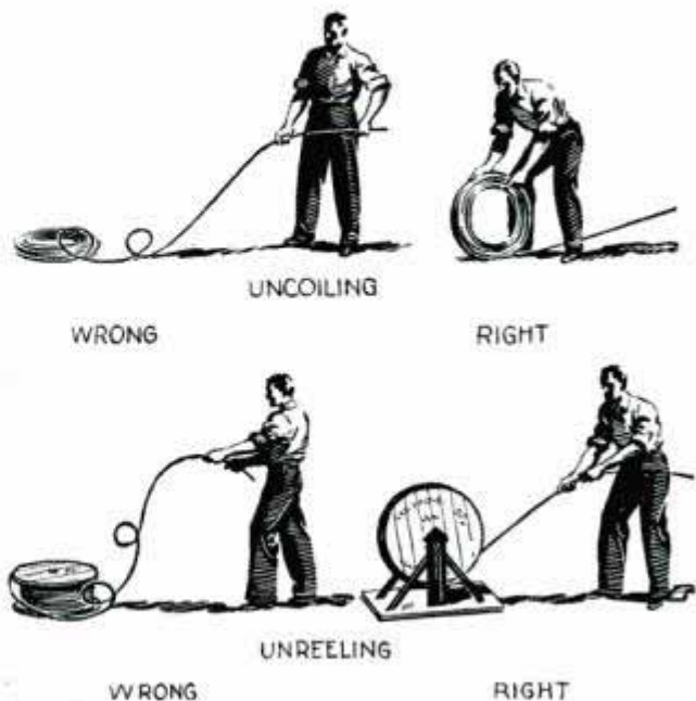
Life of wire rope determined largely by the way it is handled in uncoiling or unreeling
