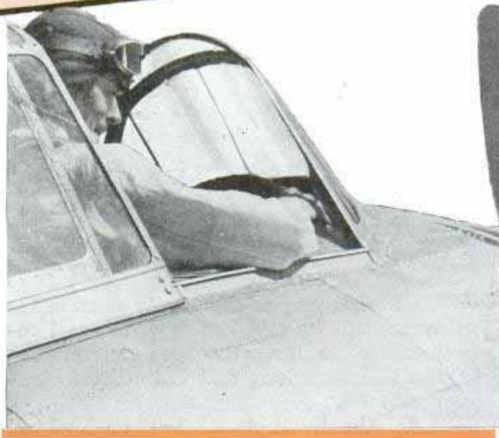
Transparent canopy slides forward and protects pilot from air blast in tests
