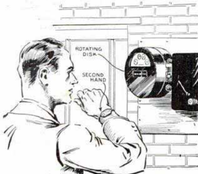
It's easy to figure current consumption of electrical appliance that does not have wattage on nameplate
