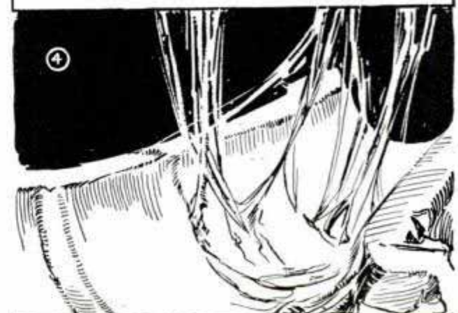
Before the aggregate sets, the webs are lifted out of the molds
