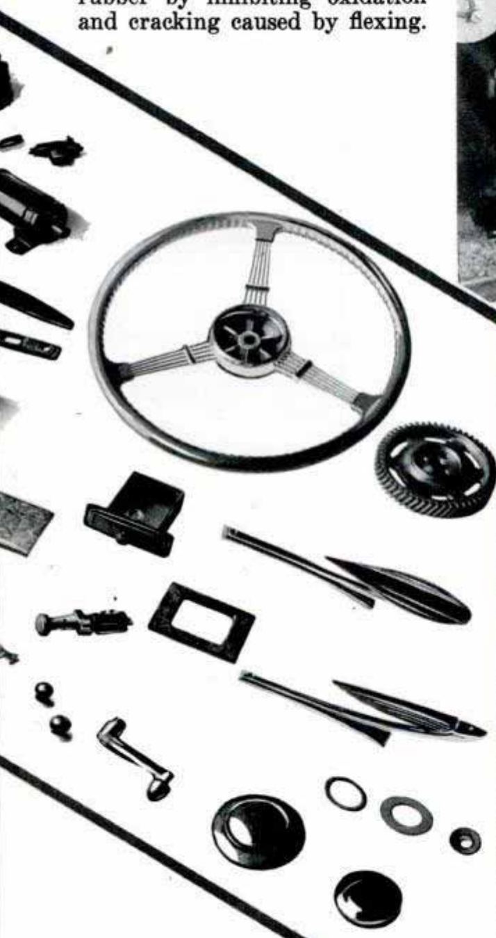
PLASTIC materials used in Hudson car, including wheel, ignition parts, timing gear and washers, interior fittings and radiator ornament.
