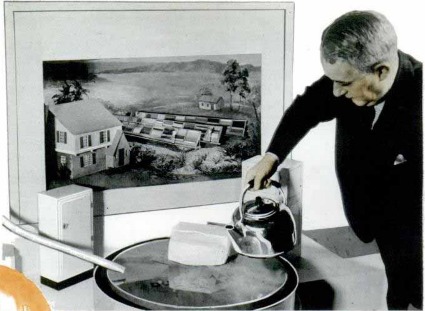
DEMONSTRATING the durability of a synthetic resin finish by subjecting it to temperature of "Dry Ice" and then to boiling water.
