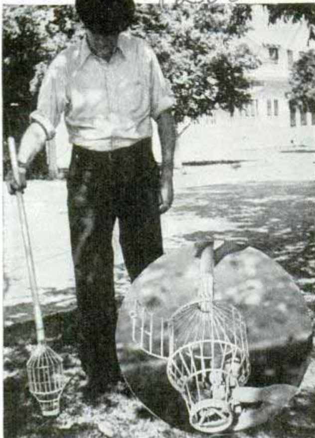
Picking up nuts with "bird-cage" harvester. Inset shows triangular springs that grasp walnuts
