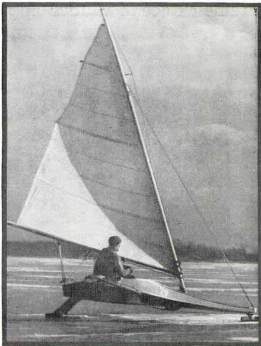
Top, heeling over a bit as he makes a turn. Bottom, view of "Skeeter" showing springy type of runner plank most satisfactory for attaining high speed on the ice
