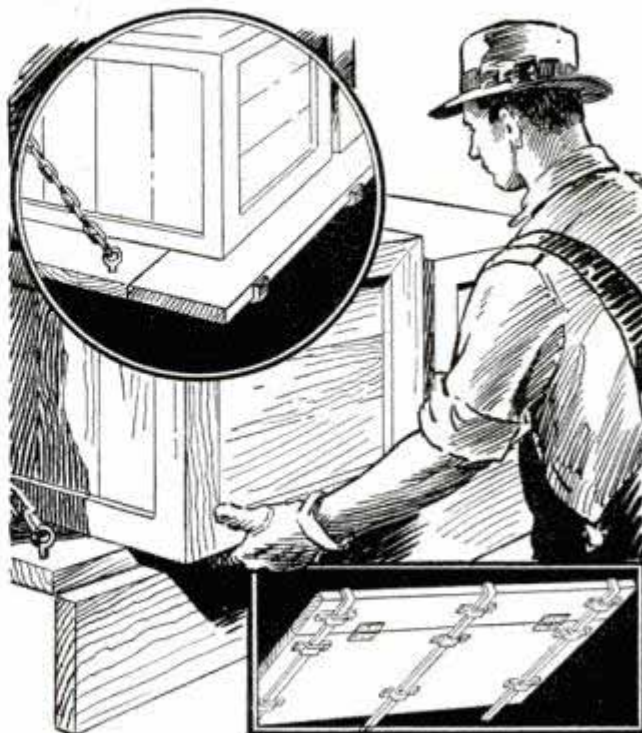
Boxes extended onto a lowered tailboard easily unloaded if upper part is hinged to drop down
