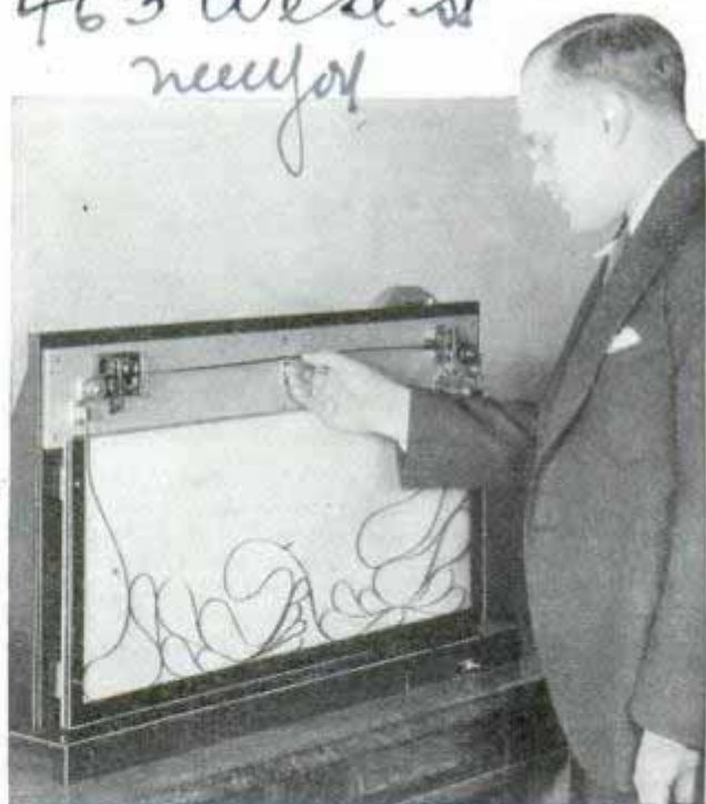
Magnetized steel ribbon on which telephone message is parked until repeated on loudspeaker
