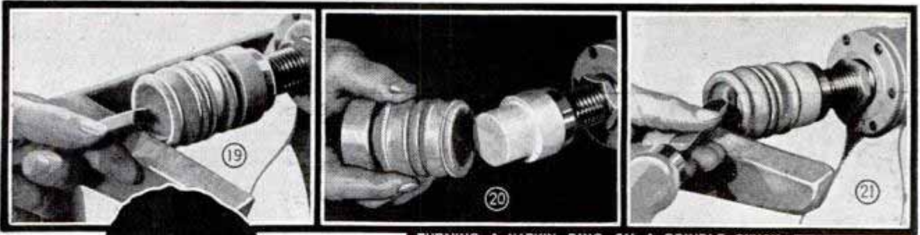
TURNING A NAPKIN RING ON A SPINDLE CHUCK
