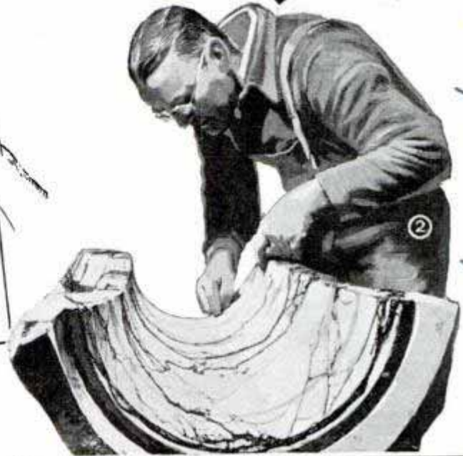
After webs are dipped in colors the bundles are spread and arranged in the greased mold
