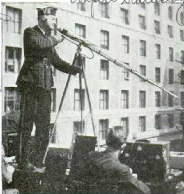
Aiming the machine-gun microphone at source of sound, a passing parade
