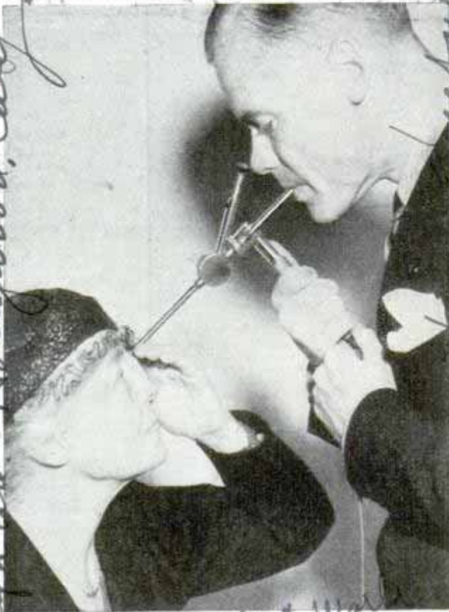
Both teacher, at left, and speaker can "see" latter's voice through tube containing maze of mirrors
