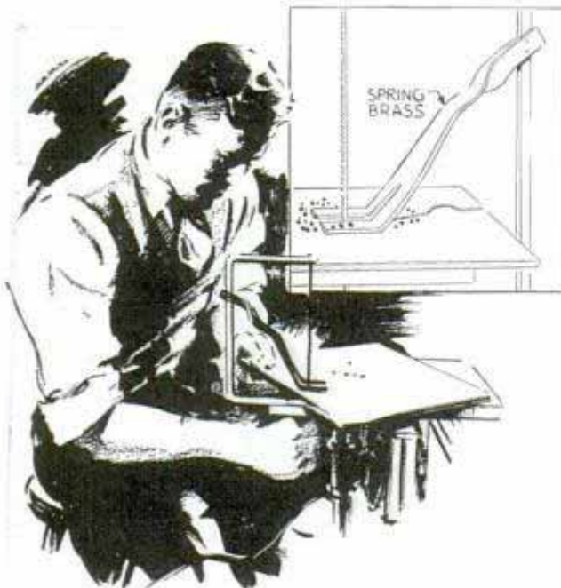
This pressure foot will keep small or thin work from moving up and down while cutting it with coping saw
