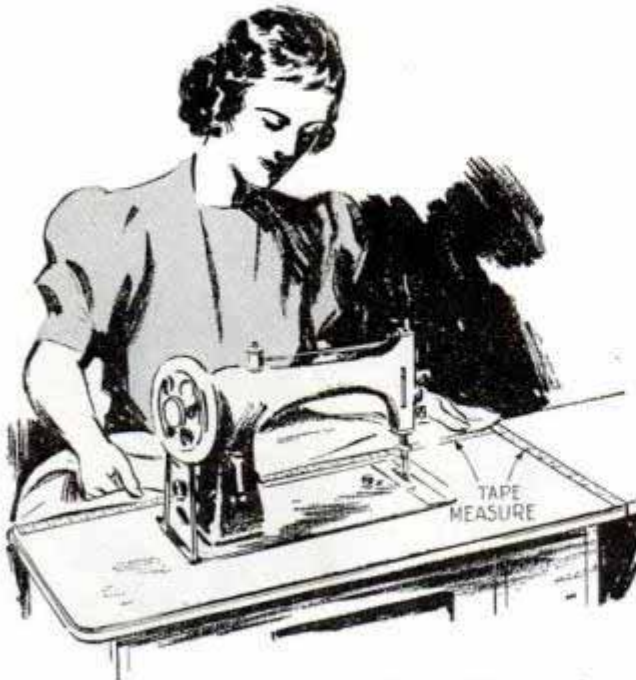
Scale along edge of sewing-machine cabinet is always at hand for quickly taking measurements
