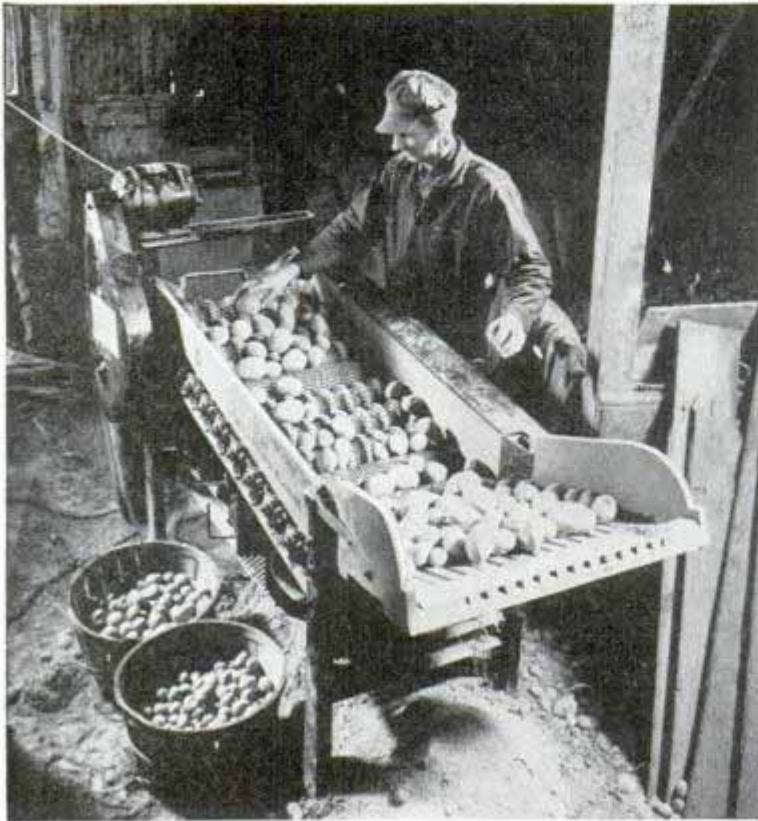
Here is the potato cleaner and sorter in operation. Electric motor at rear end drives the rubber-finger mechanism
