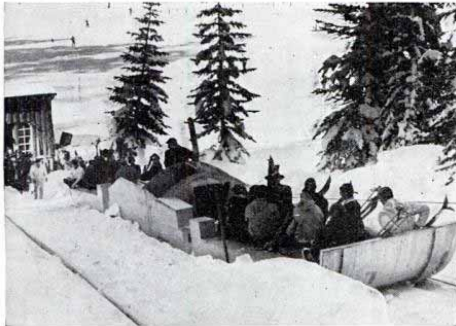
Double sled with motor at center hauls ski parties in Yosemite Park
