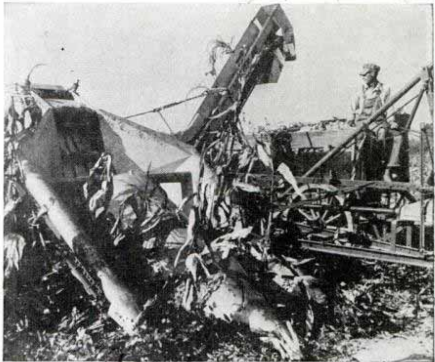
Working on two rows at a time, this mechanical corn picker harvests 800 bushels a day, squeezing ears from stalk and loading them into wagon
