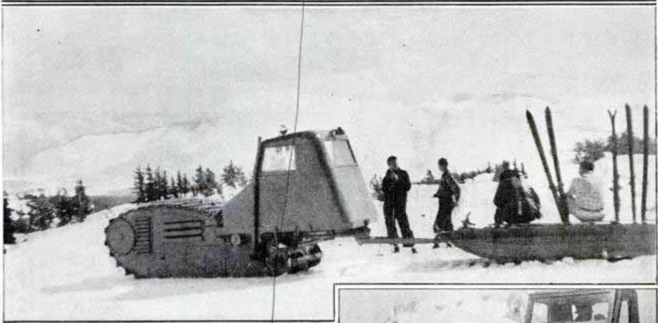
Ski party boarding twenty-five-passenger sled for ride up mountainside behind tractor. In front view at right, notice single track made of angle irons which grip snow
