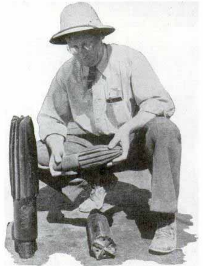
Milling tools used for curving well to reach oil pool at one side of derrick site
