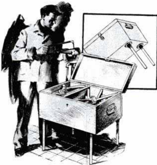
Plumbers and others will find this tool-chest bench handy on jobs away from the shop
