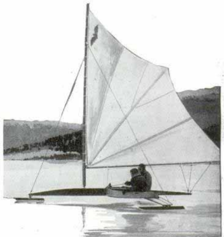
Here is another view of the front-steered boat rigged with batwing sail
