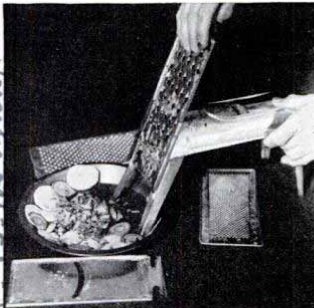
Feeding vegetable into shredder. Note that danger of injury is reduced
