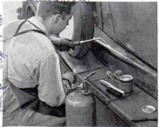
Tinning on auto is made easy with steel wool and a new granular flux
