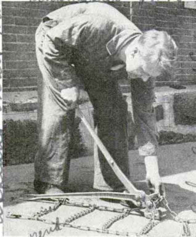
Closing new link in tire chain after worn link has been spread open and removed by second jaw of tool
