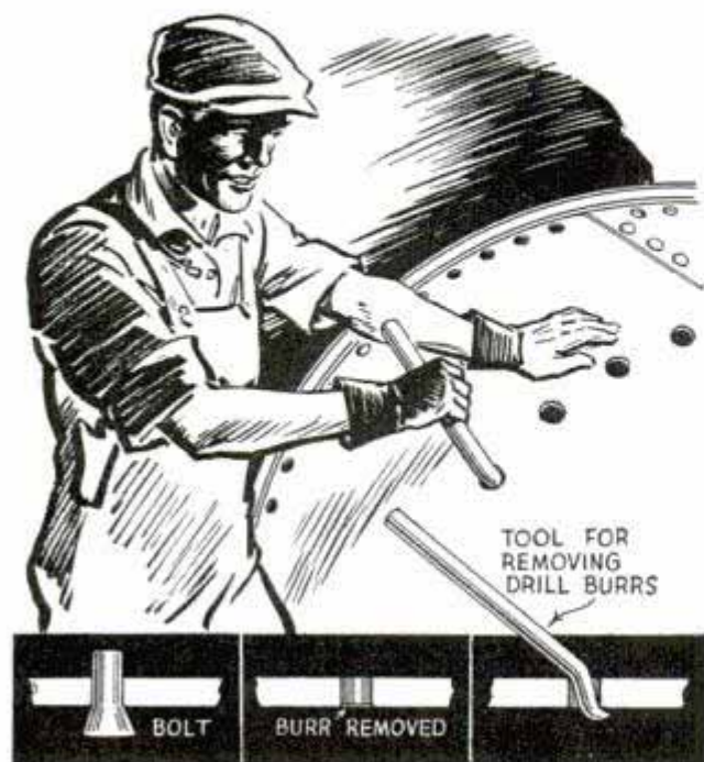
This tool quickly removes burrs from holes drilled through boilers and other cylindrical objects
