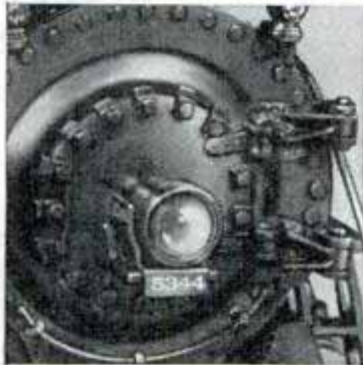
Headlight is projected in parallel beams through optical lens. Lamp is concealed inside the smoke box.
