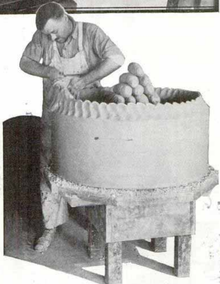
Top, operator reading spectrum plate with instrument which discloses tiniest fractions of an element. Inset, spectrum plate. Bottom, making glass melting pots from clay
