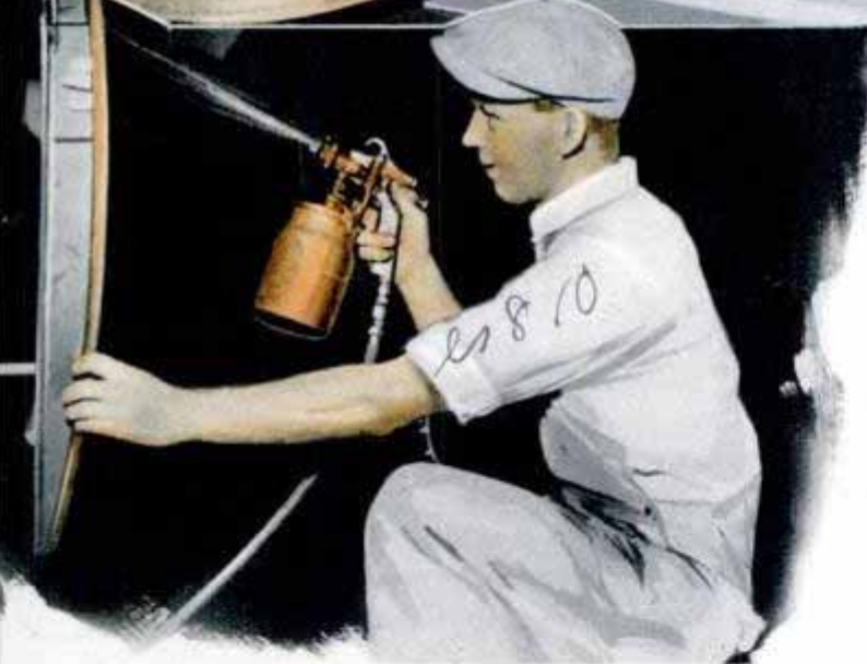
SPRAYING body of car in Pontiac plant. Durable, quick, drying finishes developed by chemistry have made possible the mass production of automobiles. Top, demonstrating a chemical agent for flameproofing fabrics. Untreated fabric is at left, the treated one at right. At far left is treated mattress on which gasoline has been ignited. The gasoline burns, the mattress does not catch fire.
