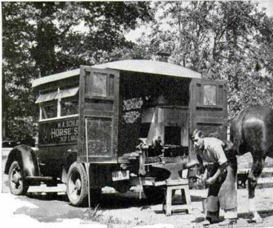
This blacksmith shop installed in a truck enables the operator to drive in search of business and to do the job right on the spot
