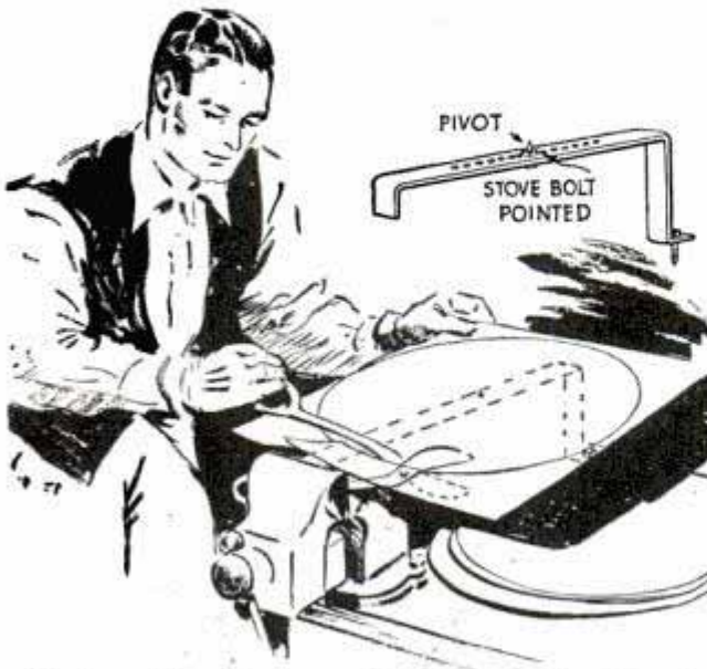
Sheet metal rotated on adjustable pivot bolt to cut disks of almost any desired diameter
