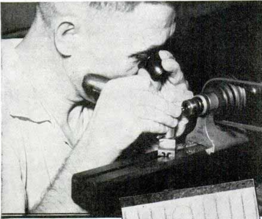
Top, centering photographic lens. Center, magnified view of tiny lens on millimeter rule. Bottom, Elmer Cronk, who has spent fifty-six years grinding tiny lenses
