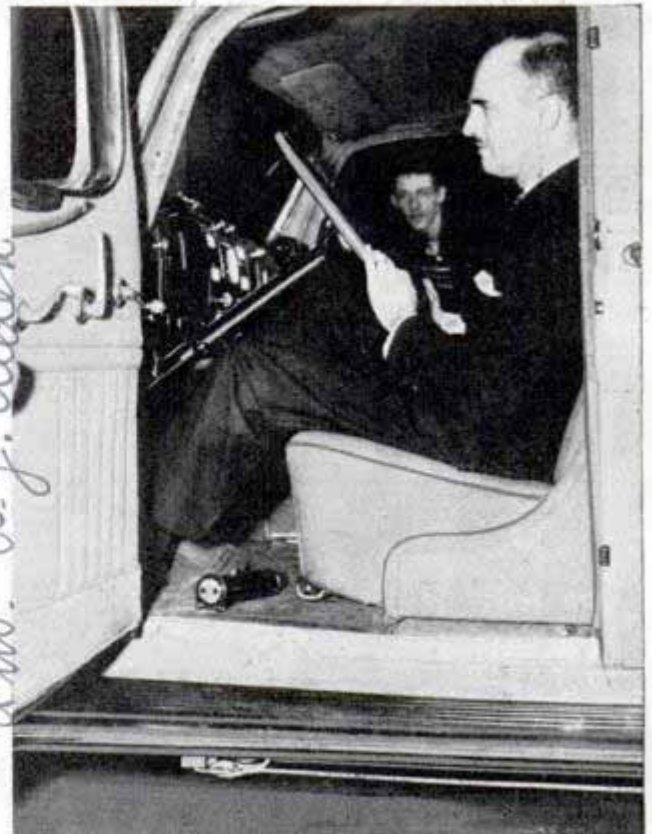
Checking up on safety of automobile brakes with flashlight tester, seen on floor of car
