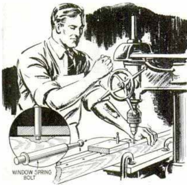
Boring jig on drill press has self-engaging indexing pin for boring evenly spaced holes
