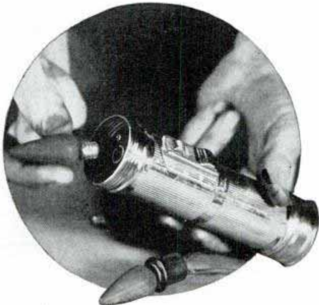
Screw those questionable Christmas-tree lamps into your flashlight to see if they are in good condition
