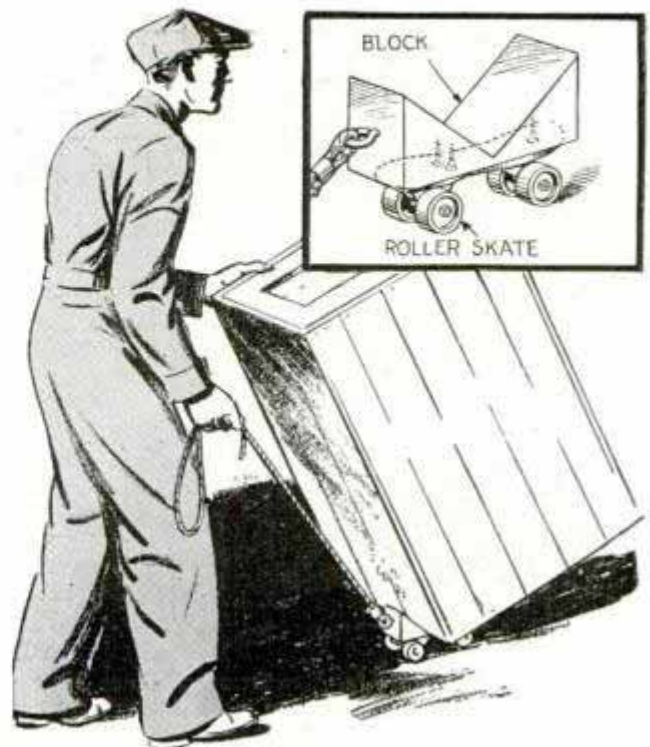
Heavy boxes and crates up-ended on this V-block dolly are easily moved
