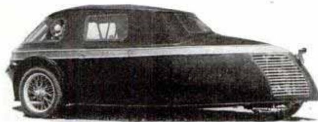
What looks like radiator grille at right is really the rear vent of air-cooling wind tunnel through car
