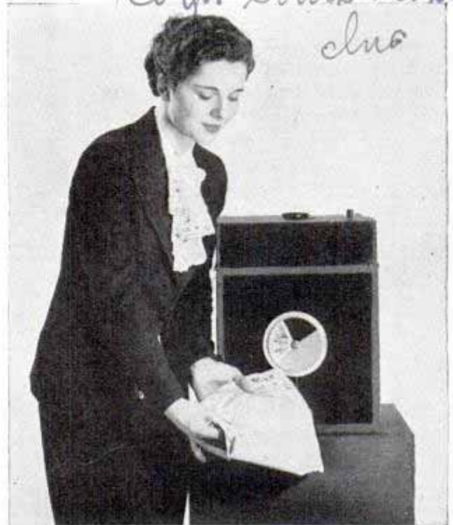
When the tri-colored wheel is rotated rapidly the blend will match fabric's color
