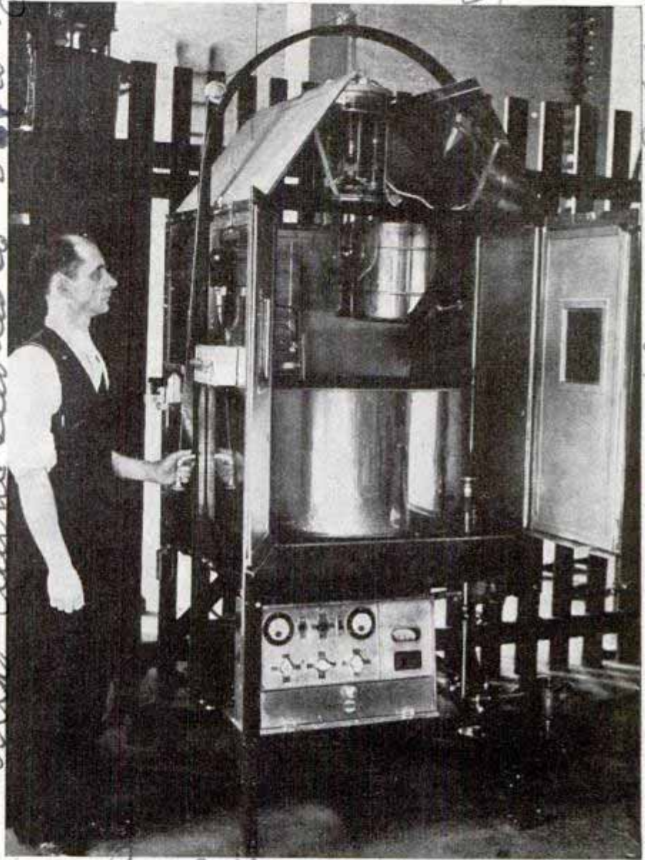
You can literally "turn on the weather" in this cabinet, designed to test the durability of paint, rubber and other materials
