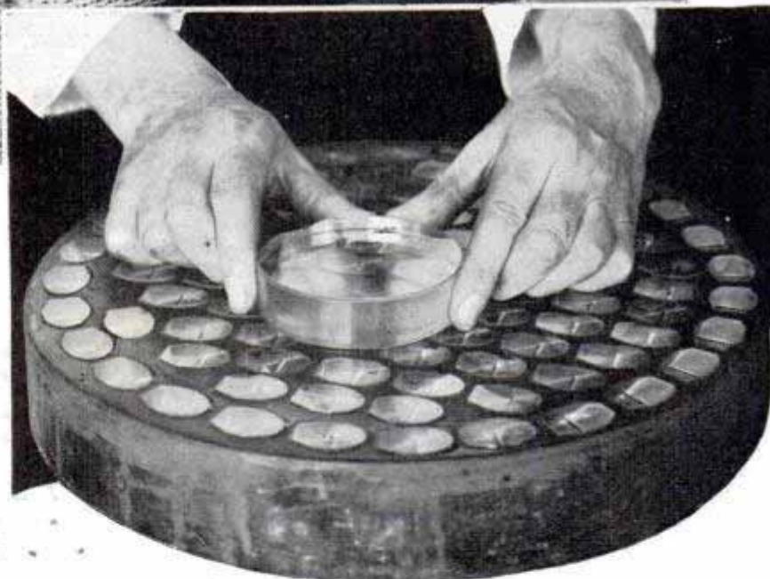
Top, scientists check spectrograph built for Maj. Albert Stevens' stratosphere flight. Bottom, testing binocular prisms with an optical flat to determine accuracy of their surfaces
