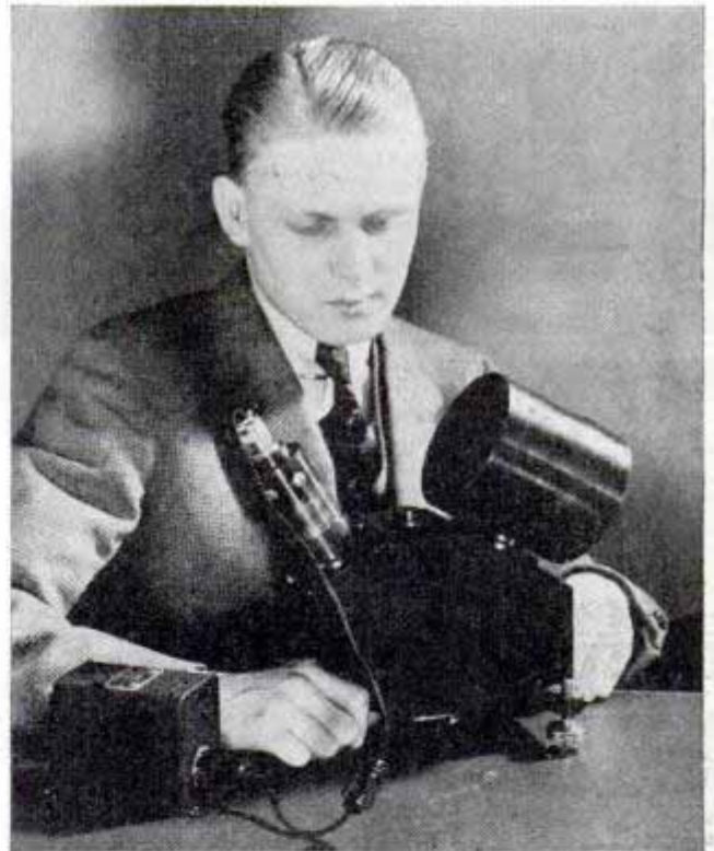
The vibrometer which photographs jolts and jars and measures vibrations
