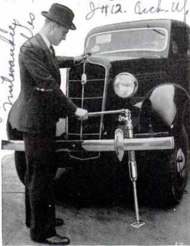
Notice pump and release valve are at top of hydraulic jack and motorist can pump while standing
