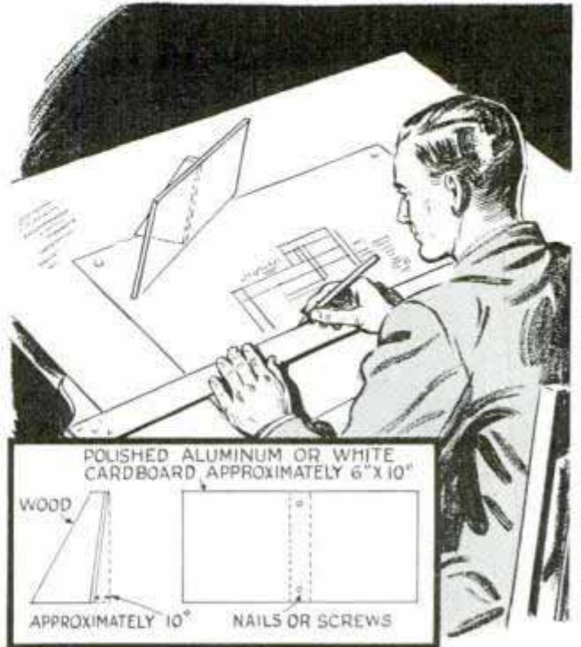
This reflector is quickly adjusted to direct a soft light on any part of a drawing board
