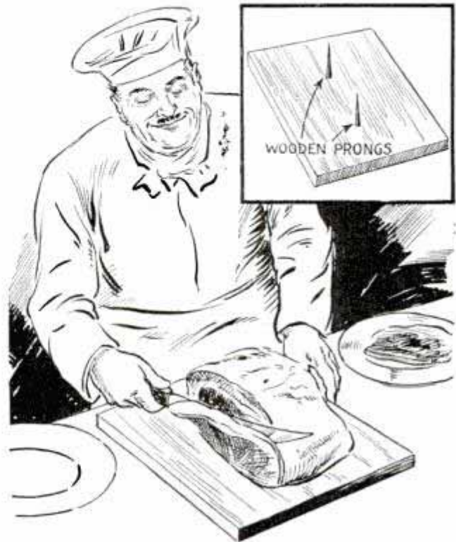
Roasts, chickens, etc., are easily sliced when impaled on the prongs of this carving board
