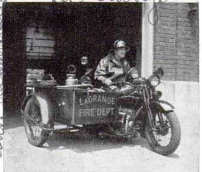
All equipment necessary to battle small fire is packed in sidecar of motorcycle, inexpensive to run
