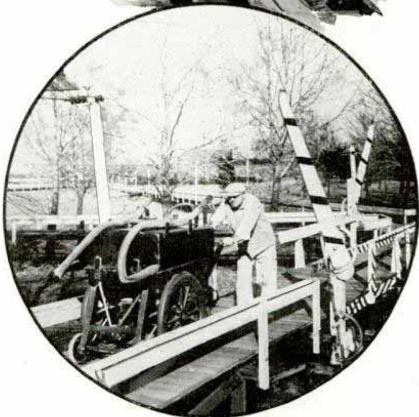
Top, taking loose dynamite from mixing house to cartridge packing machine. Bottom, wheeling nitroglycerin "buggy" from store house to mixing house. Note semaphores and railing to protect the "buggy" and its contents
