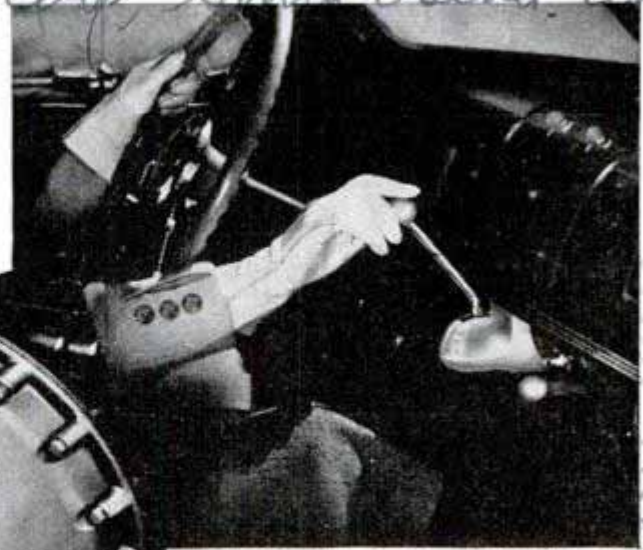
Top, vacuum shift lever. Center, transmission shown turned on its side. Bottom, vacuum shift. Shift lever is at top right. Exhaust manifold from which power is derived is at upper left. Vacuum booster is at center bottom, and transmission at bottom right
