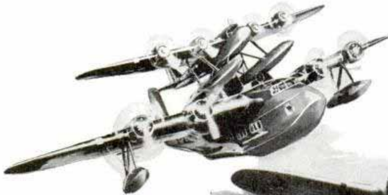
Top, the composite aircraft, consisting of large plane and smaller ship on top, in flight. Bottom, the "mother" plane landing after a test hop. This arrangement is intended to help heavily loaded planes to start long journeys without the usual takeoff problems
