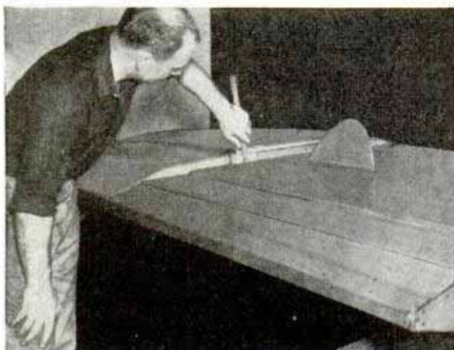
Bottom of outboard racer, showing small step and overlapping longitudinal steps
