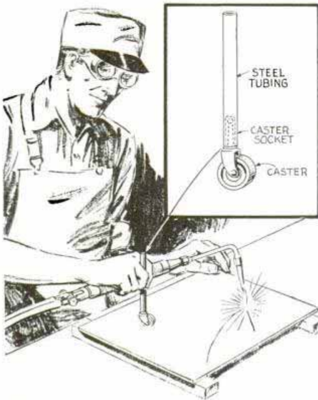
This support for welding torch allows it to be manipulated without undue strain on the arm
