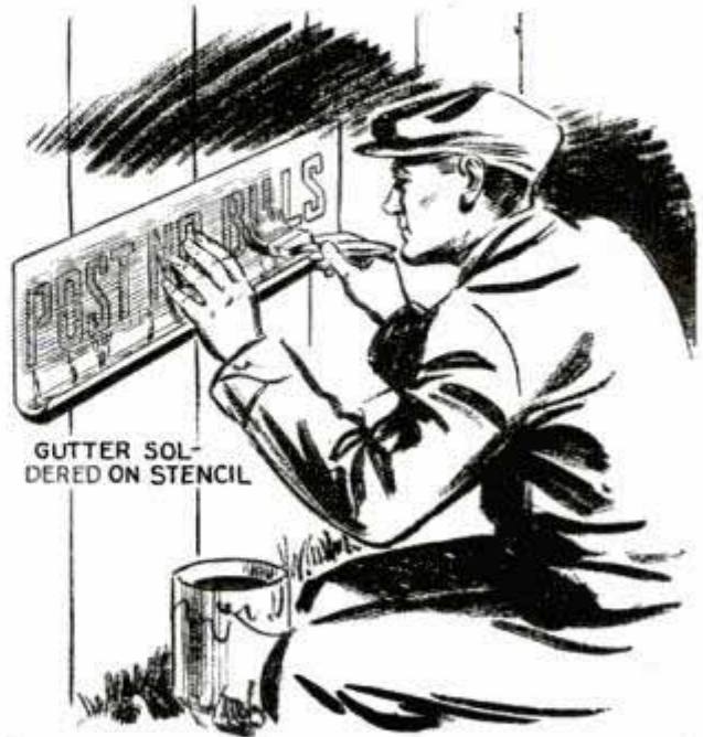
Gutter on bottom of sign painter's stencil catches surplus paint to avoid marring finished work
