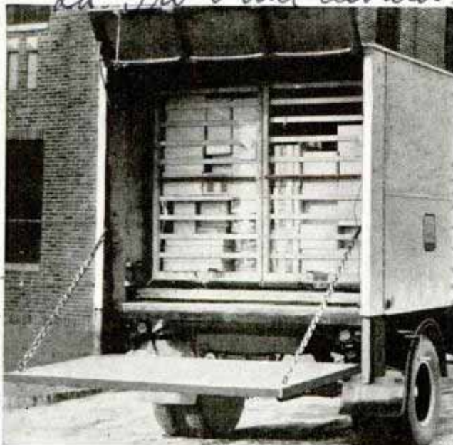
Heavy merchandise can be loaded or unloaded from truck by using tail gate as elevator run by motor
