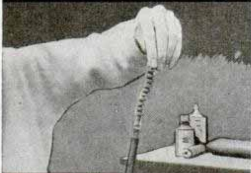
To clean barrels of shotgun, run this brass wire brush through them
