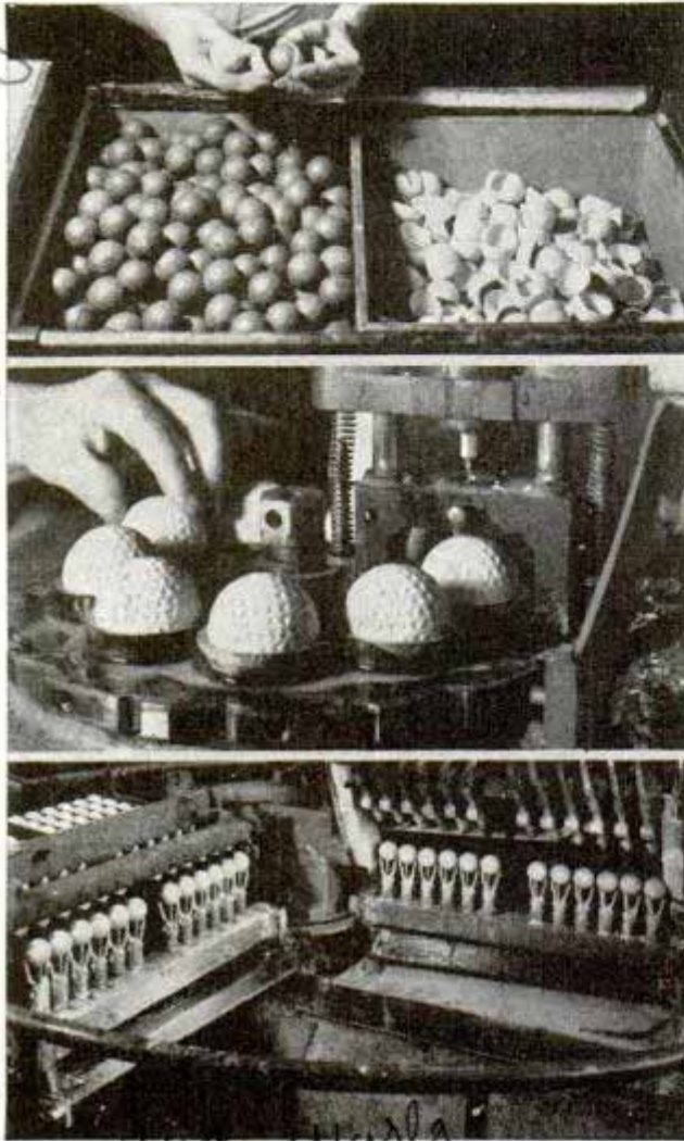
Top, putting cover on core; middle, needling, and bottom, spraying durable white paint on golf balls
