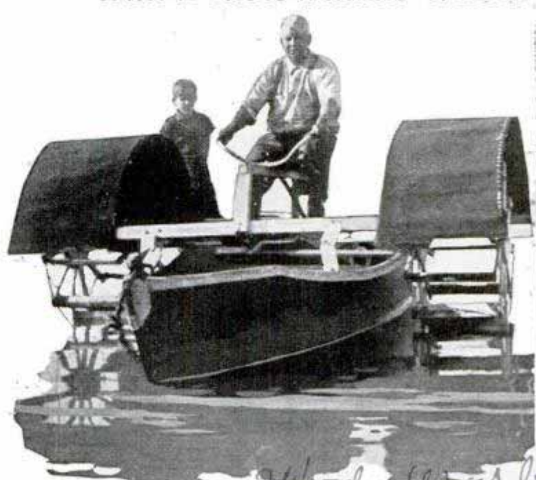
Here is a rowboat that is pedaled instead of rowed. A bicycle frame is mounted in it, and the pedals turn paddle wheels
