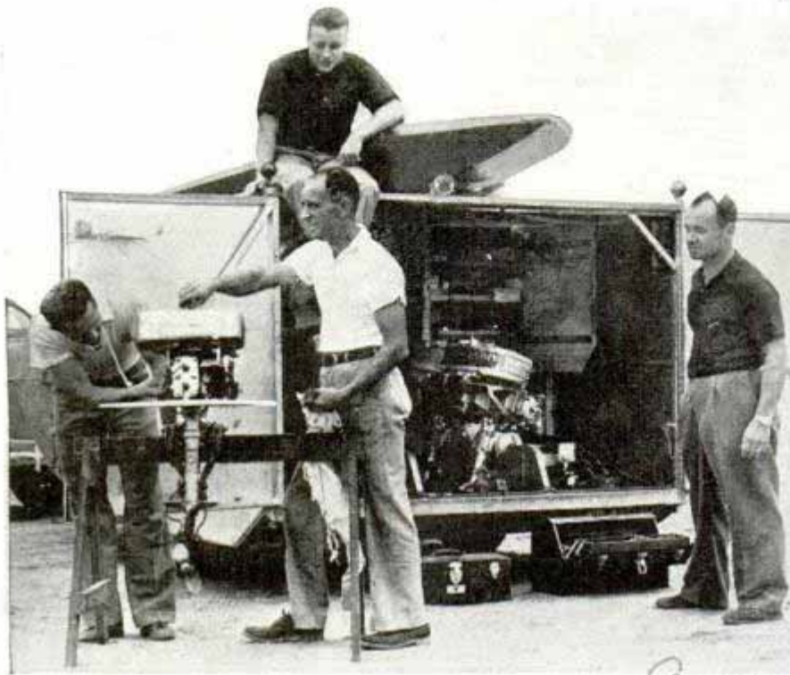
This auto trailer not only houses a repair shop with complete equipment for overhauling outboard motors, but carries five boats on its roof
