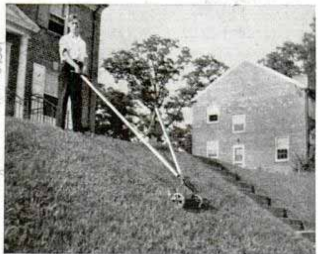
This extension handle on lawn mower makes it easy to cut grass on slopes
