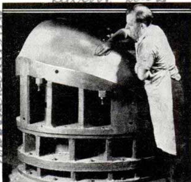
Administering a final polishing to one of the big steel dies that will shape automobile fenders
