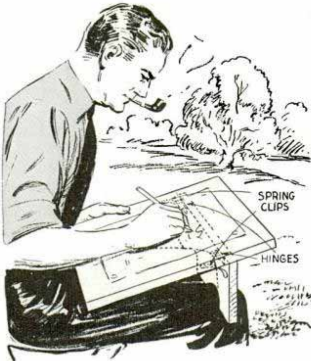
Both your hands are free when you use this hinged support on your portable sketching board
