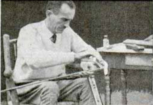
Small patch moistened with nitro solvent dissolves powder in barrel
