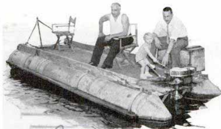
Acme This raft on pontoons is handy for water sports. Propelled by outboard motor, it attains a speed of seven miles an hour
