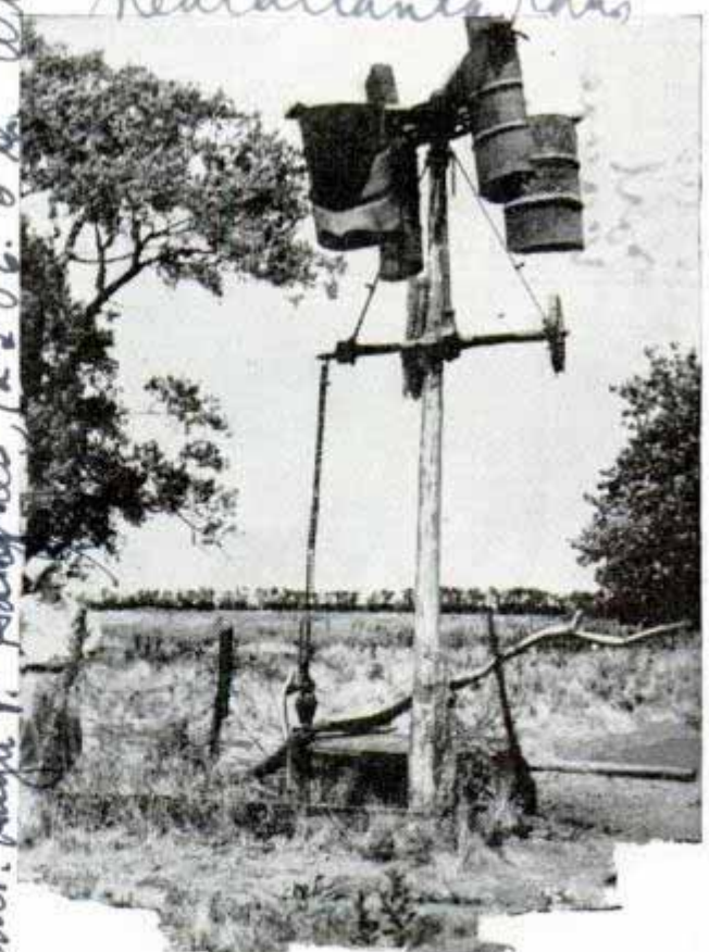
As wind turns half-barrels, drive shaft and rear axle of junked car revolve and pump water
