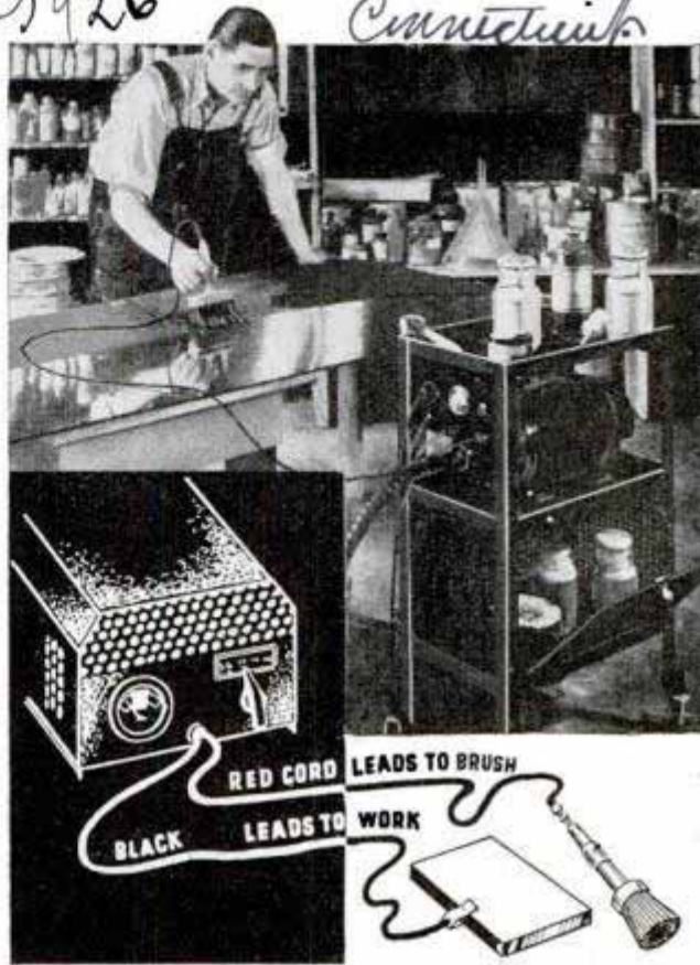
"Painting" metal on metal with the electroplating brush. Drawing shows electric circuit.
