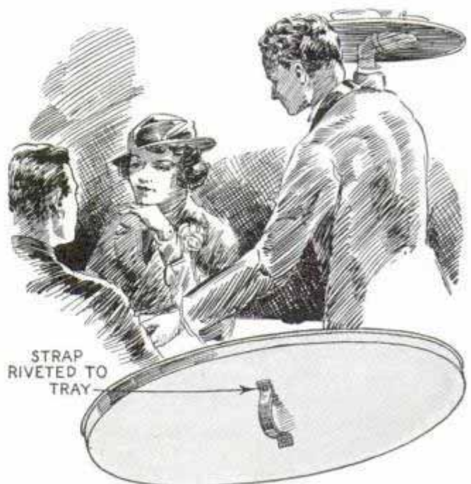
Hand loop on bottom of serving tray enables waiter to carry it without danger of slipping
