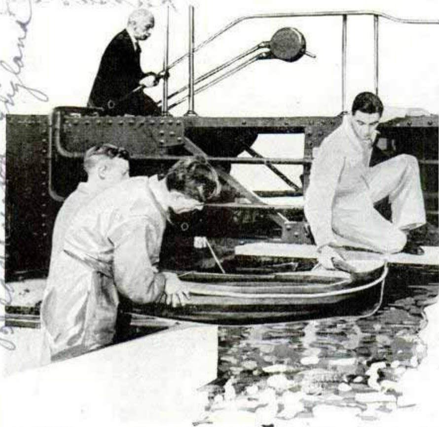
Model lifeboats are given a real test of their seaworthiness in man-made "storms" on the water in an English laboratory
