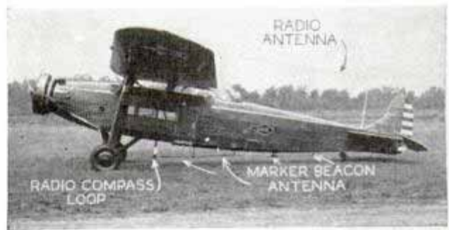
Plane used in experimental landings is equipped with three types of radio antennas
