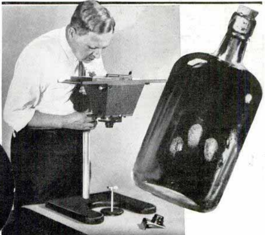
Top, comparing shoe with footprint obtained by moulage. Center, how fibers and human and animal hairs differ under microscope. Below, orthostereo camera and fingerprints on bottle. Left, fingerprint magnified
