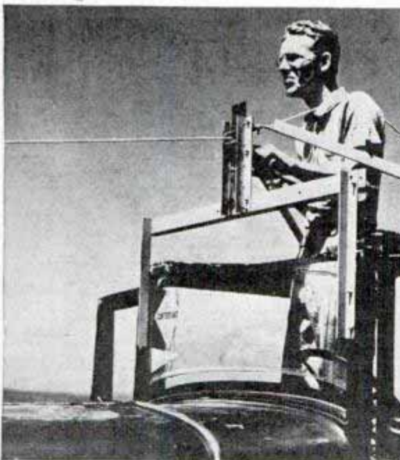
Above, sometimes the rope with which the glider is launched into the air by towing becomes entangled. This apparatus for guiding the tow rope on top of an automobile is equipped with a heavy knife which cuts the rope if the pilot is unable to cast it off his ship. Note the close attention with which the operator watches launching to guard against accidents. Right, utility glider making a flight at the eighth annual contest sponsored by the Soaring Society of America at Elmira, New York
