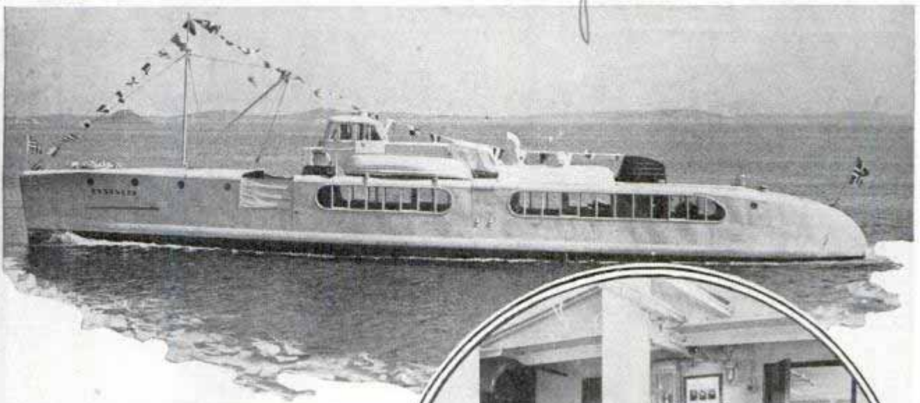
Streamline Diesel motorship built as passenger ferry and parcel carrier for Norwegian line. Notice seating arrangement, right
