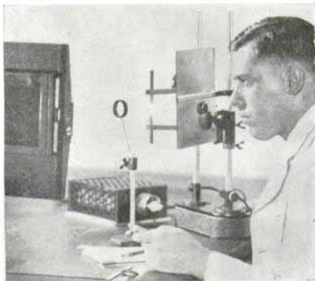
Small quartz spectrograph used for detection of metallic poisons in blood or viscera
