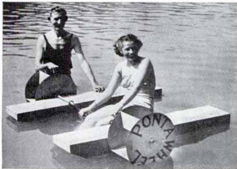
Here is the paddle-wheel watercraft. Note that it is propelled by turning the hand-cranks set on each side
