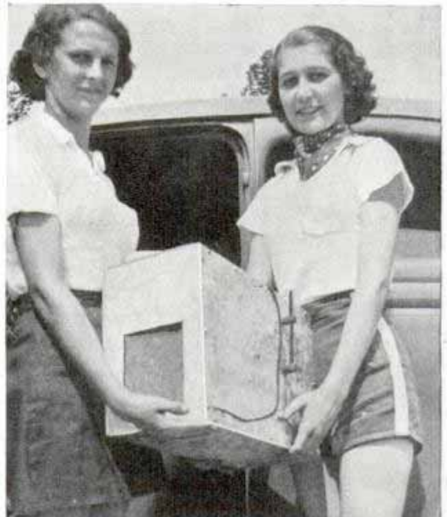
This home-built air conditioner using filter, fan and cracked ice cooled interior of car by ten degrees
