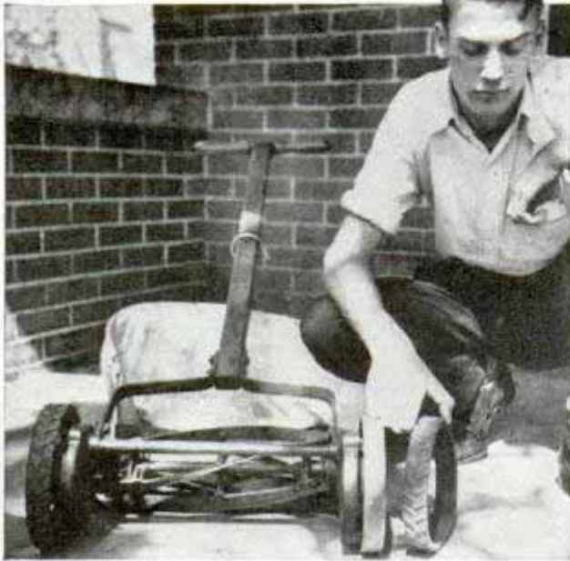
Here are demountable rubber tires that you can slip on and off the lawn-mower wheels without a tool
