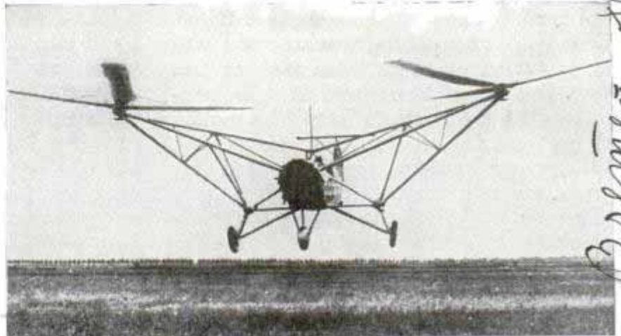
Twin-rotored autogiro leaves the ground for a test whirl over the Bremen airport in Germany. Observe its wingless framework
