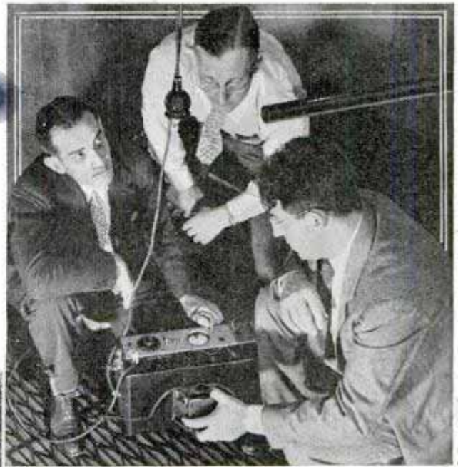
Top, measuring auto's noise piped from "silent room." Center, the vaultlike soundproof building. Bottom, moving an automobile into the building for noise tests. Note the double doors which help to keep air within two rooms so still that the silence is almost oppressive
