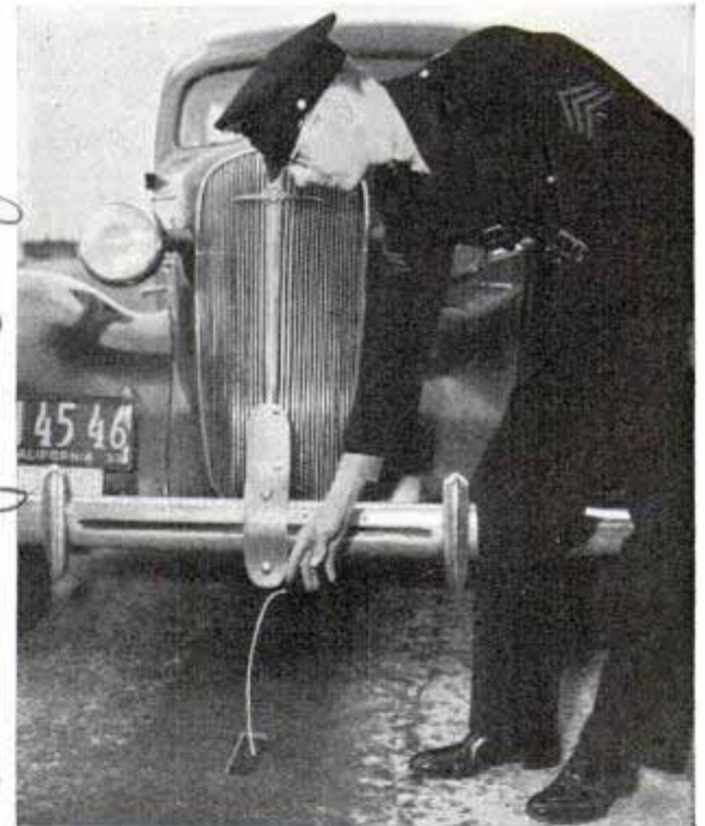
Showing "catwhisker" which short circuits static electricity from car to bridge
