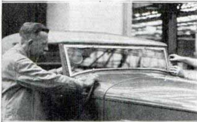
Using sculptor's clay to find means of reducing sound of wind blowing on windshield
