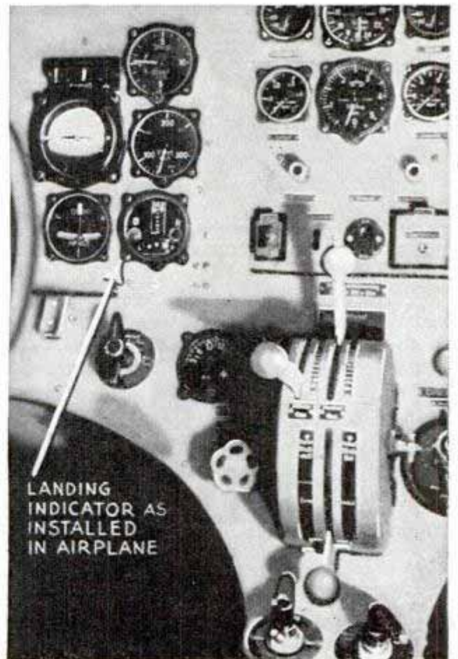
Above, inset, Lorenz visual indicator. Bottom, indicator mounted on instrument panel of plane in which numerous test landings have been made
