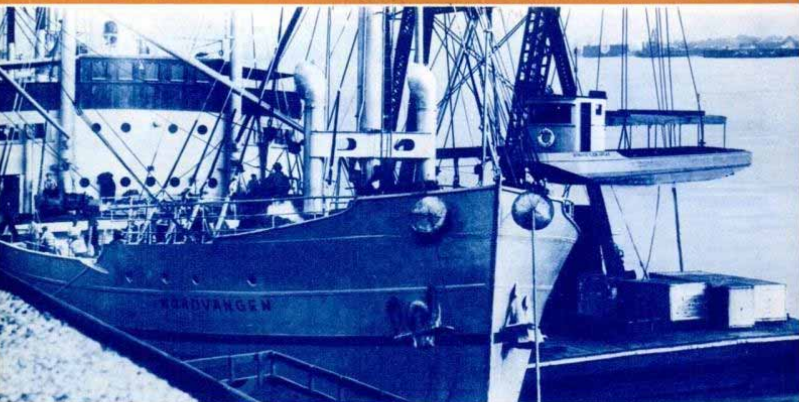
LOADING a forty-two foot "tunnel boat" built of steel, top, to deck of steamer. Below, boat with "spoonbill" bow negotiating shallow waters.
