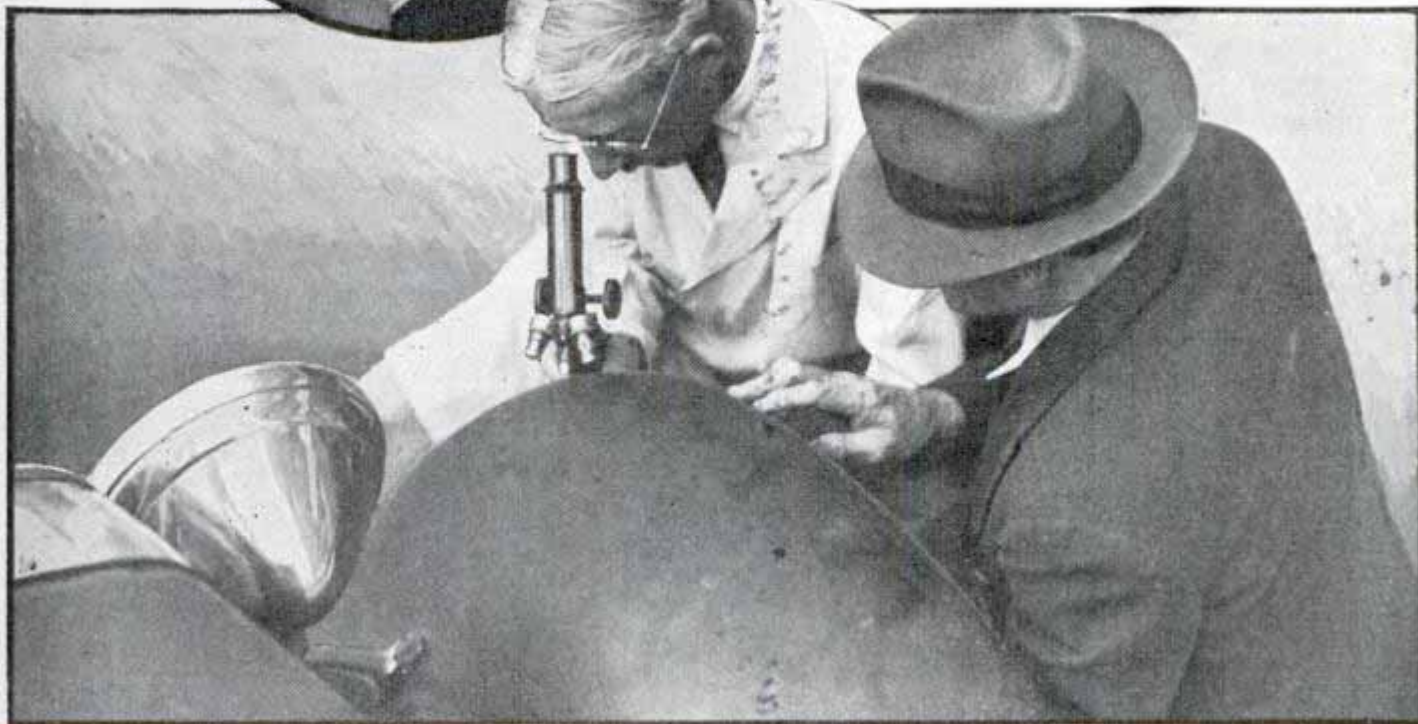
Top, examining kit of tools in burglary case. Center, taking a sample from steel safe for spectro assay to compare with shavings from suspect's drill. Bottom, using microscope to collect tiny flecks of material from dented fender to prove guilt of hit-run driver
