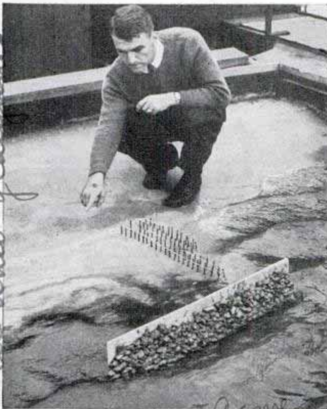
Model of ocean beach with tiny breakwater built to show whether it protects sand slope from waves
