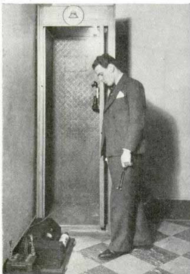
Transmitting photo by wire. Note distance from phone receiver to sending machine
