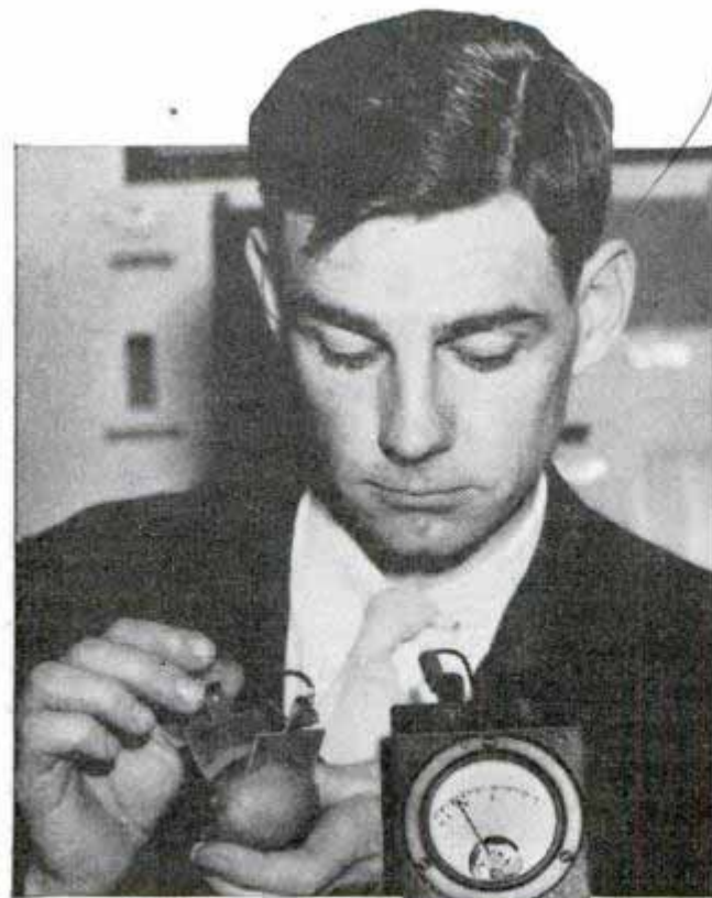
Reading the "current" from a lemon on ammeter connected to metal "spades" inserted in fruit
