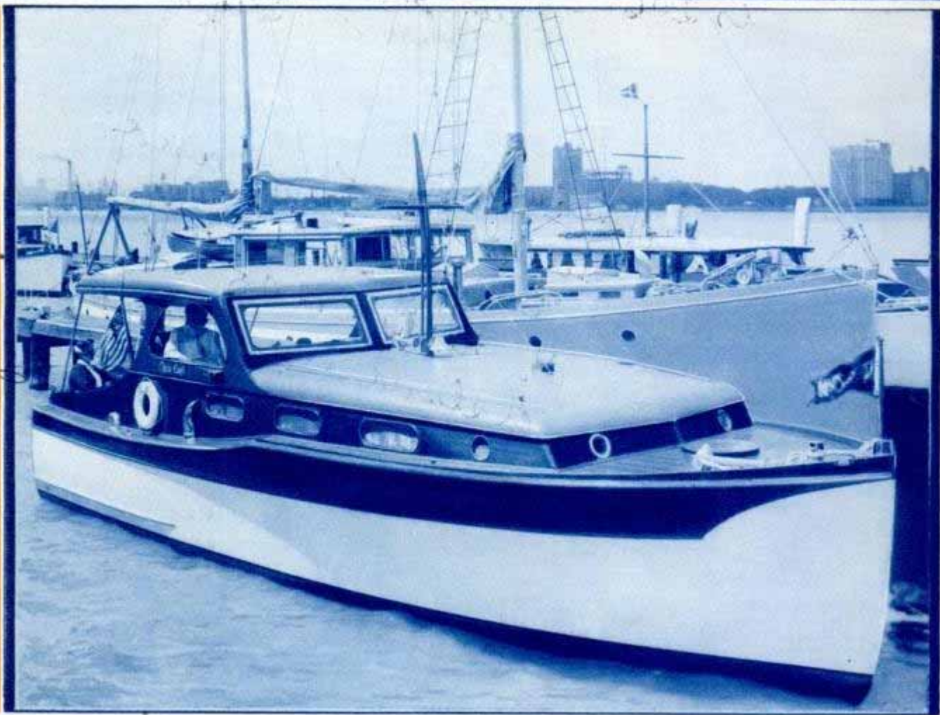
THIRTY-TWO foot double stateroom cruiser constructed of mahogany and white oak. It has a double-planked bottom.
