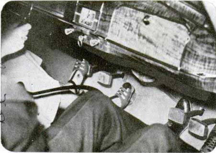
Note the second set of controls at right of car. This enables instructor to prevent accidents while teaching students to drive
