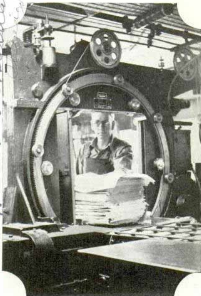
Newspaper bundle is tied with wire at touch of foot switch and then shoved on to conveyor to be shipped
