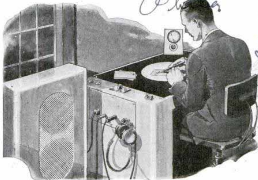
P. H. ... Peter Esterbrook Test operator writes on paper lying on special disk and sound of the pen's "scratch" comes out of the loudspeaker at left
