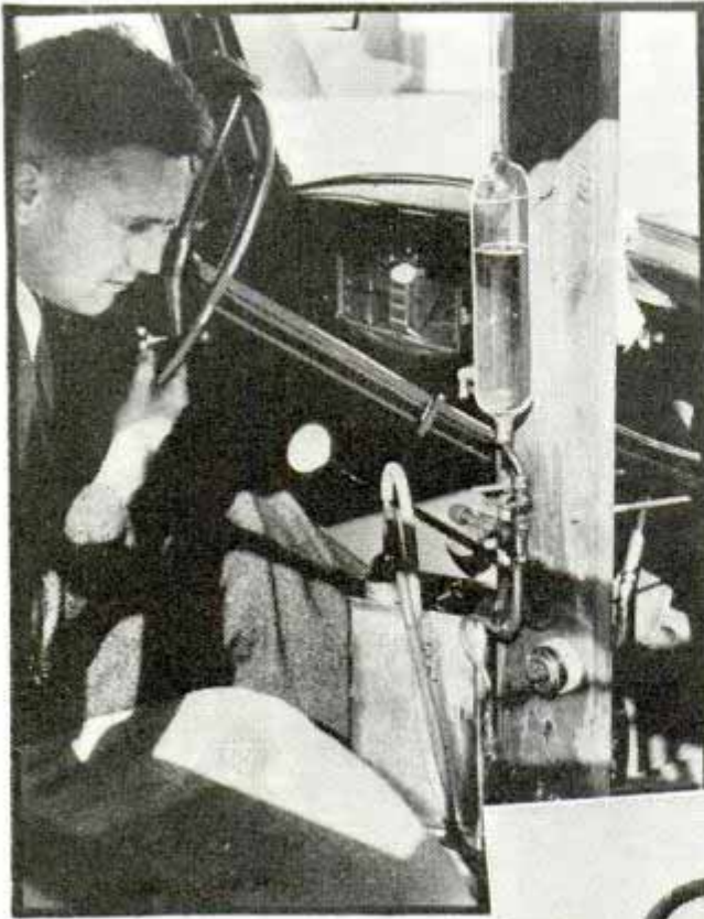
Above, driver testing power of new high-octane gasoline. Right, top of cracking tower in which evaporated petroleum molecules are broken apart into gasoline molecules
