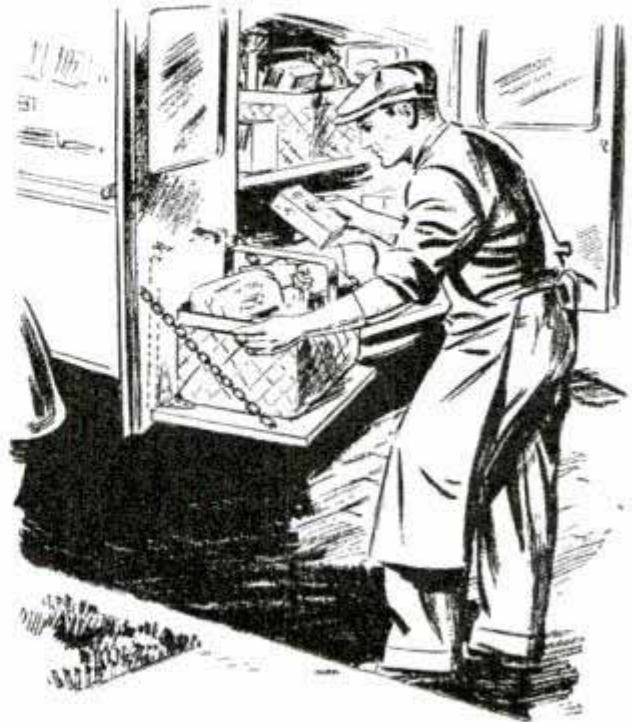
A hinged shelf on the door of your delivery truck is handy for holding baskets while sorting articles
