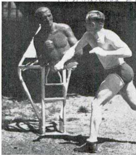
Left, boxer in training with robot sparring partner which weaves and rebounds in unexpected ways. At right is the robot with meter registering power of boxer's punch
