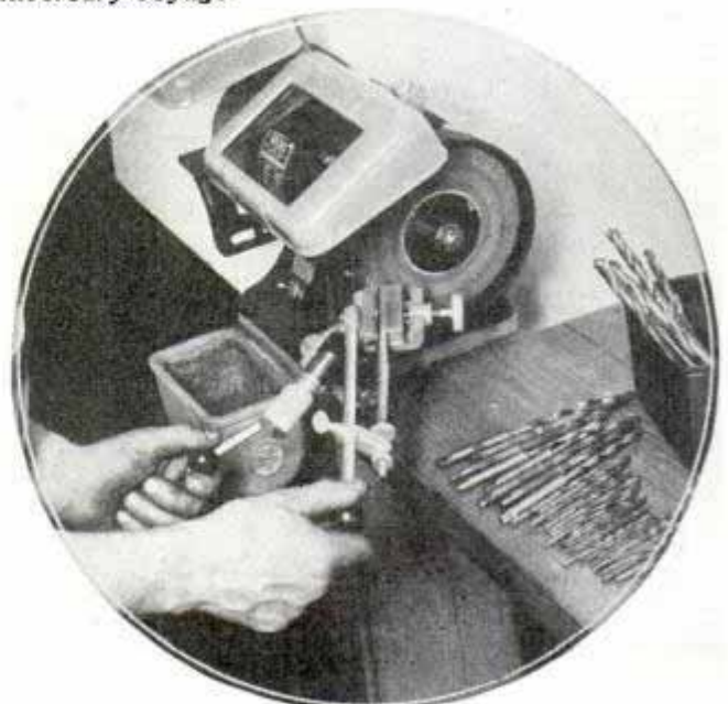
In two minutes you can sharpen a drill with this automatic grinder, which fastens to workbench
