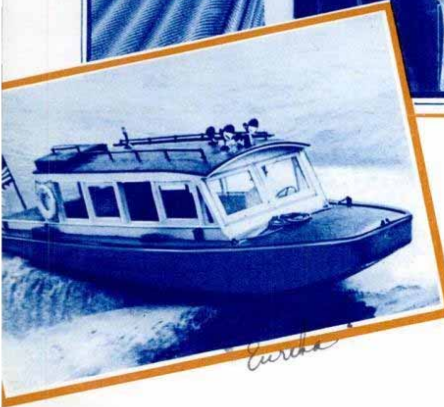
BOAT with "spoonbill" bow running over floating log. Such obstructions are no hazard to a craft like this. Top, thirty-two foot double stateroom cruiser which has a dinette convertible into a double bed and a lounge containing an upper and lower berth.
