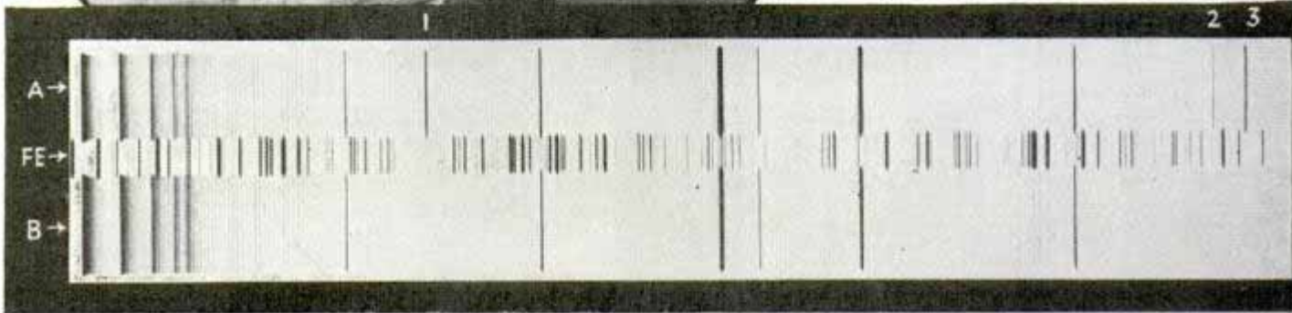
Top, taking sample of bogus coin in counterfeiting case. Bottom, spectrogram of two bullets in murder case. Note thallium lines, 1, 2 and 3, in Bullet A which are not present in Bullet B, showing the bullets to be different
