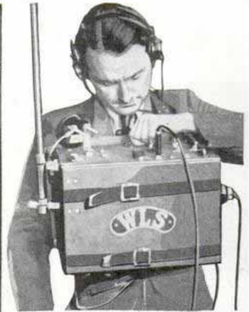
Left, a flying radio reporter obtains an interview in an airplane circling over the scene of a disaster. Right, field engineer "caddies" portable transmitter, batteries and mast antenna in covering remote story
