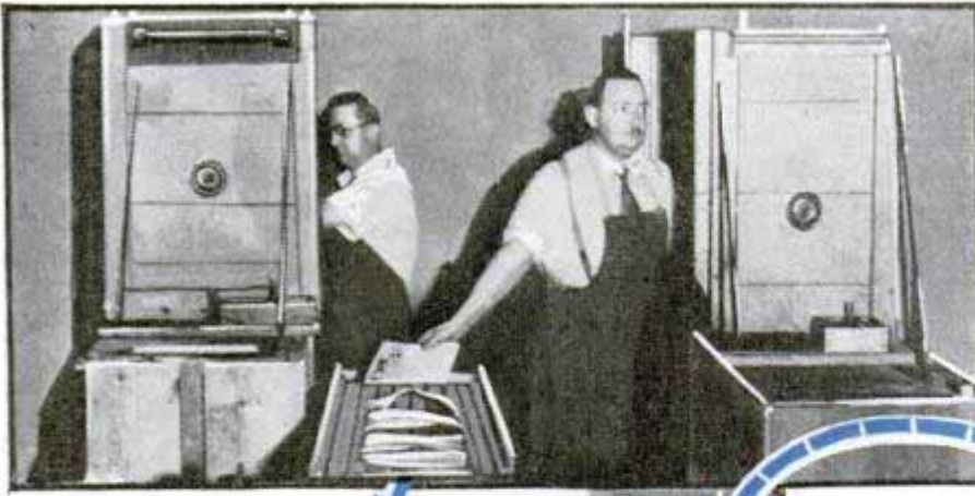
Top, center and right (following the arrow), steps taken in news-picture office. One negative received by telephone may be used in producing 7,000 prints in one day. Bottom, wired photo recording machine
