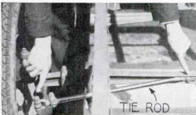
Sever the tie rod in the center and bolt the ends to the axle if you want to avoid trailer sway
