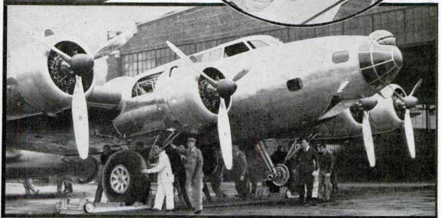
Circle, Designer Sikorsky in flying laboratory. Bottom, one of the four-motored Boeing bombers being built for U. S. army. It has 105-foot wingspread and weighs sixteen tons
