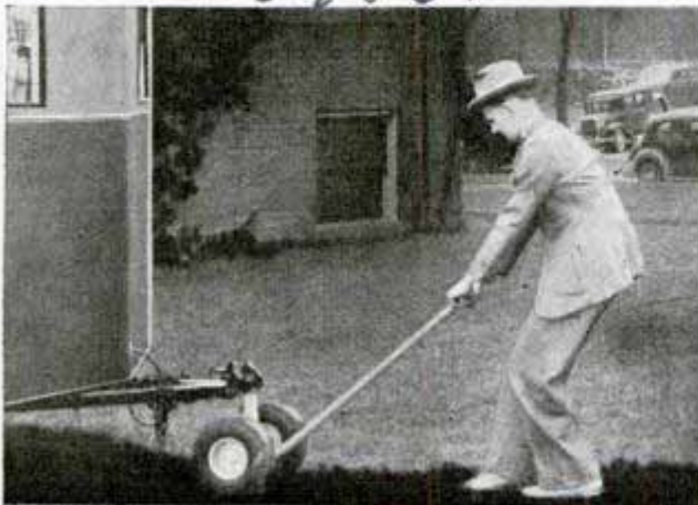
Pressing down handle of dolly lifts trailer off its parking wheel. It is easy to maneuver even a heavily loaded trailer in tight parking spaces
