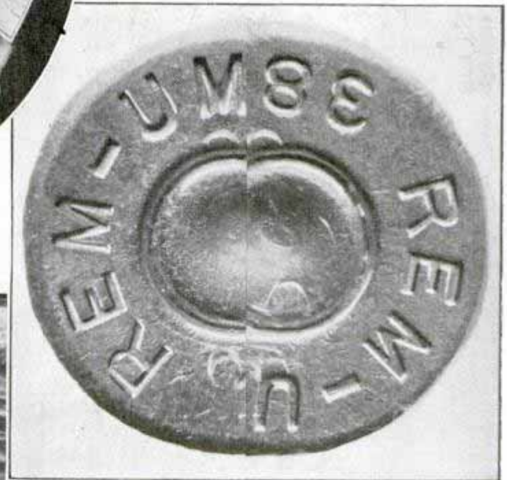
Left, photomicrograph of matched bullets. Note line of demarcation down center where two photos were fitted together, showing that the bullets match, therefore were fired from same weapon. Above, comparative photo of two shell heads, taken through the comparison microscope and camera. This shows similarity after shells have been fired
