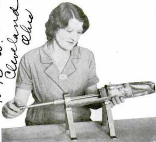
Ramming home an order of doughnuts with a transparent bag fitted over end of special doughnut loader
