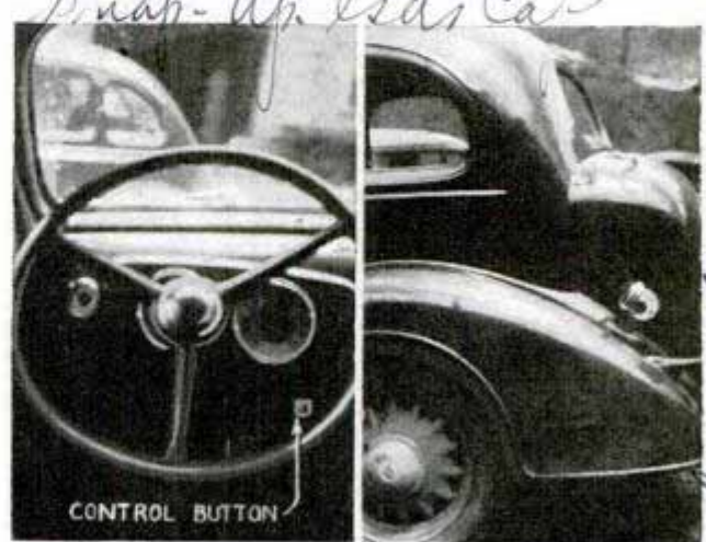
Left, control button on dash which releases gas cap, shown in photo at right
