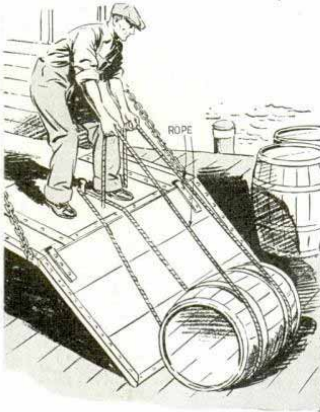
You can roll a heavy barrel into a truck with ease by using a parbuckle
