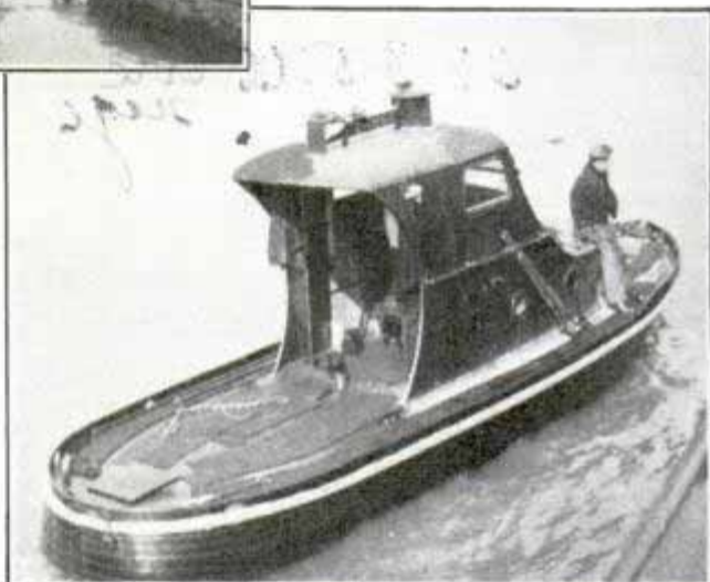
One of the midget Diesel-powered tugs which are beginning to appear on inland waters. The craft is of welded steel construction
