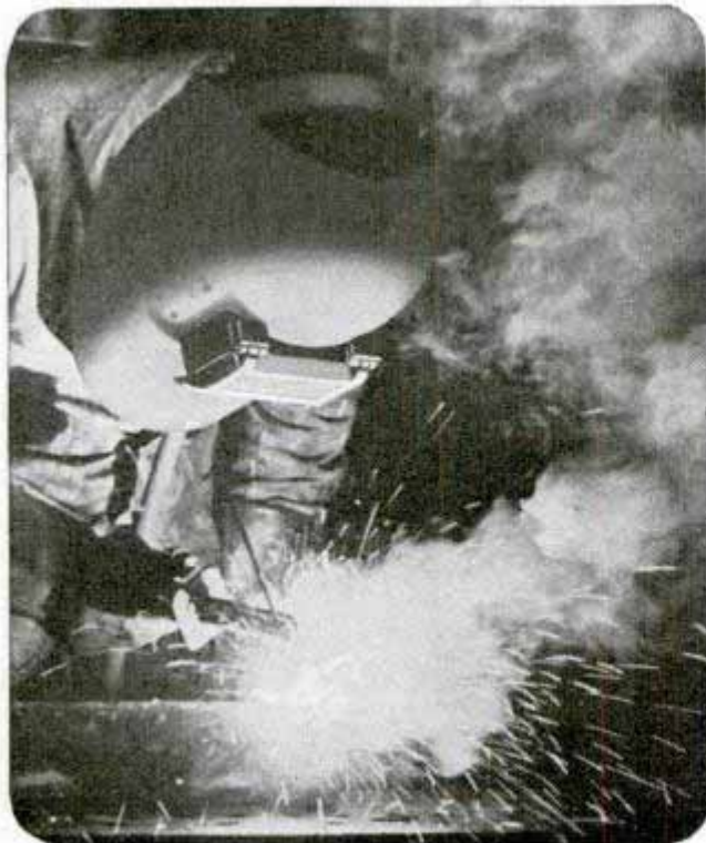
Welder on the job, protected by the one-piece helmet that fits closely about head
