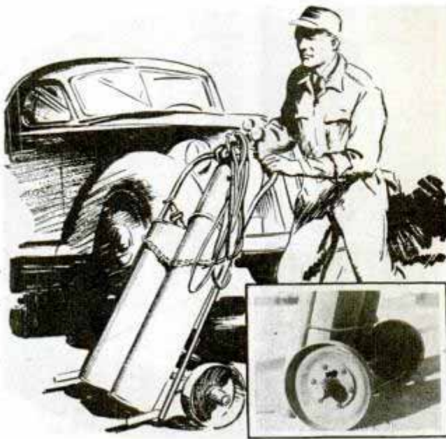
This welding-tank cart is an easy job for a mechanic, costs practically nothing and rolls easily
