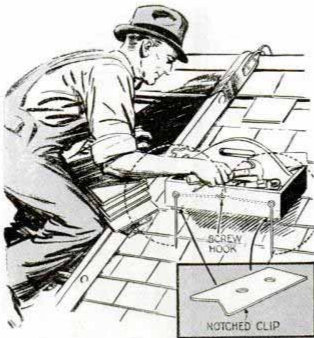
This toolbox rests level on a roof when the pointed legs are swung down
