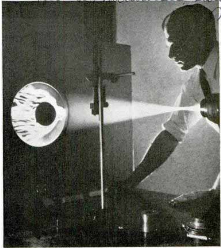
Demonstrating the way air flows around model. Engineers find this projection makes easier the study of streamlining
