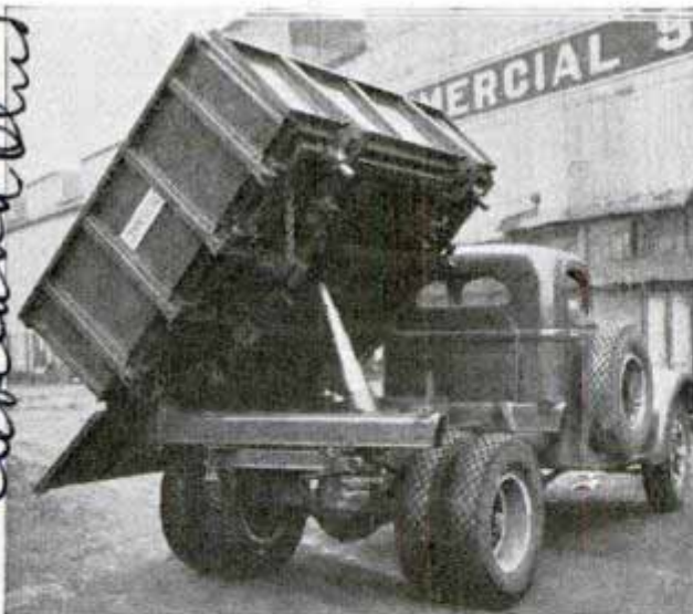
Unloading three-way dump body by tilting to left. Hydraulic hoist tilts the body
