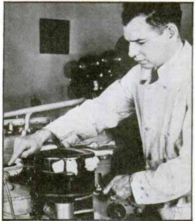
Ability of "air cleaner" to prevent flames reaching carburetor of auto is tested by inducing a backfire
