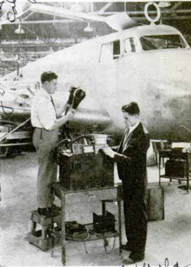
Portable X-ray equipment being used to test various metal parts of airplane
