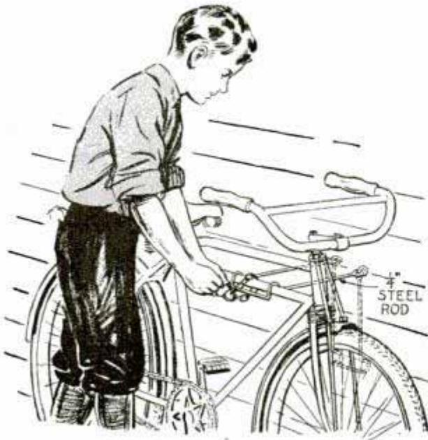
Simple holder keeps bicycle against building and permits locking to discourage theft
