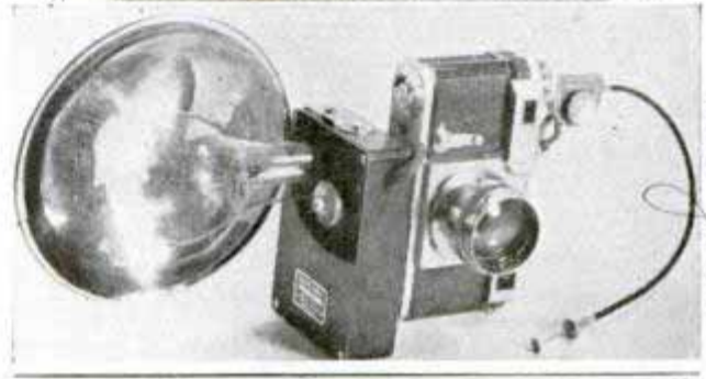
Camera with wire-filled flashlamp and synchronizer snaps action pictures like the one above
