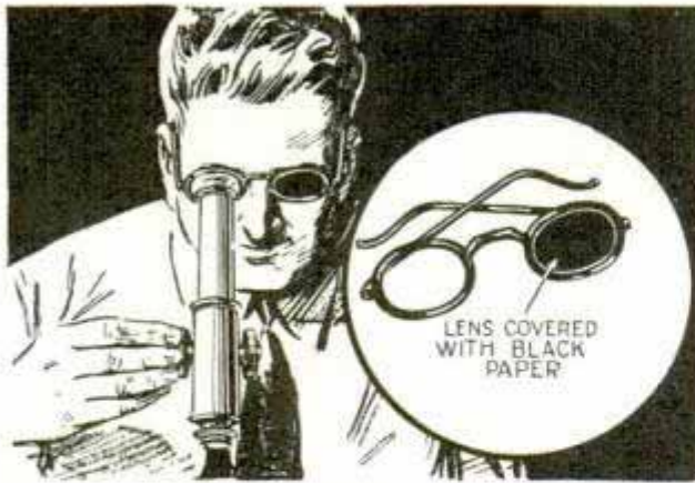
Paper disk covering one side of eyeglass frame enables user of microscope to keep both eyes open
