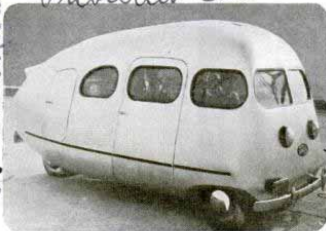
Eight-passenger teardrop car with rear engine. It has an icebox, table and studio couch for two.
