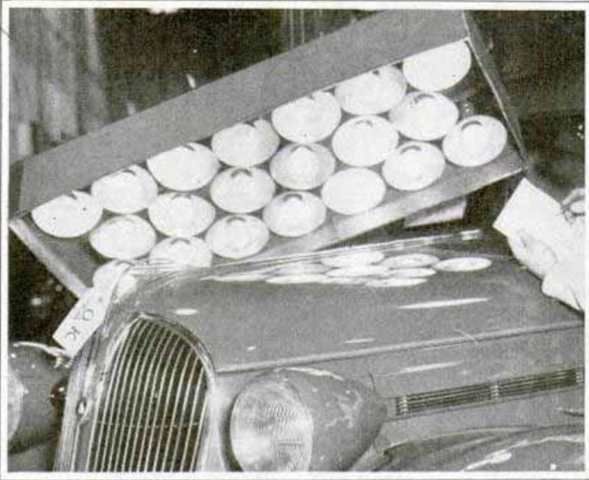
Battery of paint-baking lamps trained on hood of car in factory. This system permits accurate control of the temperature
