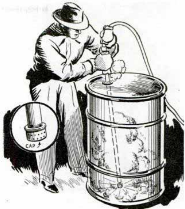
Homemade nozzle directs hot water inside of drums to clean them quickly
