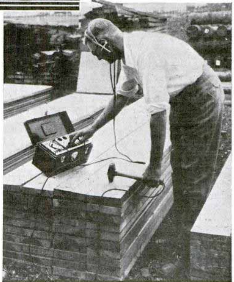
Top, removing wall panel from oven. Bottom, electrical tester determines water content of wood. If wood is air-dry it can absorb satisfactory weight of fire-resistant chemicals
