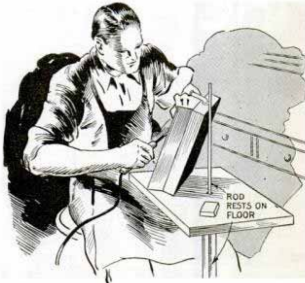
Work supported at angle against rod projecting from welder's table is easy to get at
