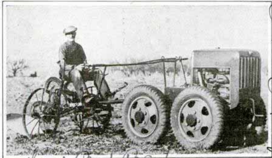
It's just like driving a horse to handle this tractor. The farmer steers and controls it by manipulating the reins leading to a control box
