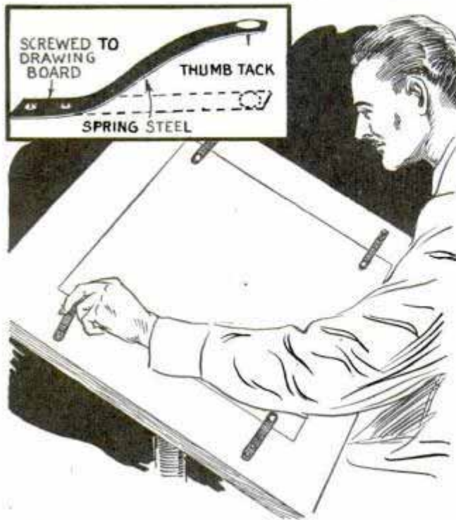
Thumbtacks on spring arm attach or release drawing paper from board quickly
