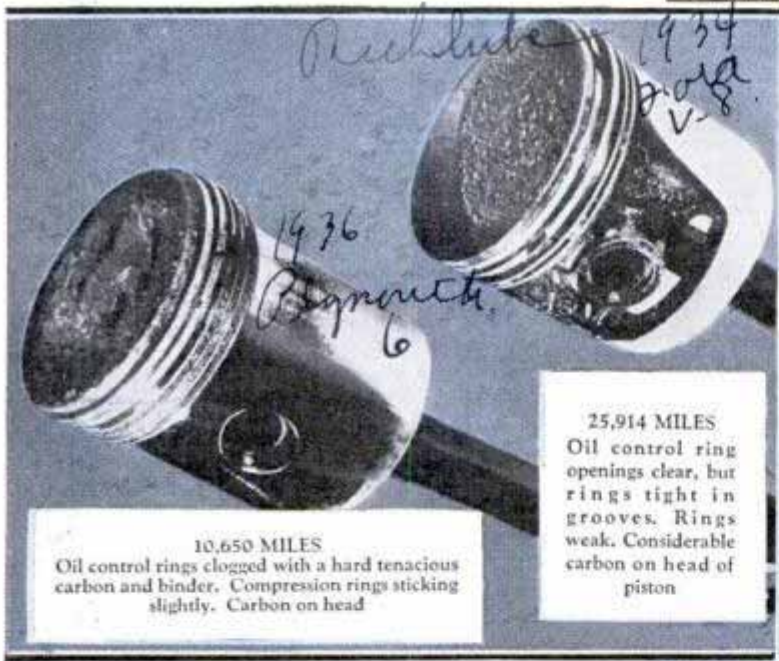
Top, burning an oil to test its flash and fire points. Left, two pistons, one after 10,650 miles operation and the other after 25,914 miles. Below, same two pistons after 1,000 miles running with oilier oil. Note how rings are cleaning up and carbon softening
