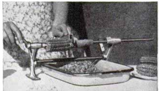
Turning the crank while knife is held on ear strips corn off the cob
