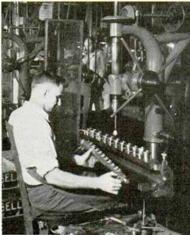
Drawing tone hole sockets, an exclusive process which makes them part of the saxophone
