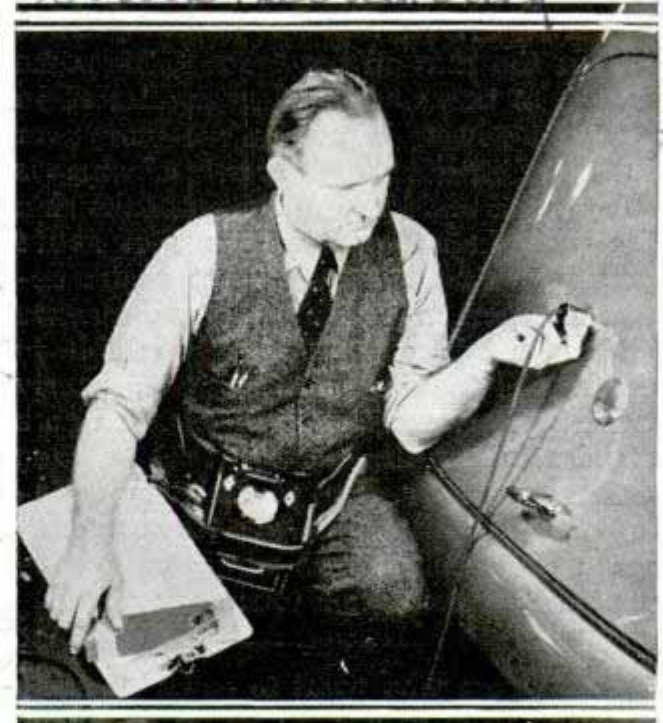
Inspector tests thickness of auto paint at factory with electrical gauge
