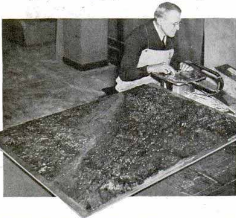
Building up a relief map with layers of plywood, cut out by jigsaw along lines traced from government contour map
