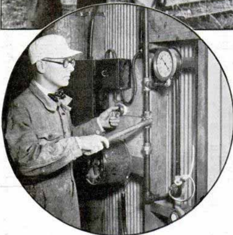
Top, experimental dust explosion shows how vents prevent destruction by permitting force of blast to escape. Bottom, ready to set off explosion in experimental building
