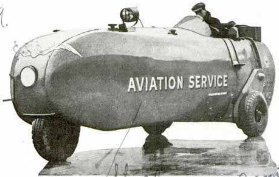
Shell Aemie Gasoline truck built for maneuvering among planes at airport. It can refuel two ships at once, and is easily steered with single front wheel
