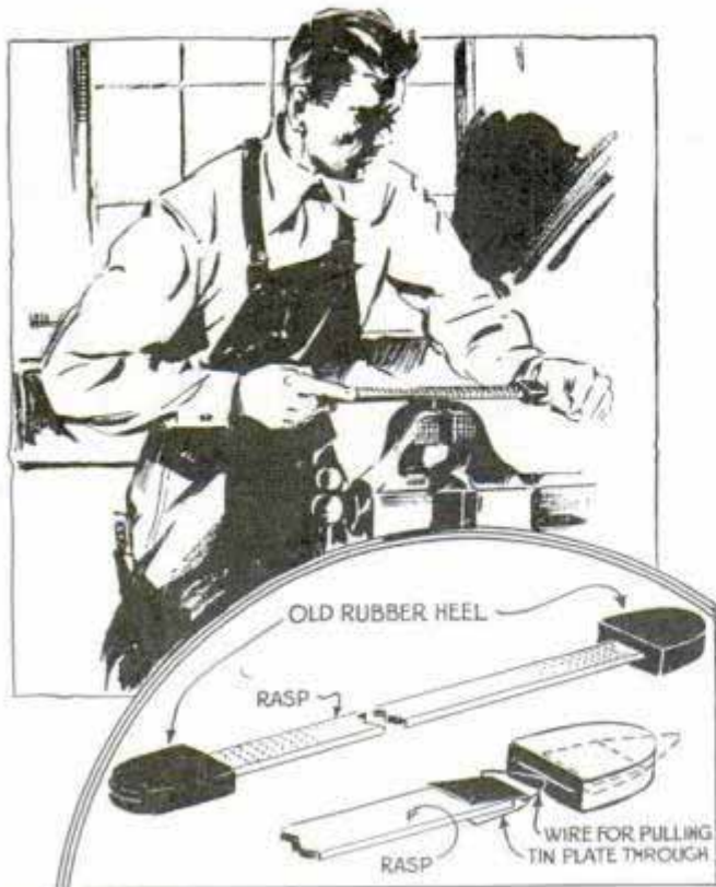
These rubber hand grips are resilient and will last the life of the wood rasp
