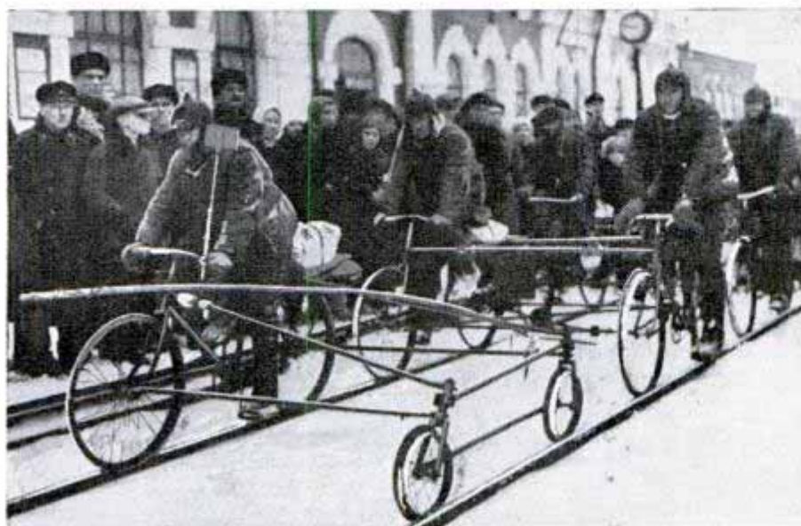
Russian bicyclists at conclusion of long tour, part of which was by rail with flanged rims and "outrigger" wheels fitted on track
