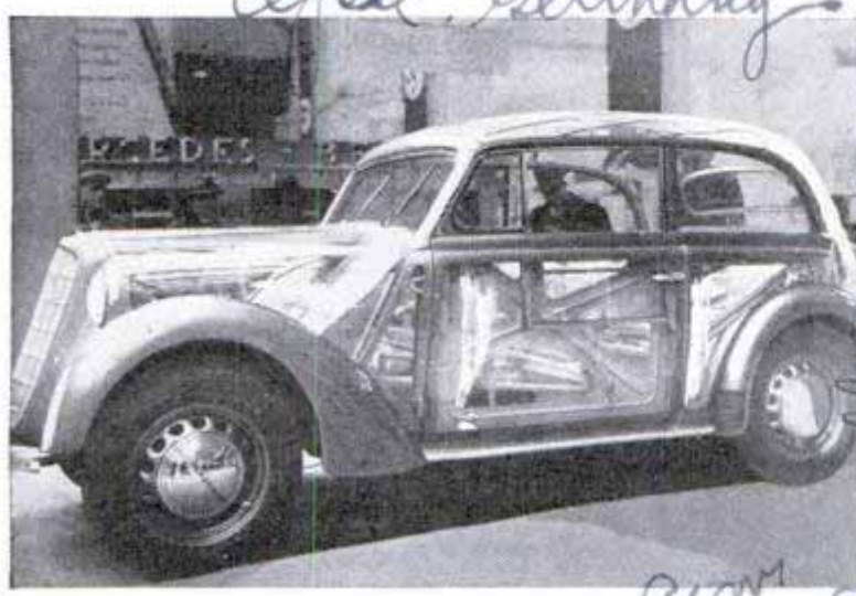
Apel Germany Prospective automobile buyers look through glass body of this car and see its sturdy steel frame
