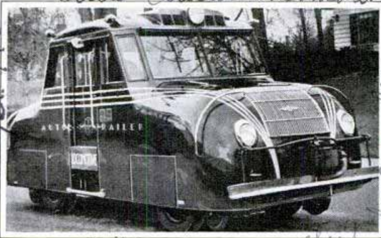
Rail-or-road switch engine which closely resembles automobile. Note retracted wheels which permit operation on rails
