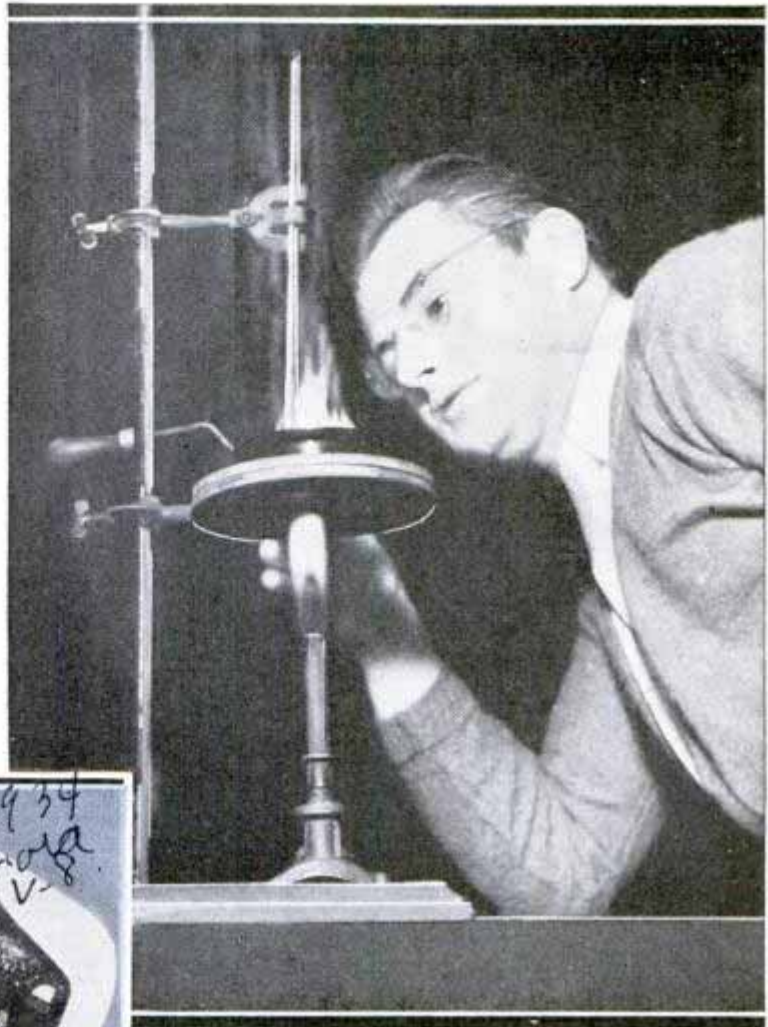
Top, burning an oil to test its flash and fire points. Left, two pistons, one after 10,650 miles operation and the other after 25,914 miles. Below, same two pistons after 1,000 miles running with oilier oil. Note how rings are cleaning up and carbon softening
