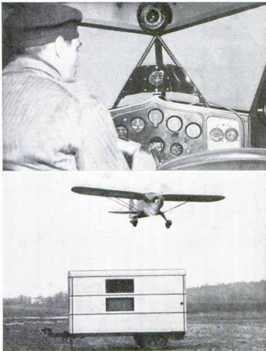
© Harris & Ewing Top, signals transmitted from trailer to plane guide pilot. Bottom, plane in air about to pass over the radio-signaling trailer
