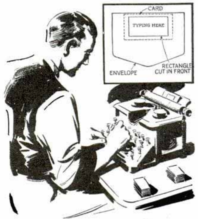
Cards inserted into a window envelope are easily fed into a typewriter
