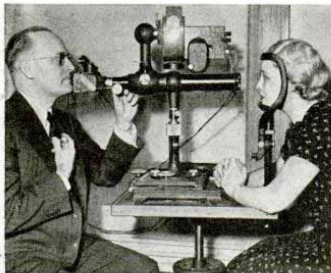
Photo courtesy Detroit Free Press Photographing the eye to show veins by which individual may be identified
