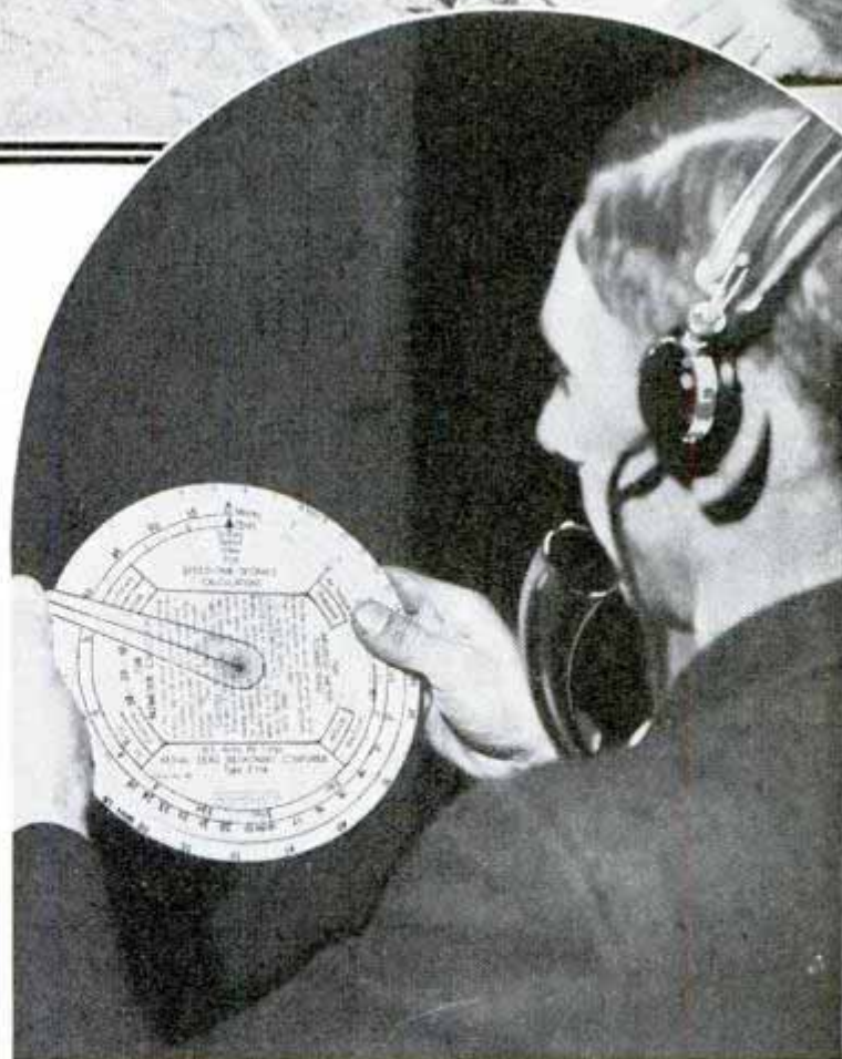
Adjusting compass span according to plane's speed. Position of ship is plotted on map every quarter hour. Land speed is computed with circular slide rule, shown below
