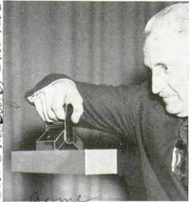
Block of metal twenty times its own weight is not too much for this small but powerful magnet to lift
