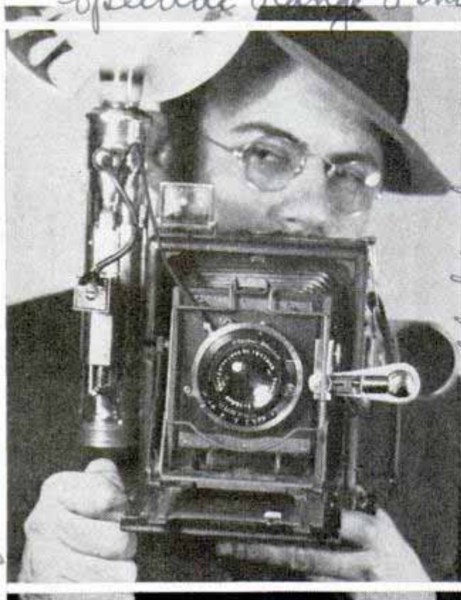
Before shooting flashlight, photographer throws light beam with electric range finder to aid focusing
