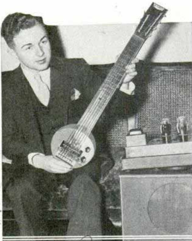
Here is the radio guitar. Note tubes which amplify tones from the strings
