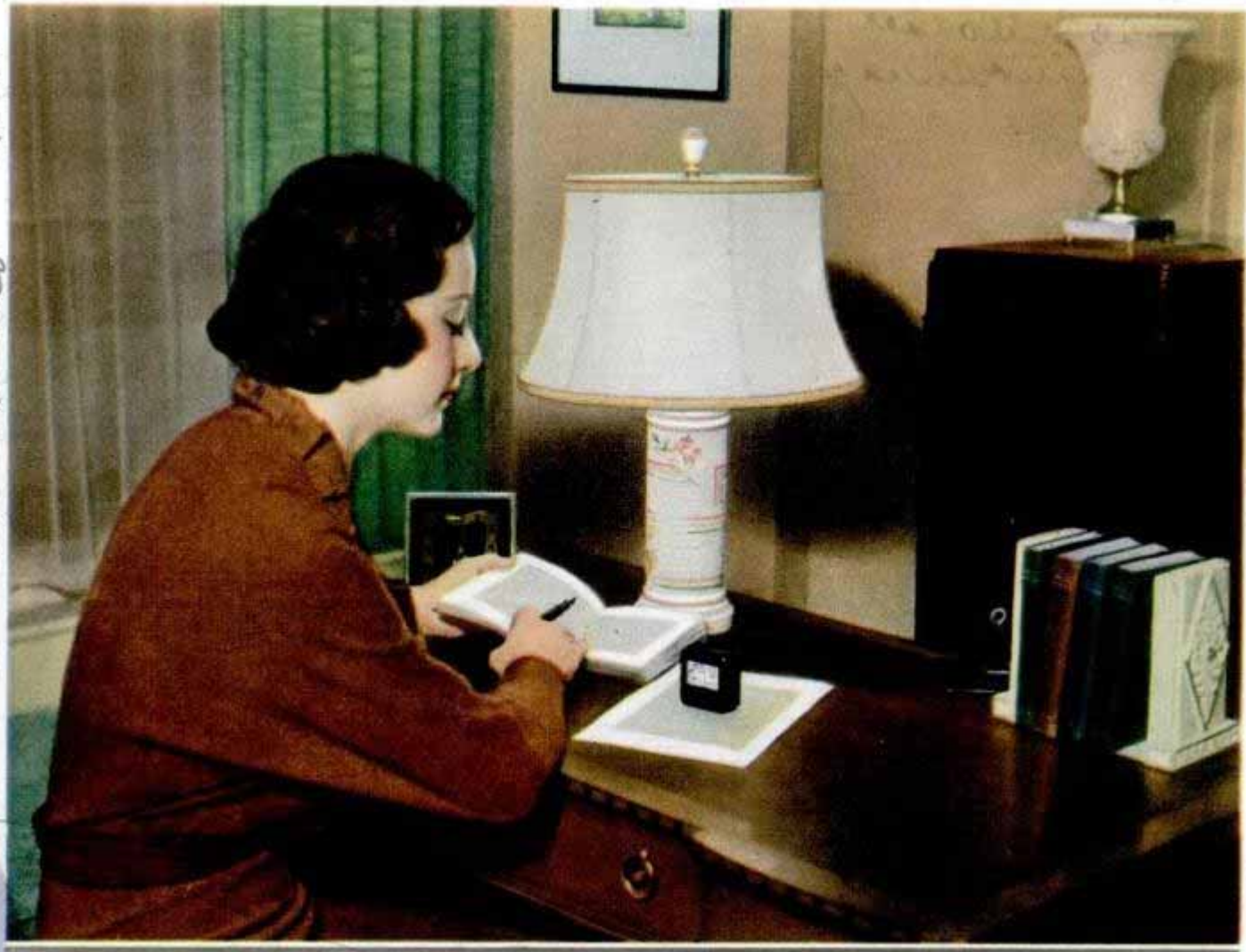
USING light meter to check intensity of illumination for reading. Below, all-purpose floor lamp with three candle sockets and large bulb with three light intensities.
