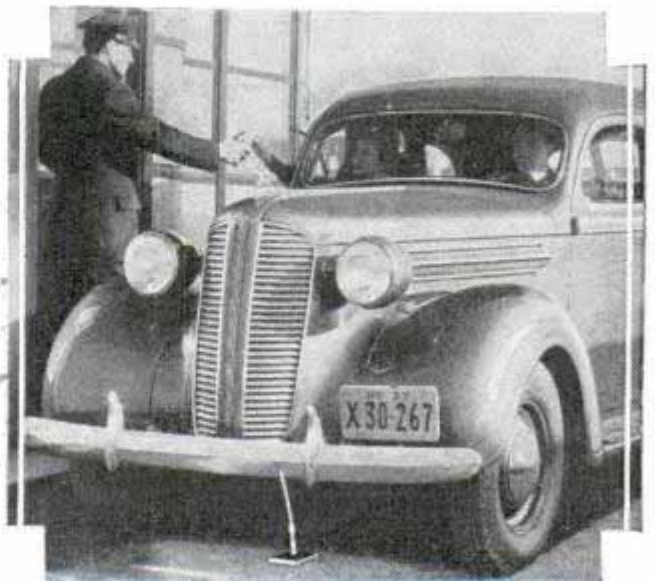
Small rod shown touching bumper of car releases static charge and prevents shock
