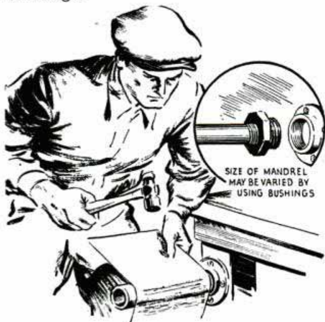
Pipe nipple on bench leg provides mandrel which can be removed when not in use
