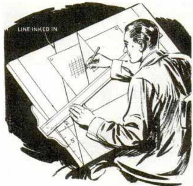
Using a T-square and a regular triangle to draw the guide lines for letter work
