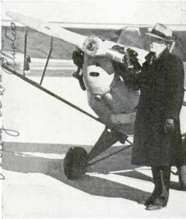
It looks like half a propeller, but this single blade outdoes performance of conventional type
