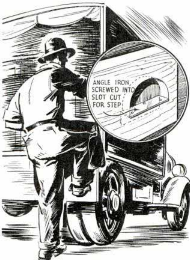
This step is never in the way and is always right where you want it when the tailboard is lowered
