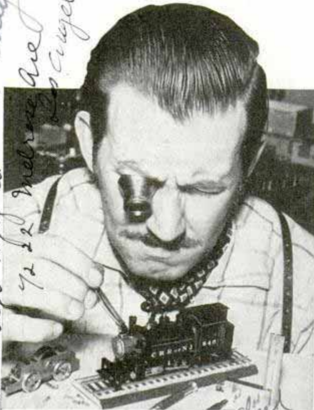
Its parts turned on a jeweler's lathe, this four-inch locomotive is run by a six-volt electric motor
