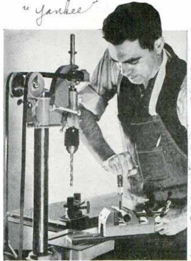
Vise removed from base may be used, as illustrated, to hold work under drill press
