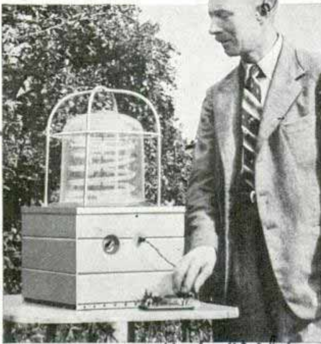
New neon lamp may be used to flash messages automatically at landing field
