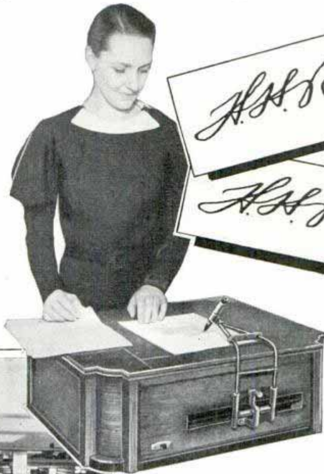
Above, reproducing pen writes a letter previously written by hand into recorder. Notice exact similarity of actual signature and robot pen's copy. Left, cabinet removed to show reciprocating plates which guide movement of penholder arm
