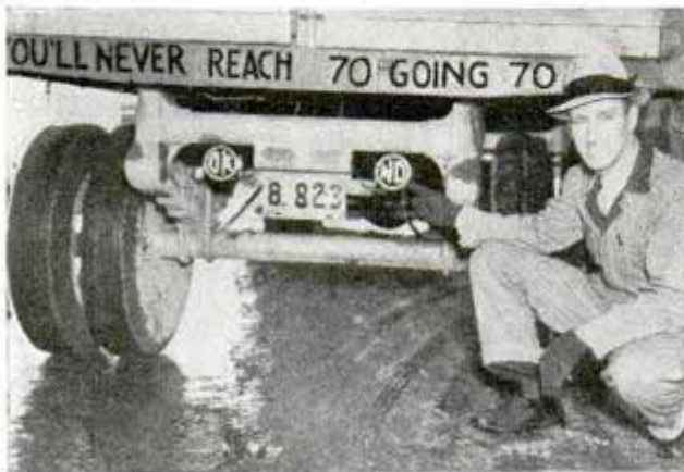
Driver points to signals which he controls from dash when car seeks to pass
