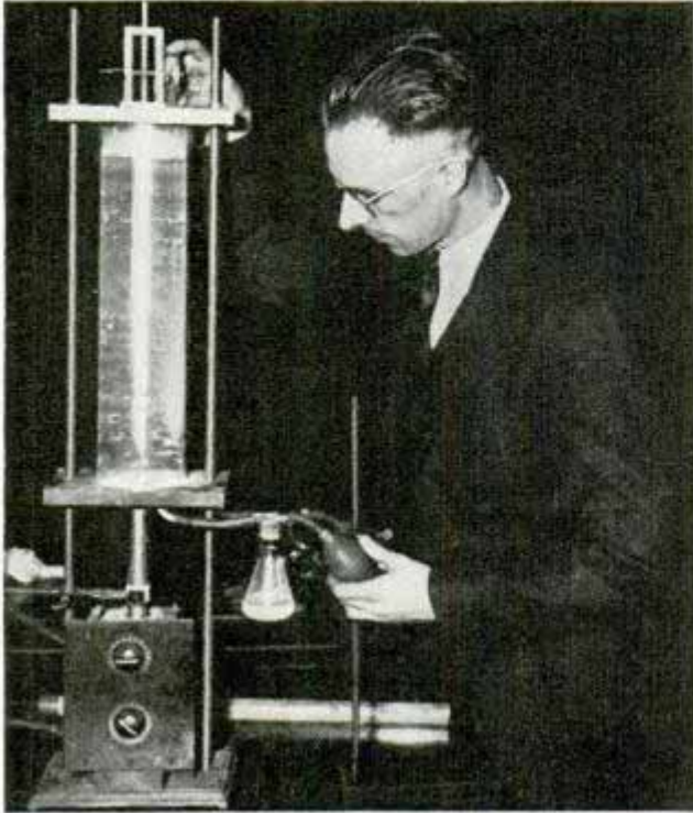
Smoke precipitates in flakes and settles to bottom of test jar after high-pitched vibration is set up
