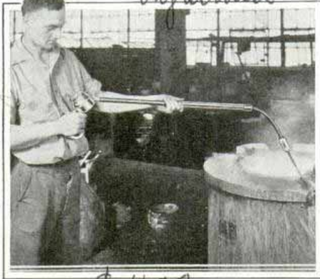
Taking the temperature of molten metal by means of thermo-electric pyrometer with flexible arm
