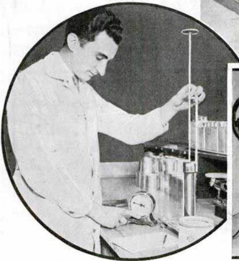
Top, W. R. Fuller of Pratt Lambert laboratories using machine to test strength and elasticity of paint. Bottom, left, testing consistency of paint. Right, immersion machine tests seaplane hull metals
