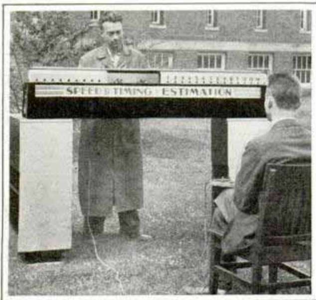
Speed and timing estimation test which shows whether you can judge clearance in passing
