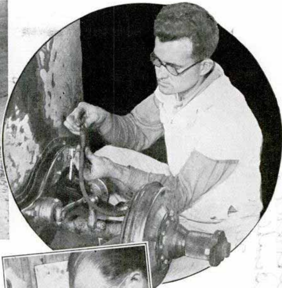
Above, testing hydraulic connection to brakes of race car. Left, fifty-dollar connecting rod used in racing engine. Below, fitting part of body to a race car chassis
