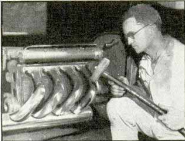
Polishing racer's exhaust pipes which provide whirling motion to gases and reduce pressure
