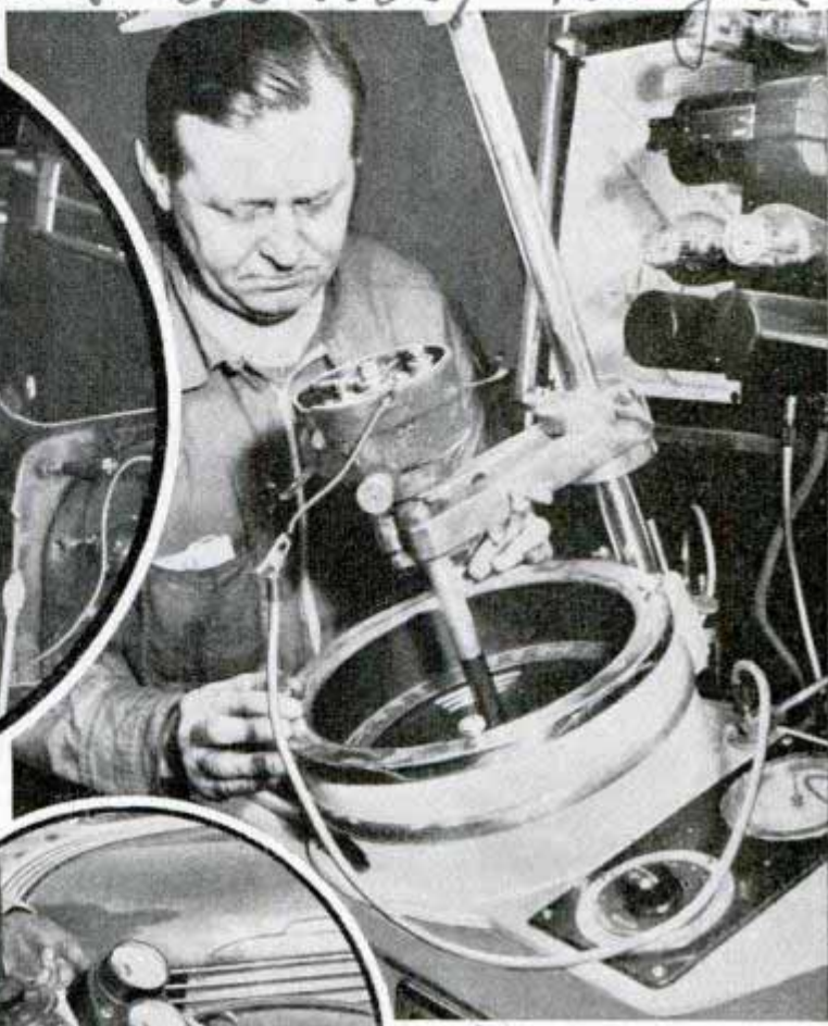
Above, oscillograph in use for testing and adjusting distributor. Left, headlamp tester which works in daylight. It records intensity of light, shows condition of car battery and reveals dirty reflectors, weak bulbs, poor contacts and other things as the causes of weak, uneven lights. The two knobs shown on the device are compensating controls
