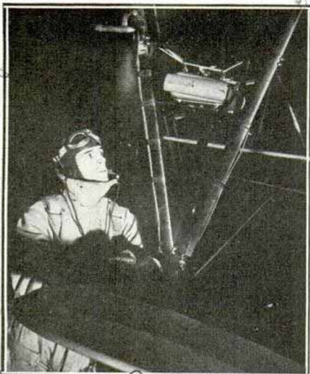
Pilot checks up fastenings of weather instruments before taking off at midnight
