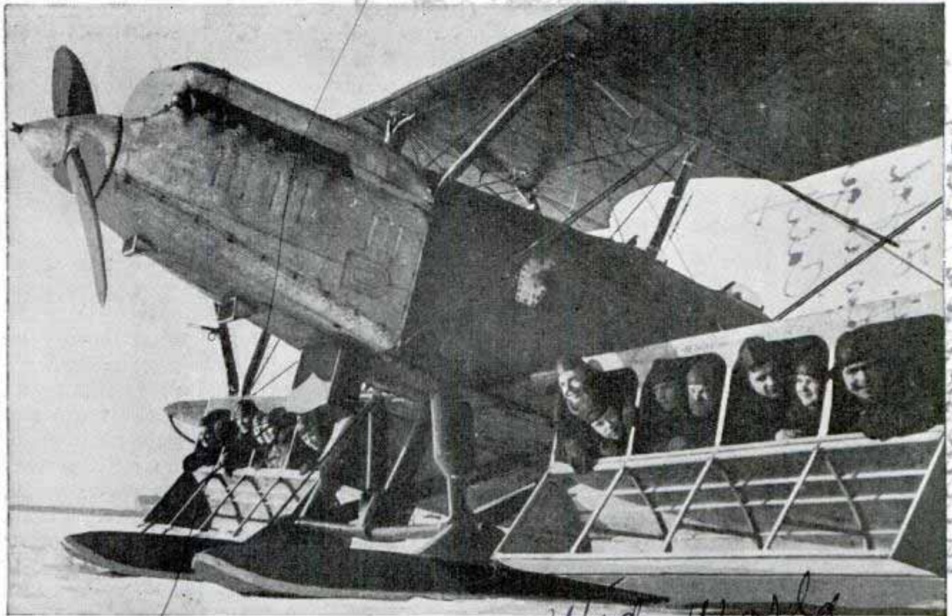
Here is how the latest two-seater plane built in Russia carries fourteen soldiers in the wings. Before taking off the hinged leading edge of the wing is closed, concealing the extra troops
