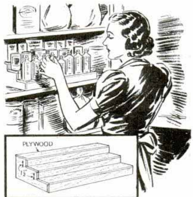
You can pick any spice at a glance if you keep the boxes on this stepped support
