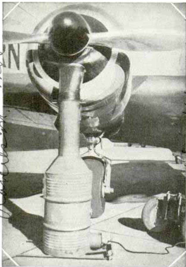
Simple heater being used to warm compartment surrounding engine of big plane
