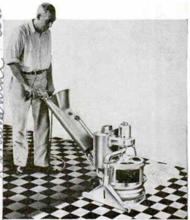
Vacuum scrubber which cleans the floor and picks up the dirty lather in one operation
