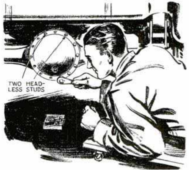
Two headless studs driven into the axle housing serve as guides when installing differential plate
