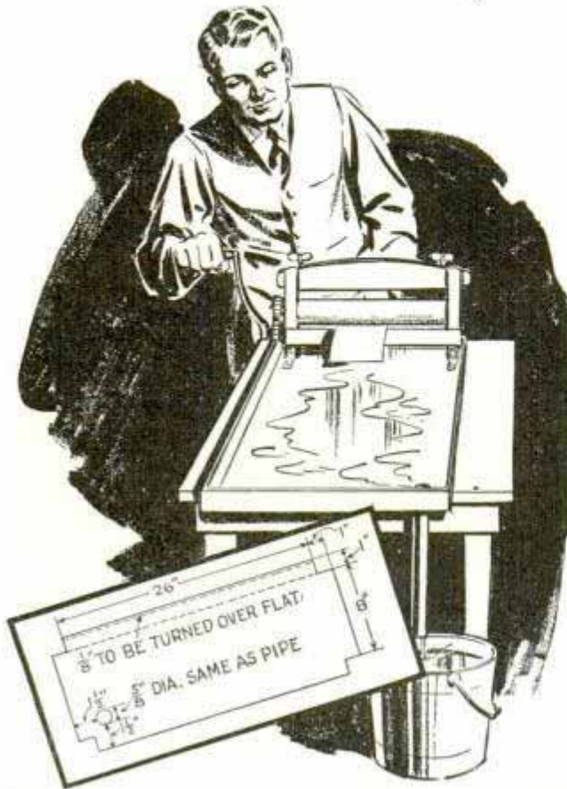
This tray carries water squeegeed from photo prints to a bucket or to the sewer
