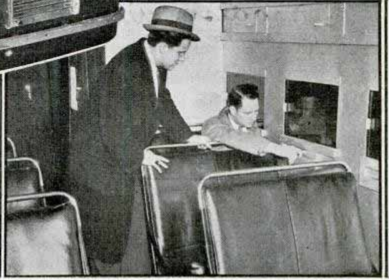
Milwaukee police are ready for action against bandits or rioters in impregnable steel-and-aluminum fortress on wheels with windows one and three-sixteenths inch thick. A machine gun took more than an hour to pierce glass. Steel shields drop to ground to protect tires in battle. Top picture shows engine mounted inside, as are siren, gong and spotlight. Left, and below at right, notice slots above windows for throwing bombs, and gun slots under windows. Bottom, left, officers emerge from car carrying full-length metal shields
