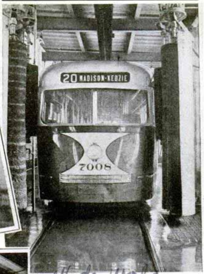
Top, street car is first sprayed, then passes between two pairs of revolving brushes which scrub it thoroughly. Second pair, at window height, rotates in opposite direction. Below, a bus takes a shower
