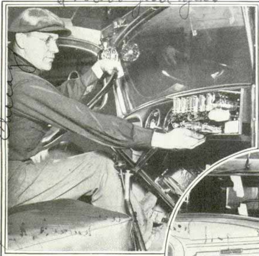
Left, truck driver pressing secret combination of six hidden electric buttons before starting motor. Steel case has been removed to show the heart of the alarm system. Center picture shows driver turning key of timing device before entering cab. Below, siren mounted under truck
