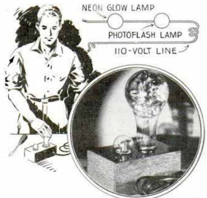
Neon lamp glows if bulb is good and passes insufficient current to flash it
