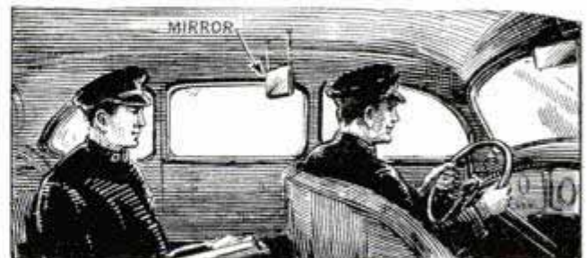
Extra mirror in squad car enables officer in rear seat to see behind car without turning his head
