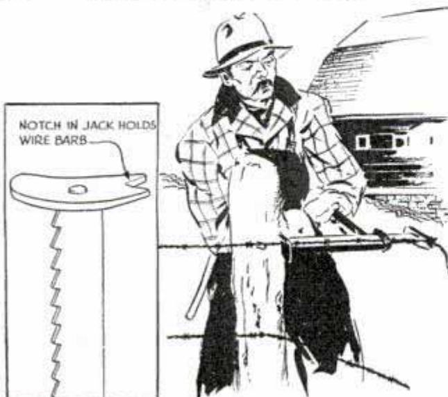
An auto jack will quickly stretch short lengths of barbed wire when repairing a fence
