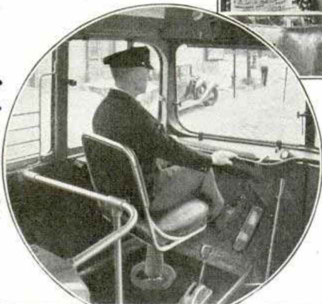
Three views of 1937 street car. Notice similarity of controls to those of an automobile. Magnetic brakes can be seen between wheels in bottom picture
