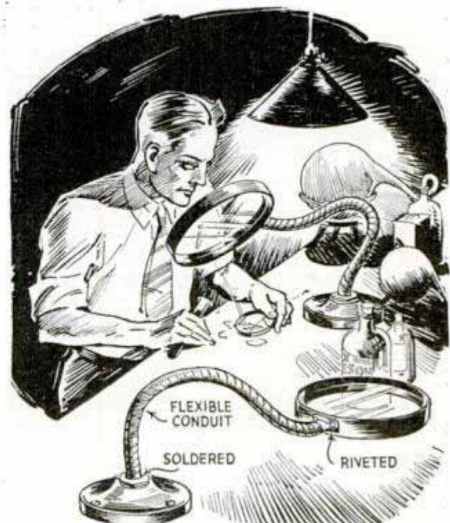
Quickly swung into position, the shield is readily assembled from parts easy to obtain
