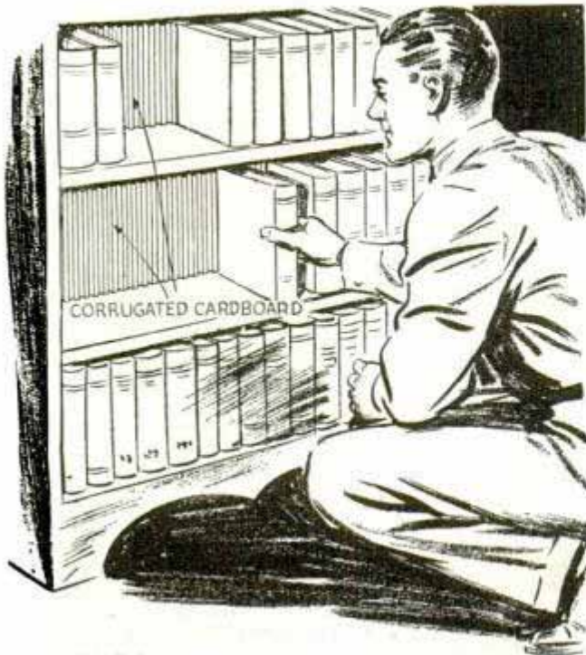
Books will not tip when one is removed if corrugated cardboard is glued to the back of the case
