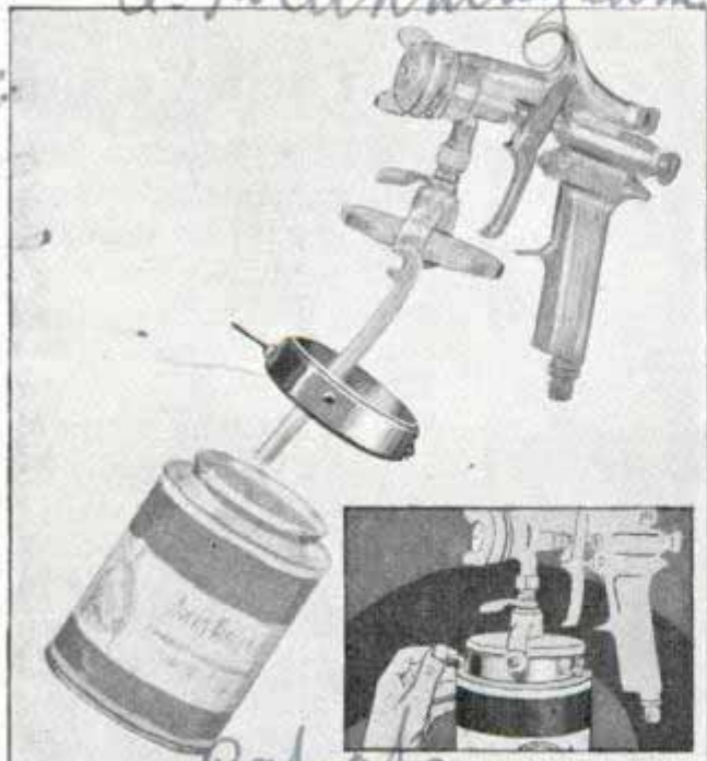
Drawings show how adapter fits rim of paint can allowing spray gun to draw directly from can
