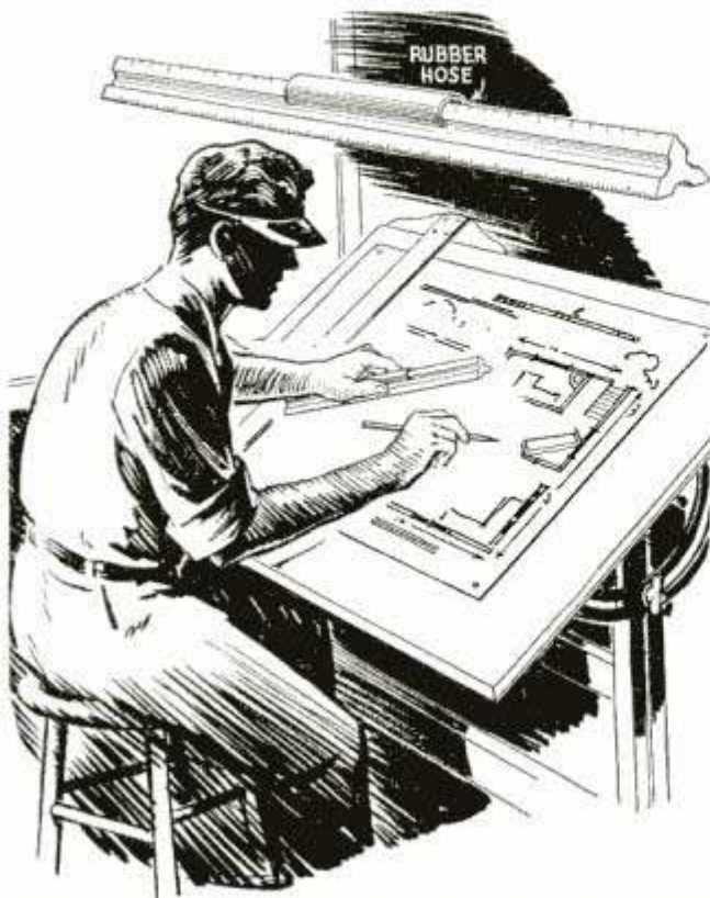
Rubber handle is quickly moved to the edge of the ruler carrying the scale being used
