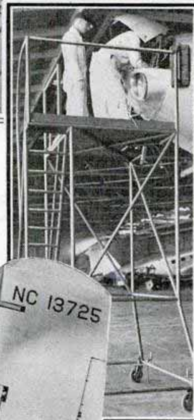
Above, stand used for work on rudder. For tail inspection a padded part rests on stabilizer. It can be placed at footing desired without interfering with tail surfaces. Below, steel frame for towing skyliner permits tractor to turn without bumping tail surfaces
