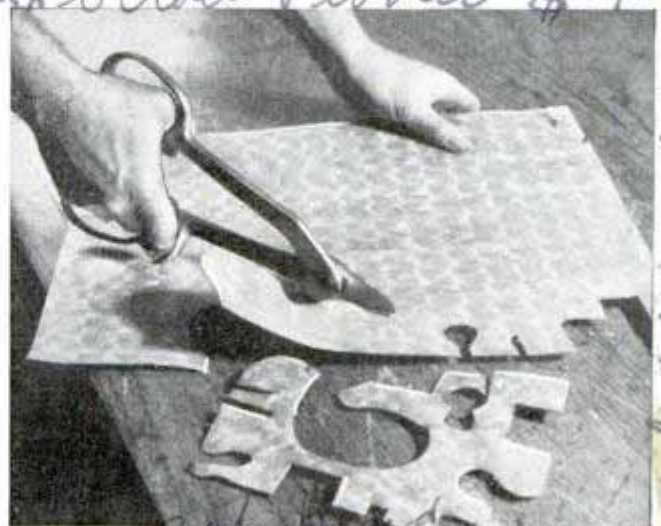
Examples of shapes cut by flat-bladed metal snip
