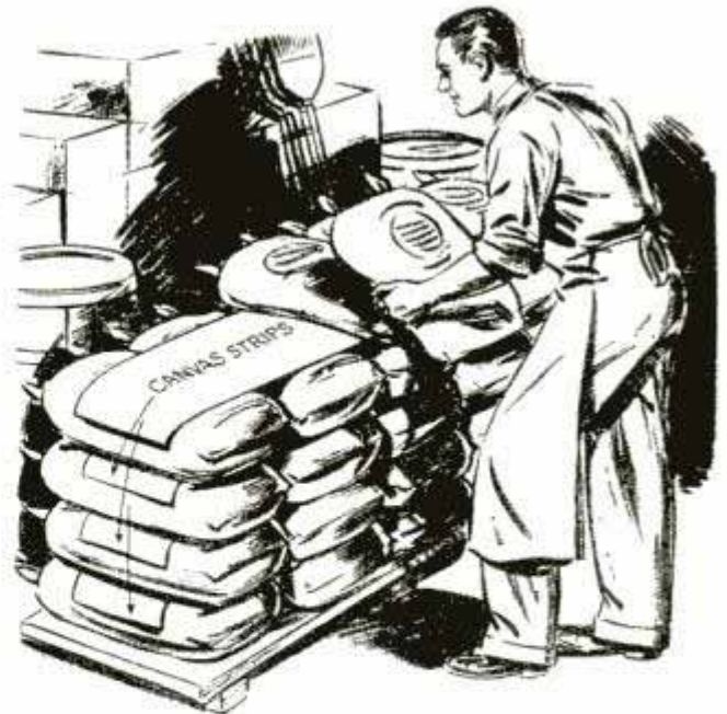
Sacked material readily stacked in high piles, without risk of falling, with aid of canvas strips
