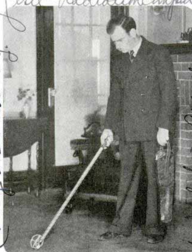
Figuring cubic space in house by running a wheeled computer along the three dimensions
