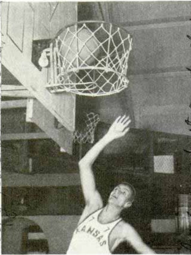
Ball trips metal loop as it falls through basket and turns on light momentarily, indicating a score
