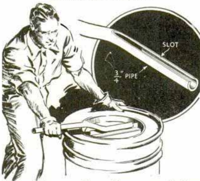
Plenty of leverage to loosen the screw top of a large can is provided with this handle
