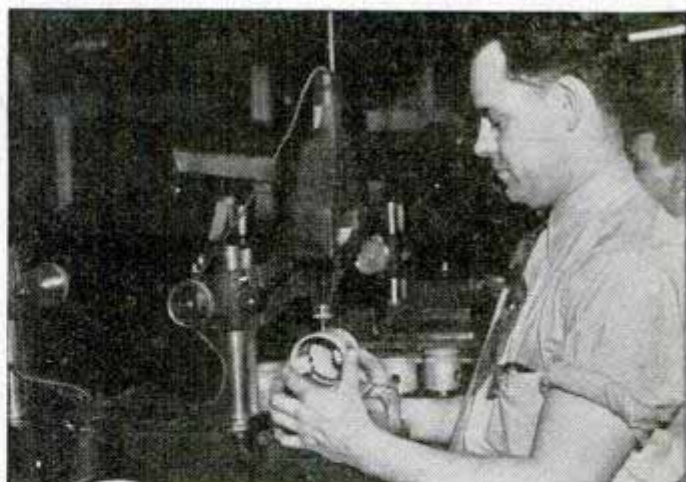
Inspecting Ford Pistons for accurate diameter and roundness on quick-reading amplifying type of gage.
