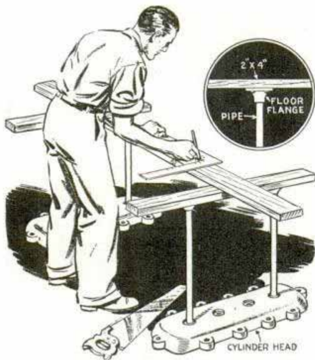
Two lengths of pipe, two floor flanges, an auto cylinder head and a plank make this sawhorse
