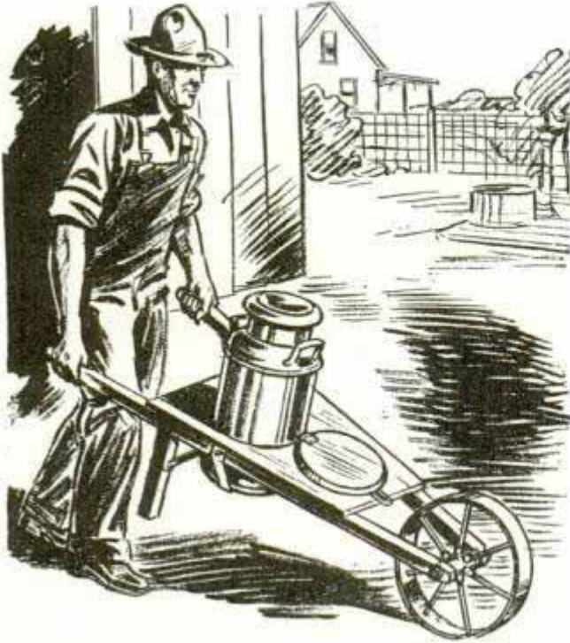
Milk can rests in hole of wheelbarrow floor to lower center of gravity of the load
