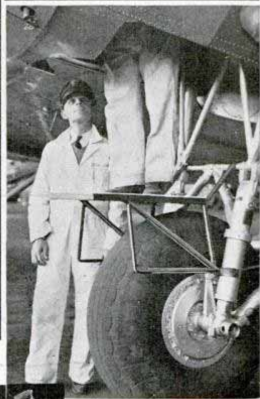
Center, working on nose of air liner is made easier by stand providing eighteen square feet of space. Right, platform which fits landing-gear structure provides footing for mechanic to do work inside nacelle
