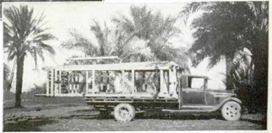
Truck carrying tower for inspecting date palms for scale and, above, the tower extended and two inspectors at work
