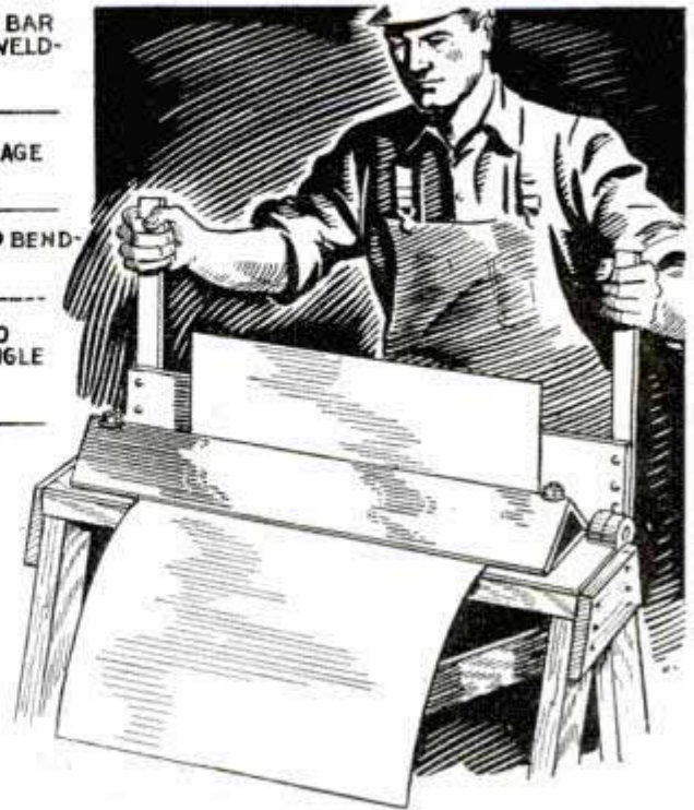
This bending brake will make clean, sharp bends in No. 16-ga. sheet metal, and will take a sheet up to 30 in. in width. It's made from steel bar and angle stock
