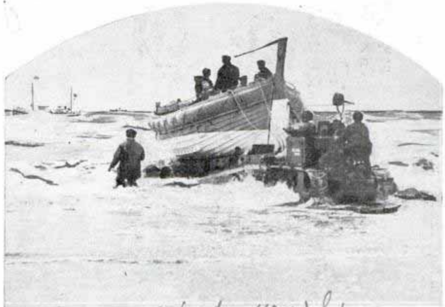
Wide World Dutch coast guardsmen starting out on a rescue mission, driving their boat into the surf on a specially constructed truck pushed by a tractor
