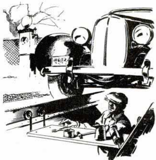
Holding tools and parts, this shelf is quickly moved to any part of a greasing pit
