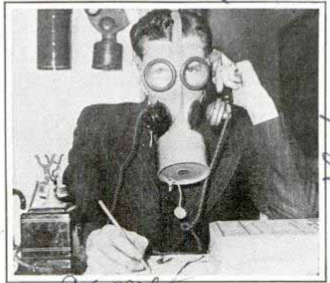
Microphone fitted inside this gas mask permits the wearer to talk over the telephone
