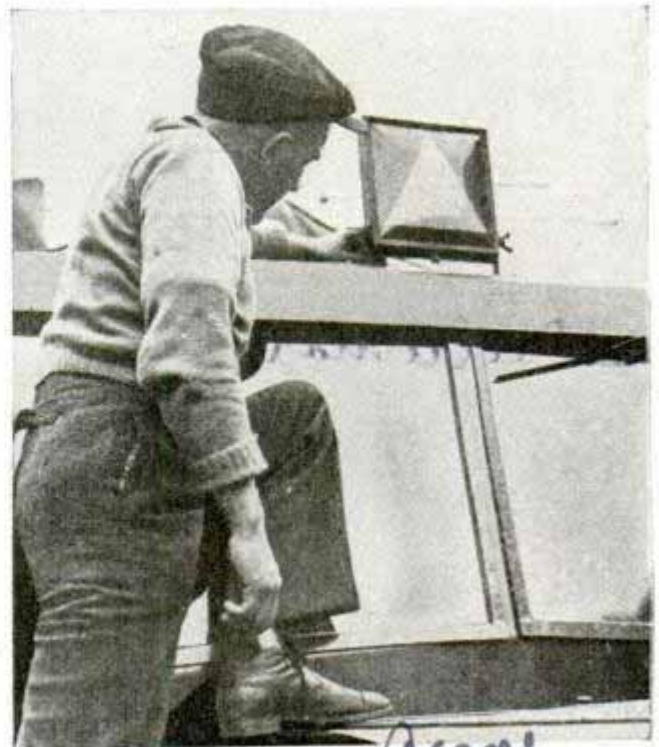
Yellow triangle set in a blue square above windshield gives night and day warning of wide truck
