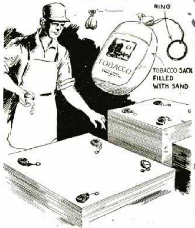
If a number of small sacks are filled with sand, they make paperweights which are easy to handle
