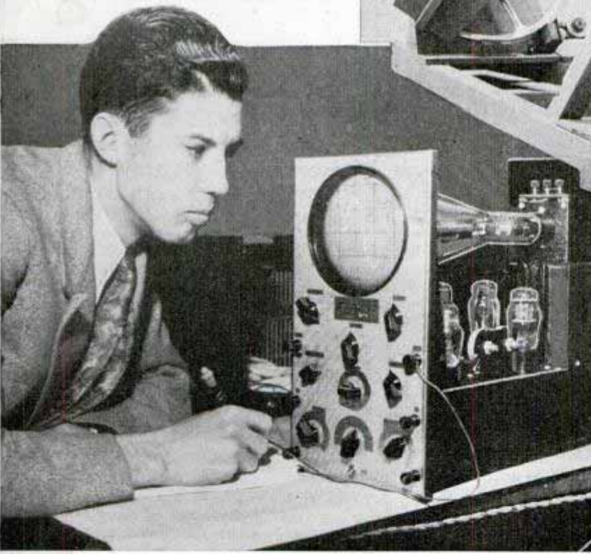
Top, cosmic-ray telescope which "rings up" incoming rays on counter. Below, using cathode-ray tube as sensitive voltmeter to measure the strength of radio signals from space in an effort to determine their source
