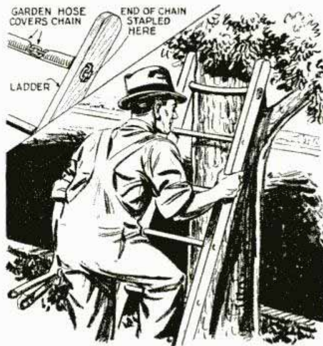
The upper rung of this ladder adjusts itself to the curvature of a tree to prevent slipping
