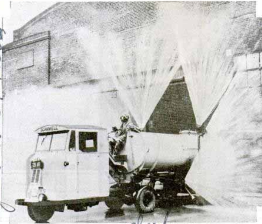
dent. Fan-shaped sprays of water shooting in all directions disinfect street, air and walls after poison-gas attack upon city in London.
