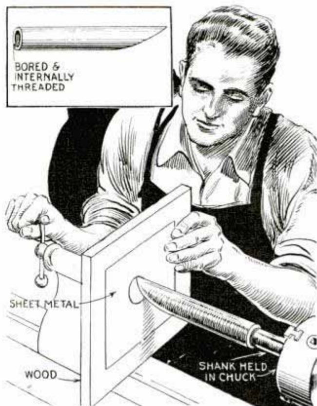
Disks and washers of light sheet metal are easily turned out in quantities with this tool
