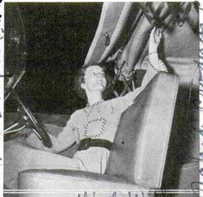
Pressing switch releases compressed air and causes this auto top to fold back out of sight
