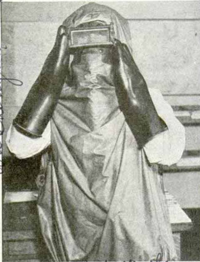
Did work Dangerous dust is excluded by this rubberized silk hood, protecting the sandblaster from silicosis
