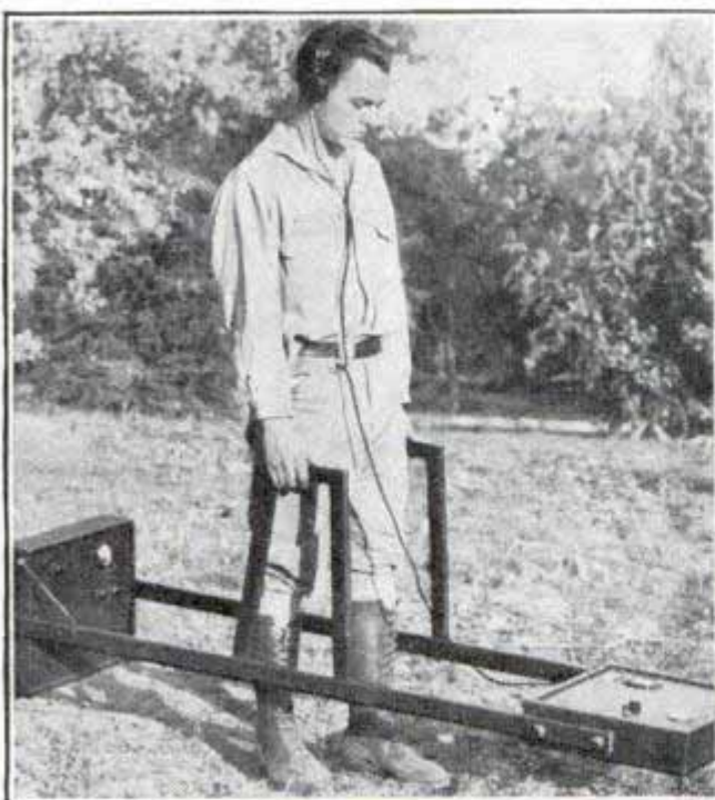
Successful inductive electrical apparatus that indicates buried metallic materials
