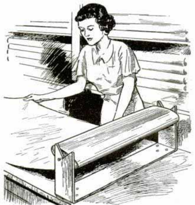
Customers quickly inspect cloth in this rack, which permits the bolt to rotate freely.
