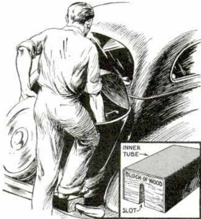
Block slotted to fit on bumper makes handy step when lifting luggage from trunk
