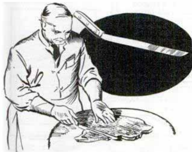
A knife with the handle bent to an angle gives full use of the entire cutting edge
