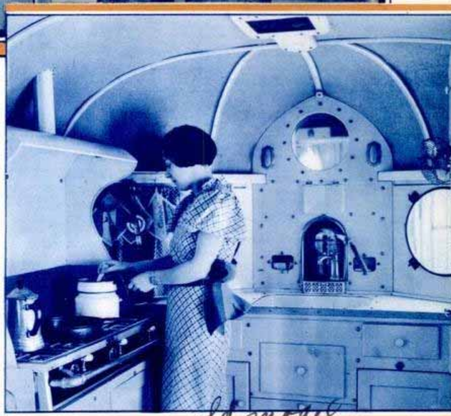
GALLEY of modern trailer, complete even to an electric fan and a stack for carrying off cooking fumes and heat from the gasoline stove. Top, trailer interior, showing the many built-in fixtures.
