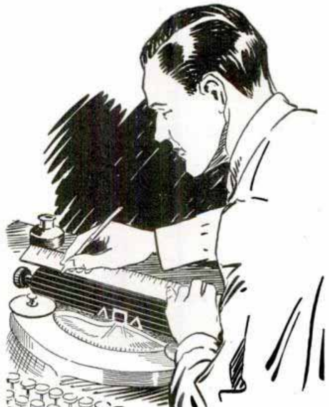
Small work is easily alined with the aid of these parallel lines
