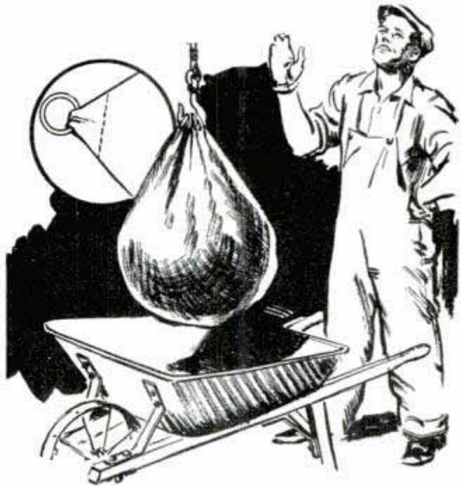
False canvas bottoms on wheelbarrows hold sand to be hoisted without delaying workmen
