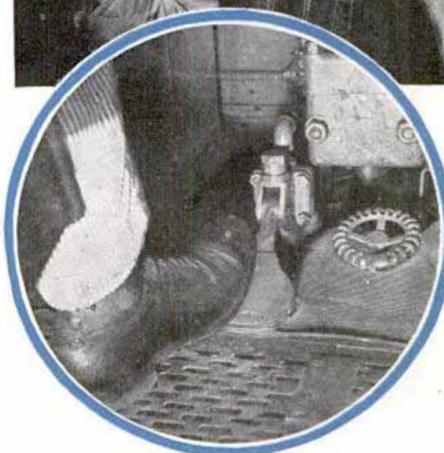
Engineer at controls of the "City of Denver." Center, engineer conversing with train crew by "telephone." Bottom, the "dead man's" throttle which stops train if pressure of foot is released
