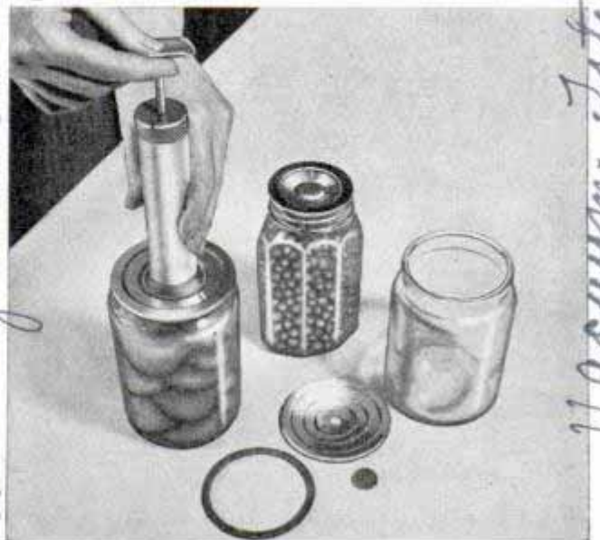
Equipment for vacuum canning, including pump, rubber band, metal top and tiny rubber seal
