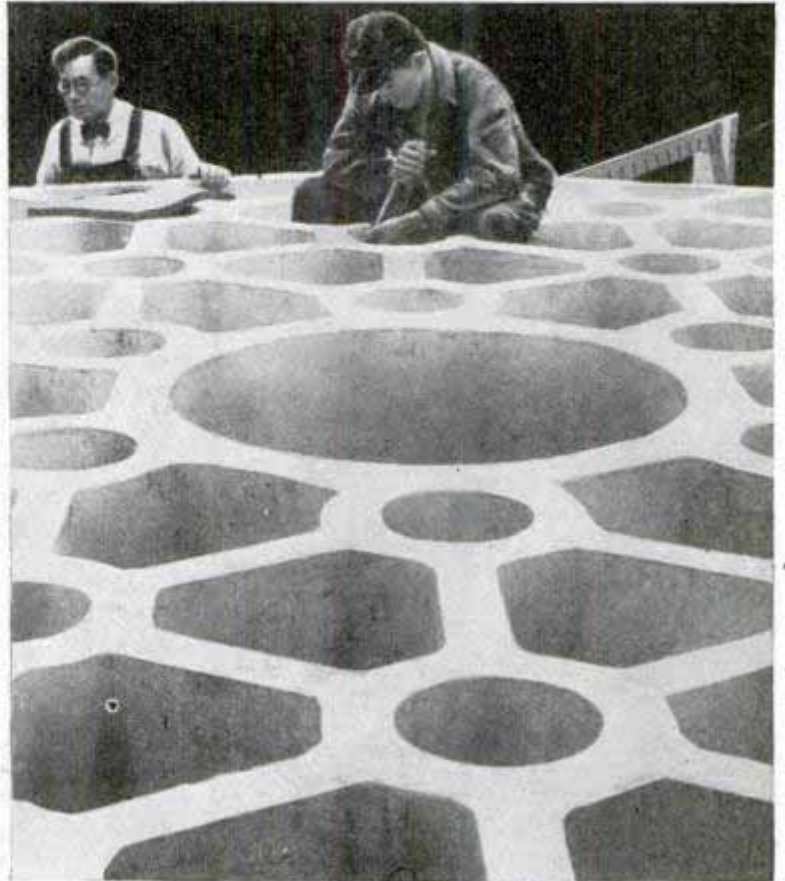
Experts at their job of cutting away the heavy ribs from the giant mirror which will be installed in observatory
