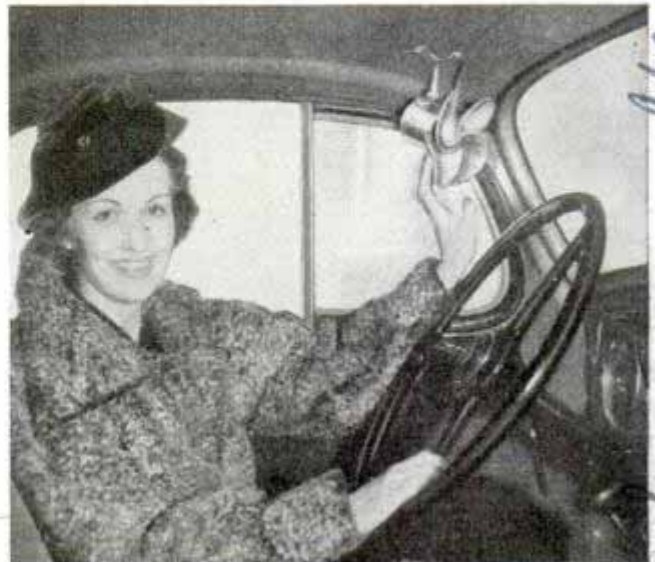
Flexible rubber blades on windshield fan cannot injure a finger, but they provide plenty of wind
