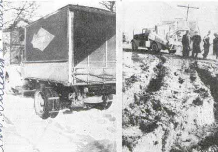
Notice the broad lugs attached by a single chain to dual tires. A truck equipped with these successfully navigated the sticky mire at right
