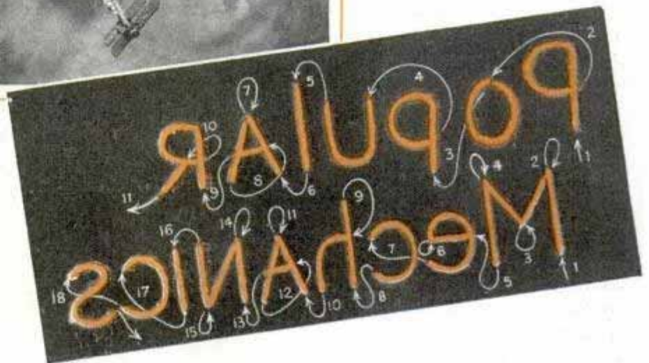
Skywriter above is stunting. His smoke is not holding well enough for lettering. The chart shows how a flyer would maneuver to write "Popular Mechanics" in block letters, which are easier to line up than script
