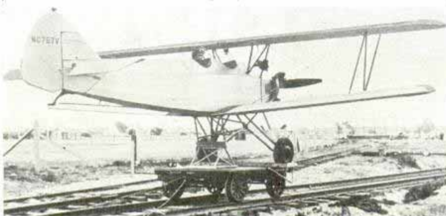
After run of 400 feet the plane takes off from the handcar. The plane's propeller drives handcar until the takeoff
