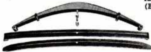
Springs for 1937 Ford V-8s are provided with an oil groove for interleaf lubrication as shown at left.
