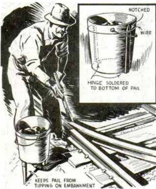
Legs keep trackwalker's grease bucket level when it must be set on inclined roadbed
