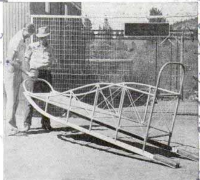
Tubing framework of latest sled. Weight has been reduced fifty per cent
