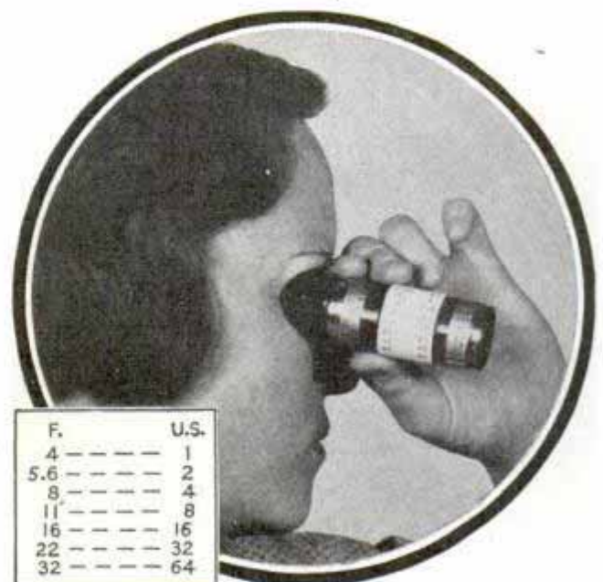
Conversion table on exposure meter serves as reminder and shows at glance setting for camera
