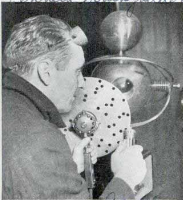
As electrician focuses light on amplifier, interruptions by perforated disk cause musical chords
