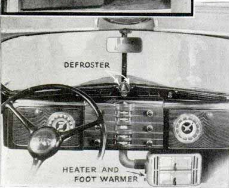
Top, fleet-appearing Chevrolet. Center, interior of Plymouth, showing chair-height seats and instrument panel with recessed controls. Bottom, heater and defroster in supercharged Graham
