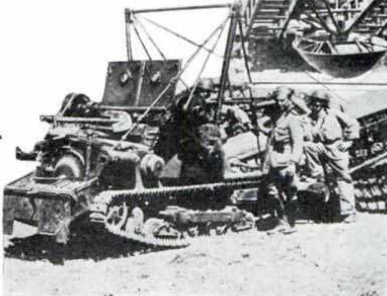
Top, bridge extended by tank to show how stream would be spanned in time of war. Bottom, view of the bridge-carrying tank as it appeared in maneuvers of Italian army
