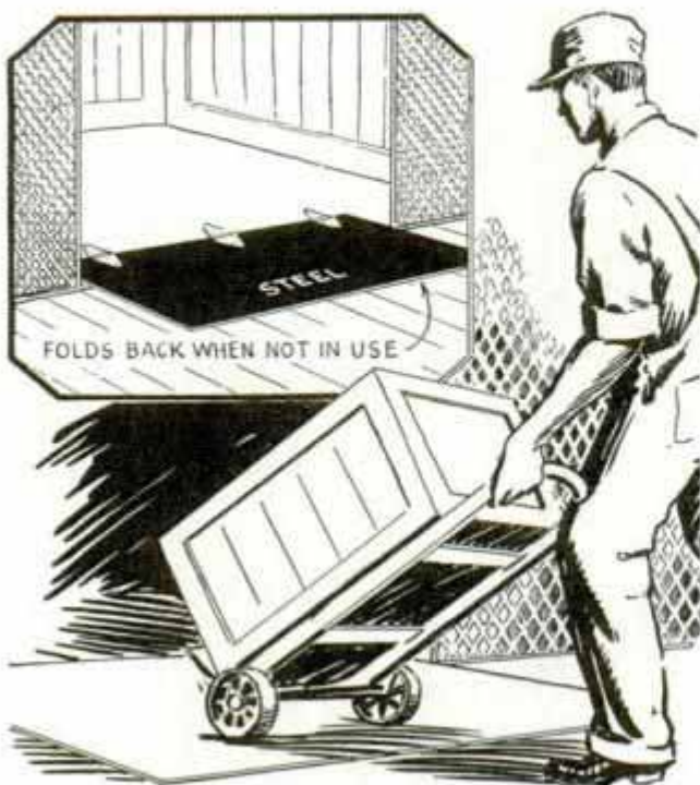
Steel plate serves as "bridge" between elevator and floor over which to push hand trucks
