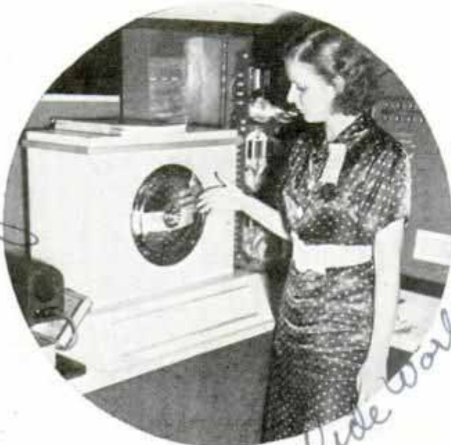
Passing hand near model of vault alarm system causes bell to ring
