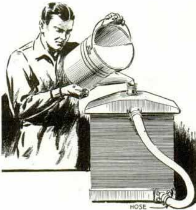
It takes only a couple of minutes to connect the radiator outlets with a hose to make a test
