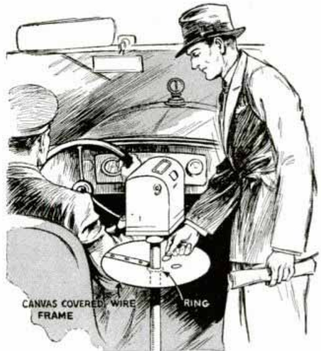
Coins dropped by passengers while paying their fare in this bus are caught in a receptacle
