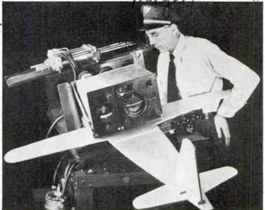
Before taking over controls of a transport plane, the automatic pilot is "taken for a ride" on a tester that simulates motions of flight
