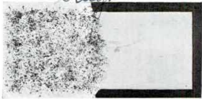
Sparks of metal pitted ordinary glass at left but did not affect specially treated glass at right
