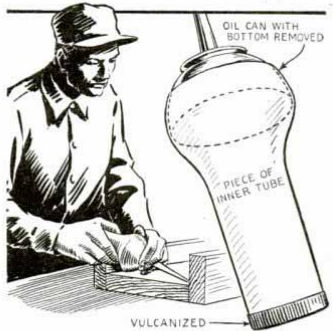
This gun will take care of glue jobs where it is difficult to use a spreader
