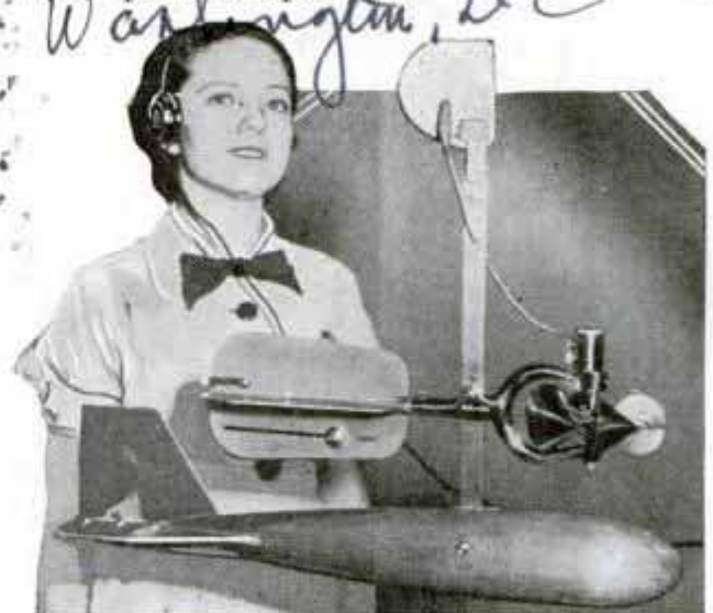
© Harris & Ewing With streamline weight to keep it pointed upstream, this bucket wheel measures velocity of current
