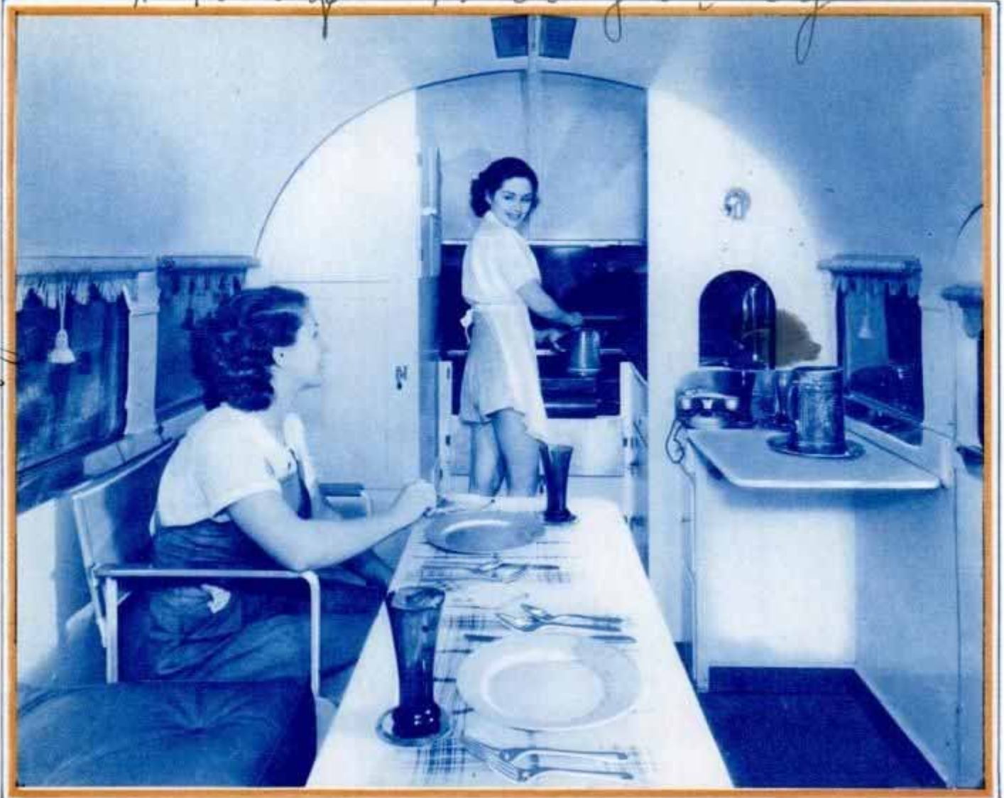
COLLAPSIBLE dining table in trailer coach. Note telephone set at right which connects through plugs to driving compartment of tow car.
