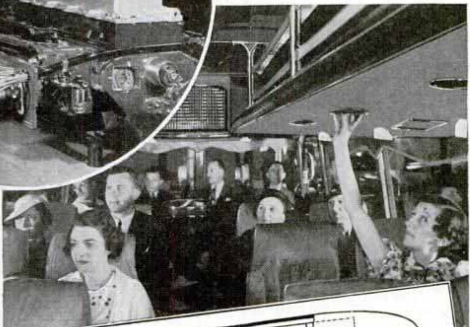
Streamline, air-conditioned motor coach built by the White Motor company and the Kelvinator company to demonstrate possibilities in bus travel is shown above. At left is 180-horsepower twelve-cylinder "pancake" engine which is mounted under the floor
