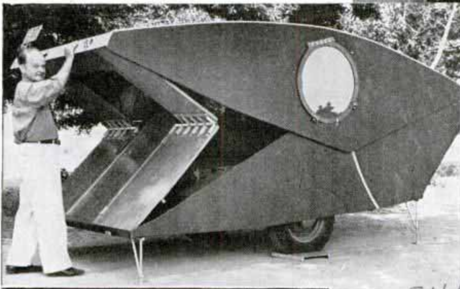
Top, ready for camp. Notice how roomy the trailer is; no need for stooping. Center, folding up for travel. Springs act as a counterbalance making it easy to raise or lower, and corner supports are adjustable to level the floor. Below, the trailer in its streamline form, its top below the automobile window
