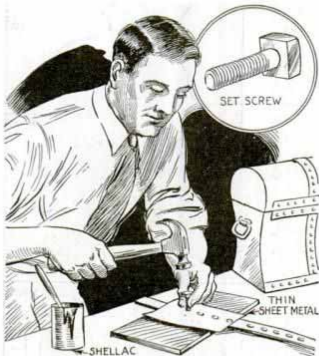
Anyone can simulate rivets on the binding strips of fiber chests with this simple method
