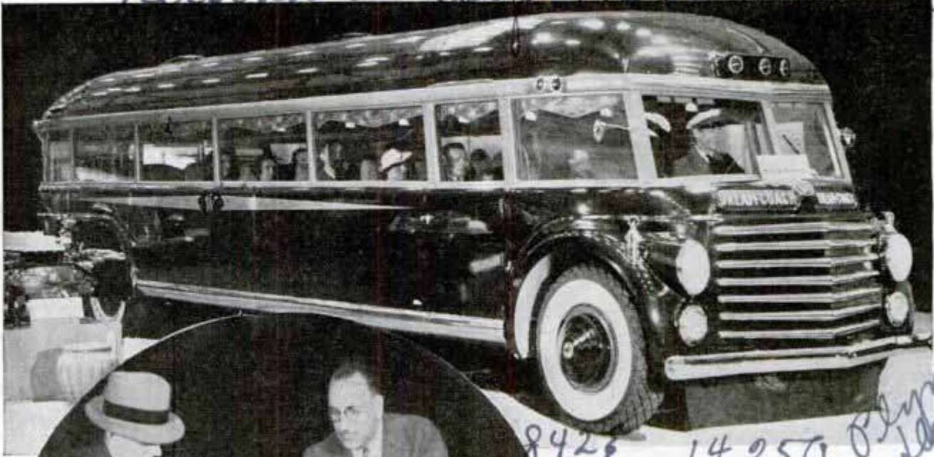
Streamline, air-conditioned motor coach built by the White Motor company and the Kelvinator company to demonstrate possibilities in bus travel is shown above. At left is 180-horsepower twelve-cylinder "pancake" engine which is mounted under the floor
