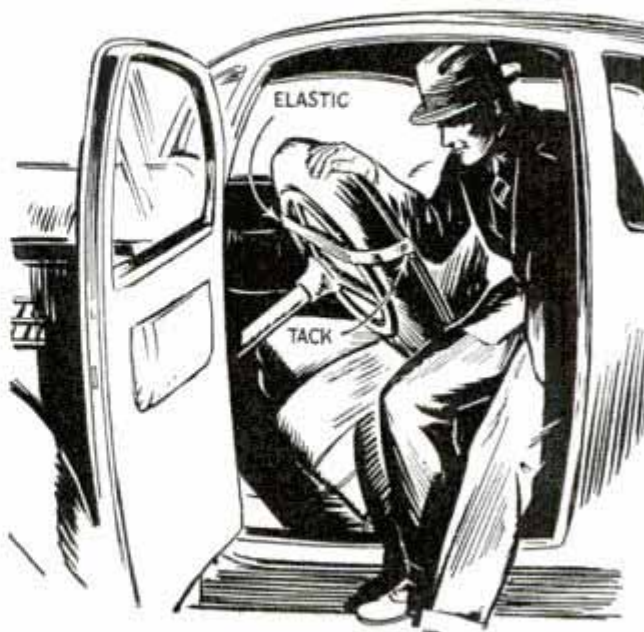
Driver's seat in coach car held against steering wheel by elastic strap
