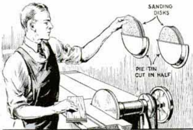
Sanding disks and grinding wheels are always at hand if kept in these holders
