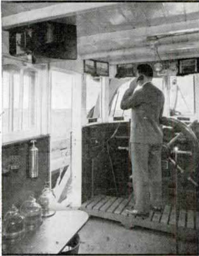
Two views of radiophone in use on commercial craft in New York harbor. Simplified system permits two-way conversations between the boats and dispatchers ashore. Both land and boat radio transmitters and receivers operate on short wave, five-watt sets being used afloat
