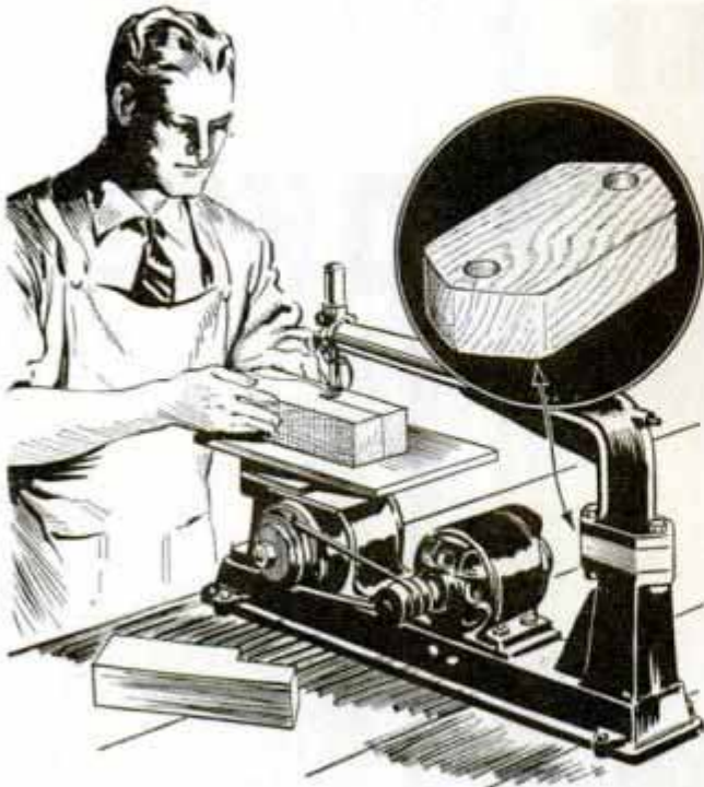
Capacity of some jig saws can be increased by using spacer block where the arm joins the base
