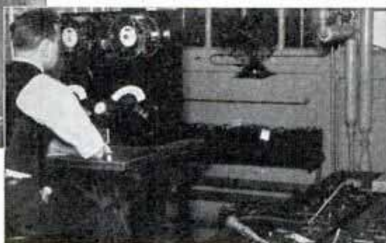
These sensitive meters accurately measure battery capacities. The batteries in the tank to the right are undergoing a normal discharge test.
