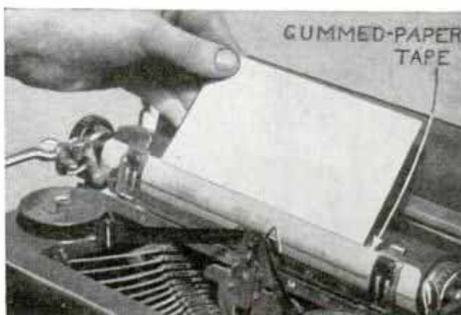
Tape confines edges of work so that it will pass around platen easily
