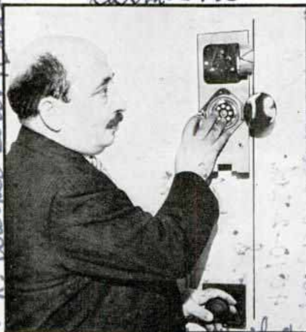
20 K. Wachter Electric Co. Wide World The right combination releases this electric lock; push the wrong button and an alarm rings
