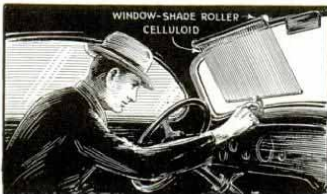
This adjustable glare shield is instantly raised or lowered to any height desired
