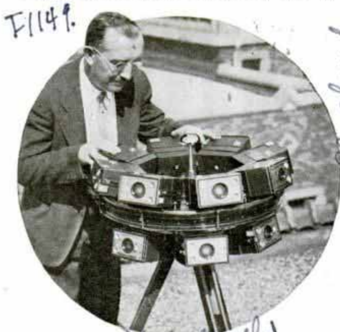
Wide World Three stationary cameras and battery of eight revolving four times a second photograph lightning
