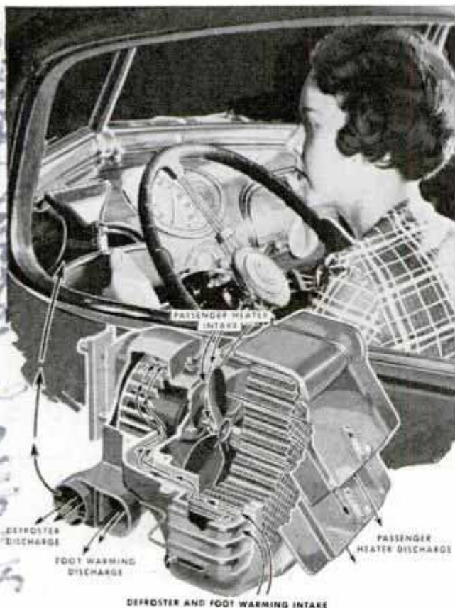
Top, defrosting unit of heater. Bottom, cutaway view of combination heater
