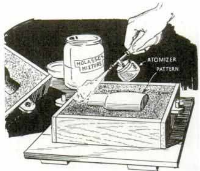
Dampening the sand around a pattern with an atomizer assures a better casting
