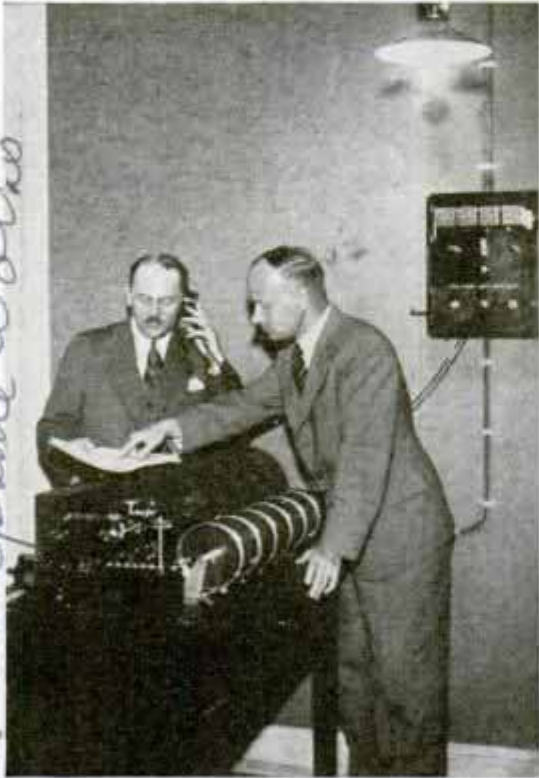
Weather bureau officials setting telephone robot to give forecast. Right, two views of the machine which "talks" to subscriber asking about the weather. Bottom view shows cabinet which houses the machine
