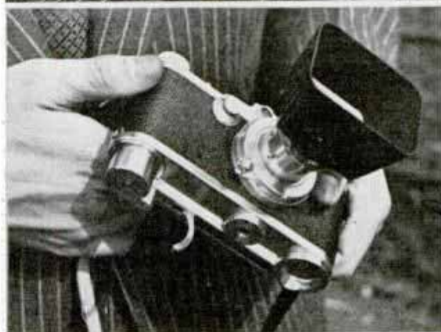
Position for taking fast sequence pictures, and view of rapid-winding trigger on miniature camera
