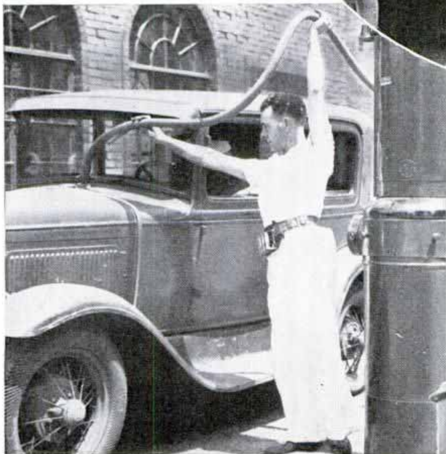
Right, arrow points to the visi-gauge on gasoline pump. Note that the gauge is only partly full, indicating that the pump has not been primed. When the gauge is in this condition, the motorist does not get full measure. Inspectors warn customers to watch the gauge on this type of pump. Where portable pumps and old-style pumps without gauges are used, the customer is forced to rely on operator's honesty
