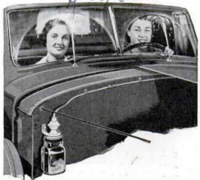
Spray of clear water from jar under hood cleans windshield at touch of button on dashboard
