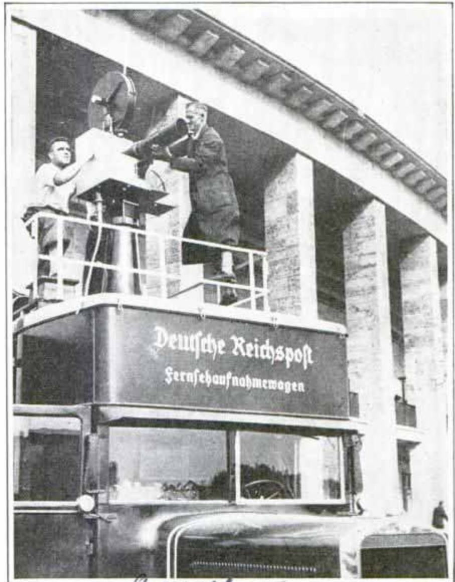
Making movies of Olympic games atop a truck, preparatory to developing the film in the truck and transmitting television images
