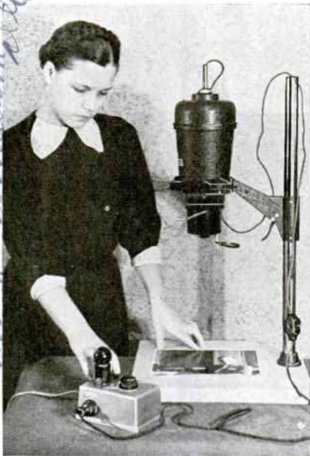
Automatic timer, on table, turns off photo enlarger at expiration of interval set on its dial
