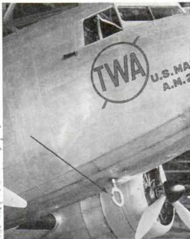
Arrow points to the shielded loop antenna which reduces static to minimum on direction finder
