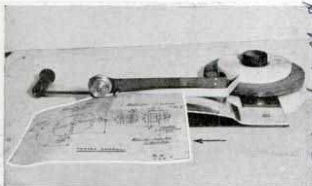
Taping machine which binds edges of sheet of paper with border which prevents mutilation from handling
