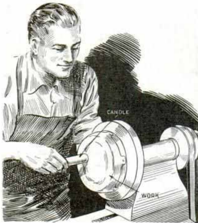
A candle rubbed on the surface of metal-spinning work lubricates it nicely
