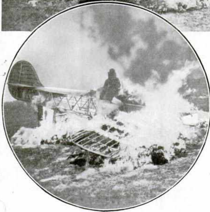
Photos by Authenticated News Fire fighters clothed in asbestos suits standing amid flames of blazing ship and, below, man in asbestos leaving plane after sitting in blazing cockpit for five minutes
