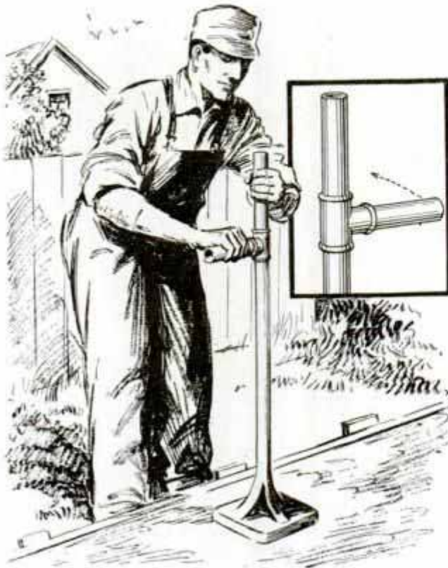
Twisting the tamper slightly tends to break the vacuum between it and the wet material
