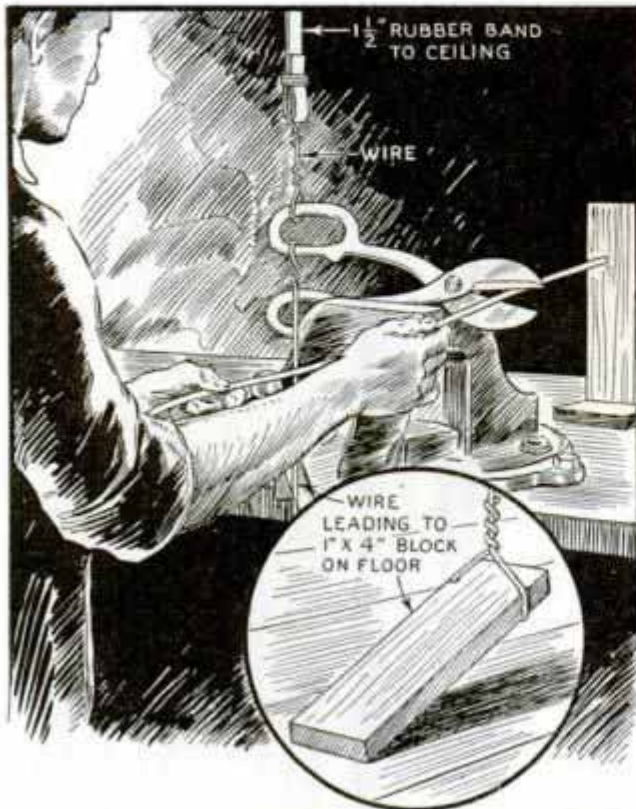
Small shop owner quickly turns out large order for short wires with foot-operated shears
