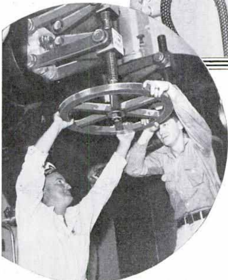
Top, baby steering wheel attached to "metal mike" on bridge with which liner may be steered. Below, opening main steam line leading to turbines. Getting up steam requires several hours on a modern ship
