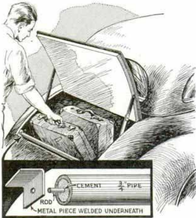
Lifting and straining is unnecessary to remove heavy luggage when you use this roller
