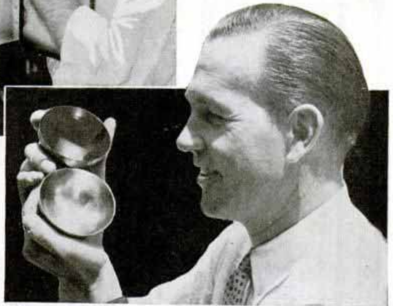
Testing volatility of fuel to which dope has been added and, below, discoloration of upper dish shows excessive gum formed in a doped gasoline
