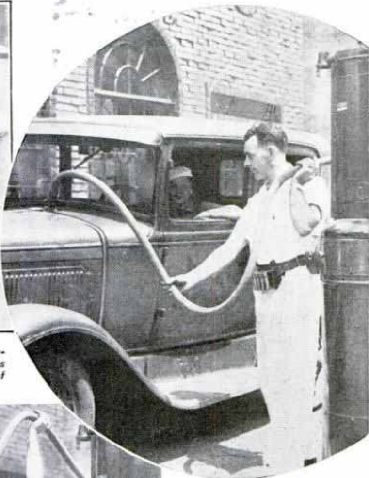
Above, improper way to drain "dry" type of hose. This type has no valve-controlled nozzle and motorist should receive all the gas in the hose. Bottom, left, proper way to drain hose so motorist gets what he pays for. By holding hose in this manner, all the gas runs out of line into customer's tank. Shortages up to one and one-half quarts result from improper drainage
