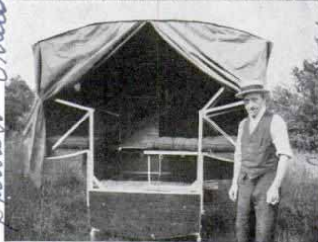
One-wheel trailer which folds into compact unit on road and expands into a home when parked
