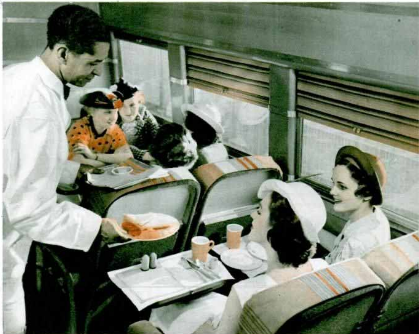
LUNCHEON on the transcontinental streamliners is served on a tray that folds into the seat ahead.
