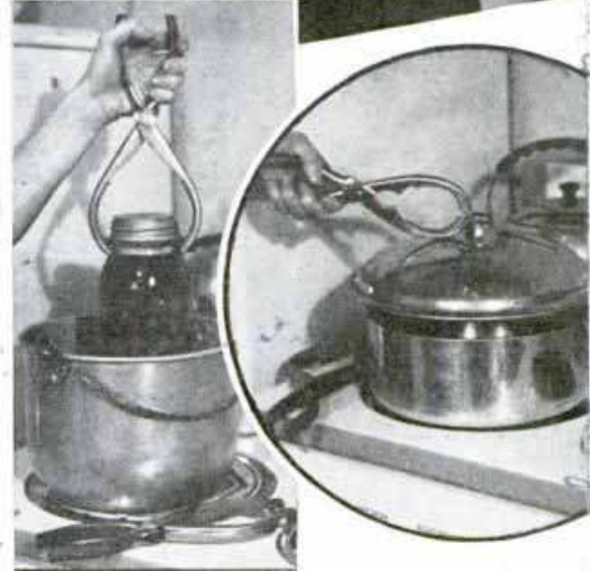
Rubber-toothed wrench is put to varied uses around kitchen lifting hot dishes and gripping jar lids
