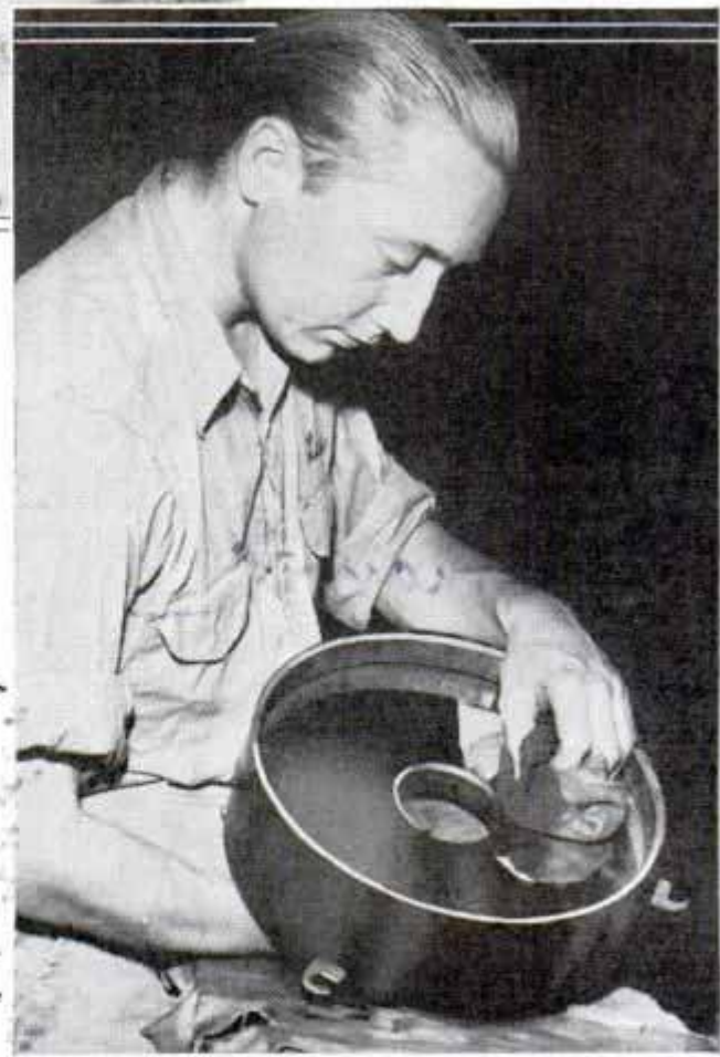
Polishing surface of twelve-inch mirror, and large amateur telescope with skeleton tube
