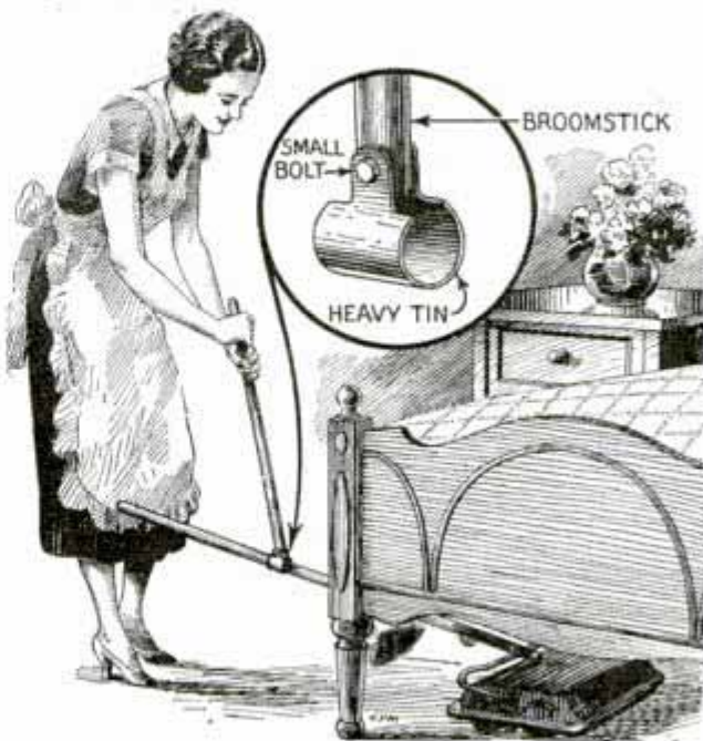
You can clean under low furniture with this sweeper without stooping sharply
