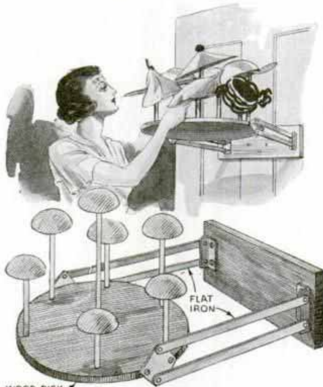
WOOD DISK This rack raises and lowers, the parallel links holding it horizontally in any position
