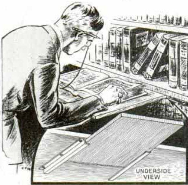
Sliding board saves steps by holding books while looking up reference data
