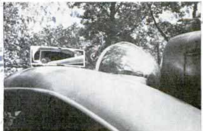
Mounted on left front fender of his automobile, this curved mirror gives deaf motorist a broad view of traffic to rear
