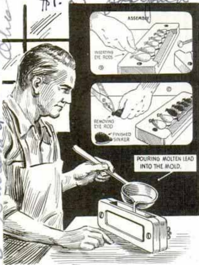
Sinker mold for the angler which turns out smooth, balanced pellets in six sizes
