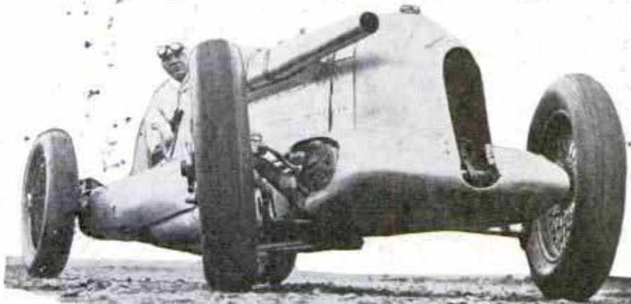
Acme It looks like a cannon mounted on an armored car, but it is really the air intake duct for the supercharger of a racing automobile
