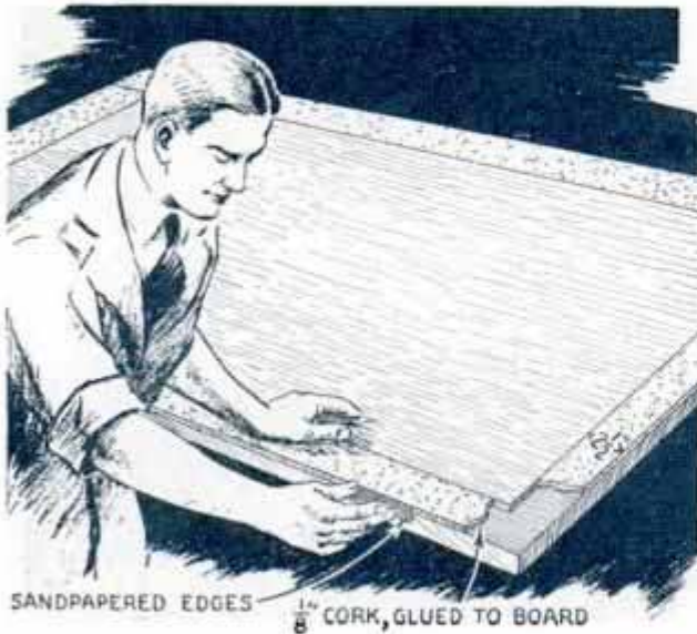
Drawing boards that are marred near the edges from thumbtacks are renewed with cork inlay
