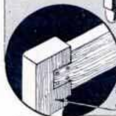
MORTISE ON HINGED LEGS. LEG IS CUT AWAY ON ONE SIDE
