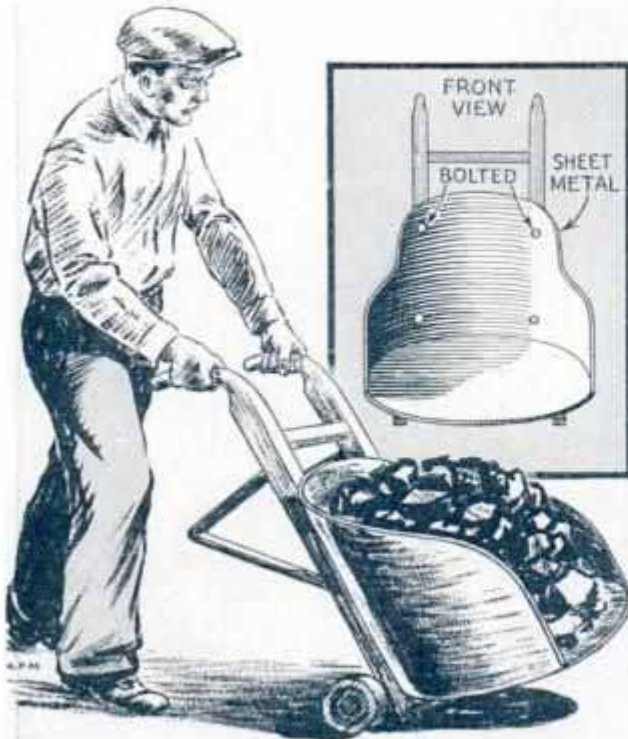
This scoop is handy for moving dirt, ashes, or objects that are too heavy to carry
