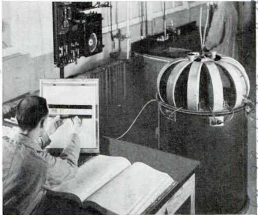
Apparatus used in taking "fingerprints" of unknown chemical substances for comparison with "prints" of compounds already identified
