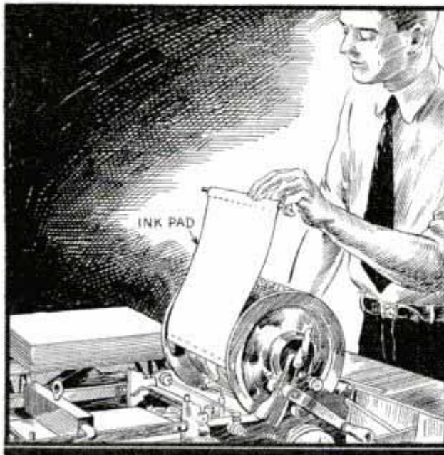
Lifting one end of the ink pad shifts the cloth fibers to make the pad porous
