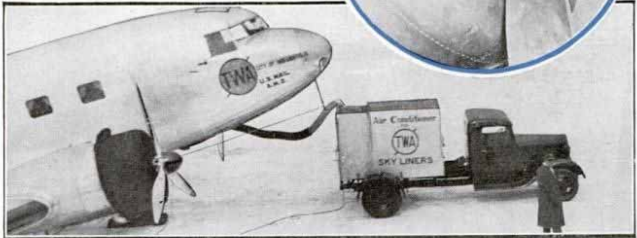
Keeping log of arrivals and departures in traffic control tower. Below, air-conditioner cooling cabin of sky liner and de-icing tubes on propeller hub
