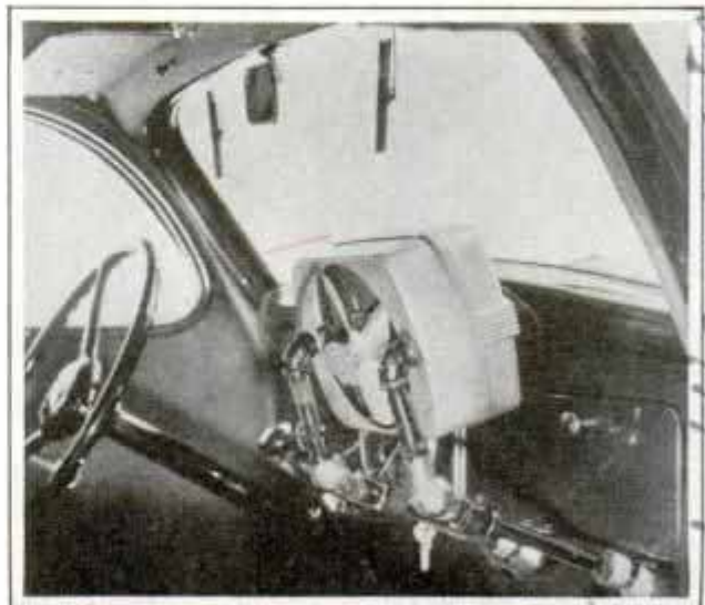
Heater swung up to windshield, ready to eliminate frost. It adjusts to several positions
