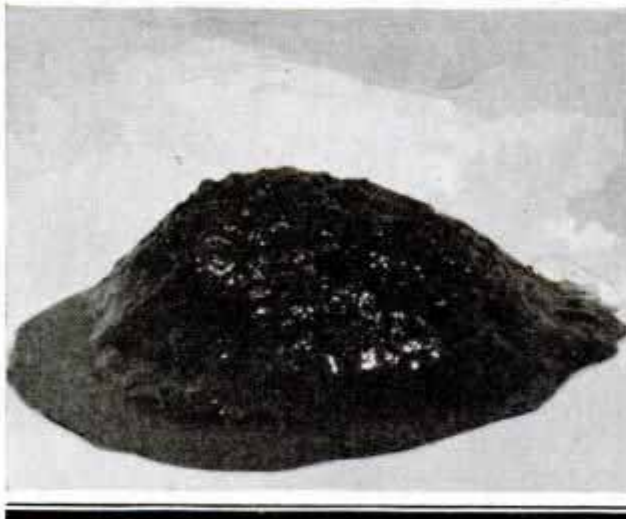
Top to bottom: Cracked block caused by overheating due to corrosion; corrosion spots; clogged radiator core, and sediment from cooling system
