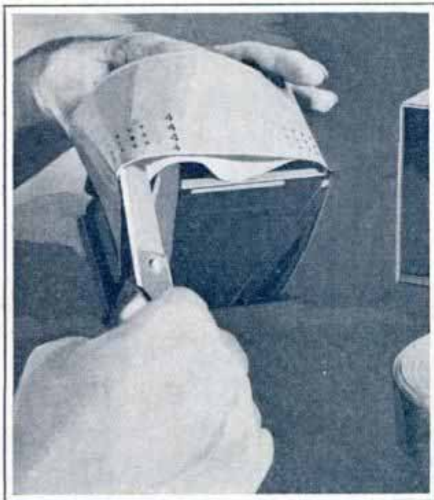
Just cut off exposed film and cement end of unexposed film to paper backing
