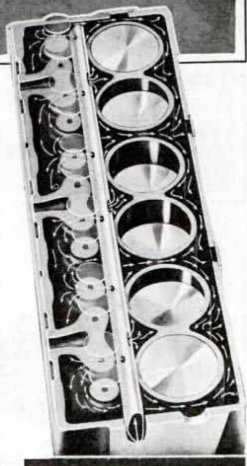
Top, testing engine. Bottom, engine with valve seats sprayed by water must have clean cooling system
