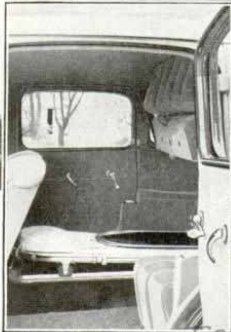
Top, cutaway showing patient on stretcher in police car. Bottom, left and center, views of stretcher in car. Right, stretcher folded in trunk
