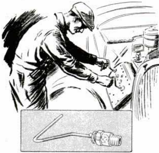
These hand grips screw into the spark-plug holes so both ends of the cylinder head are lifted evenly
