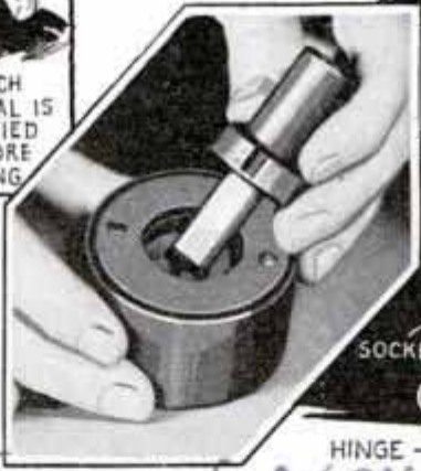
Above, chassis die for punching socket holes in metal bases; Right, tube socket mounted on small hinge provides variable coupling with plug-in coils
