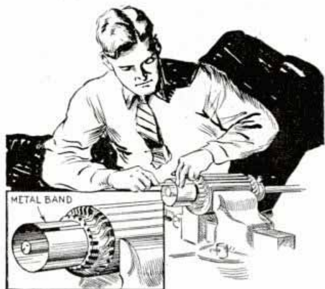
Sleeve with slot in side shields commutator segments when undercutting the mica strips
