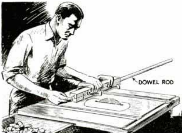
With this jig, you can cut any number of dowels quickly without feathering the edges.
