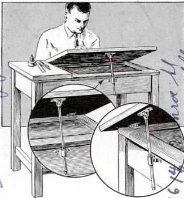
Self-locking adjustable table top is a convenience for the artist or the draftsman
