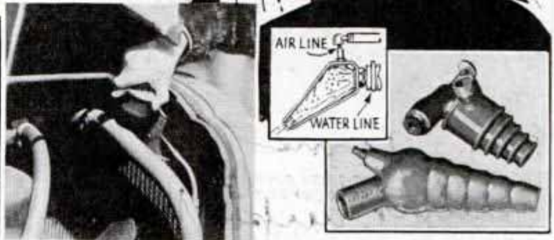
Several views of method and equipment used in pressure cleaning of auto cooling system. Air pressure is necessary to remove heavier sediment. The radiator core may be tested by removing the cap and watching water level as engine is raced. If water rises and spills over, the core is clogged
