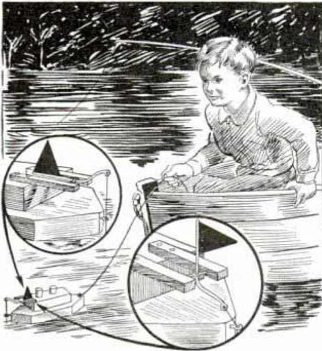
The flag on this fishing float rises suddenly when a fish takes the bait
