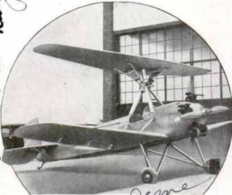
Acme Vertiplane is designed to hover in air supported by upper wing which rotates after gaining altitude
