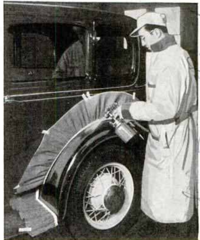
Adhesive tape which leaves no mark holds crepe paper protecting body of car while painting
