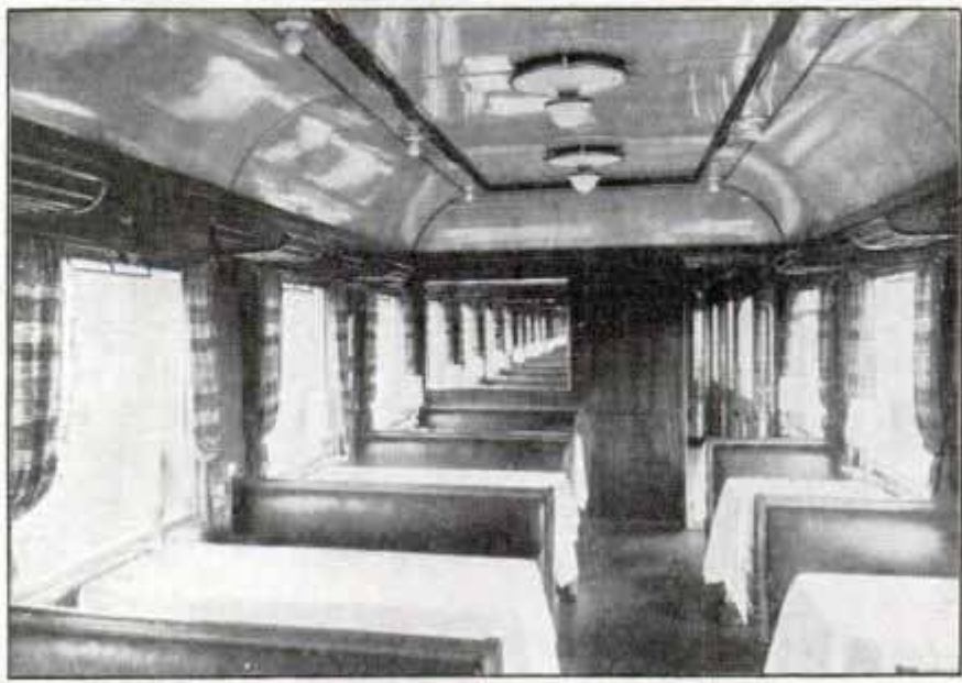
Dining car of the German lightweight train, the "61,001," with double tables on one side and singles on the other
