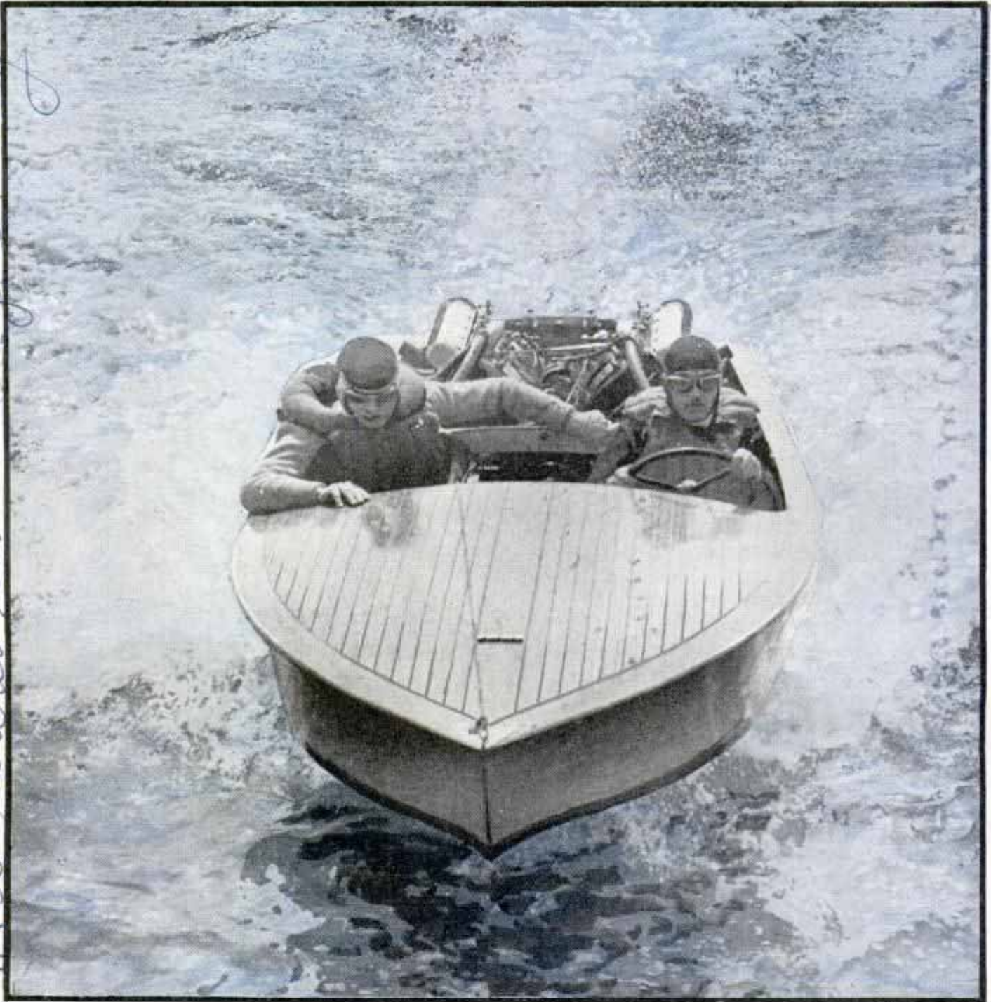
A. L. Bobrick and mechanic roaring down the course in his hydroplane, "El Torbellino," a fourteen-foot torpedo driven by a 400-horsepower airplane motor
