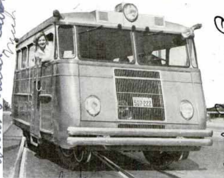
Hauling up the flanged wheels, the driver of this eight passenger car steers away from rail to highway on rubber tires
