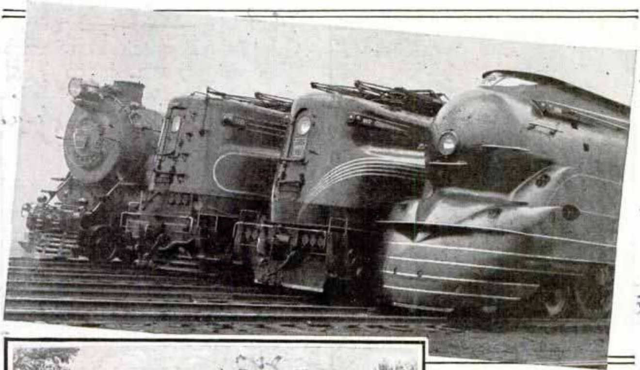
The line of locomotives above shows how the cowcatcher has gradually disappeared behind a solid wall of steel as streamlining has advanced. Left, an early cowcatcher
