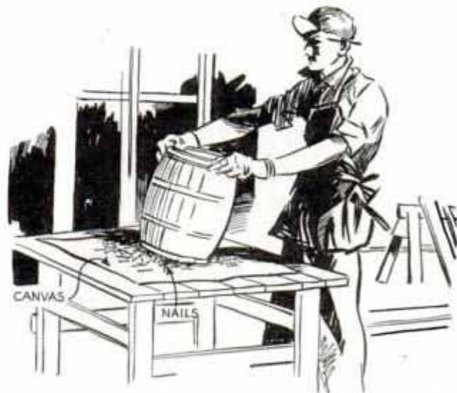
Carpenter quickly fills his apron when nails roll from inverted keg on canvas-covered bench
