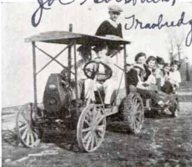
Small tractor constructed of old auto parts. It does light hauling about the farm
