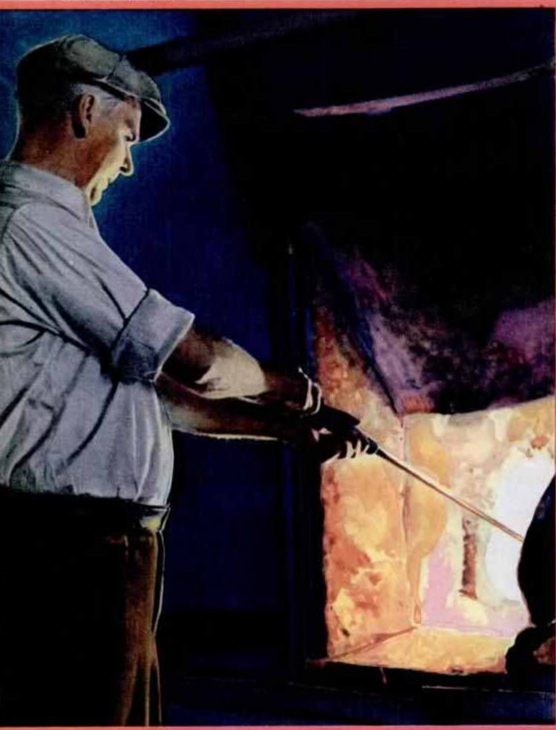
G LASS gatherer removing a white hot ball from the melting furnace for the blower. Temperatures of from 2,400 to 2,800 degrees Fahrenheit are required to melt the mass of sand and other raw materials which compose glass.
