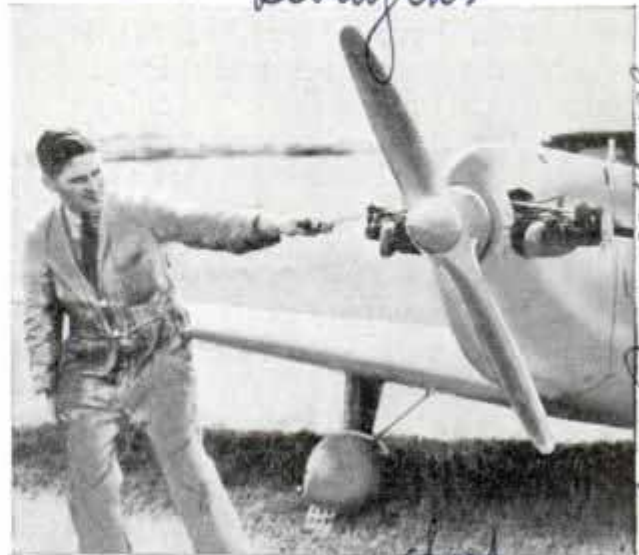
Using pull cord to start engine of British plane in same manner as outboard motor is started
