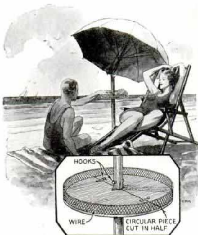
Tray for small articles is quickly removed when umbrella is folded for carrying
