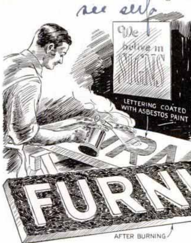
Lettering coated with asbestos paint is untouched while surrounding wood surface is deeply charred
