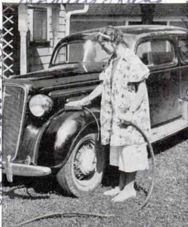
Rubber sponge for washing car is supplied with water by attaching tube to garden hose
