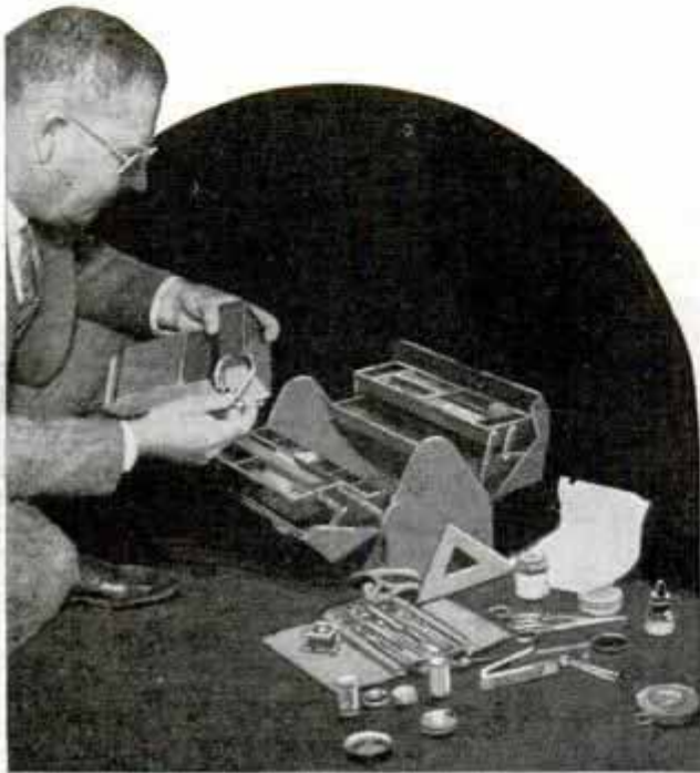
Instrument kit carried by fire detectives when searching for the cause of a blaze
