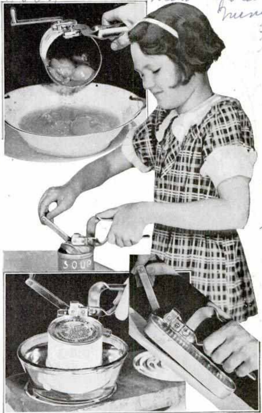
Above, using can opener as holder. Center, removing top by turning crank. Bottom, lifting can from hot water and removing rectangular top
