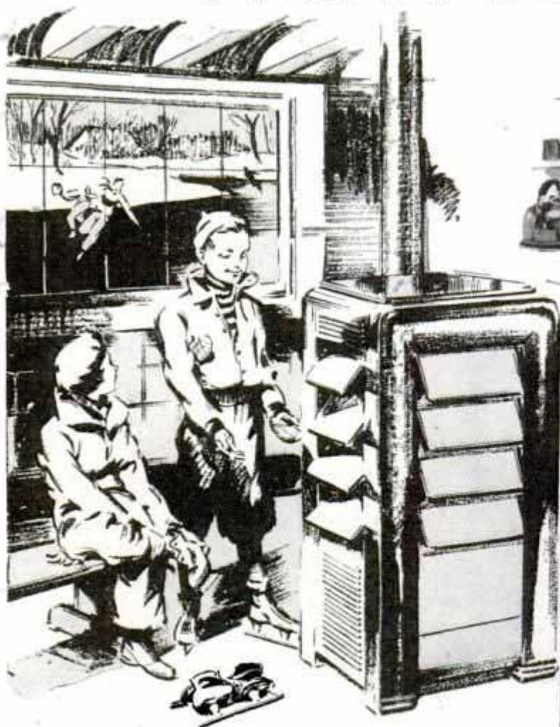
Left, oil-burning heater with adjustable shutters to direct heat where desired. With shutters open, radiating heat is supplied, and with shutters closed, the heat is circulated. It burns fuel oil without requiring machinery, wick or lighting ring to atomize the oil. Above, aluminum mixing bowl with electro-hardened finish. Note the grip under which the hand slides
