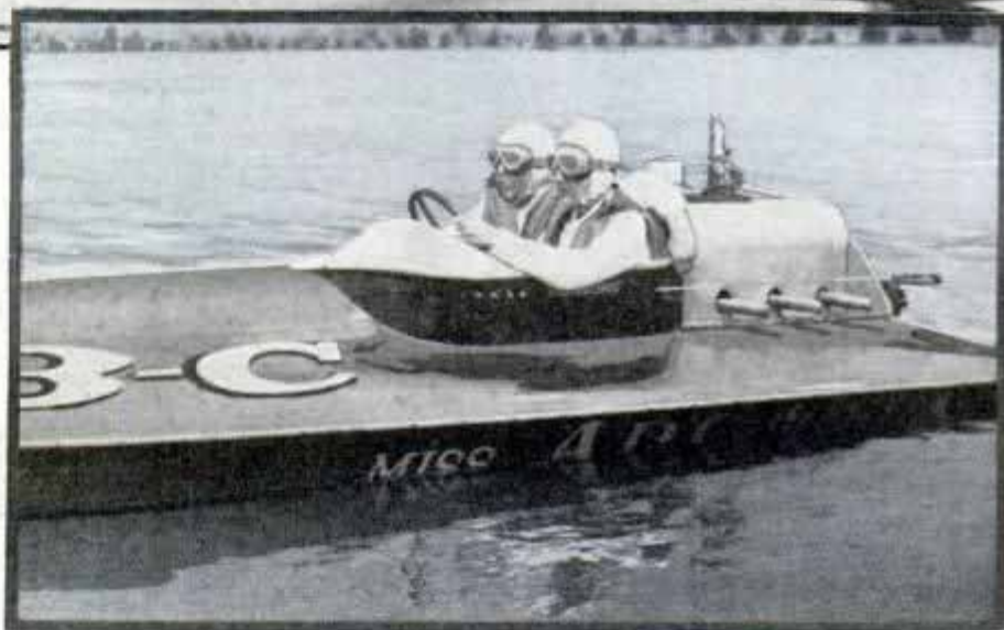
Top, outboard speedboat riding on "step" which reduces drag of water. Below, 225-class speedboat with V-8 engine in rear
