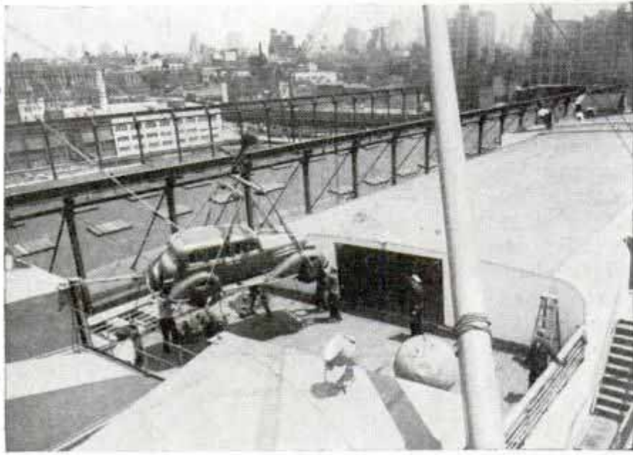
Hoisting tourist's automobile by crane to deck of ocean liner, where it is stored in garage during trip
