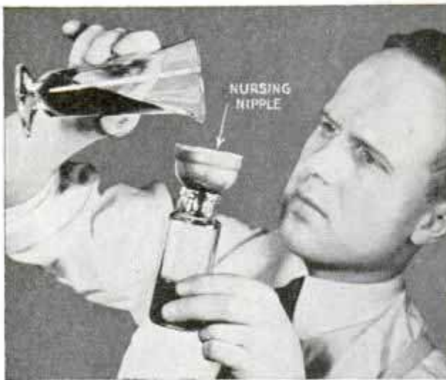
Cut off the tip of a rubber nipple and you have a handy funnel for use in the home laboratory
