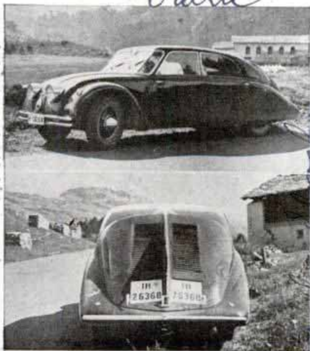
Back and side views of rear-engine car
