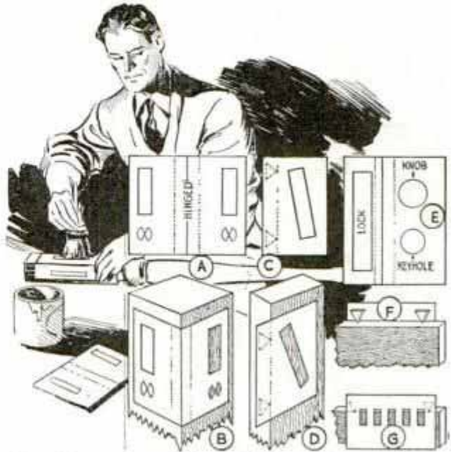
Hinged stencils used instead of templates to lay out mortises, grooves, dovetails and similar work
