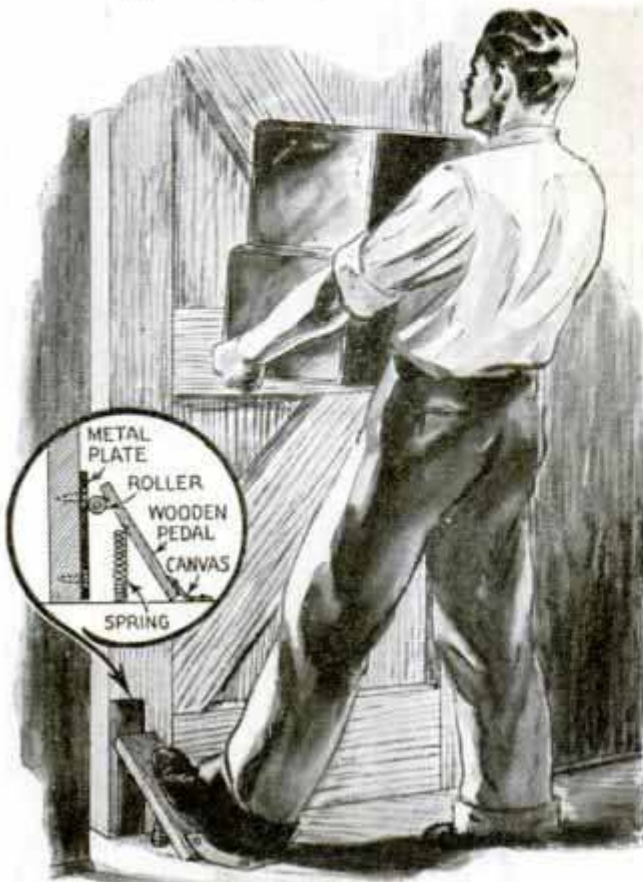
Workman approaching with both hands full steps on treadle to swing heavy door open
