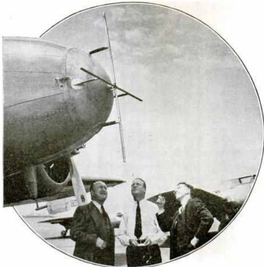
New antenna on nose of plane picks up signals which make possible blind landings with an automatic pilot at the controls
