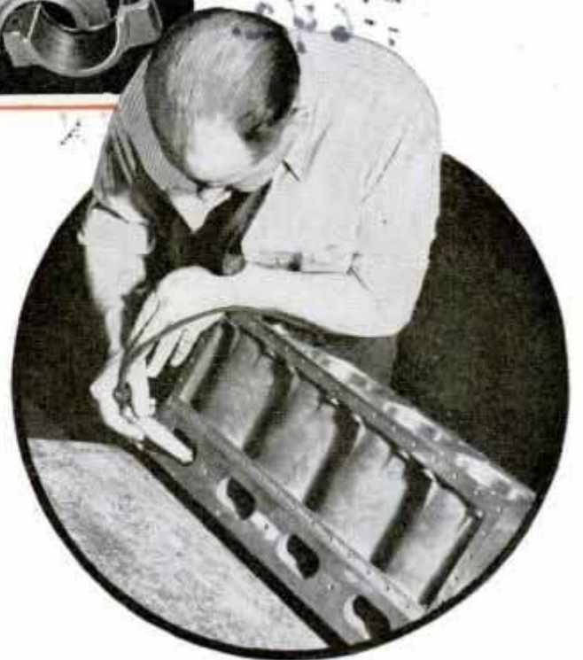
Top, lathing bell housing. Center, from forging to finished connecting rod. Bottom, polishing ports in engine head, shown upside down
