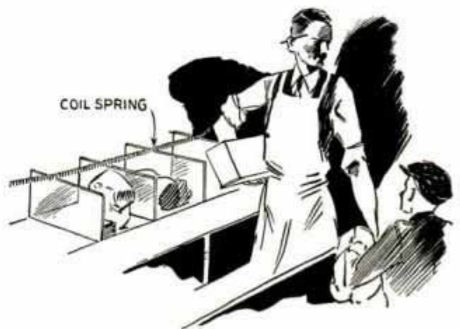
Compartments are quickly made to any size and the dividers can be stored when not in use
