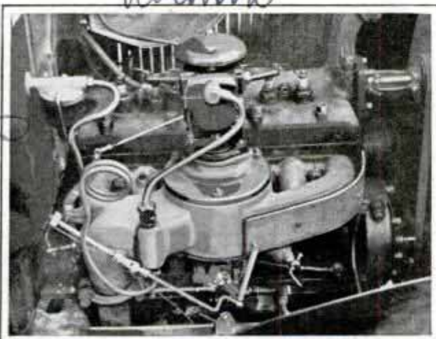
Carburetor for converting auto to oil burner is shown attached to motor
