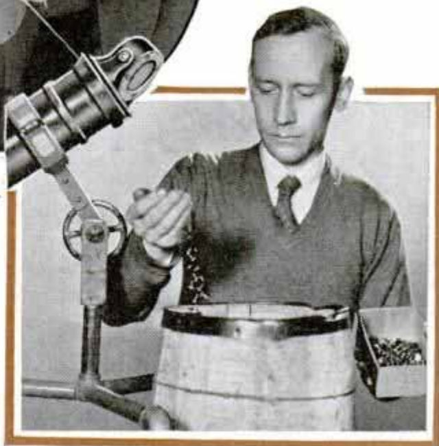
Dropping tacks in a barrel sounds like rocks falling on a roof after the noise has been passed through the movie microphone and recorded on reproduction equipment
