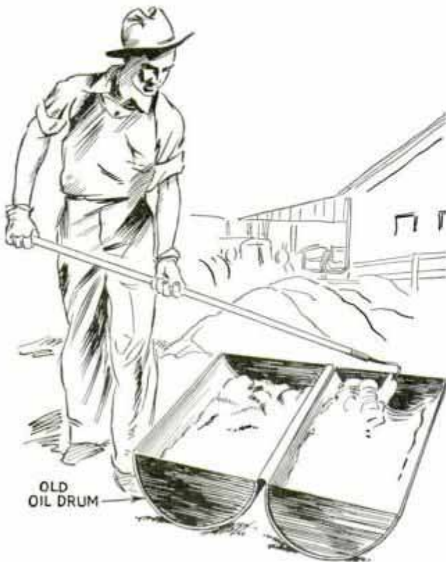
The sloping sides of the box make it easy to scrape the mortar from one compartment to the other
