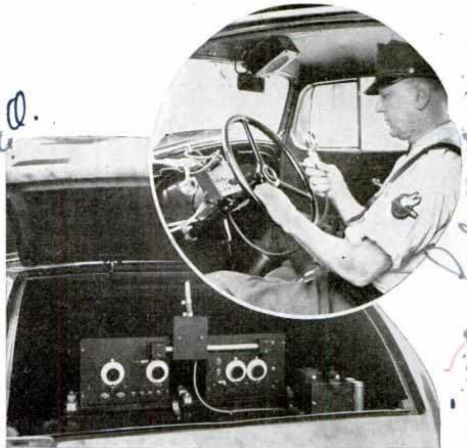
Dual sending and receiving sets are mounted in trunk at rear. Operator throws switch on dashboard to send power to receiver or transmitter
