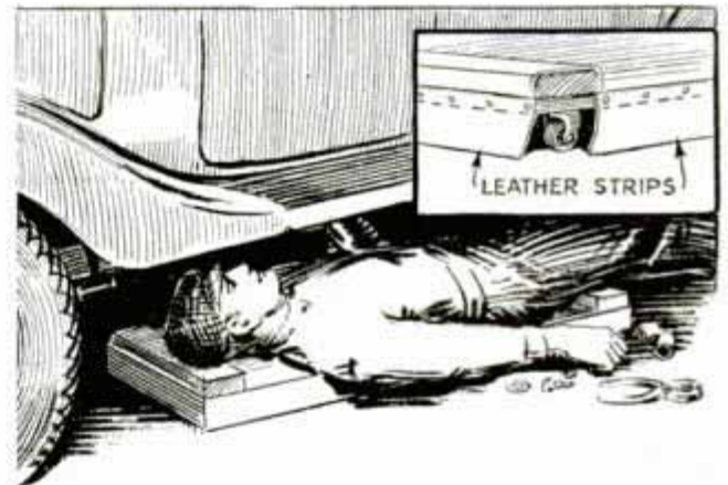
"Fishing" for small parts that have rolled under a creeper is stopped with this apron
