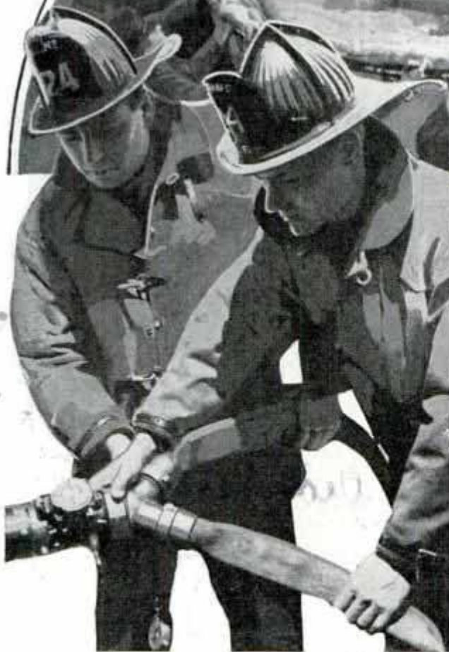
Attaching a "siamese" to large hose to get two smaller streams of water
