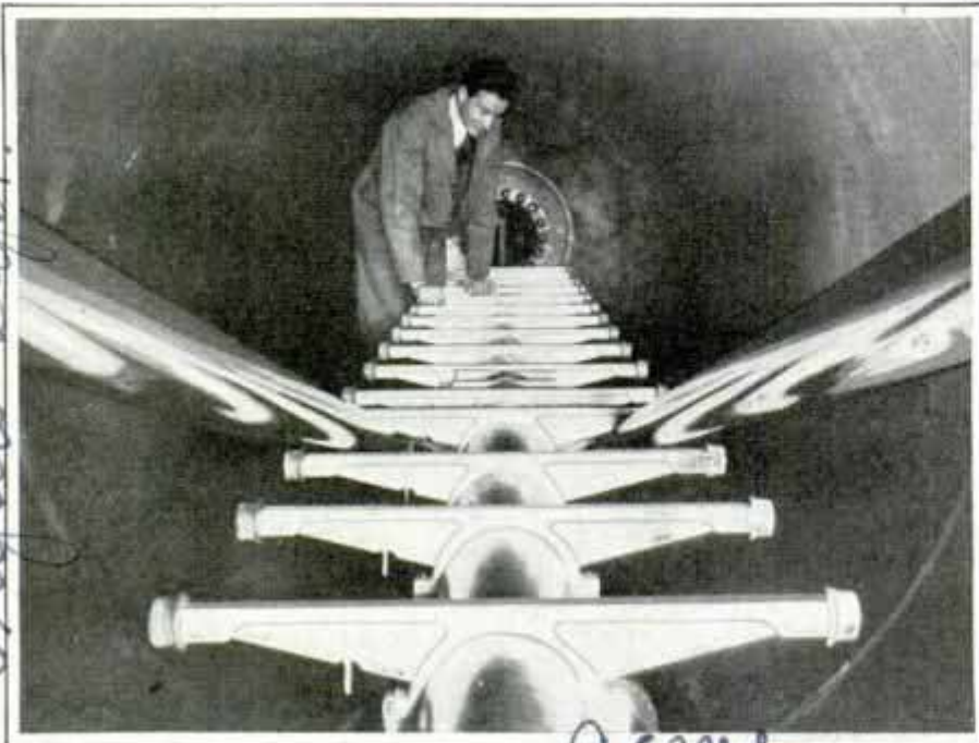
Interior of giant generator which manufactures the electrical charges to be fired into the heart or core of the atom
