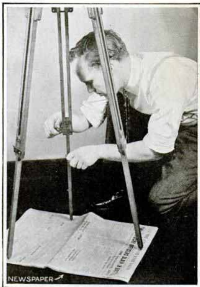
Several layers of newspapers will keep the feet of a tripod from slipping on a hard surface
