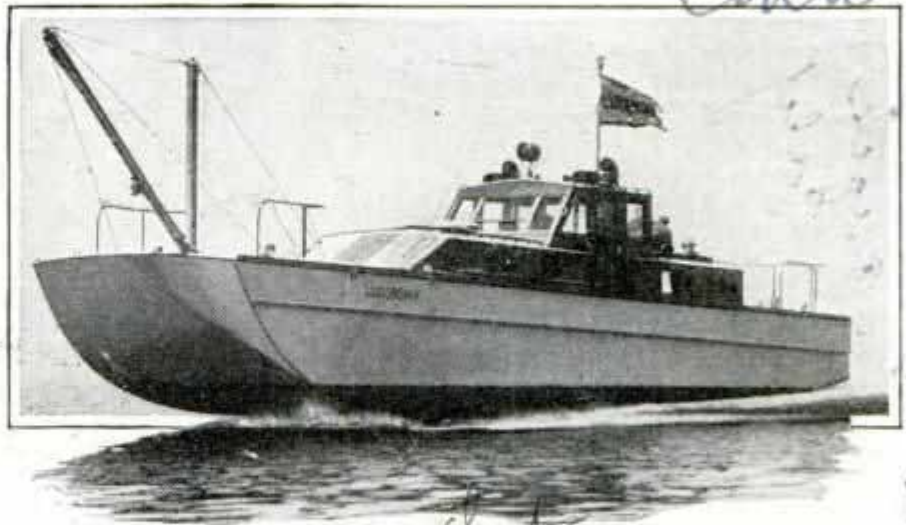
Crash boat equipped with derrick for salvage work and first-aid hospital travels at thirty-nine knots to aid seaplane in trouble
