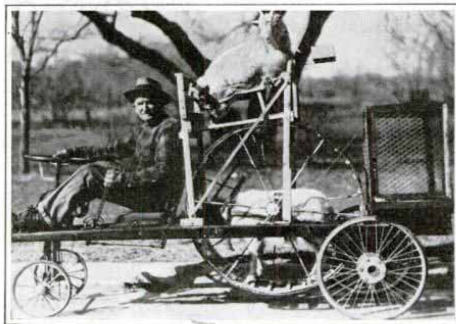
Complete to steering wheel and brake, this animal-power vehicle moves slowly but surely. Note the extra "motor" riding on top
