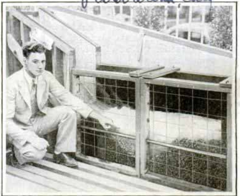
Glass model demonstrates how rush of water at foot of spillway cuts deep into bed of stream
