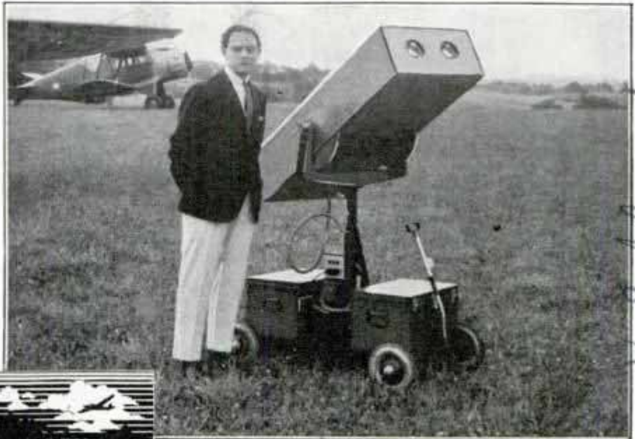
Top, Petoscope's twin eyes watch sky above airport. Left, light reaches photocells through lenses and screens of opposite pattern
