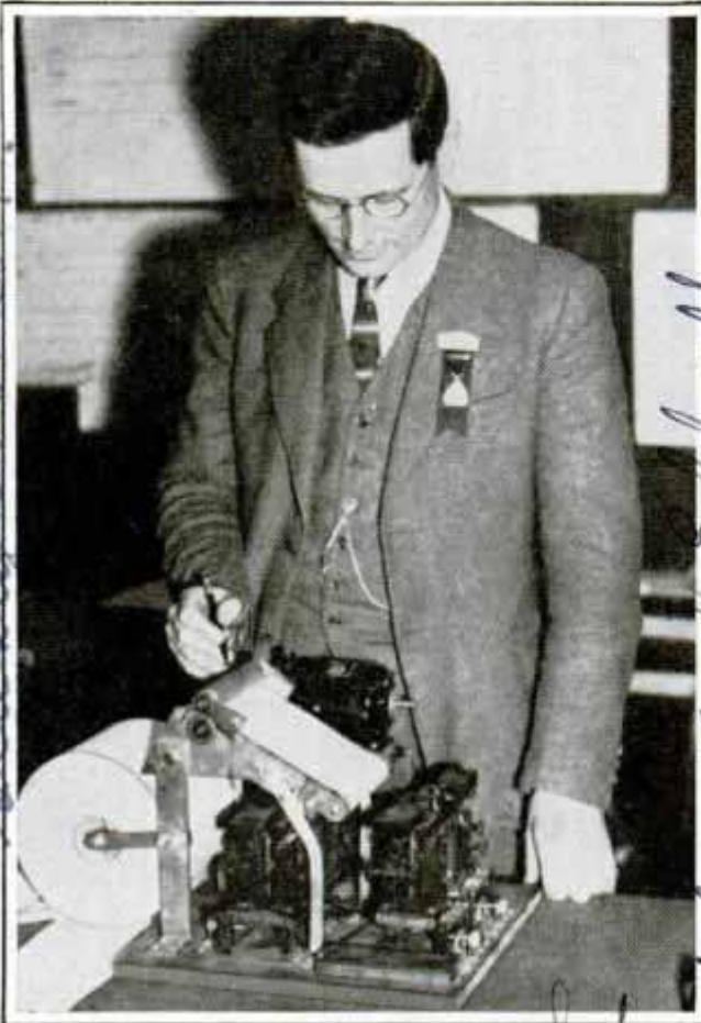
Electrical impulses generated in the human brain are measured and recorded by this "meter"
