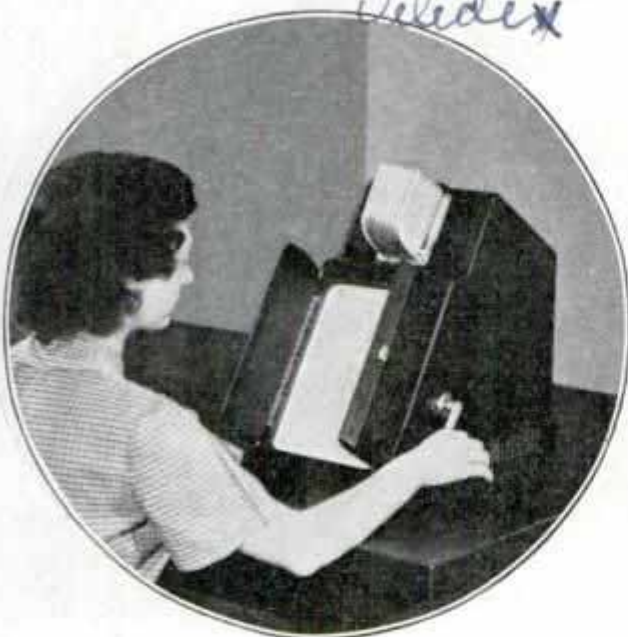
Operating the reading machine which magnifies the small film to book page size. Note that the machine is small, designed for individual use
