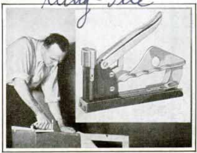
Self-feeding hammer, worked with one hand, drives tack with trip-hammer effect when lever is pressed
