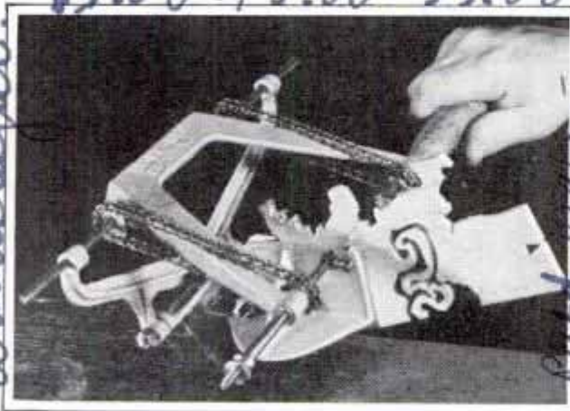
Plywood is held firmly in grip of vise while hand guides fret saw in intricate pattern
