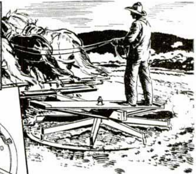
The blade of this weeder rotates slowly as it is pulled forward, thus having a tendency to free itself of trash as it loosens the soil and destroys the weeds
