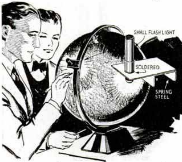
Turn globe to bring lettering under ring and then adjust flashlight directly above it
