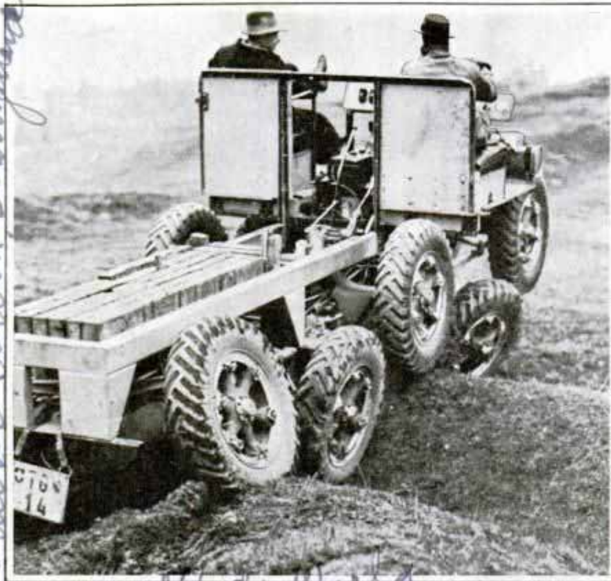
Note how body of truck remains level while the articulated wheels rise over high spots or sink into depressions while traveling rough country
