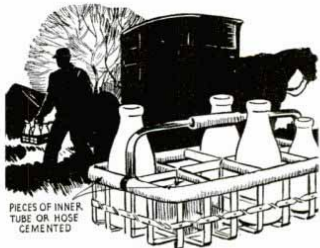
Rubber strips wrapped around upper members of tray prevent empty bottles from touching metal frame
