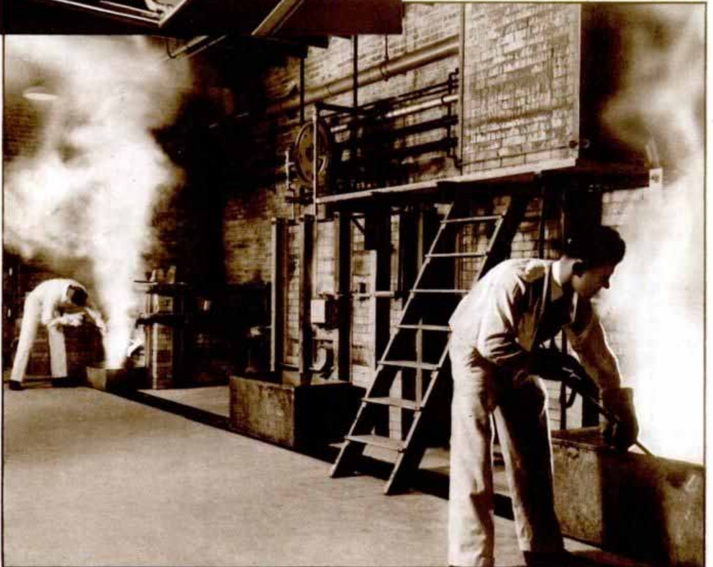
REFLECTOMETER , above, being used to determine opacity or light reflecting properties of a sample of porcelain enamel. Below, tapping off a batch of molten enamel in experimental smelter of Chicago Vitreous Enamel Product Company's "Lusterlite Laboratories."
