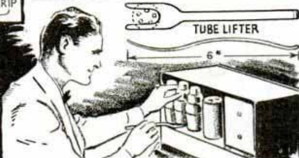
Upper left, small porcelain lead-through bushings make handy insulated supports for mounting fuse or high-voltage knife switch. Left, oil-filled transmitting condenser in round aluminum can, is provided with a metal mounting ring. Below, simple tool for removing tubes from midget receivers is formed from a piece of thin steel, or other stiff metal, and shaped like a wide-tined fork. The space between the curved tines is slightly wider than the distance between opposite tube prongs
