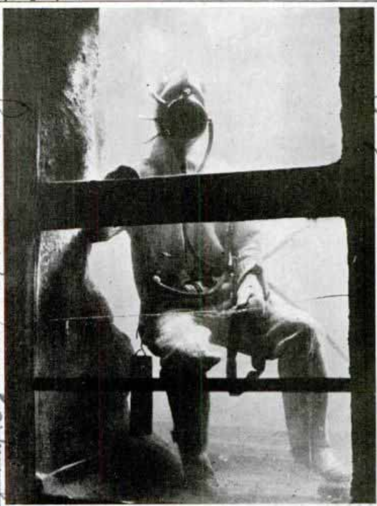
Inventor demonstrating the heated suit which, by means of hot water pumped from the surface, keeps diver comfortably warm
