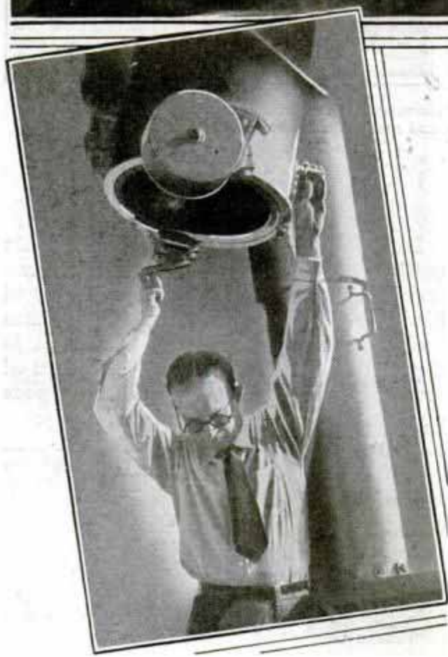
Training mirror of sun telescope on spectrohelioscope for studying sun's elements
