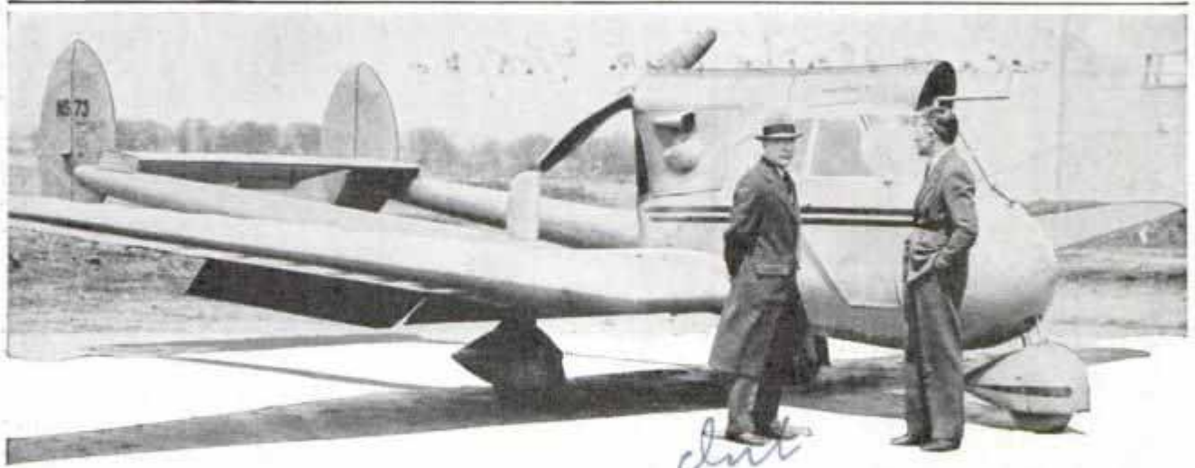
Int Low-wing Hammond monoplane tested by department of commerce inspectors. It purposes to meet the need for a "foolproof" ship that an inexperienced pilot could fly safely. Notice landing wheel under nose
