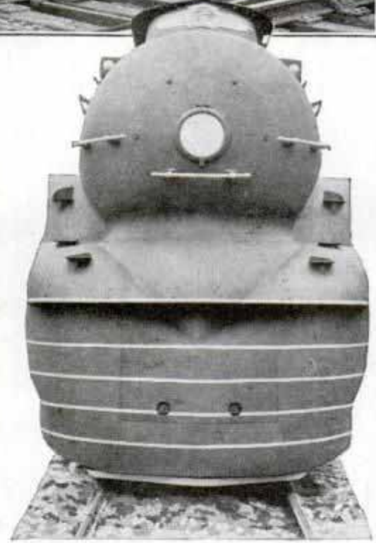
Top, Pennsylvania's standard steam locomotive, two electric types and new streamliner. Drawings show path of smoke above old and new engines. Right, nose of streamliner showing smoke "wings"
