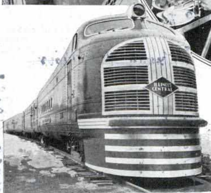
A head-on view of the "Green Diamond," and the control cabin. In addition to the sixteen-cylinder, two-cycle, high-compression Diesel engine which generates the electricity to run the train, the power car also contains an engine cooling and exhaust system, storage batteries, charging equipment and an auxiliary engine for lighting and air conditioning
