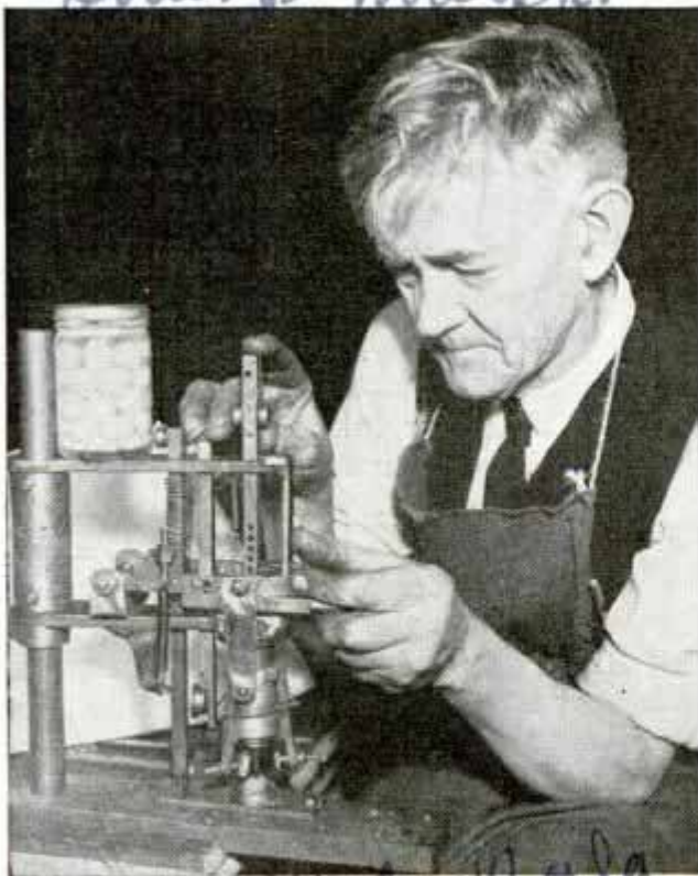
Cherry and olive pitter which removes seed when vertical bar is pressed and raised
