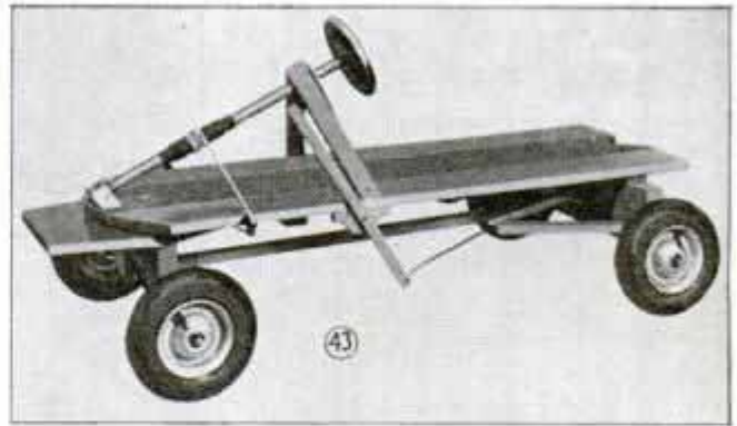
It's important that the ropes or cables of the steering gear pull evenly and in line. On the car shown above, the steering gear swings the front axle
