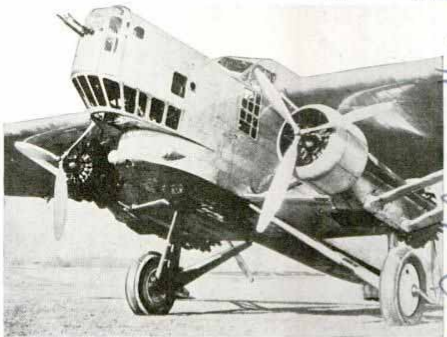
Giant bombing plane recently adopted by French army. Note the turret with twin guns for fighting off enemy aircraft
