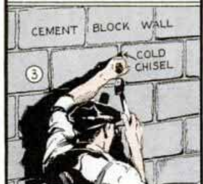
FOR BRICK, STONE OR CEMENT-BLOCK FOUNDATIONS ALL MORTAR JOINTS ARE CUT TO V-SHAPE, THEN BRUSHED WITH CEMENT
