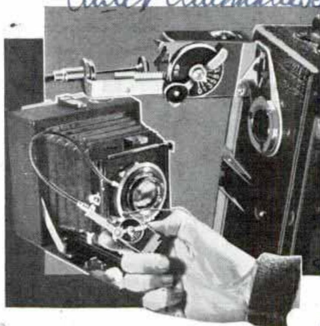
Self-timer for camera shutter, showing how dial is set for time exposure with delayed release
