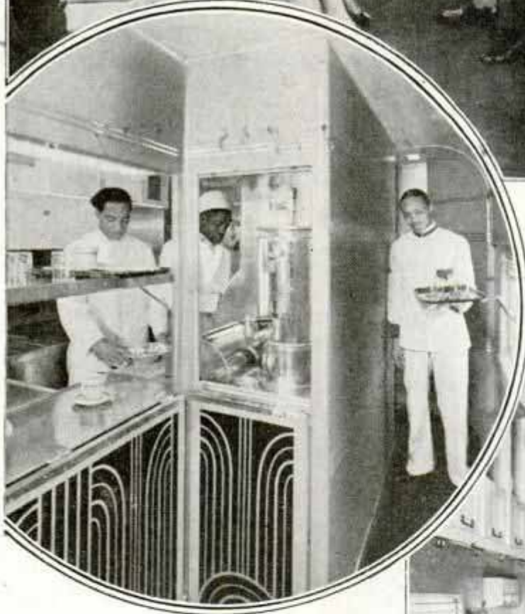
Kitchen and mail-handling section of mail-baggage car of the "Green Diamond." The train is constructed of steel and aluminum, is air-conditioned, weighs 230 tons, half the weight of a standard steam train, and is expected to make its 300-mile run in less than five hours
