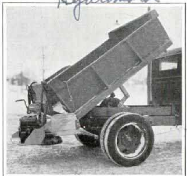
Body of truck in dumping position, controlled by balanced power, gearless hoist
