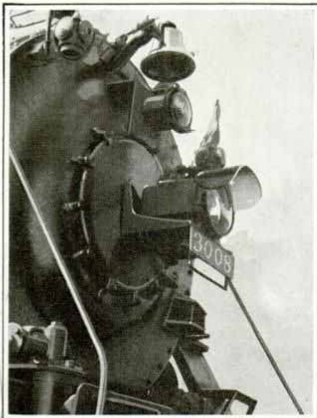
Red headlight directly under bell flashes warning that tells crew of passing train to stop immediately
