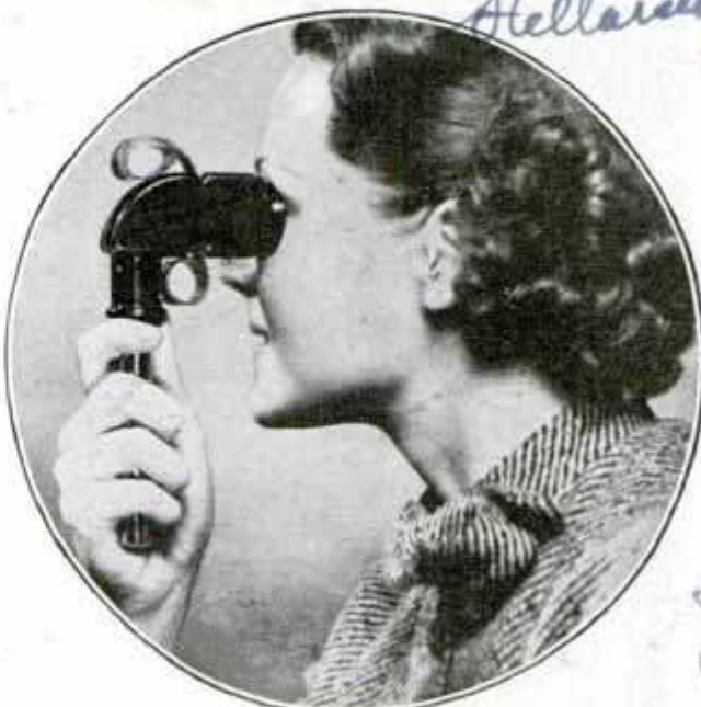
Demonstrating the stellarscope. Film shown at top and bottom contains sky maps
