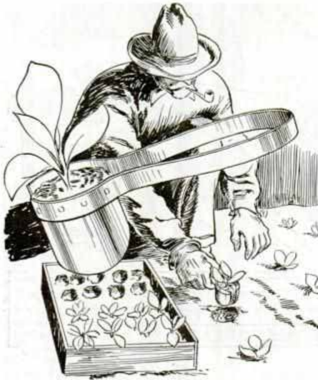
Immediate growth of transplanted flowers is not retarded when this tong-spade is used
