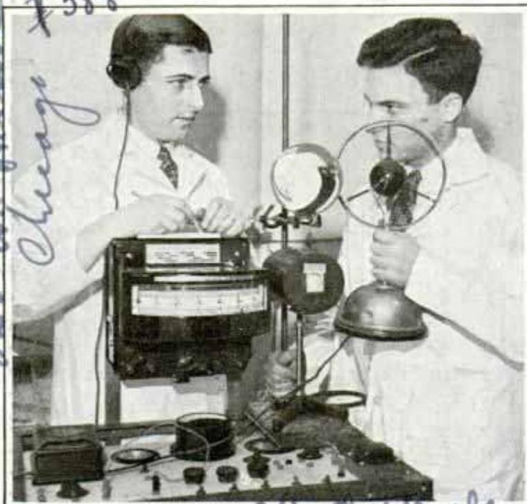
Talking into microphone, speaker's voice travels over infrared wave to photocell and is translated back to sound
