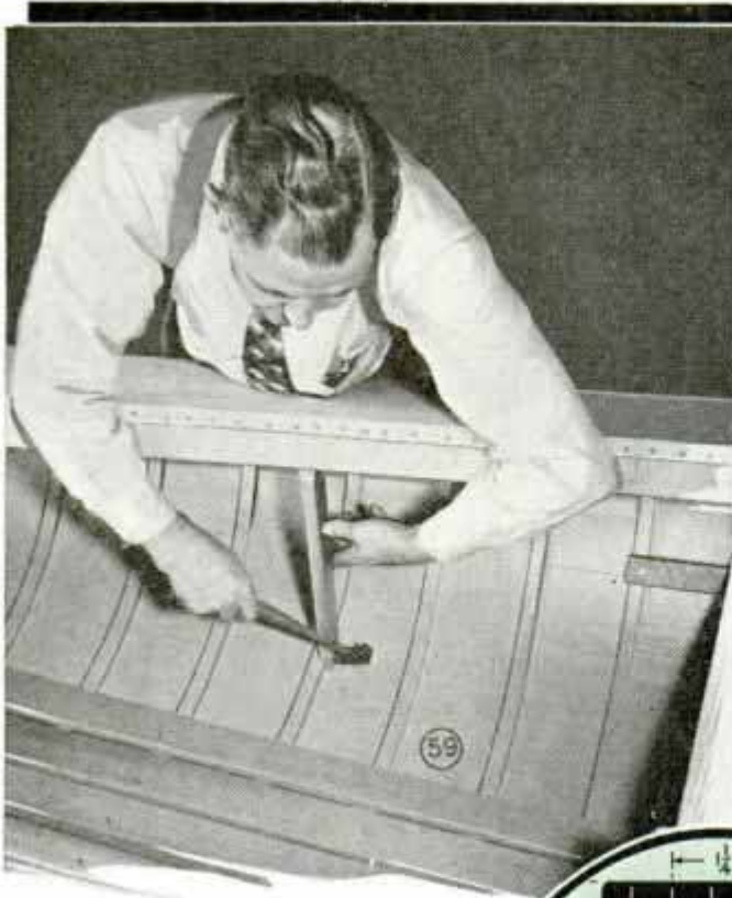
Braces along the sides of the cockpit carry the strain down to the ribs, thus giving ample strength to support persons sitting on the edge of cockpit
