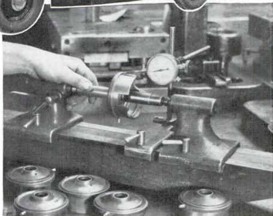
This gage makes sure that the distributor bearing is at right angle with the face of the advance housing flange.
