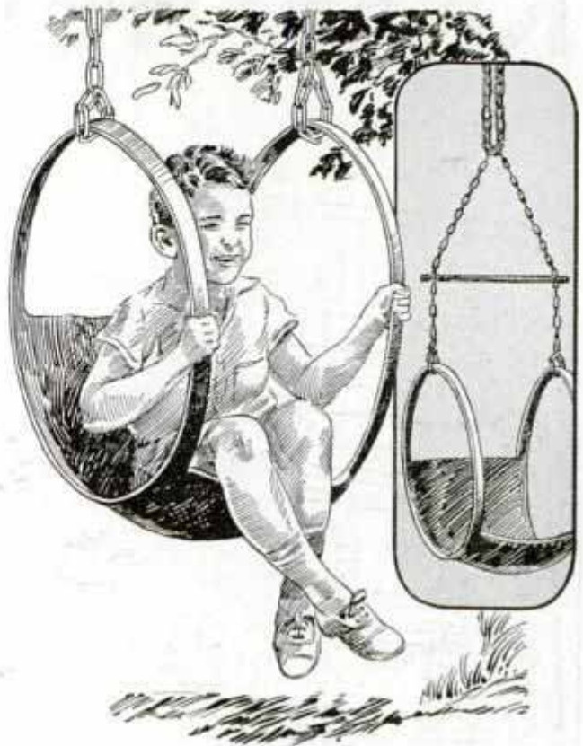
Carcass of truck tire between the beads is cut away to leave enough tread for a comfortable seat
