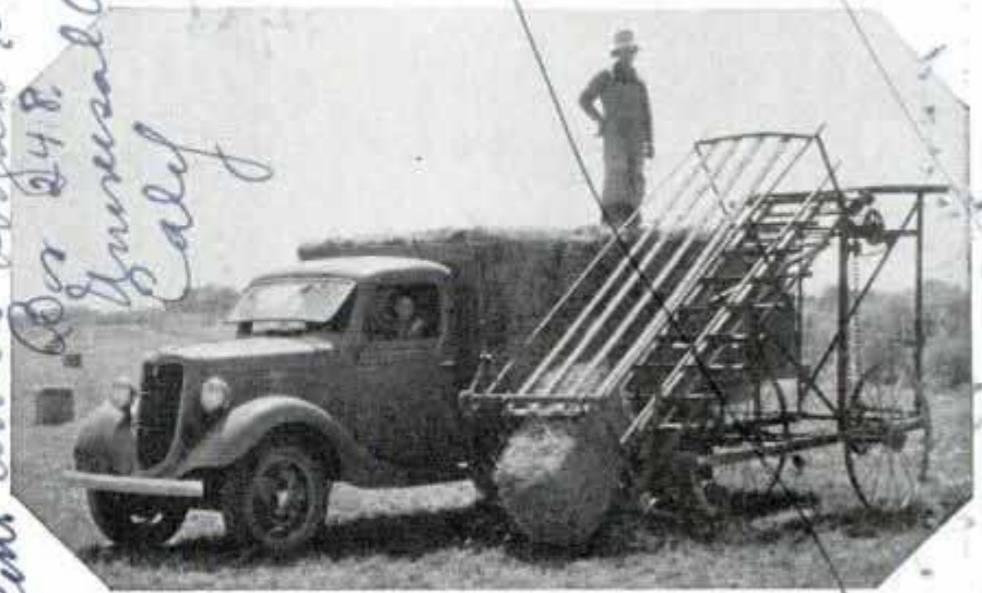
Homemade mechanical elevator takes place of pitchfork crew, hoisting bales of hay aboard farmer's truck
