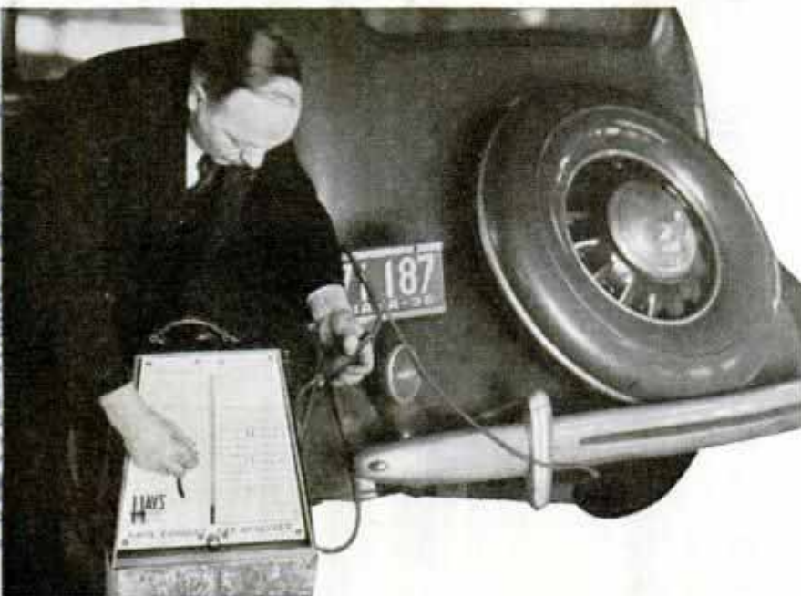
Taking a sample of gas from exhaust pipe of his car, the motorist can tell by reading the dial how efficiently his engine is operating
