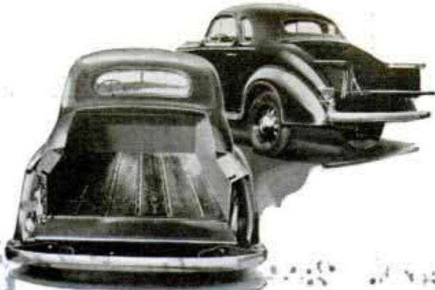
Two views of coupe with pickup body for carrying large load of small packages
