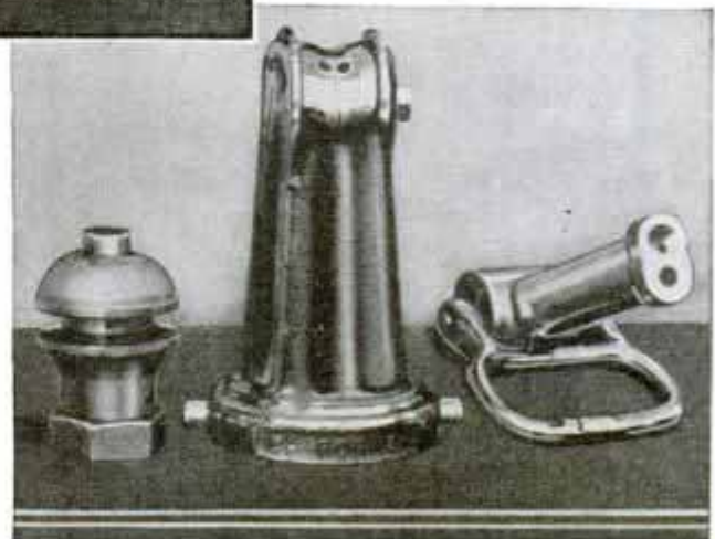
Types of fog nozzles, oil derrick equipped with fog nozzles, and spraying man-made fog
