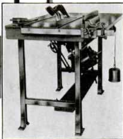
Two views of the worktable with counterbalanced power saw which can be tilted at any angle
