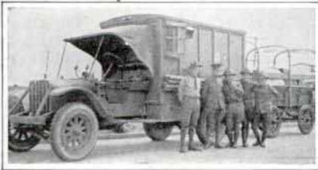
Army weather station on wheels. Radio-equipped truck carries meteorological instruments
