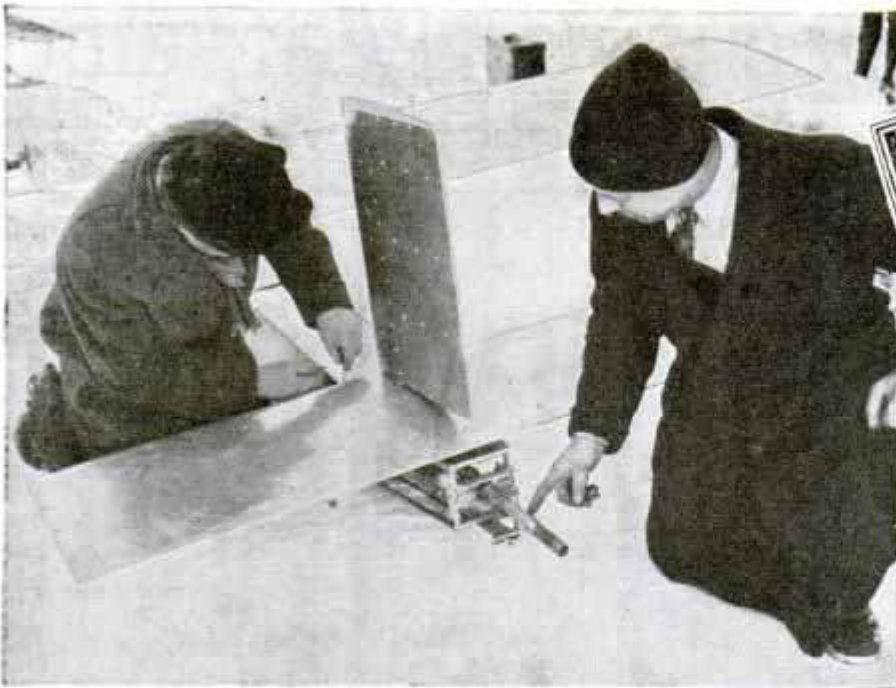
Left, powerful two-pound reaction motor of rocket mail plane. Above, rocket mail plane stamp. Below, how fuel tanks are stored in fuselage
