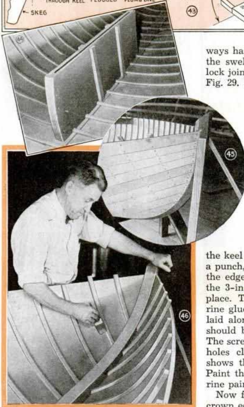
Two yokes and an upright brace at the forward end of the cockpit give rigid support to the mast step and the centerboard well. Position of step gives the mast a rake of \frac{3}{4} in. aft. Before the deck beams go on apply two coats of marine paint to the interior of the hull as in Fig. 46. Paint should be worked into corners at ribs and keelson
