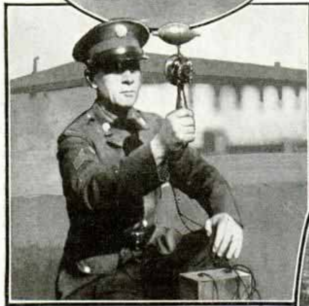
Left, instrument for measuring air current to show how gas will drift. Right, signal corps weathermen
