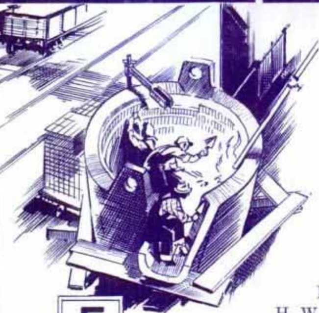
LEFT , the melter, the sentinel of steel, watching from his platform as an open hearth furnace is tapped and 150 tons of molten iron rushes into the ladle. Center , filling ingot molds with molten metal from a huge ladle which moves down the long row of molds. Right , fingers of a giant crane lifting a cherry-red ingot from the soaking pits. From here the ingot goes to the roll train and the "blooming mill" rolls it into a long slab.
