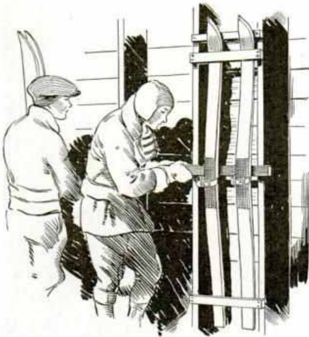
Adjustable crosspiece slips behind skis, springing them to shape to prevent warping
