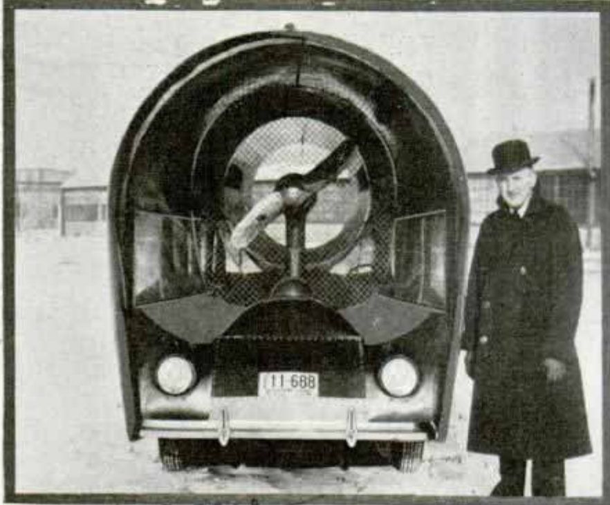
Side and front views of "vacuum rocket" car, showing the propeller that forces air back through the tube in the upper interior of the car
