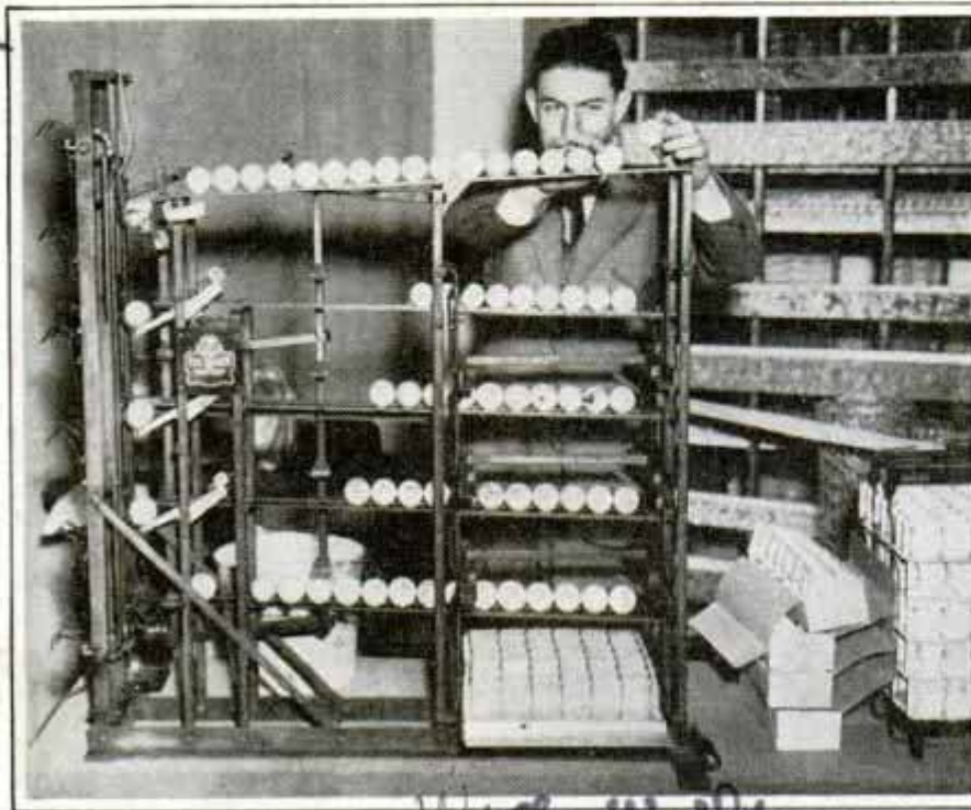
Selectors sort eggs as they ride down conveyor at left, dropping them off according to weight in one of four channels leading to cartons
