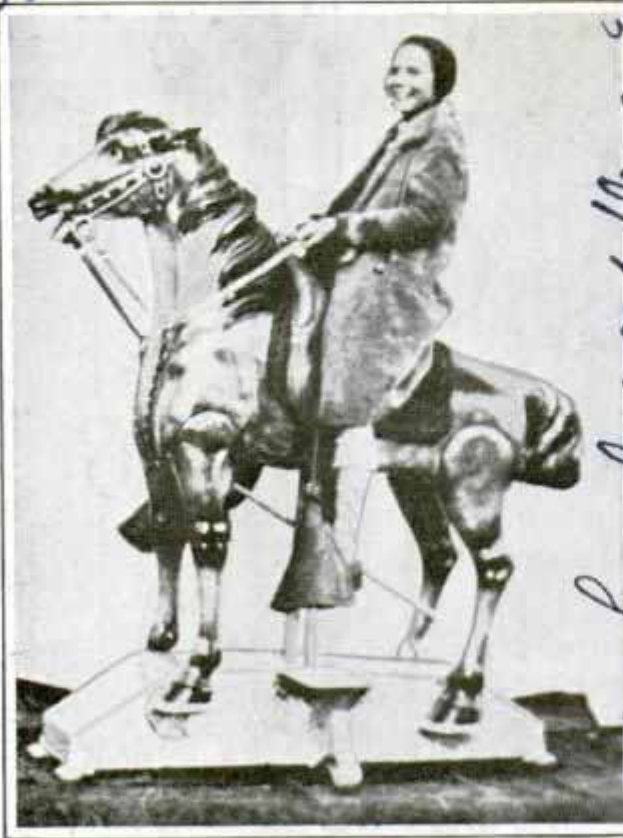
Electro-mechanical horse with five gaits ranging from a trot to a running gallop
