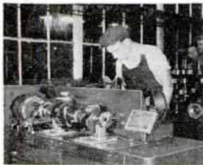
The completion of the Ford V-8 crankshaft is one of the longest tasks undertaken in building the V-8 engine. Every completed crankshaft is tested in this "dynamic balance tester."
