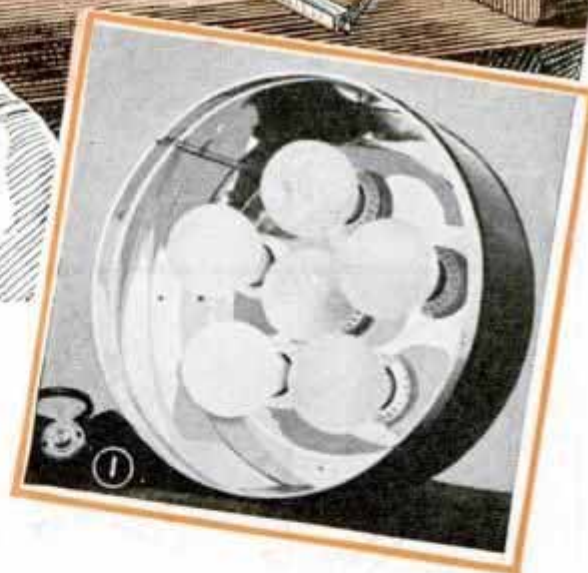
There's no need to buy an extra lens for this enlarger. Instead, you simply use the camera with which you took the picture
