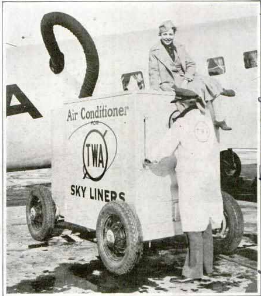
Photo snapped on cold day shows air conditioner supplying warm air for cabin of big transcontinental transport plane
