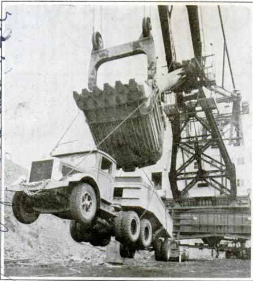
Tractor-trailer unit loaded with 50,000 pounds of coal being lifted and swung about with ease by the huge strip shovel
