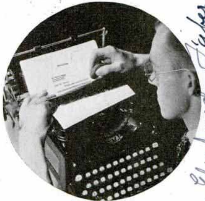
Type-cleaning "dough" removes excess carbon from lettering of typewritten copy to make neat erasures
