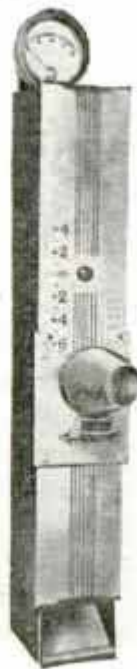
Testing headlights for brightness and focus with "electric eye"
