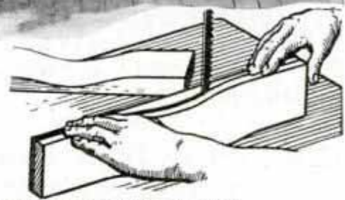
1 ST. OPERATION "BOW-CUT" MADE WITH BLOCK IN A VERTICAL POSITION
