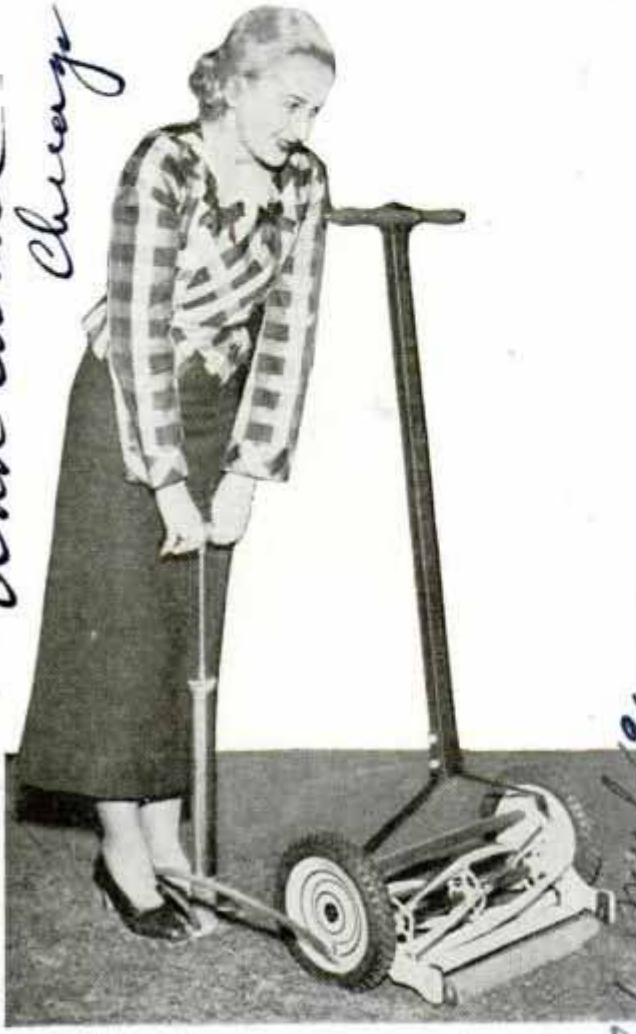
Low air pressure in the pneumatic rubber tires makes the lawn mower run more smoothly
