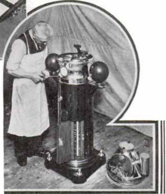
Stitching compass points on silk. Right, finishing shockproof pedestal for "Queen Mary's" compass
