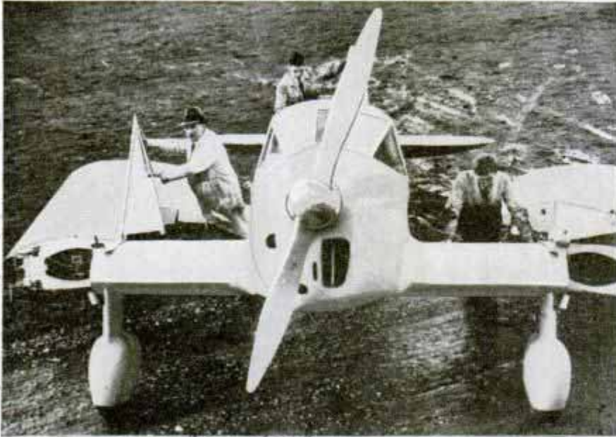
Demonstrating how hinged wings can be folded to permit housing the plane in ordinary garage. The ship cruises at 150 miles per hour
