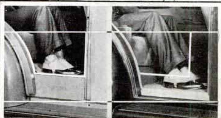
Left—"Low seat-high floor" that cramps legs, knees. Right—Plymouth's lower floor and chair-height seats... a more natural and more comfortable sitting position.
