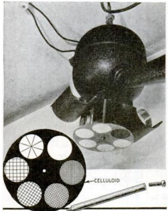
Any degree of light diffusion needed is selected by simply rotating the disk to the proper screen
