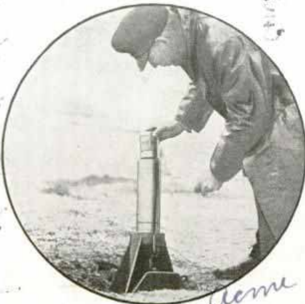
Firing smoke bomb from mortar at Croydon airdrome as signal to pilots flying above fog blanket
