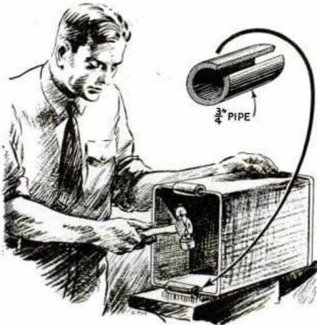
Pieces of pipe slit along one side and hammered over edges of cans, serve as finger grips
