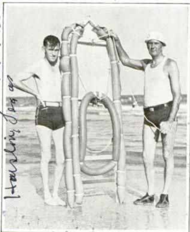
Wave-riding boat made of inner tubes attached to cypress framework with canvas strips
