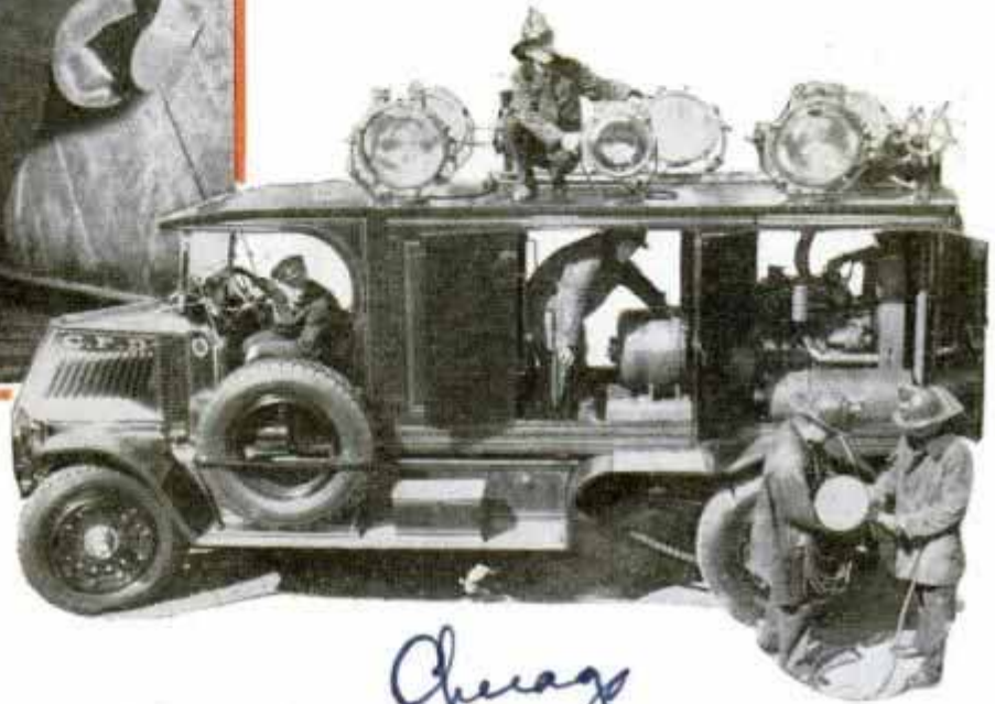
Firemen wearing oxygen masks and helmets insulated against electricity rescue victim overcome by smoke. Battery of floodlights at right guides squads at night fires
