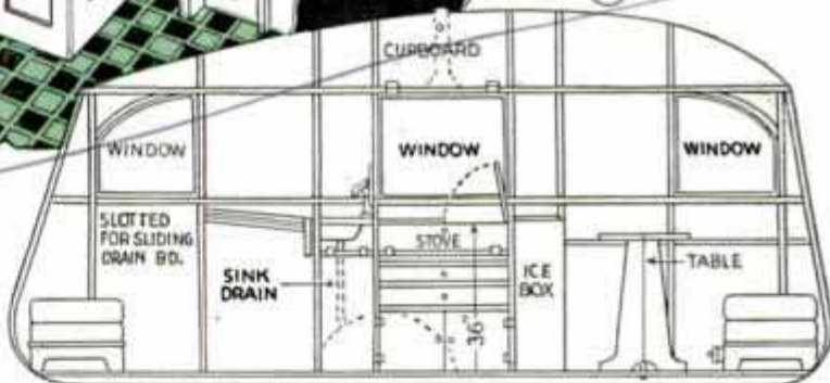
Above you have the "kitchen" equipment, a stove, sink, icebox and cabinet and also the dining table. At the right is a plan and elevation showing where to build in the cabinet. The lower cupboard houses the storage battery which furnishes current for the lights
