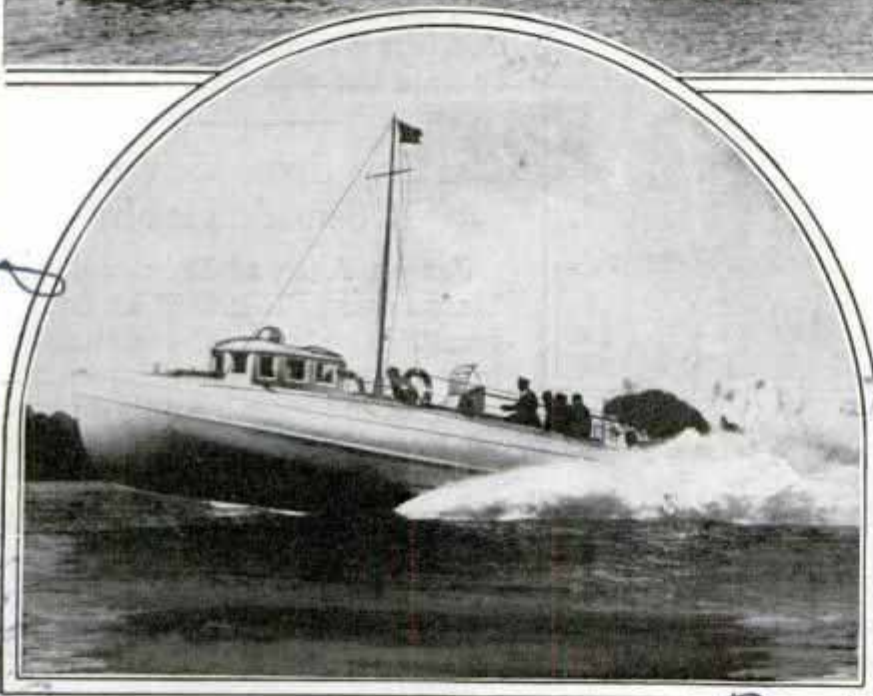
Top, one of Germany's "pocket battleships," a tiny cruiser with twin 550-horsepower gasoline motors. Left, another of the "mosquito fleet," secretly armed, doing forty miles an hour
