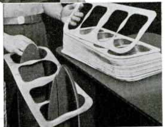
Partially completed Model A gasket showing how flange is curled over asbestos liner.
