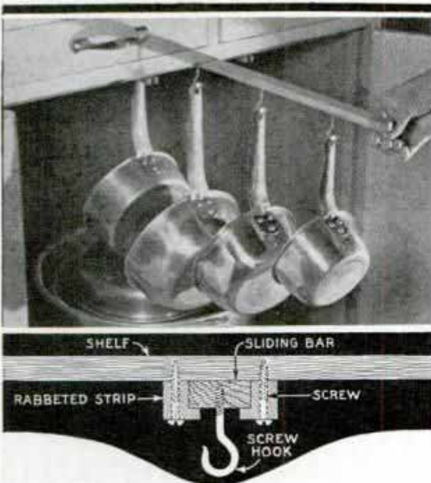
With this sliding arm on your cabinet you can reach utensils without getting down on your knees
