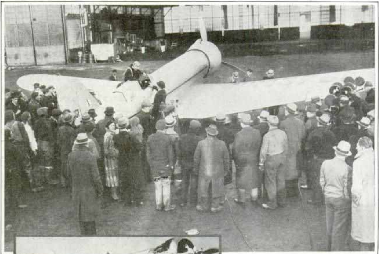
Two views of the slim, racy monoplane in which Howard Hughes set a new coast-to-coast speed record Northrop Airplane C an hour. The plane, a Northrop Gamma, with constant speed propeller, carried 700 gallons of fuel and had 100 to spare at the finish. The radial motor develops 925 horsepower at sea-level and a supercharger maintains high power at high altitudes.
