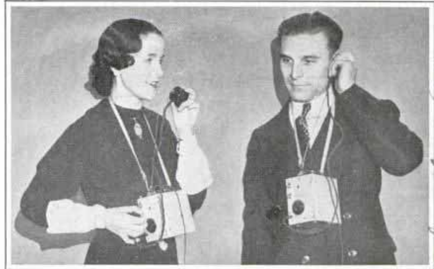
Mouthpiece doubles as receiver for this tiny two-way radio set. Battery and all, compactly boxed, weigh only three pounds
