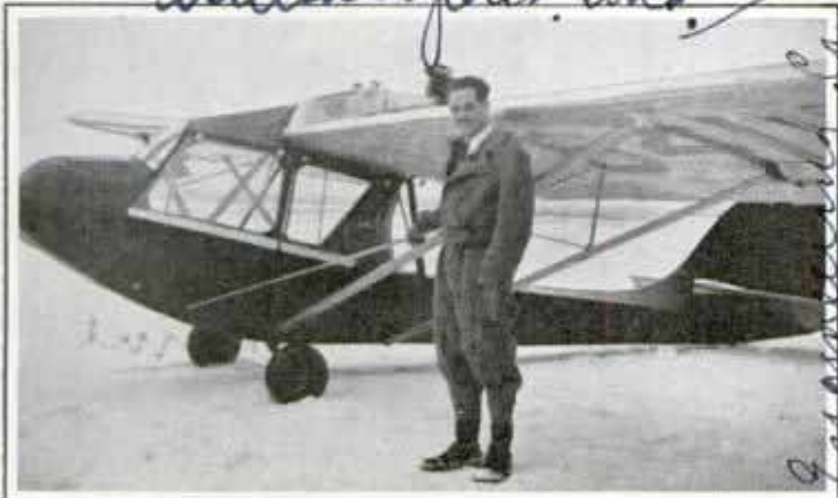
Enclosure is shown in place around cockpit, making this plane an all-weather craft. Vision is not obstructed
