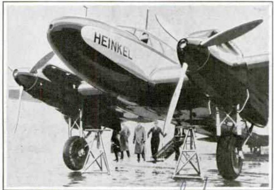
Twin-engine transport plane developed in Germany. It carries ten passengers and makes a speed of 250 miles per hour
