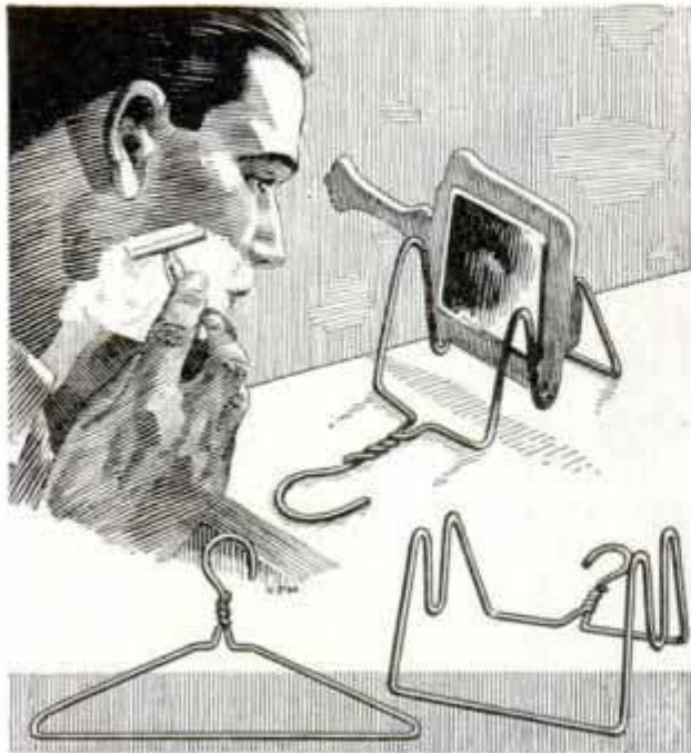
This holder leaves both hands free when shaving or dressing in front of a small mirror
