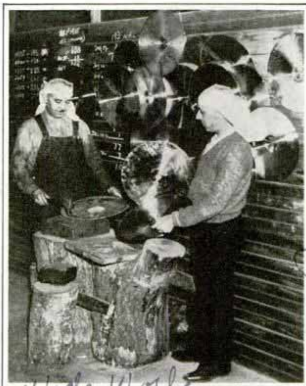
One corner of foundry where cymbals are tempered carefully to obtain tone purity
