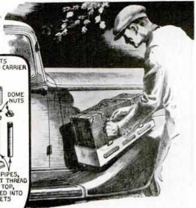
Here's a carrier for that extra suitcase. There's nothing to rattle and no part of carrier or luggage can touch the car finish
