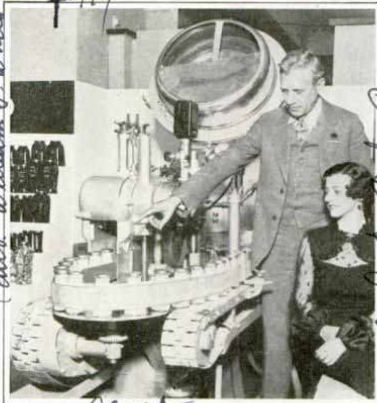
Capping machine as it applied metal sealer to bottles for keeping milk fresh over long periods
