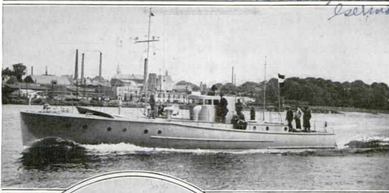
Top, one of Germany's "pocket battleships," a tiny cruiser with twin 550-horsepower gasoline motors. Left, another of the "mosquito fleet," secretly armed, doing forty miles an hour
