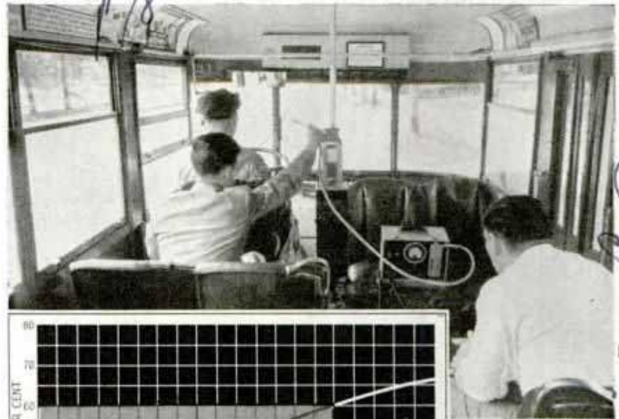
Continuous carbon monoxide detector installed in car and chart showing carbon monoxide concentrations which will cause headache, unconsciousness and death
