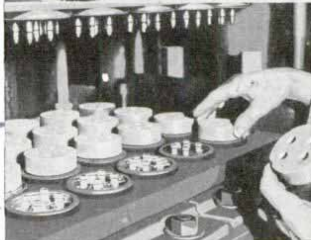
© Ewing Galloway Soy bean "soup" and some automobile parts, including distributor terminal plates, fabricated from it
