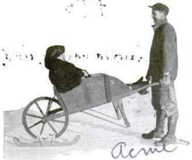
Fastening runner rigidly to the wheel converts wheelbarrow for year-round use
