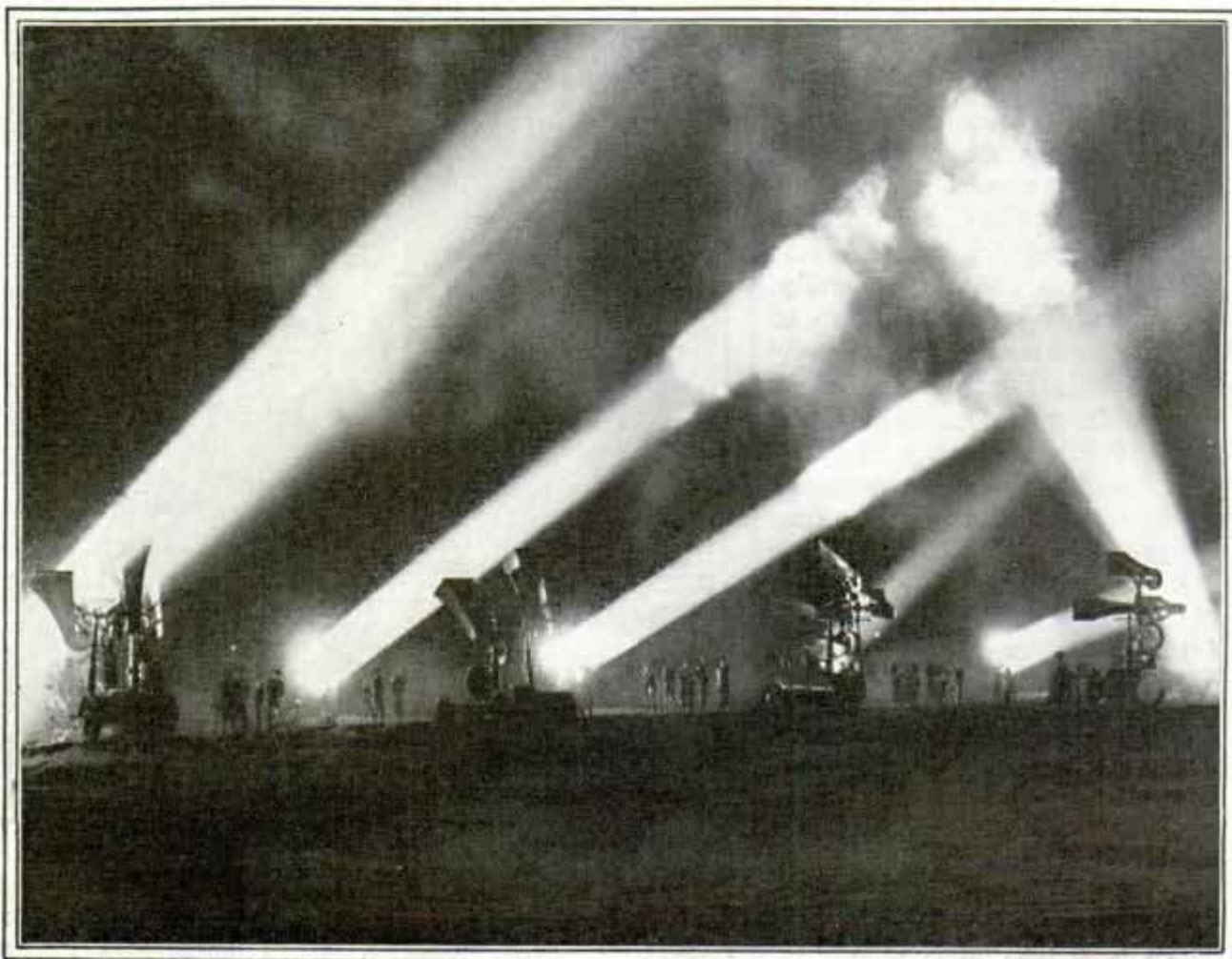
U. S. army searchlights throwing 100-mile beam. In front of lights are sound detectors which pick up whir of airplane propeller and enable the soldiers to turn beam on "enemy" aircraft
