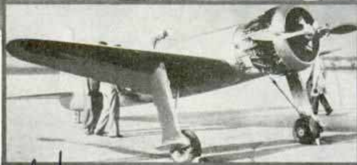
Two views of the slim, racy monoplane in which Howard Hughes set a new coast-to-coast speed record Northrop Airplane C an hour. The plane, a Northrop Gamma, with constant speed propeller, carried 700 gallons of fuel and had 100 to spare at the finish. The radial motor develops 925 horsepower at sea-level and a supercharger maintains high power at high altitudes.
