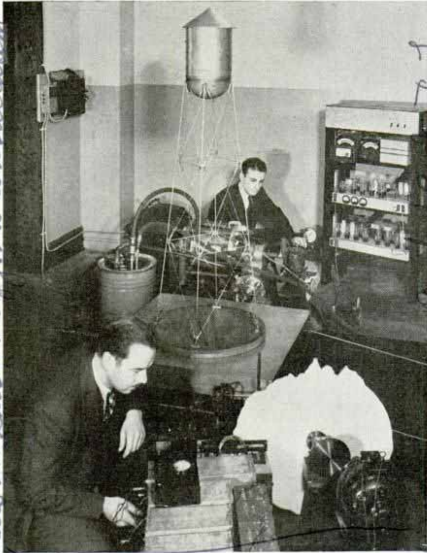
White outline in foreground is shadowgraph of quake. Tank on table is shaken as equipment converts shadowgraph lines into motion
