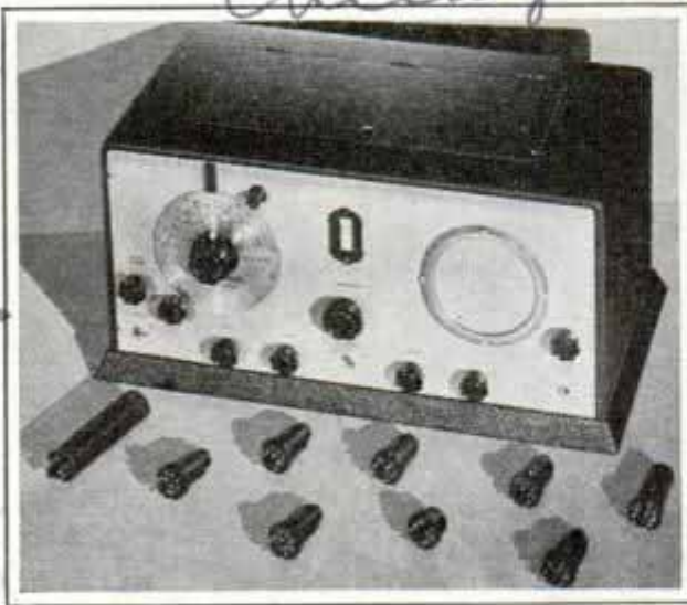
Five-band superheterodyne with vernier band-spread dial, built-in speaker and nine metal tubes
