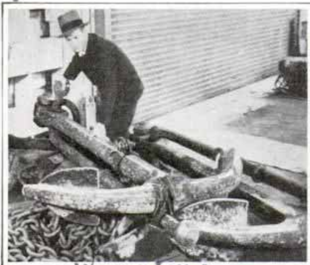
Modern air liners will be "hitched" to these old anchors which were discarded after long service on ocean-going boats
