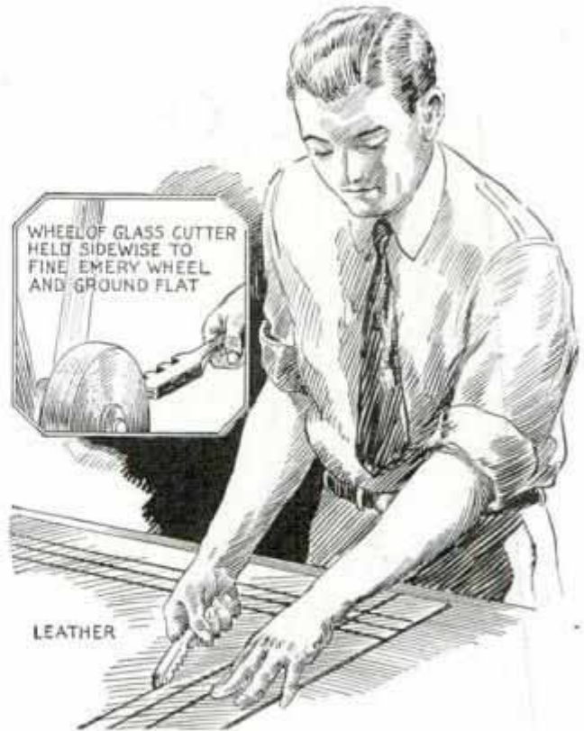
Glass cutter with edge of wheel flattened on grinder, tools borders on leather
