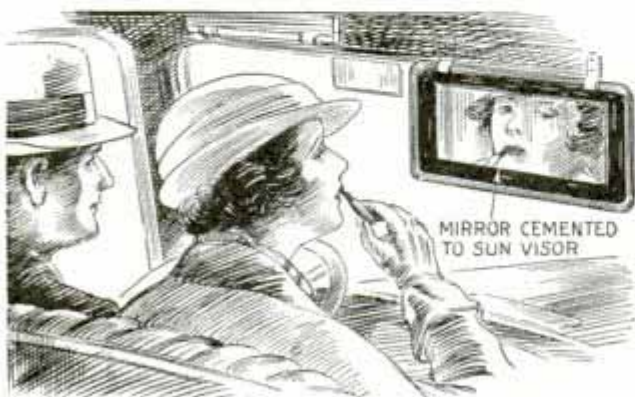
Adjusting visor as in shielding the eyes brings mirror at a convenient height for use
