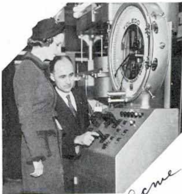
acme Demonstrating remote-control board. Weight recorded on scales is transmitted over wires
