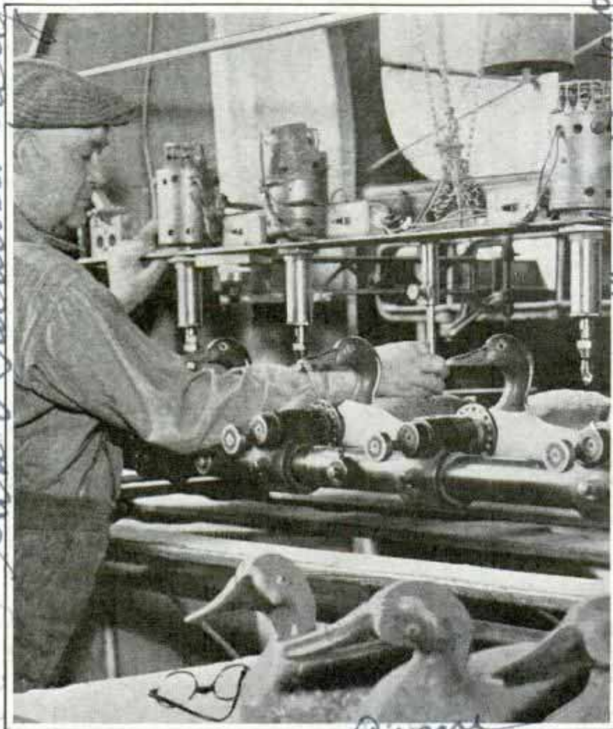
Using one bird at center as "master," Frank Mackay fashions several duck decoys from same model in his workshop
