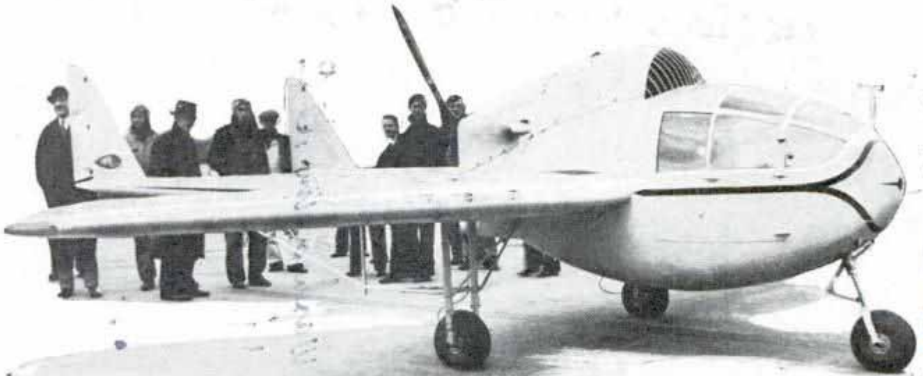
Designed for the private flyer, this two-passenger monoplane has its engine mounted high at the rear of the cabin, thus subduing noise and giving the pilot the maximum visibility
