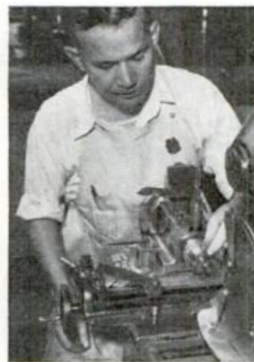
Checking spacing of spline gage with a combination of 3 Johansson Gage Blocks.
