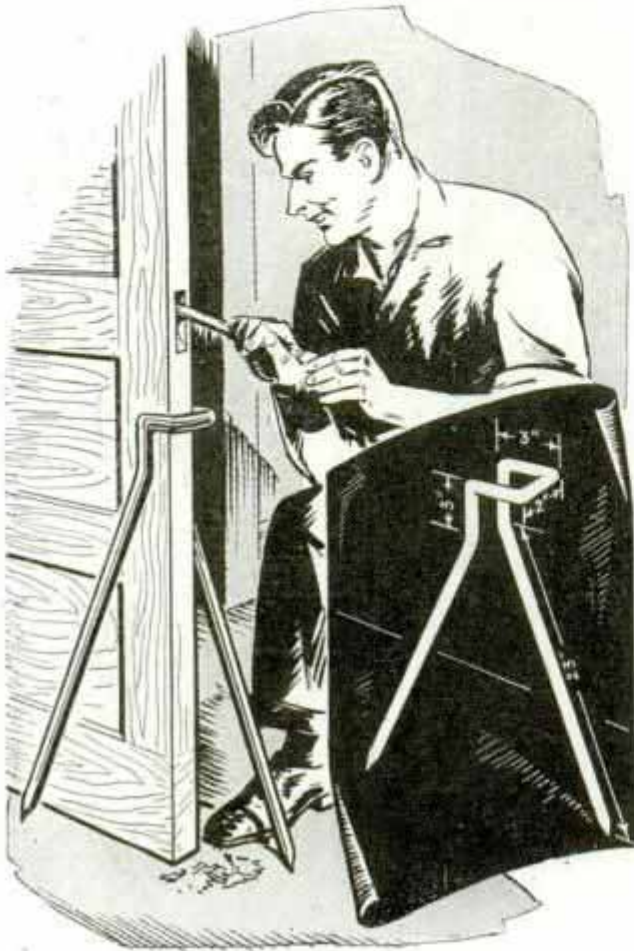
The jig is made of \frac{1}{2} -in. iron rod and the ends are pointed on a grinding wheel
