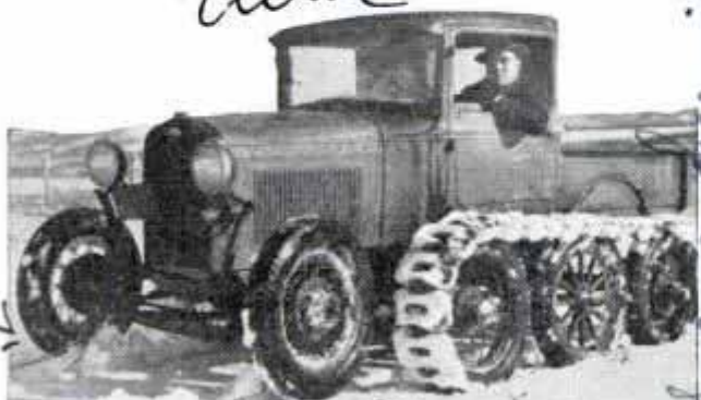
Extra rear wheels and flexible track enable this car to conquer deep snowdrifts
