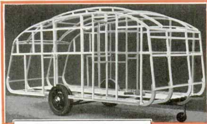
Provision is made in the framing for building in a sink and a compartment for a gas stove, also storage cabinets for clothing, food and cooking utensils
