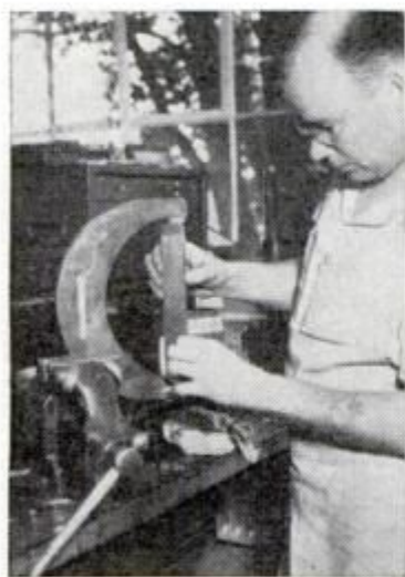
Verifying the accuracy of a "go" and "no go" snap gage.
