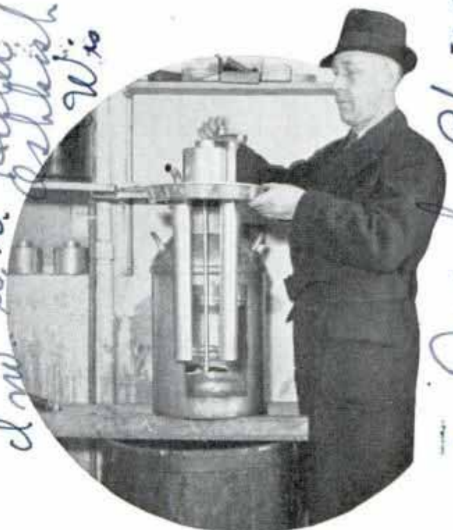
Cooler is inserted in can and water flows through tubes while agitator keeps milk circulating
