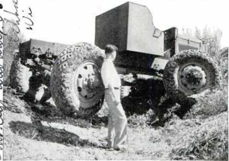
Even with one wheel in the air, power is delivered to three other wheels and with front and rear steering the truck can maneuver out of trouble
