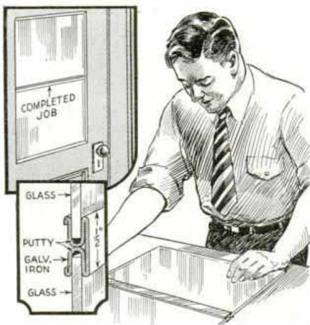
Putty between the glass edges and the metal strip makes the joint rain and wind proof
