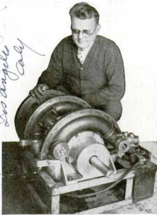
Pistons Describe a Semi-Circular Stroke in Curved Cylinders of This New Type Motor
