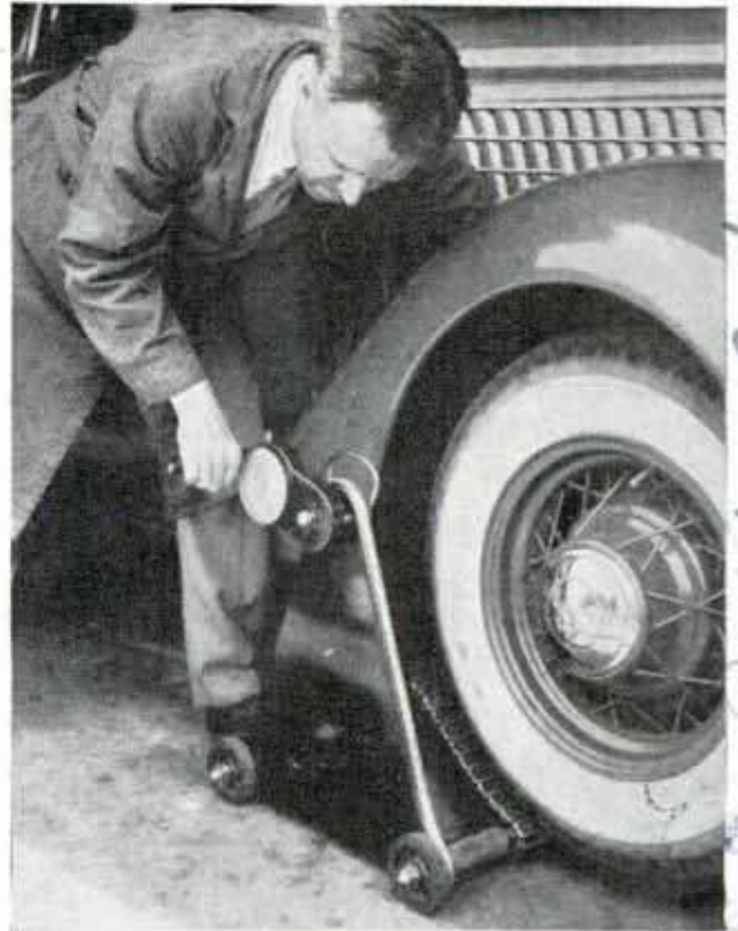
Handy Equipment for Equalizing Brakes Is Operated Easily by One Man
