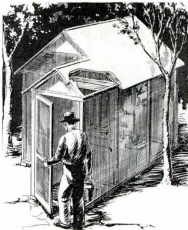
Both Doors Should Be Fitted with Coil Springs and Also with Hooks on the Inside
