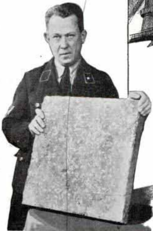
Block of Inexpensive Building Material Made from Berlin's Waste and Rubbish and Suitable for Partitions
