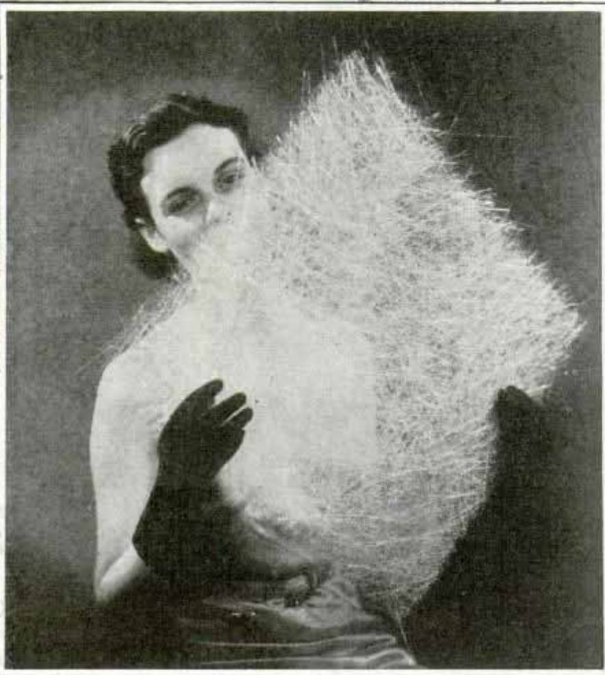
Section of Glass Wool from Which Yarn Is Woven; Cloth Made of This Yarn Has Remarkable Wearing Qualities
