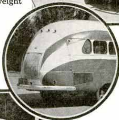
Back and Side Views of Light-weight Streamline Motor Coach Showing Engine Mounted at Rear, Easily Accessible When "Wings" Are Opened
