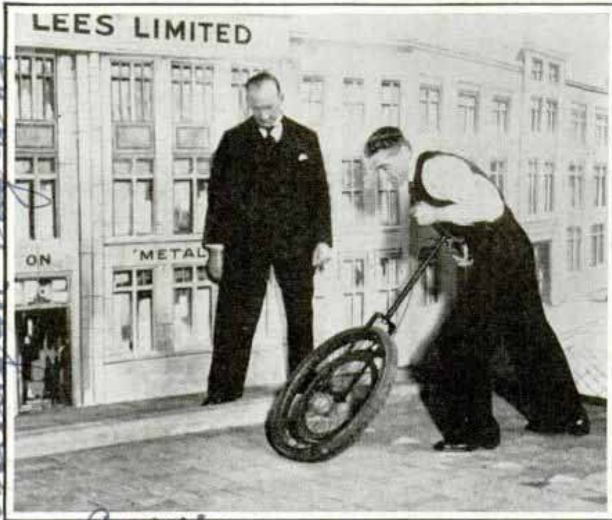
Testing Skidproof Metal Paving in England by Attempting to Push a Rubber-Tired Wheel Across It at Right Angles
