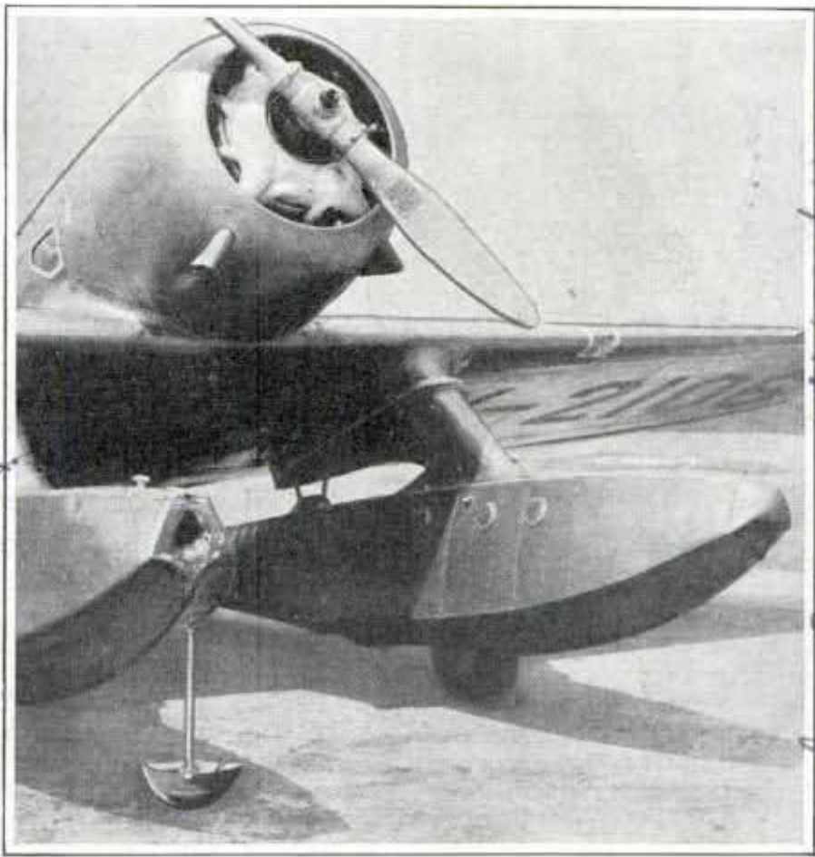
Stem of This Mushroom-Like Anchor Is Withdrawn into Nose of Pontoon When This Speed Champion of Amphibians Is Ready to Take Off
