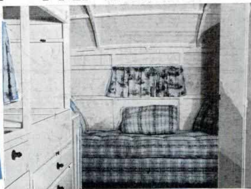
For Sleeping Quarters That Will Accommodate Four Persons, a Luxurious Studio Couch Is Placed at Each End; the Aluminum-Painted Top Reflects Heat, Keeping the Interior Cool; for Added Insulation, the Walls and Top May Be Made Double
