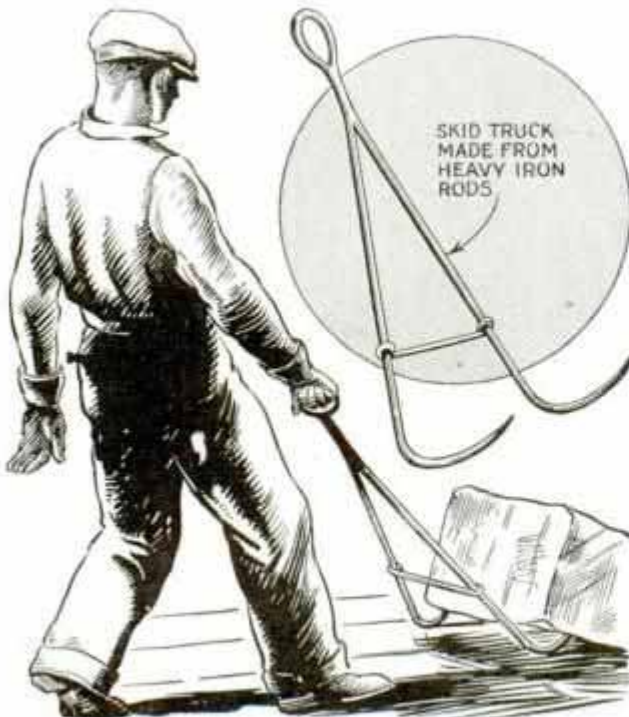
This Skid Saves Time When Ice Cakes Are Moved About on a Platform or Up a Gangplank
