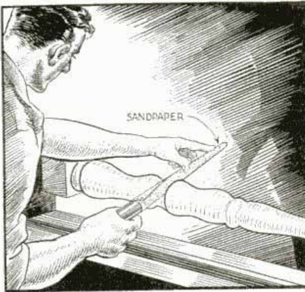
Stick Covered with Sandpaper Gets into Grooves of Turnings That Can't Be Sanded in the Regular Way
