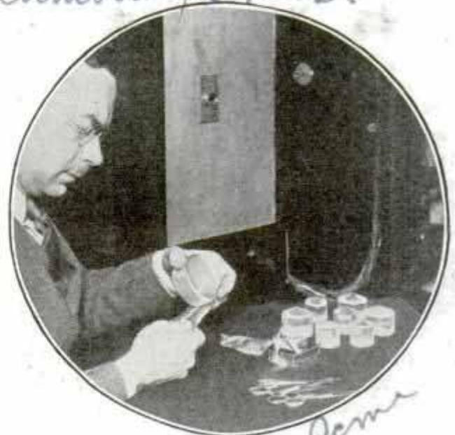
Removing Three-Inch Lithium Fluoride Crystal from Thin Platinum Crucible in Which It Was "Grown"
