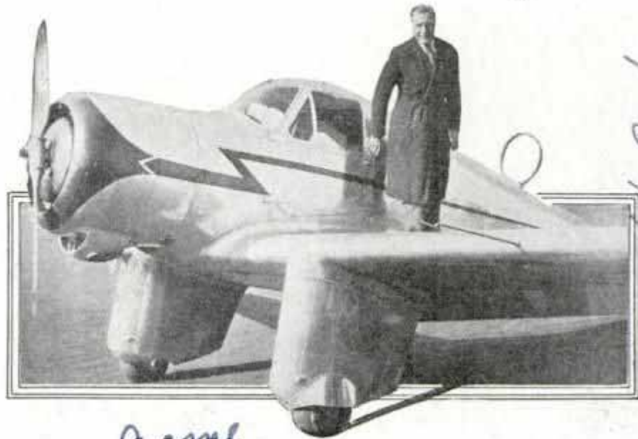
Acme Two-Place, Low-Wing, All-Metal "Flivver" Plane Which Makes a Speed of 131 Miles per Hour with a Ninety-Horsepower Motor
