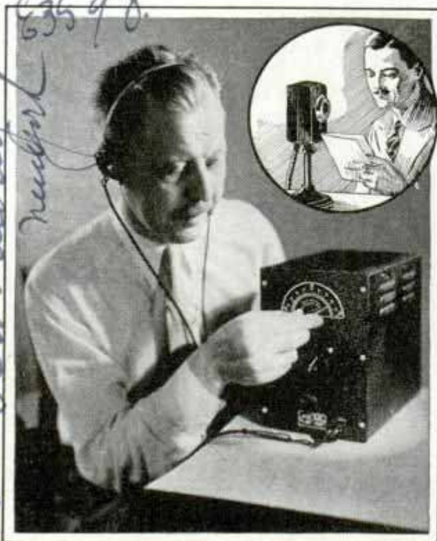
Amateur Phone Monitor Showing Tuning Dial and Band-Changing Switch Mounted on Front Panel
