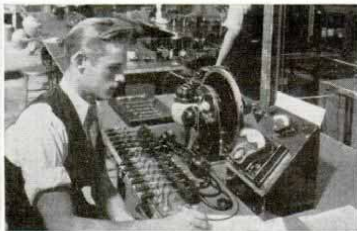
This specially designed equipment tests ignition units under conditions met in actual service.
