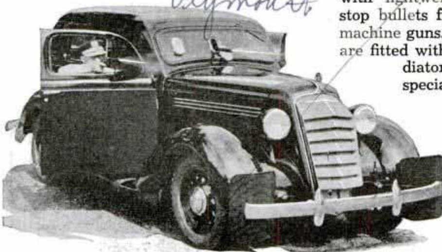
Firing from Armored Plymouth; Note Tire Guards and Radiator Shield; This Car Is Built Especially for Use of Police against Criminals
