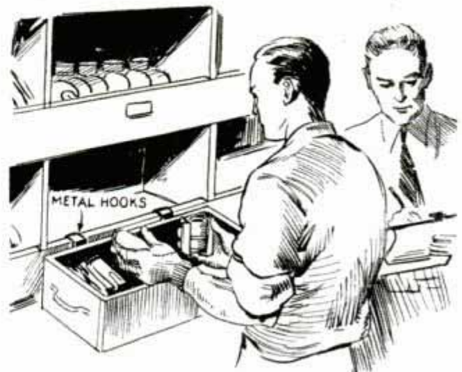
Invoicing Contents of Stock Bin Is Done Quickly by Hooking Supply Boxes on Sides of Bin
