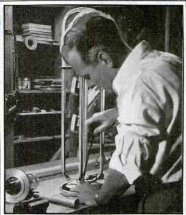
After Cutting and Bending the Parts, Assembly Is a Simple Matter; Below, Edging for Base Is Bent to Right Curvature and Hammered over at Right Angles in Form
