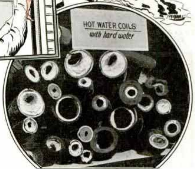
Proper Care of the Heating System Would Have Doubled the Life of These "Limed-Up" Pipes
