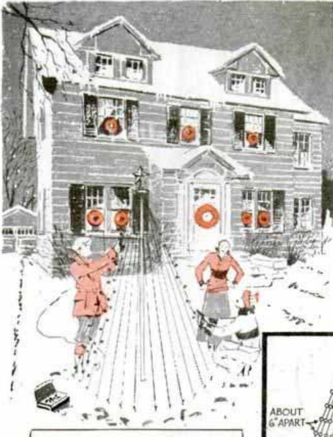
This Imitation Christmas Tree Is Made with Strings of Lights Fastened to a Center Support Pole and Staked to the Ground in a Circle
