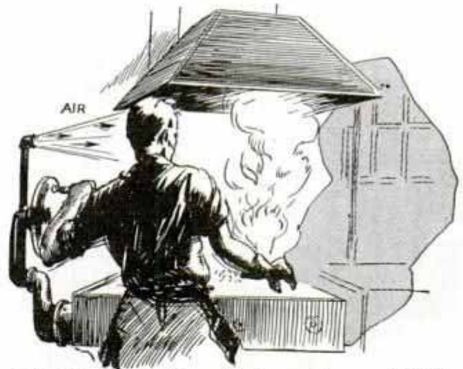
Thin Sheet of Air Forced between Forge and Worker Protects His Face against Intense Heat
