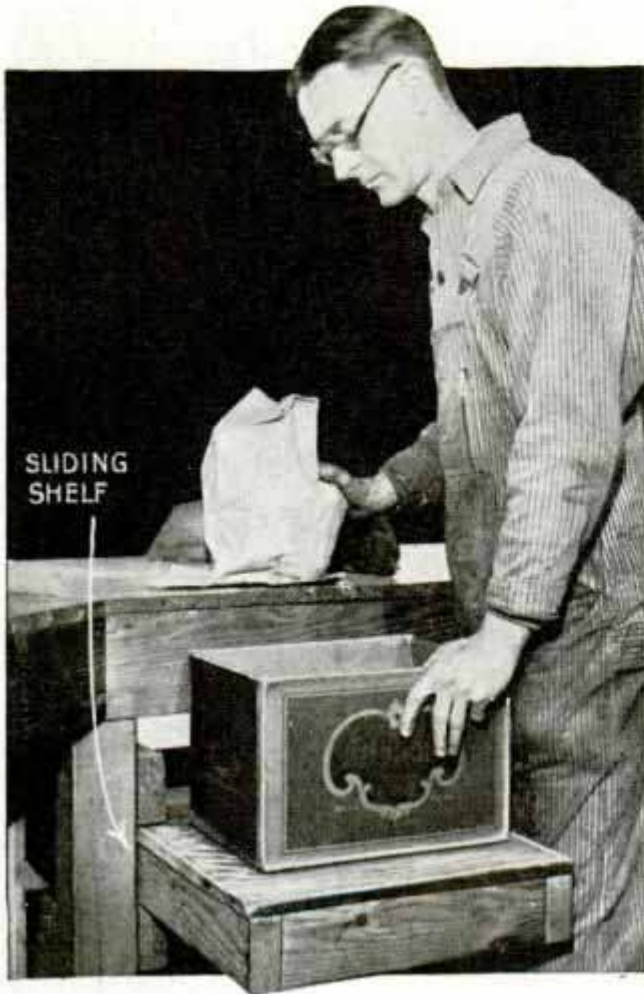
Stooping or Lifting of Heavy Boxes Is Unnecessary When Packer Uses Shelf on His Work Table
