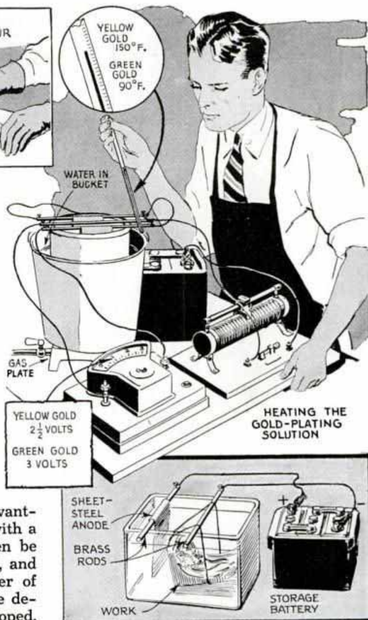
Above, While Gold-Plating, the Solutions Are Kept at Uniform Temperatures in a Water Bath; Below, After Work to Be Silver-Plated Is "Blue-Dipped," It Is Placed in This Silver "Strike" Solution
