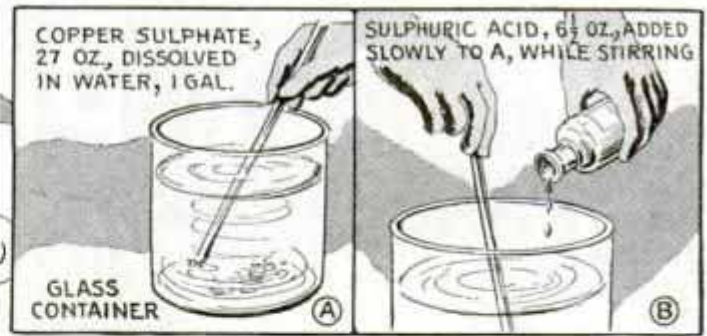
Copperplating Solution Is Made by Mixing Copper Sulphate in Water and Then Adding Sulphuric Acid
