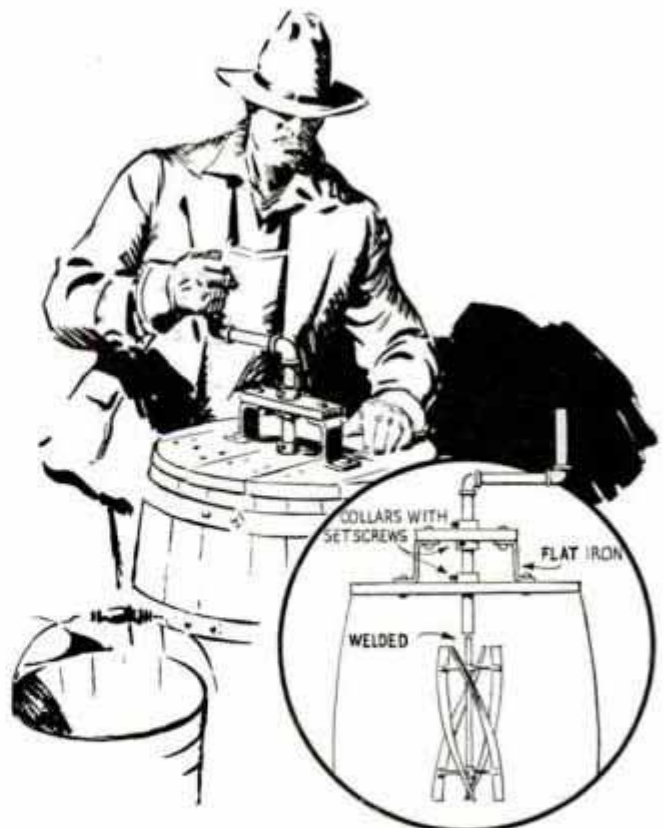
Suspended Vertically from the Lid of a Mash Barrel, the Mixer Is Turned with a Crank Made of Pipe
