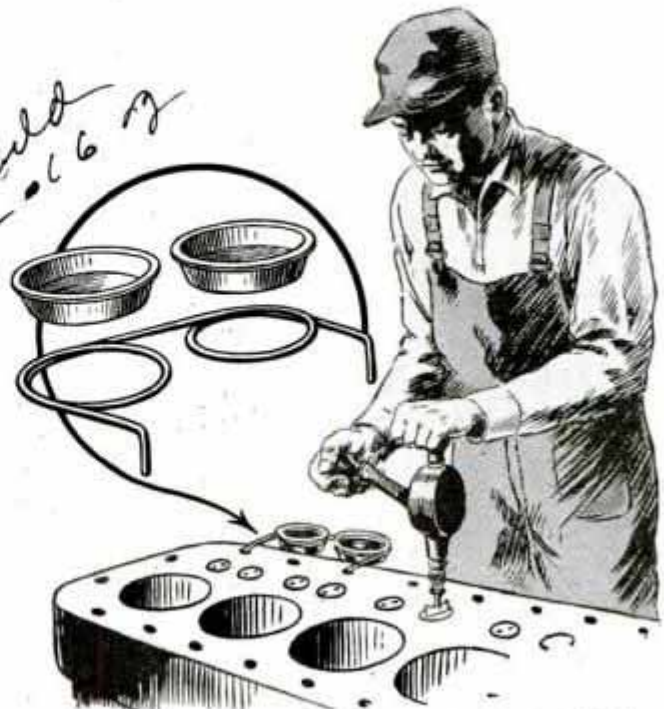
Ends of Wire Holder Hook into Holes in Block Next to Workman When Grinding Valves
