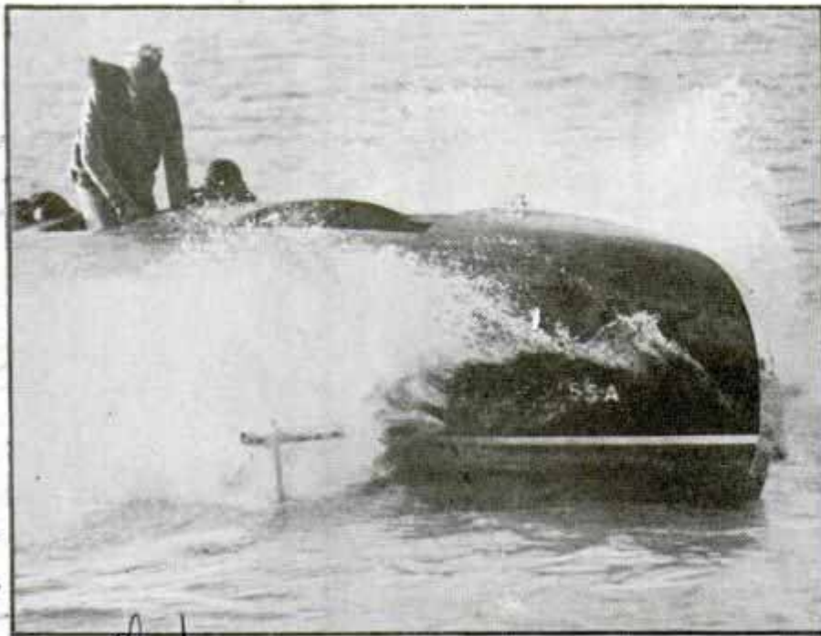
dent. "Miss U. S. III" Sends Spray Flying on Test Speed Run; Notice Plane-Like Hull Design and Outrigger Support for Wings in Water
