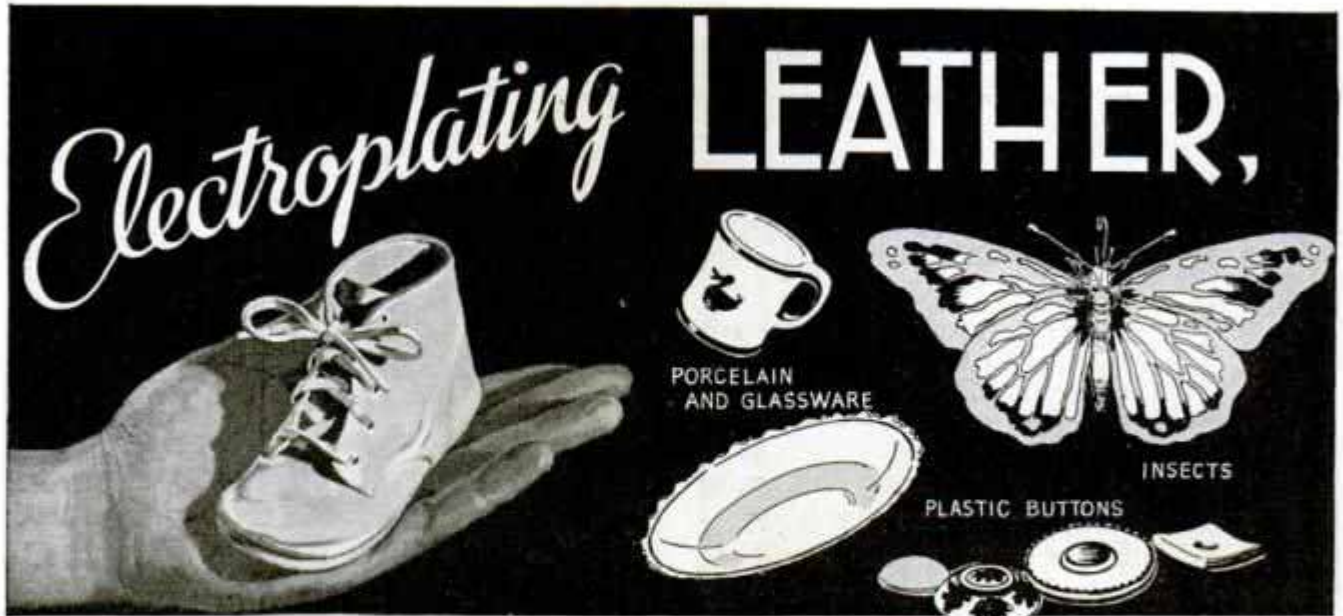
Leather, Plastics and Other Close-Grained Materials, Are Washed in Alcohol, Coated with Lacquer, Then Dusted with Graphite or Copper Powder, After Which Electroplating Is a Simple Process
