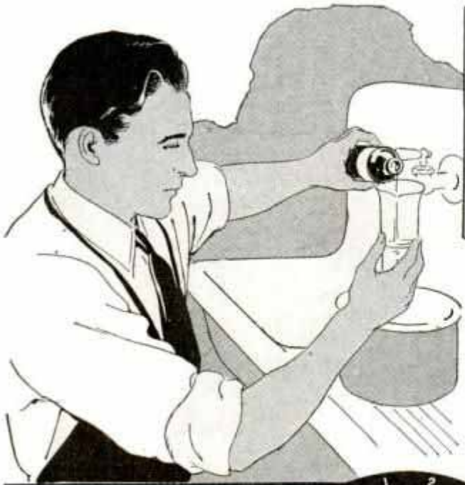
Copperplating Solution Is Made by Mixing Copper Sulphate in Water and Then Adding Sulphuric Acid
