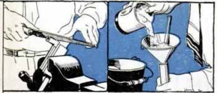
Right, Pouring Sand into Plugged Tubing before Bending; Left, Filing Ends to Fit in Joining Sleeve
