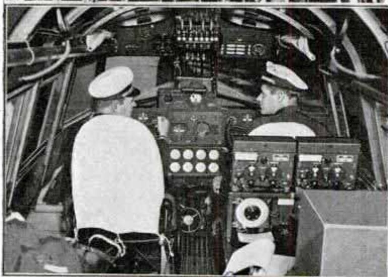
Control Cabin and an Exterior View of the "China Clipper," 51,000-Pound Luxury Liner Intended for Transpacific Service; Its Four Motors Develop 3,200 Horsepower
