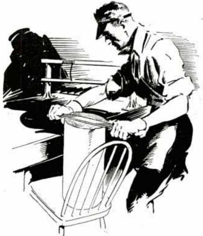
Wrapping Paper Will Not Tear Ragged along the Edges if Ends of Roll Are Roughened with File
