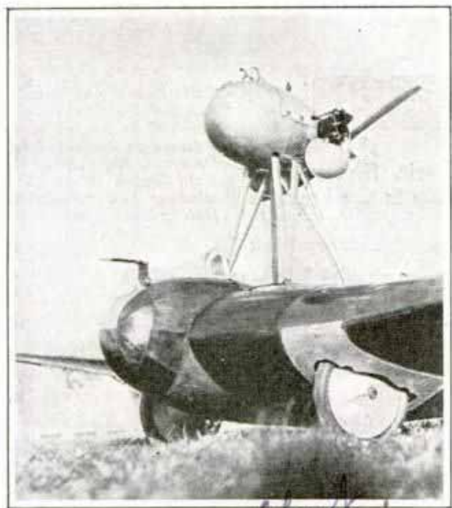
Tailless Glider Plane Equipped with an Outrigger Engine and Pusher Propeller
