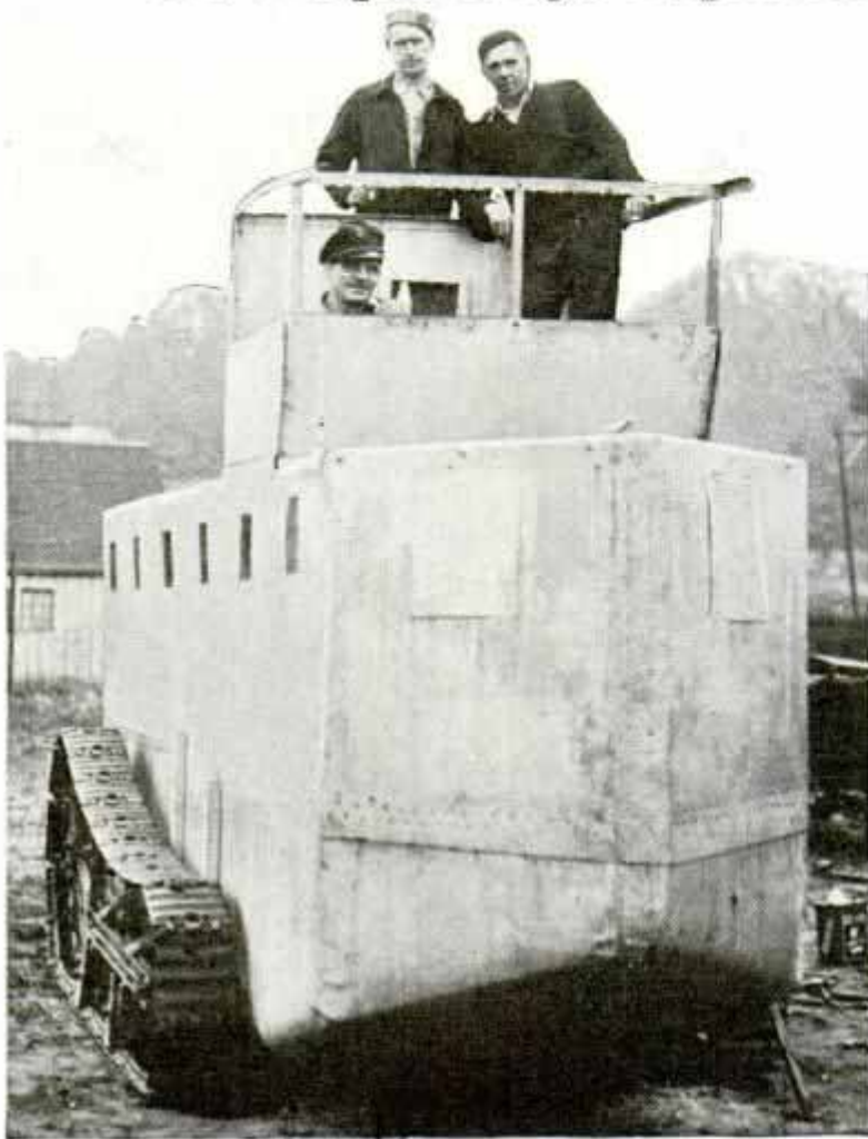
On Shore This Is a Tractor Able to Travel over Rough Terrain; Afloat It Is a Propeller-Driven, Steel-Armored Houseboat
