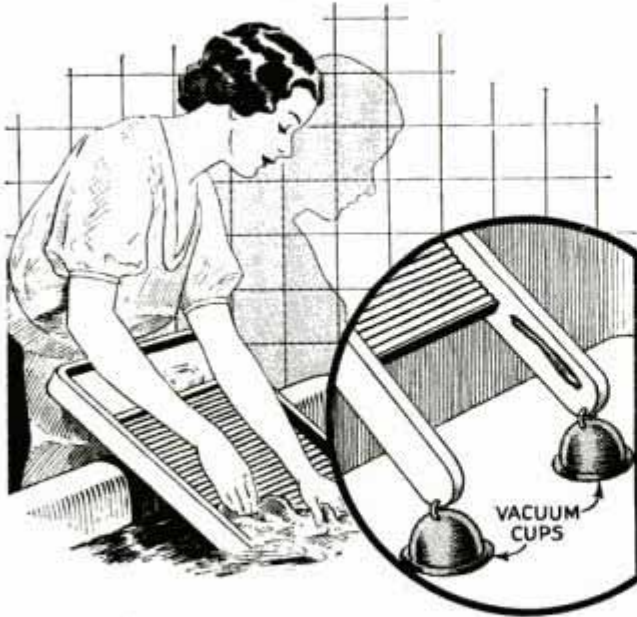
Large Vacuum Cups Attached to Legs of Washboard Keep It from Slipping in Tub
