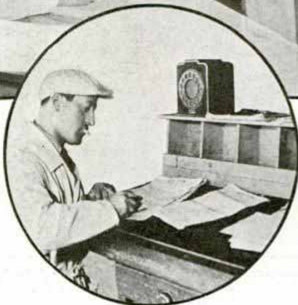
Top, Giving Orders from Office by Turning on Transmitter; Bottom, Voice Is Amplified in Shipping Room
