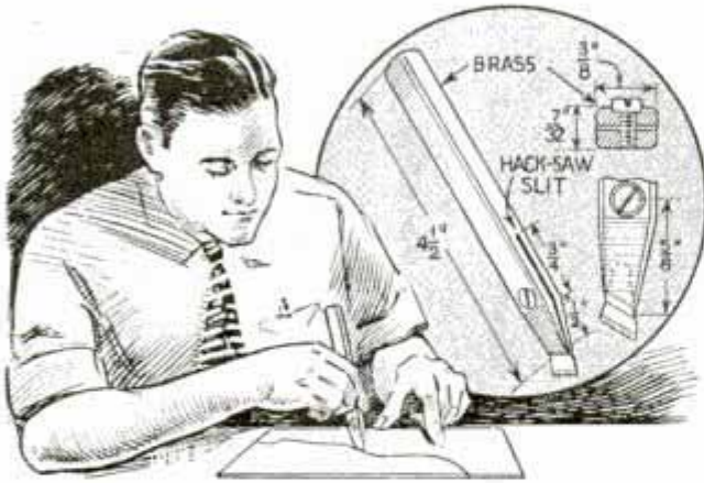
Carving Tool Uses Razor Blades, Which Are Shaped to Suit the Work at Hand
