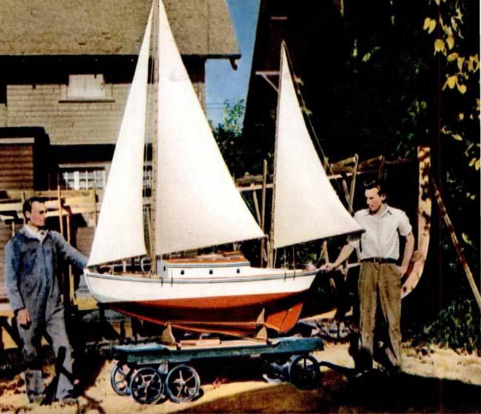
BOAT builders testing sail balance and ballast placing on a scale model before spending thousands of dollars to build a full size craft.
