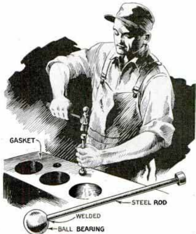
Large Ball Bearing Welded to End of Steel Rod Makes Efficient Tool to Cut Gaskets
