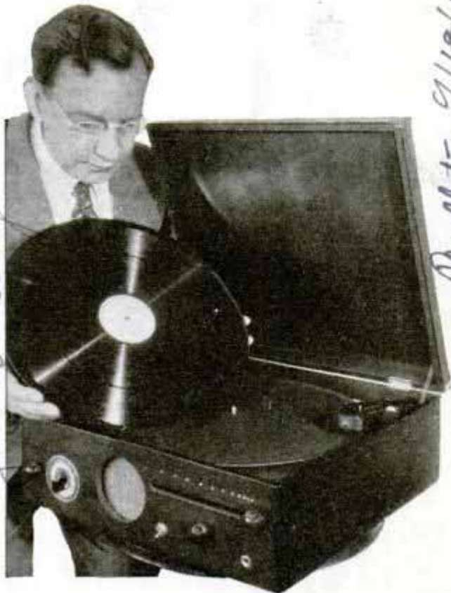
Portable Case Contains Radio and Phonograph Which Plays Wide-Diameter Records for the Blind
