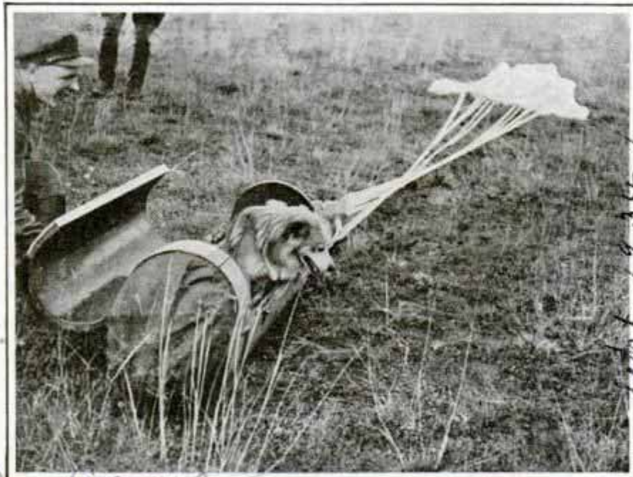
Cylinder Attached to Parachute Is Dropped from Plane and Springs Open on Striking Land, Releasing Dog Trained to Perform Task
