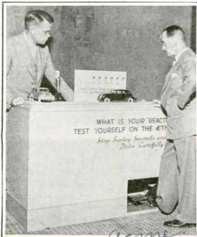
Sir Malcolm Campbell Taking Test Which Indicates Time Required for Driver to Apply Brake
