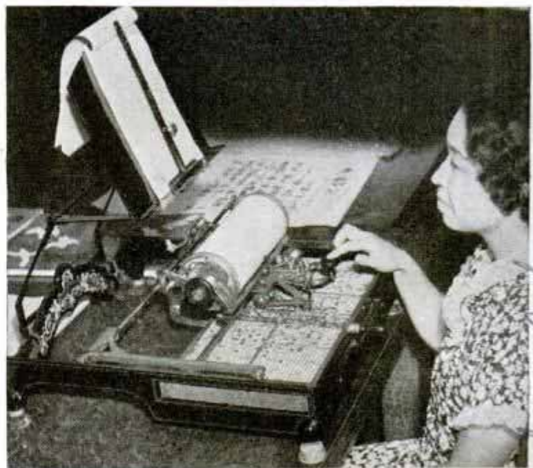
Moving Selector over Case Holding Two Thousand Japanese Characters, Typist Presses Knob to Ink and Prints Type Slug
