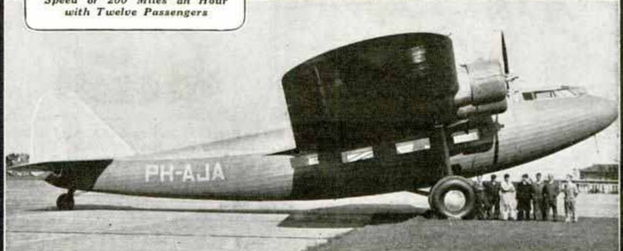
Above, Huge Fokker Passenger Monoplane Equipped with Four 600-Horsepower Radial Air-Cooled Engines; It Flies Three Miles a Minute; Below, Combat Monoplane of French Air Corps Which Does 250 Miles an Hour at Altitude of Three Miles
