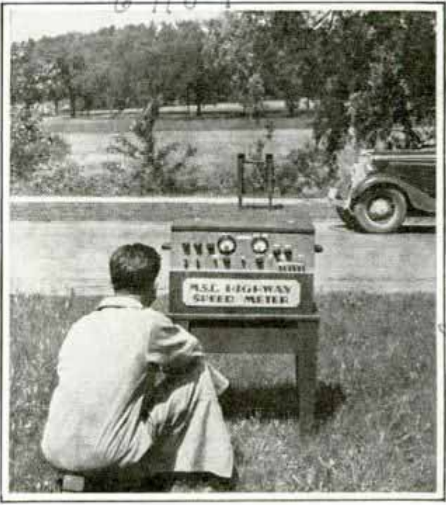
Speed Meter Which Utilizes the Electric Eye to Check the Speed of Passing Cars
