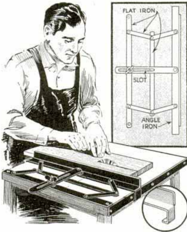
This Strong Saw Fence Is Easily Attached and Can Be Made in Any Size Desired
