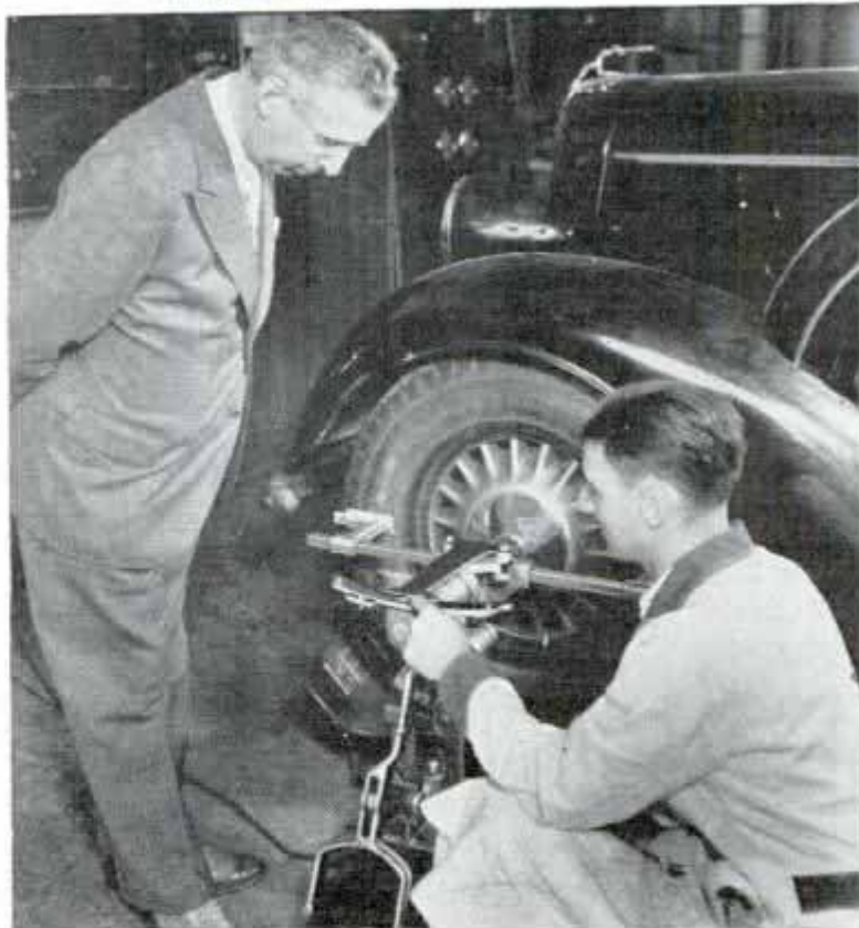
Top, Illustration of Shimmy; Bottom, Showing Car Owner How Simple Are Examination and Correction of Front-End Trouble; This Equipment Indicates Maladjustment; Pointer Shows Degree from Normal (Photo Courtesy Northmoor Motor Co.)
