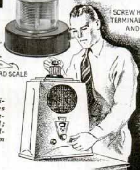
Left, Homemade Wing Nut; Upper Hole Is Drilled First, Tab Is Bent Under and Second Hole Drilled, Using First as a Guide, Then Tapped; Right, Overloaded R.F. or Rectifier Tubes May Be Drilled and Base Filled with Oil to Prevent Arcing
