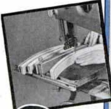
THE PANEL GROOVES ARE RUN IN WITH A ROUTER BIT ON THE DRILL PRESS
