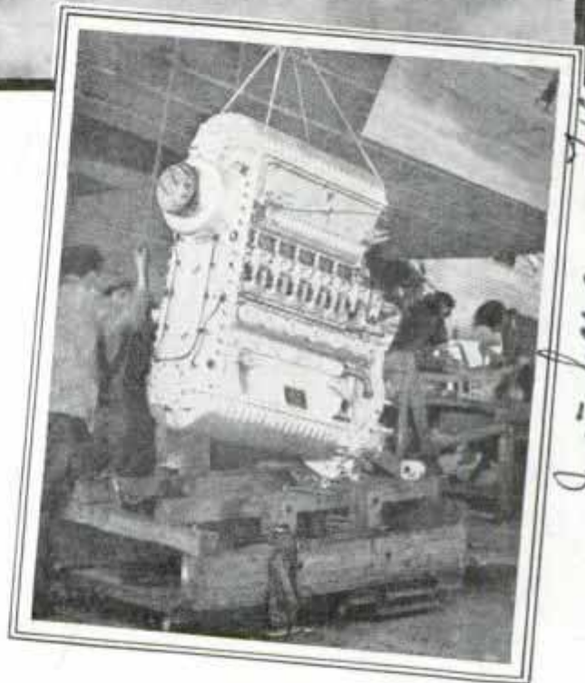
Top, Diesel-Powered German Plane in Flight; Bottom, Hoisting Diesel Unit Aboard the "Hindenburg"
