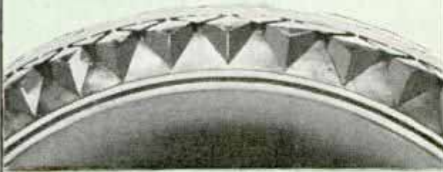
Mild Case of Heel and Toe Wear. To correct use Method A
