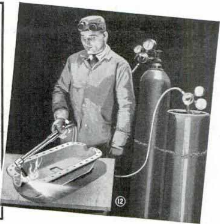
The Torch Has Many Uses in the Average Garage; Broken Parts That Are Difficult to Get for Old Cars, May Be Welded Together in a Short Time
