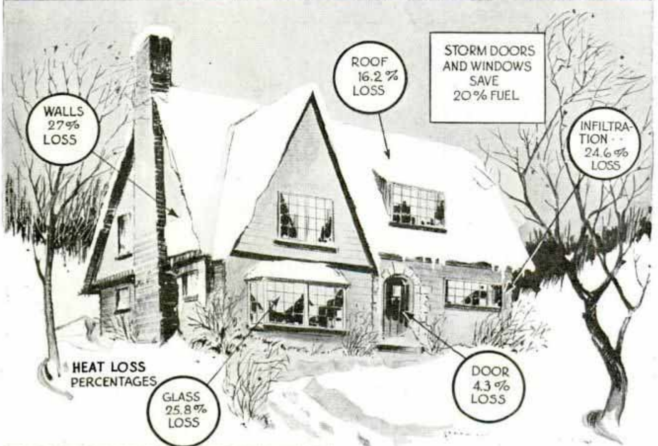
Top, Proportion of Heat Losses in Average House; Center and Bottom, Simple Humidifier That Installs in Pipe Near Furnace
