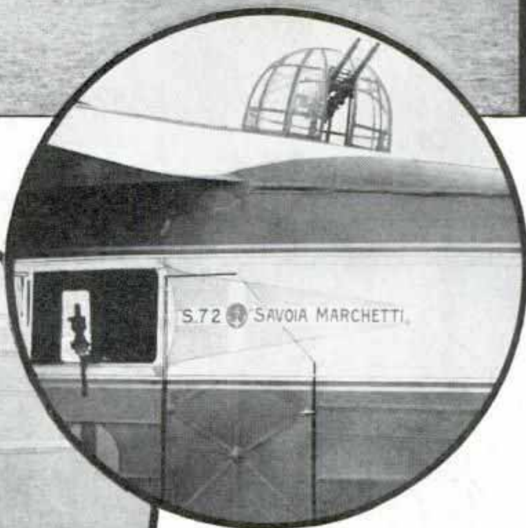
Close-Up of the Savoia Marchetti Bomber; Note Gun Turret on Top of Ship
