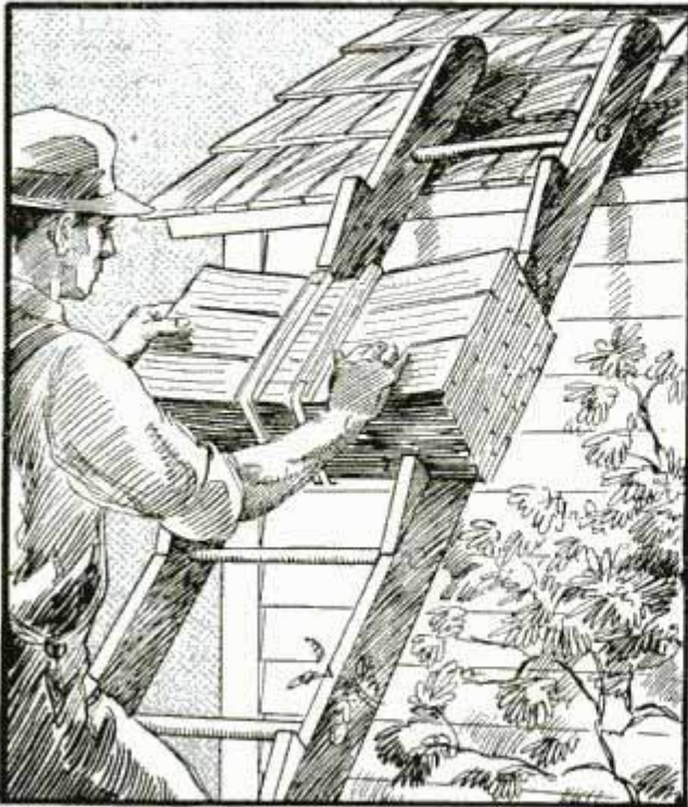
Cleats Nailed to Sides of Ladder Serve as Stops on Which to Rest the Load as You Climb
