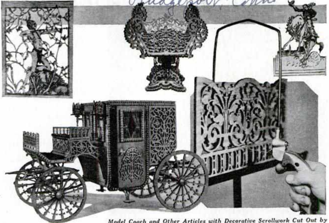
Model Coach and Other Articles with Decorative Scrollwork Cut Out by Electrically Heated Wire of "Saw" Shown in Lower Right Corner
