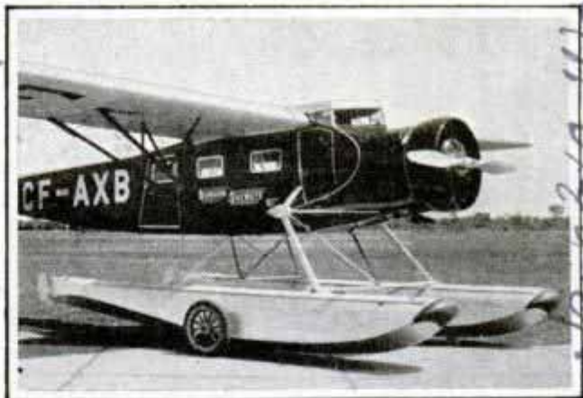
"Flying Box Car" Which Can Carry Ton of Freight and Can Land on Floats, Skis or Wheels
