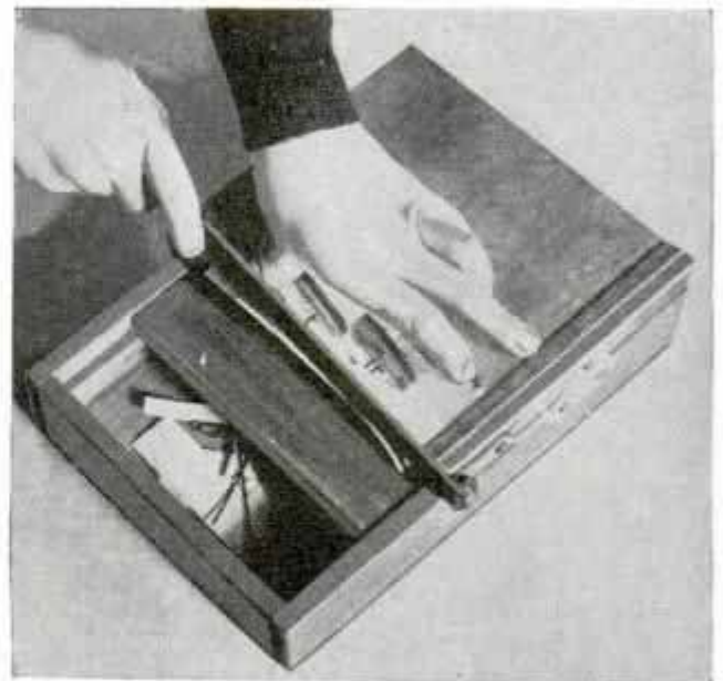
Paper Trimmer Mounted on Box, Which Catches Refuse and Keeps Workbench Clean
