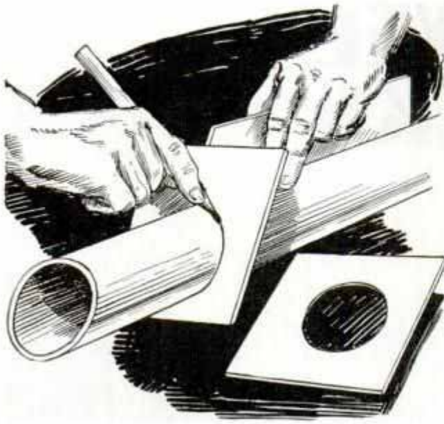
Large Pipe or Tube Cut in Two at an Accurate Angle by Using a Cardboard Template
