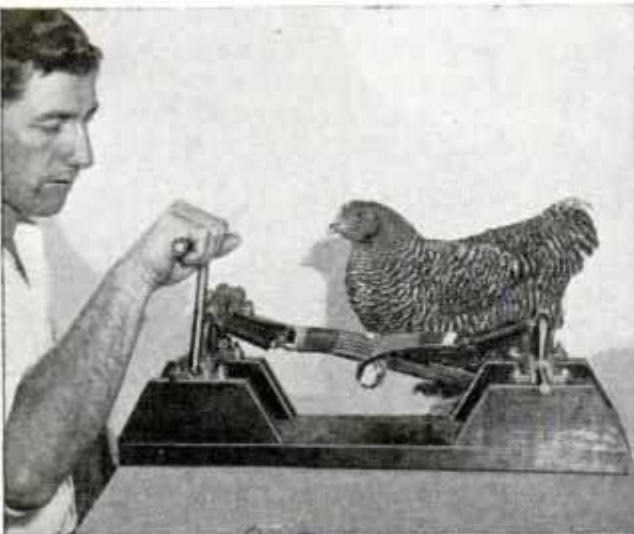
Iron "Gizzard" Testing Samples of Grit Intended for Chickens While Hen Watches the Operation
