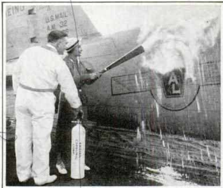
Spraying Plane with Artificial Snow; Interior Can Be Cooled Quickly by a Shower of This Frozen Carbon Dioxide
