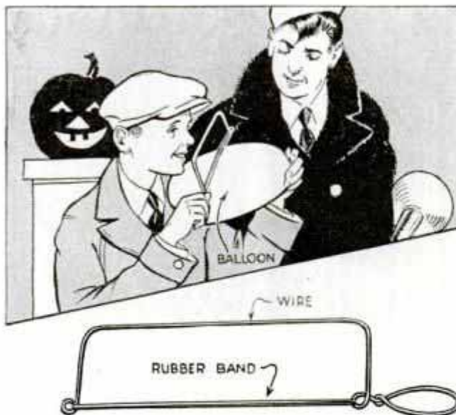
Inflated Toy Balloon Coated with Rosin and Rubbed with Rubber-Band Bow Is a Good Noise-Maker
