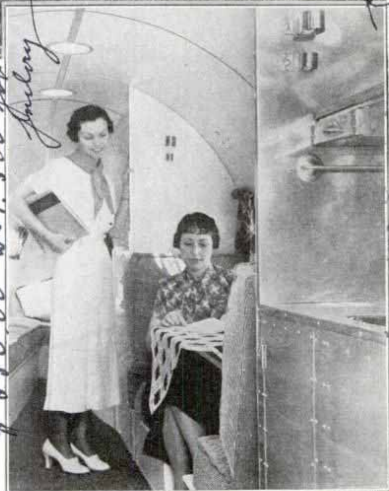
Streamline Trailer with Welded Steel Frame and Duralumin Body Has Two Cabins with Berths, Galley, Tables and Seats
