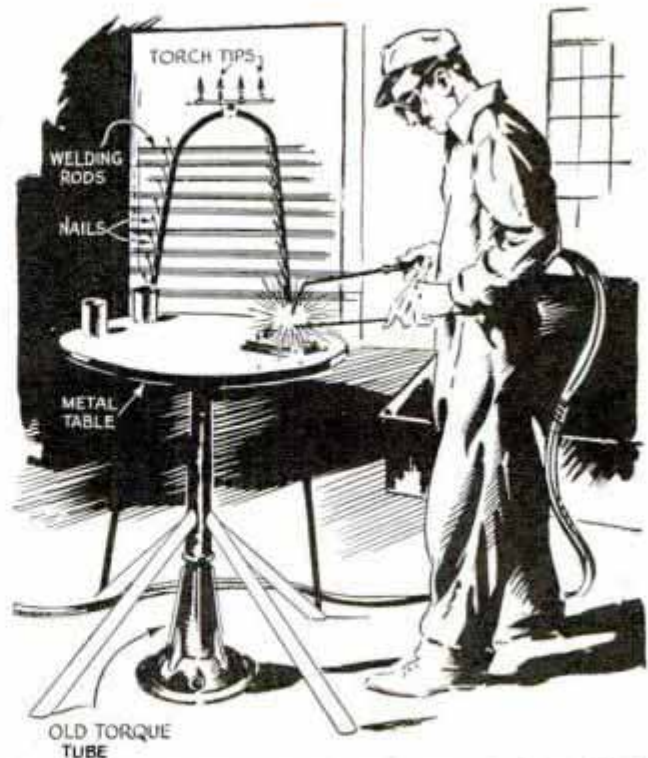
Homemade Welding Table That Has Rack to Hold Accessories Such as Flux Rods and Torch Tips
