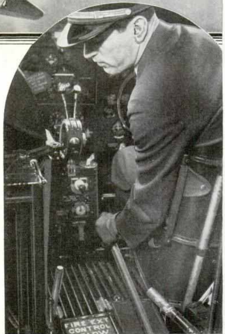
Douglas Airliner in Flight, and Co-Pilot Pumping Lever That Raises Landing Wheels into Engine Nacelles after Ship Has Taken Off and Gained Altitude
