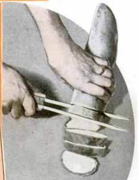
Above, Double-Bladed Knife Cuts Bread in Even Slices; Blades Are Adjustable to Almost Any Thickness; Knife Is Useful for Cutting Meat Loaf, Ham or Cheese
