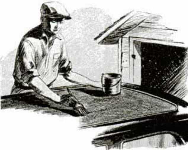
Cracked and Leaky Auto Tops Made Waterproof with Airplane Wing Dope
