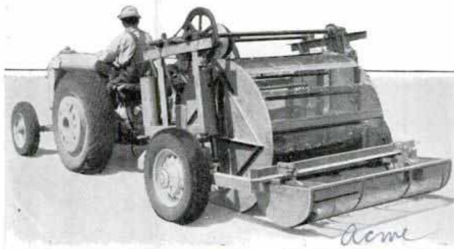
"Beach-Combing" Tractor Picks Up Four-Inch Top Layer of Sand and Sifts Out Picnickers' Rubbish, Cleaning Wide Area Speedily
