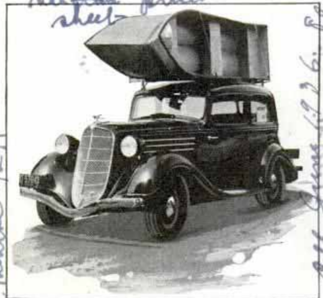
This Eleven-Foot Unsinkable Steel Boat Weighs Eighty Pounds; Its Three Seats Are Air Tanks
