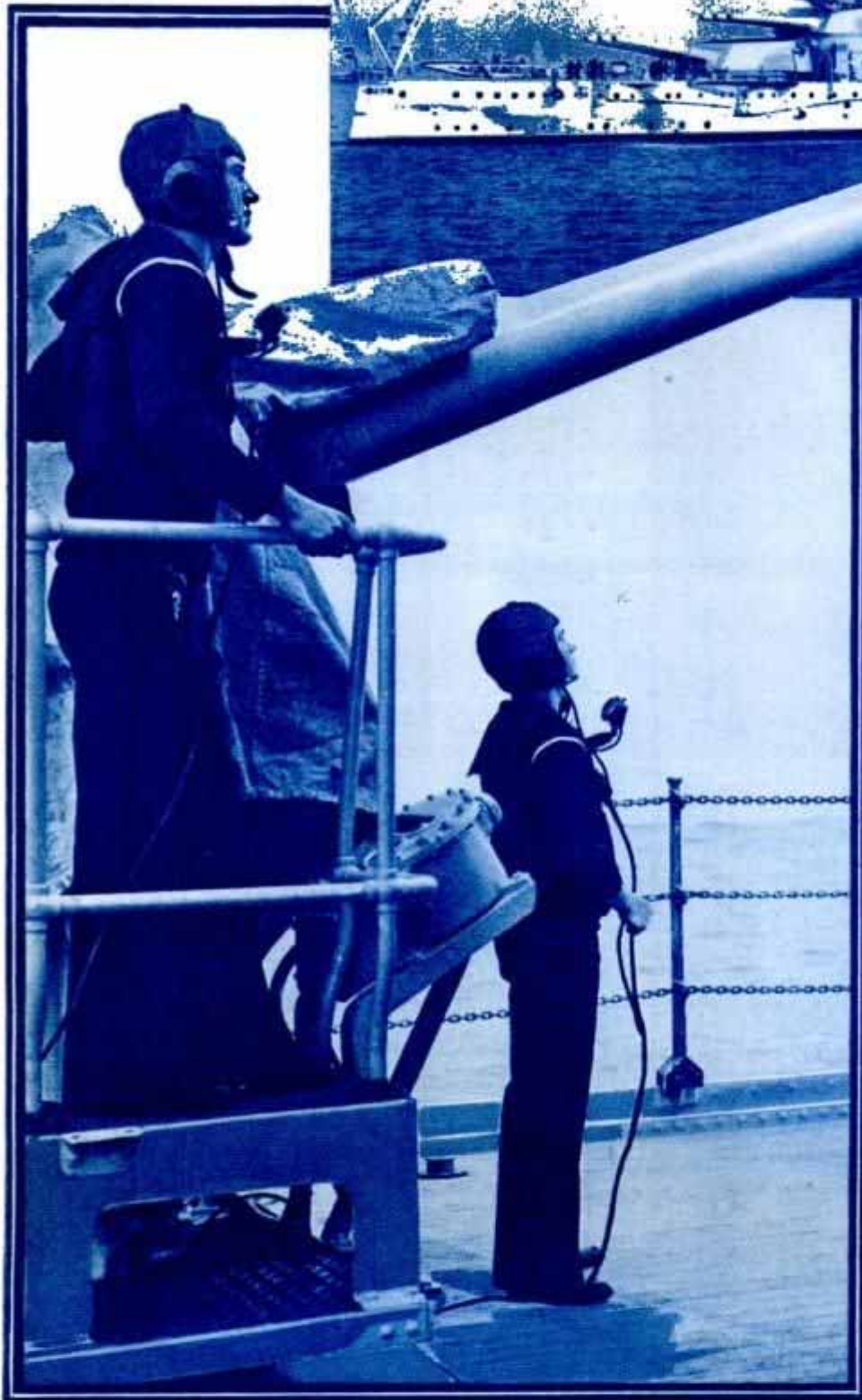
A BOVE, the U.S.S. "Idaho," one of Uncle Sam's latest battle cruisers. Left, anti-aircraft gunners watching the burst of a five-inch shell. These guns are heavy enough to bring down any aircraft. Note that the gunners wear telephone sets inside their helmets. These are for receiving orders from the gunnery officer.
