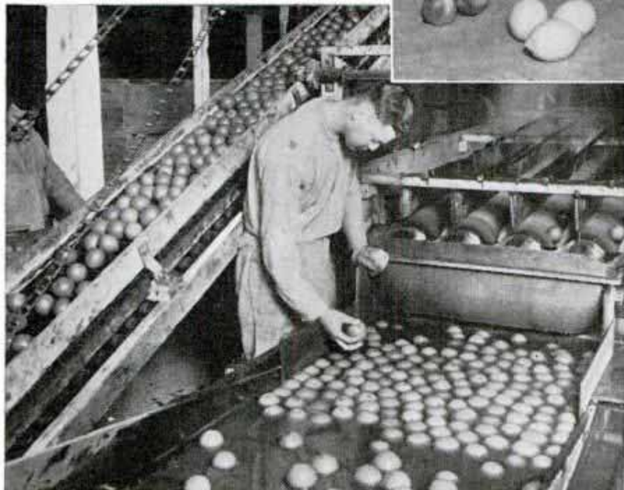
Top, Some Garden Products Kept Fresh by Waxing; Left, Oranges Are Washed, Then Sprayed with Hot Wax Spread Thin by Whirling Brushes; This Coat Checks Decay and Preserves Luster
