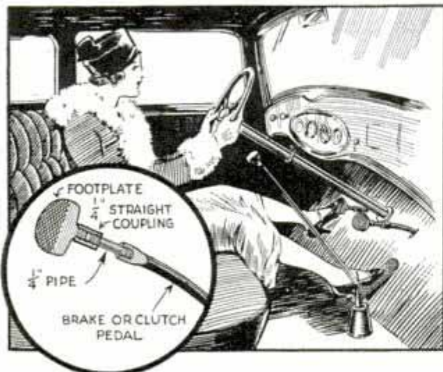
Brake and Clutch Pedals Lengthened by Attaching Footplates with Pipe Nipples and Couplings
