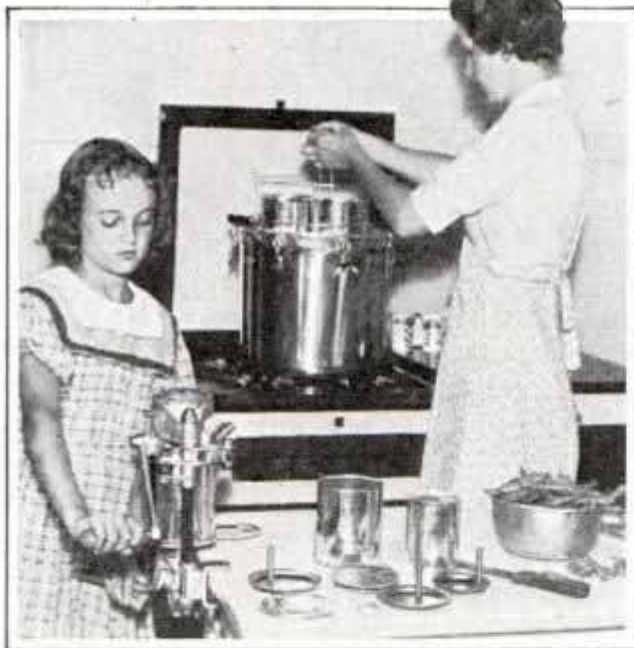
Housewife Puts Tinned Foods into Pressure Cooker While Daughter Seals Tin Cans by Turn of Crank
