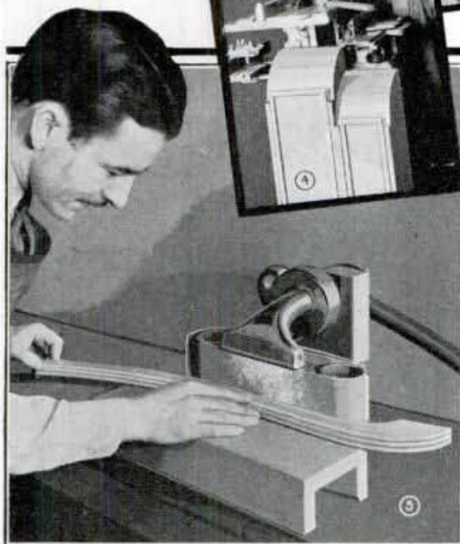
Above, a Small Vacuum Cleaner Takes the Dust Away from the Sander; Right, Method of Eliminating Some of the Dust around a Lathe
