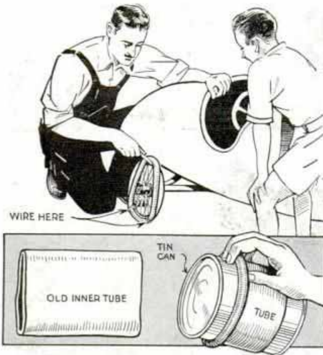
Old Inner Tube Rolled Tightly and Stretched over Rim Makes Good Tire for Coaster Wagon
