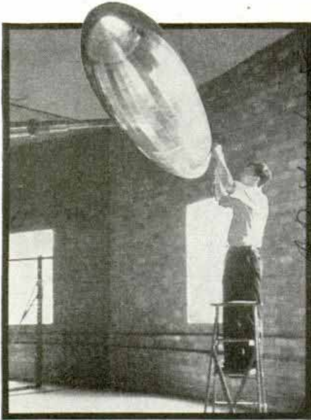
Revolving Arm Spins Model Blimps at High Speed to Test Stresses under Storm Conditions
