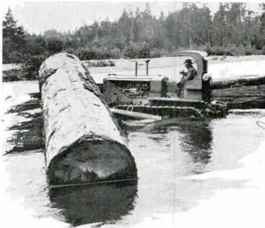
Stranded Log Is Shoved into Current and Started on Way to Lumber Mill by Tractor That Wades Stream as Easily as It Crawls on Land
