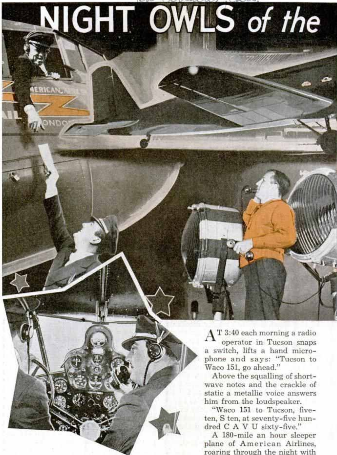
Top, Pilot Receiving Clearance Papers Before Take-Off, Night Transport Ready to Leave and Ground Operator Bringing in Fog-Bound Plane by Listening to Motors and Talking with Pilot by Radiophone; Below, Co-Pilot Using Plane's Radio
