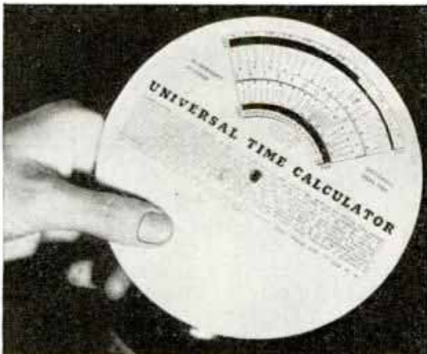
By Manipulating Disks Properly, Any One Can Determine Time at Distant Points
