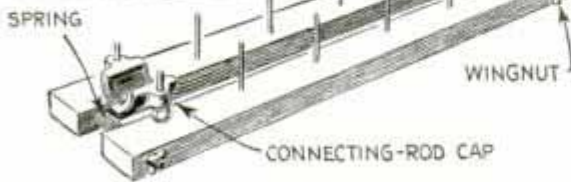
Rack to Hold Nuts, Shims and Bearing Caps Keeps Parts in Order When Overhauling a Motor
