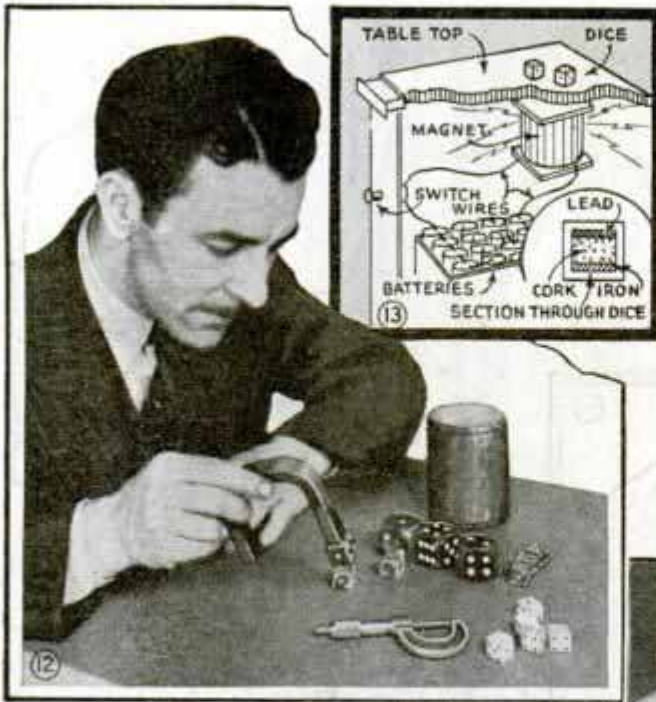
Diagram of Operation of Electric Dice, and Detecting Electric Dice with Magnet; Right, Test for Suction Dice
