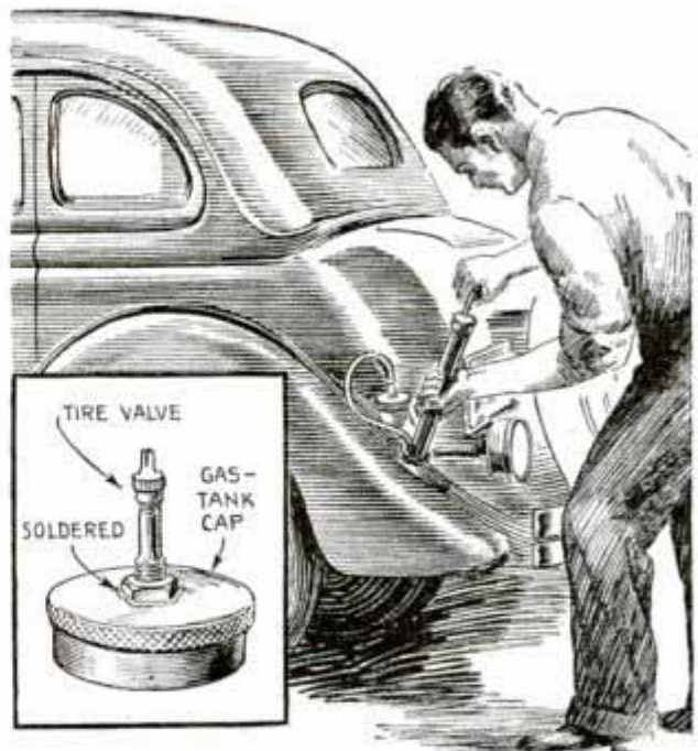
Tire Valve Soldered to Gas-Tank Cap for Use in Clearing Clogged Fuel Line
