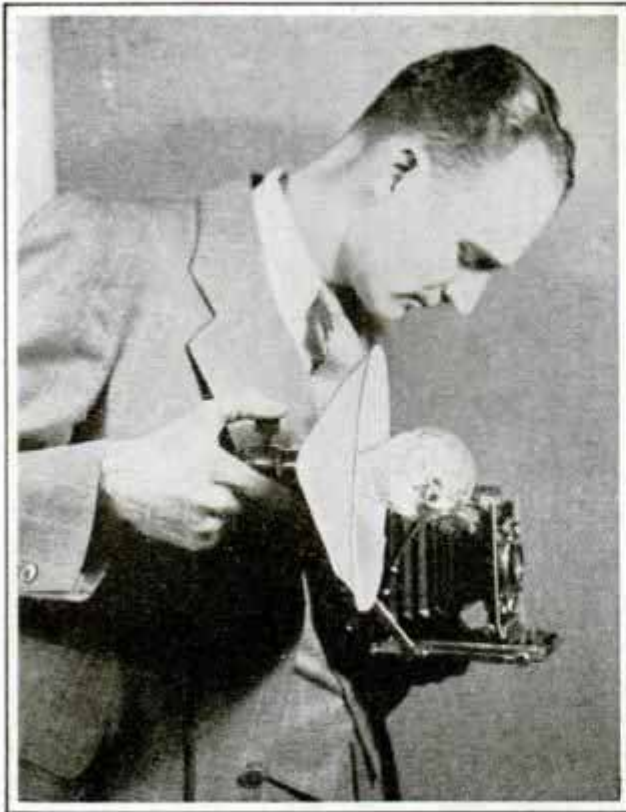
Paper Plate Slipped over Socket to Serve as an Emergency Reflector for a Photo-Flood Lamp
