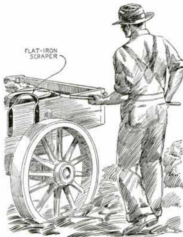
Scraper Made of Flat Iron and Screwed to Wagon Box for Cleaning Spade or Shovel
