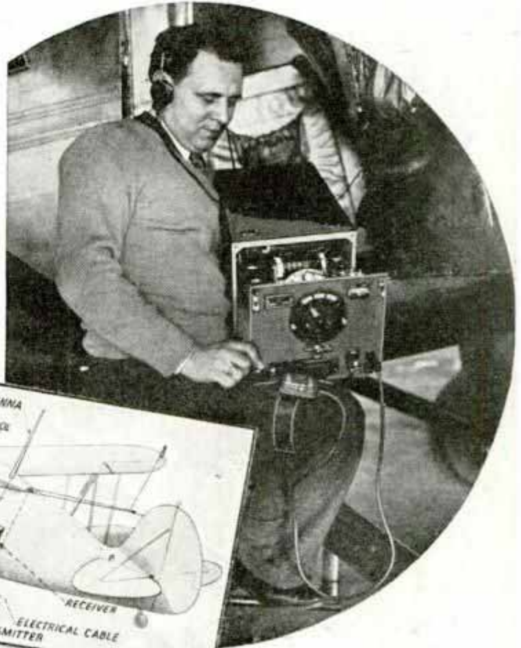
Above, Pilot Slides Chassis of Radio Telephone-Telegraph Transmitter Out of Housing for Inspection; Left, Receiving Apparatus and Compact Receiving Control Box for Instrument Board; Diagram Shows How Two-Way Radio Equipment Is Installed in Small Plane
