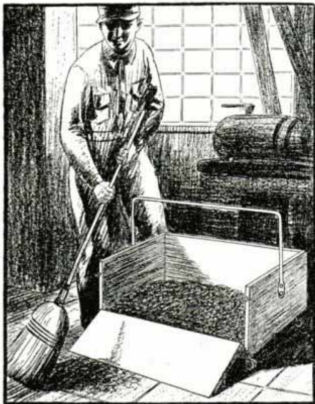
Side of Lathe Scrap Box Drops Down So That Sawdust and Shavings Can Be Swept into It
