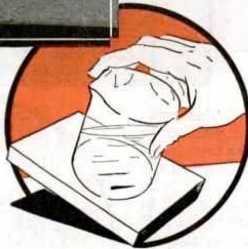
Ammonia Is Used in Refrigeration; This Experiment Shows How Air Blown through Ammonia Will Freeze a Drop of Water between a Thin Beaker and a Block of Wood, so Both Can Be Lifted Together
