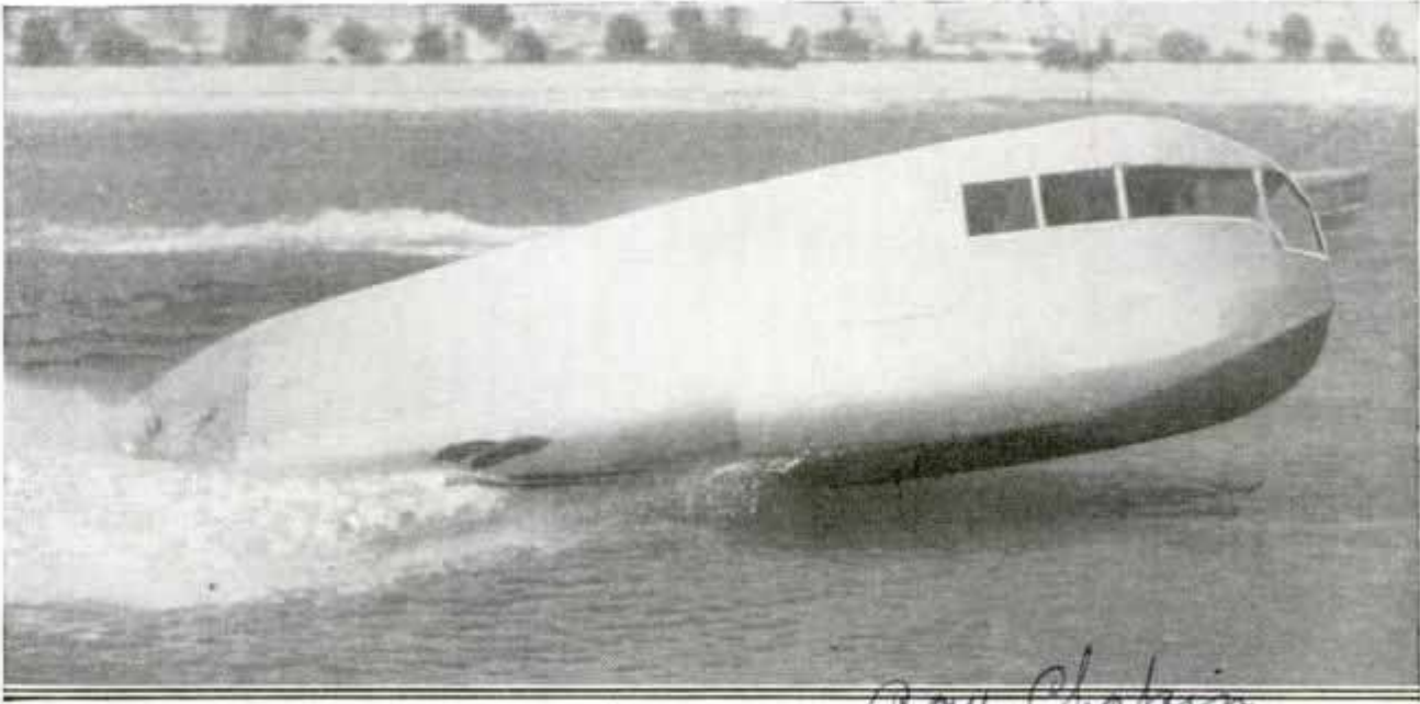
Latest High-Speed Craft Traveling at Fast Pace with Little of Its Bottom Touching the Water; Note Unusual Construction Enclosing the Entire Upper Section to Produce Resemblance to Whale
