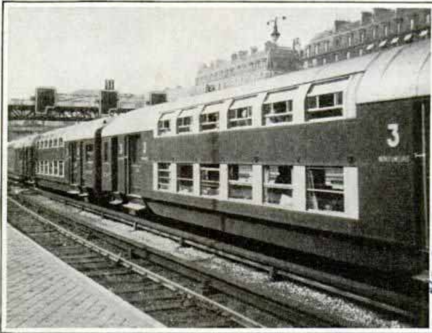
This Odd Looking Coach Has Two Decks to Carry Twice as Many Passengers, Yet Its Height Is No More Than Ordinary Car
