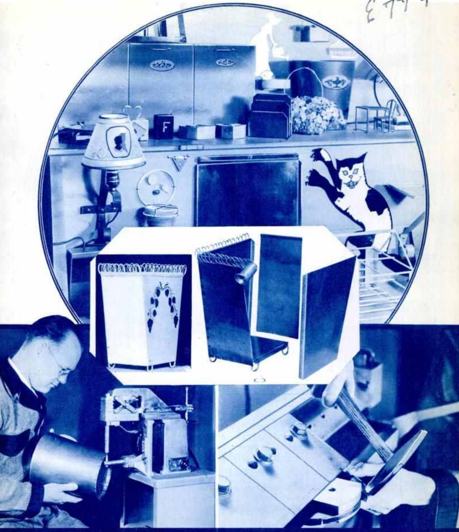
A FEW of the many articles made with the metal-working outfit are shown at the top. The wastebasket in the center can be made with the aid of the outfit in less than half an hour and at a total cost, including finishing and decorating, of less than twenty cents. Note the simple form of assembly and construction. Below, the spot welder is being used to attach the bottom to a wastebasket and, at right, a strip of metal is being shaped on the former.
