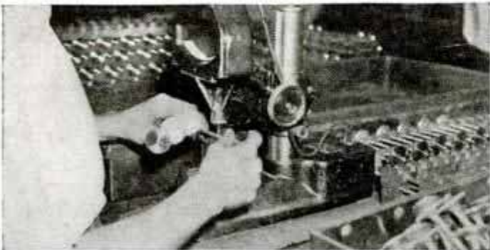
Optical and mechanical magnification gauges check valve stem diameter.
