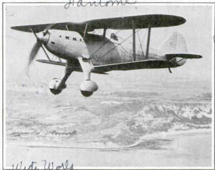
Winged Arsenal Which Carries a Cannon and Four Machine Guns; It Speeds 250 Miles an Hour in Pursuit of Foes
