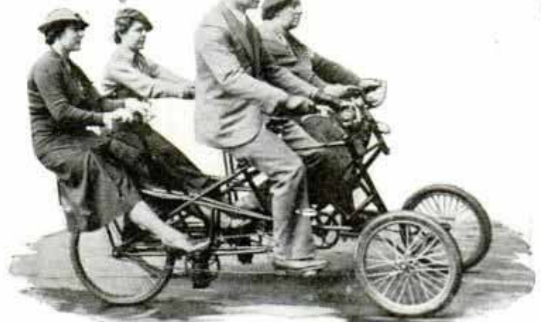
Machine Designed for Whole Family's Exercise Is Propelled by Four Persons, Two Pedaling and Two "Rowing"
