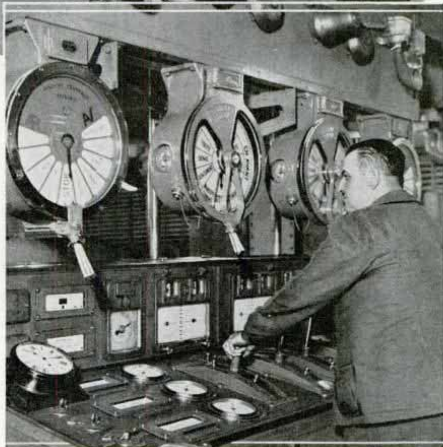
Top, Main Radio Room of the "Normandie"; Below, from This Station It Is Possible for One Man to Control the Two Starboard Engines of the Giant "Normandie," Each One of Them Rated at 40,000 Horsepower
