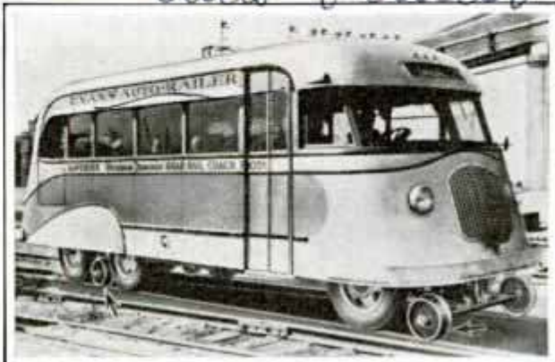
Arrows Indicate the Small Pilot Wheels Which Guide Vehicle's Wheels on Rail
