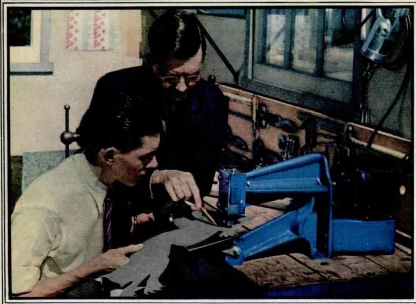
CUTTING out a metal cat on the jig shear as the first step in making a lawn ornament. The shear is operated by a one-fourth horsepower motor.
