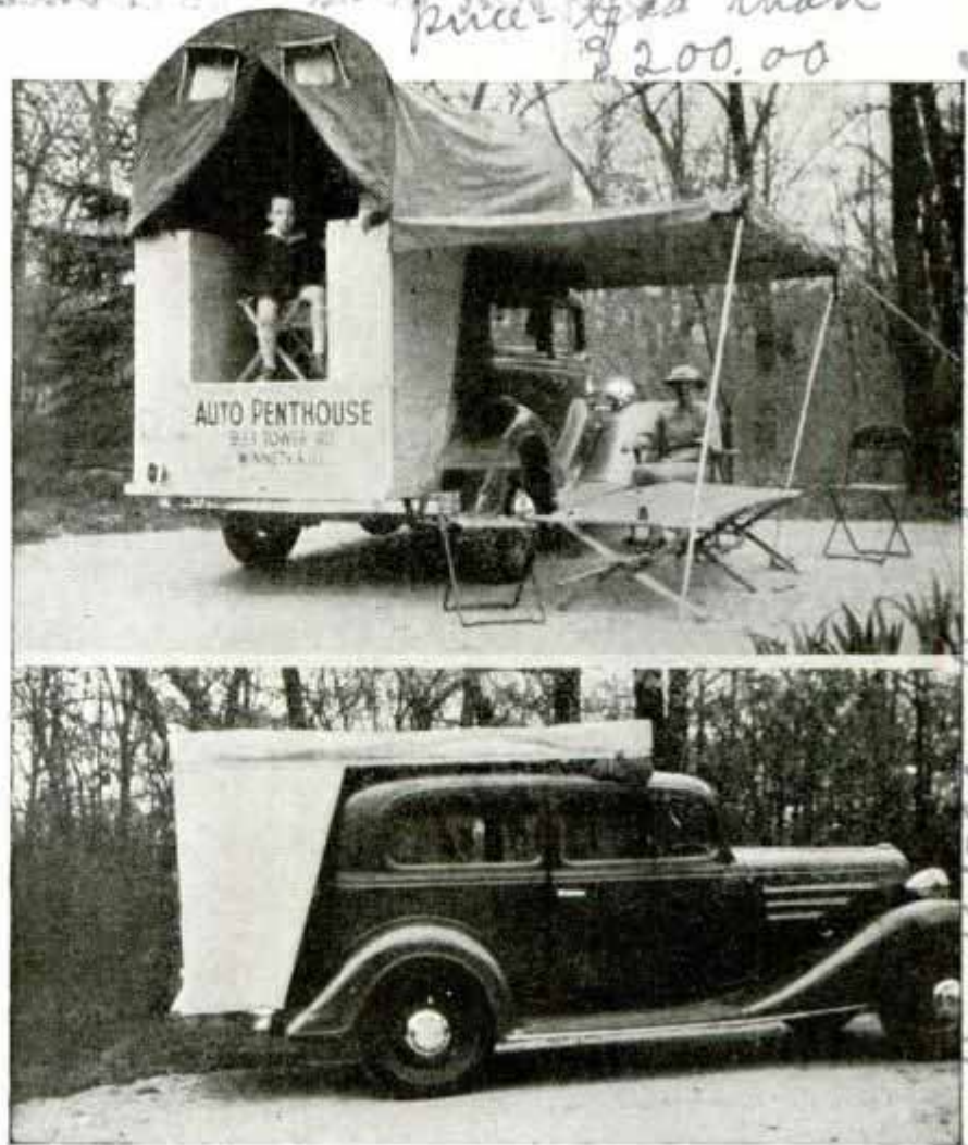
Top, Tourists Have Set Up Penthouse for Night on Road with Side Awning Raised to Shelter Cot or Table; Bottom, Penthouse Packed for Travel
