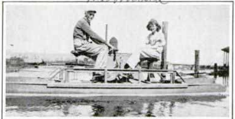
Operators Face Each Other on Dual-Operated Water Cycle Run by Hand or Foot, Standing or Sitting Down
