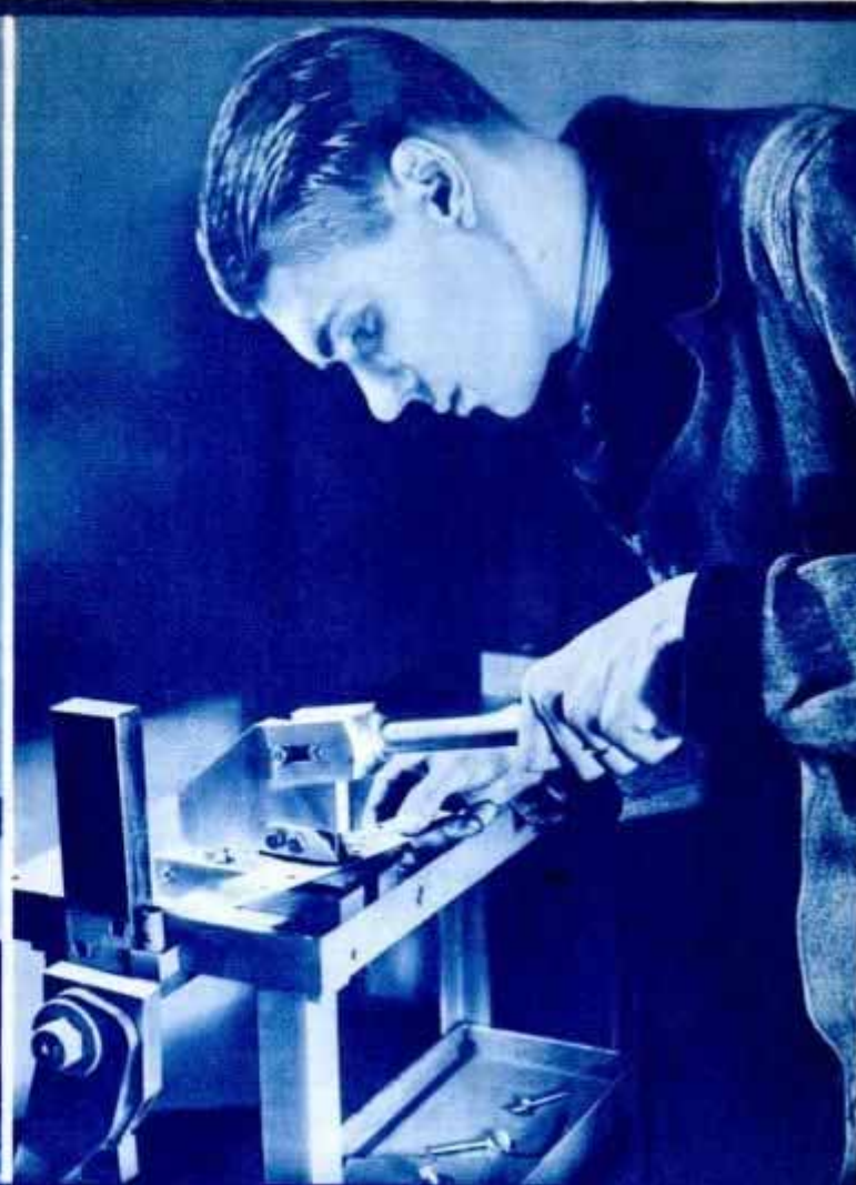
LEFT, operating the compact air-cooled spot welder which makes semi-continuous welds in metal one-twentieth of an inch in thickness or lighter, and, at right, punching holes with the aid of one of the attachments on the shaping machine.
