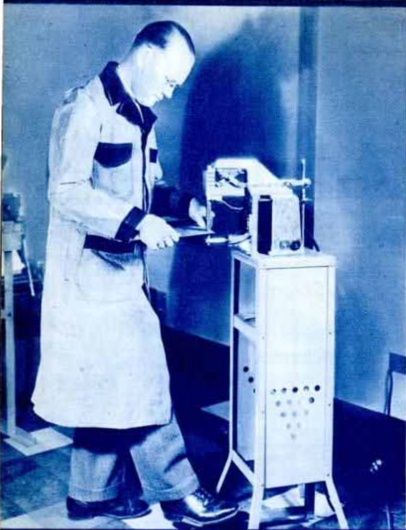
LEFT, operating the compact air-cooled spot welder which makes semi-continuous welds in metal one-twentieth of an inch in thickness or lighter, and, at right, punching holes with the aid of one of the attachments on the shaping machine.
