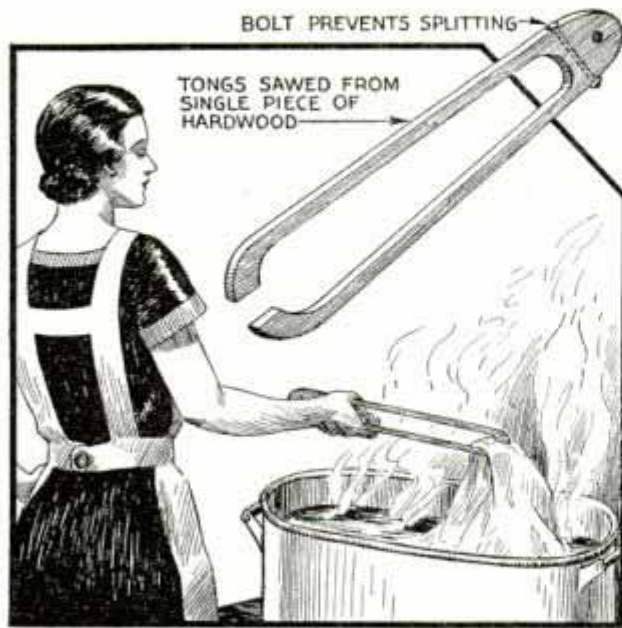
Hardwood Tongs Prevent Burning the Hands When Removing Hot Clothes from Washboiler
