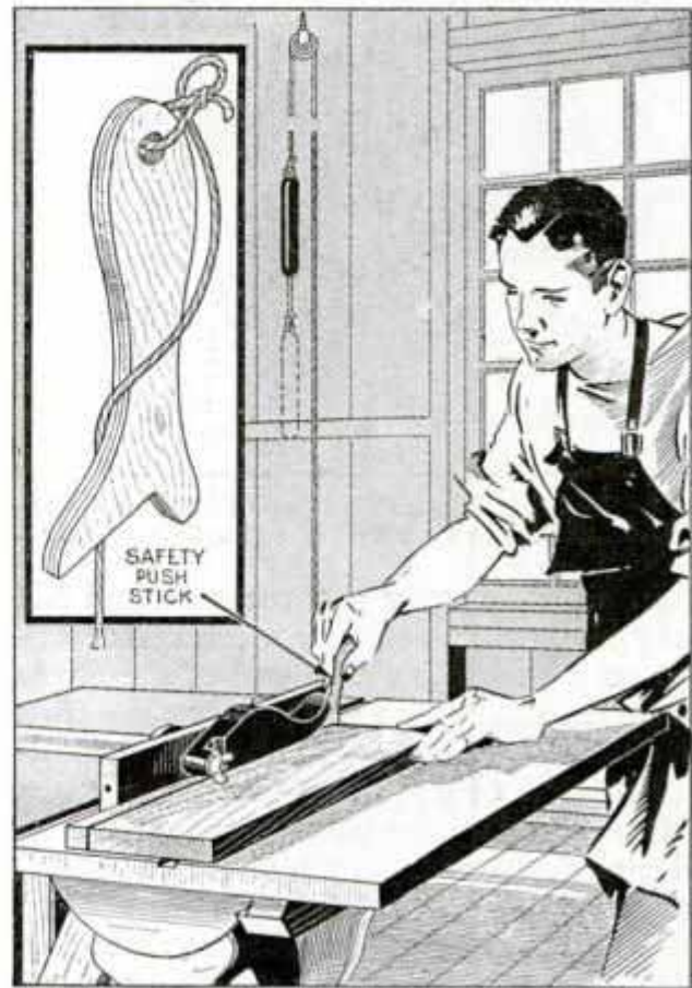
Counterweighted Push Stick Suspended above Circular Saw Always at Hand When Needed
