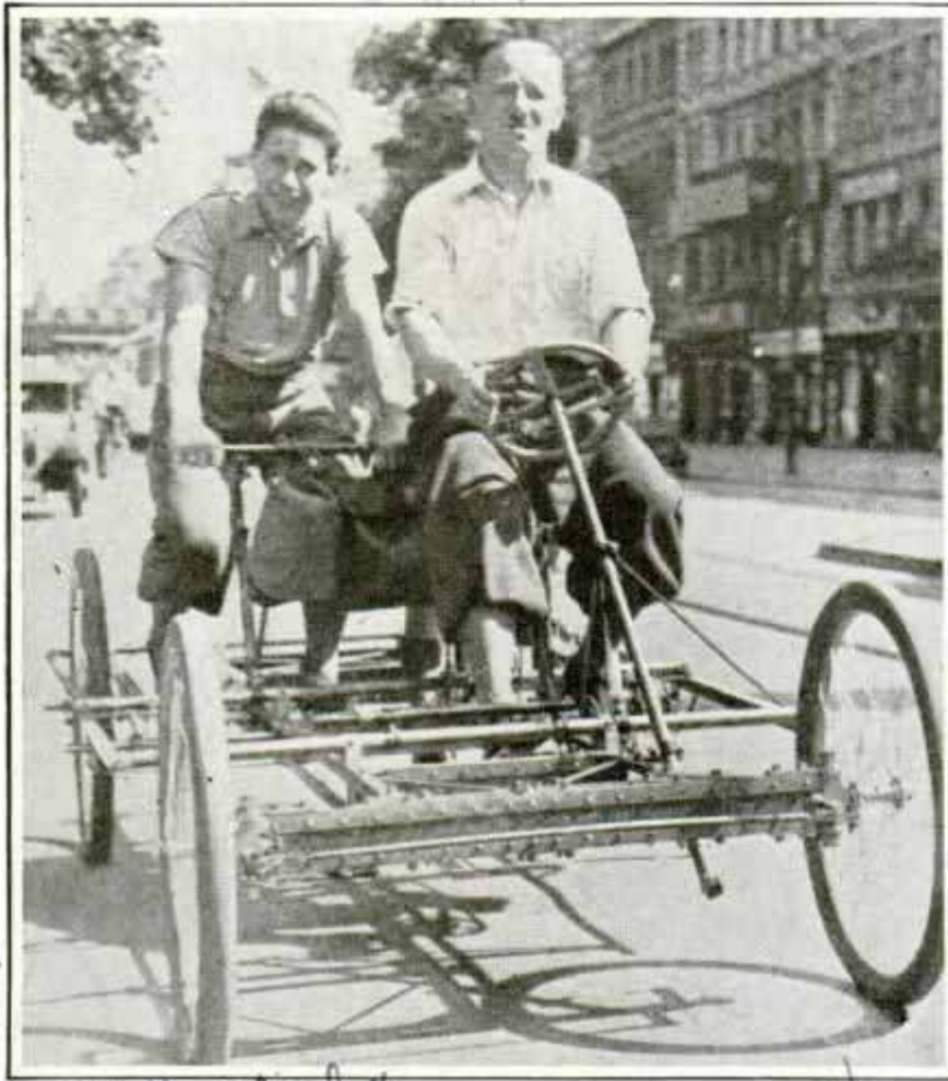
Passengers Operate Motorless Car by Pumping Pedals Which Transmit Power to Wheels
