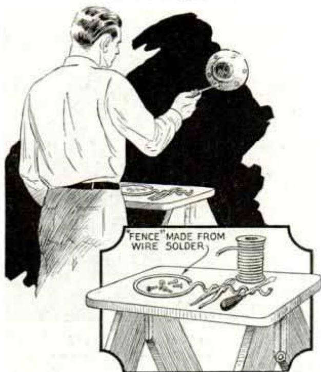
Worker Uses Wire-Solder Ring to Hold Small Parts on Top of Stepladder
