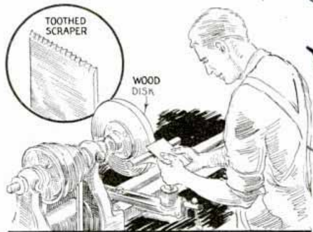
Wood Disks Turned Smoothly by Using Toothed Scraper, Which Is Made of Steel
