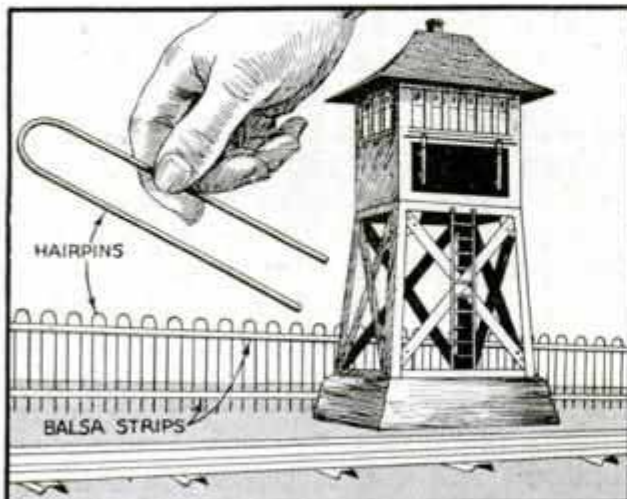
Hairpins Inserted through Thin Strips of Wood Provide a Miniature Fence Which Adds to the Appearance of Your Model Railway
