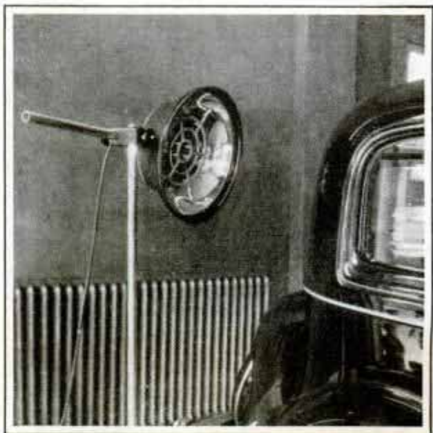
Electric Heating Coils in Portable Reflector Speed Up Job of Painting Car
