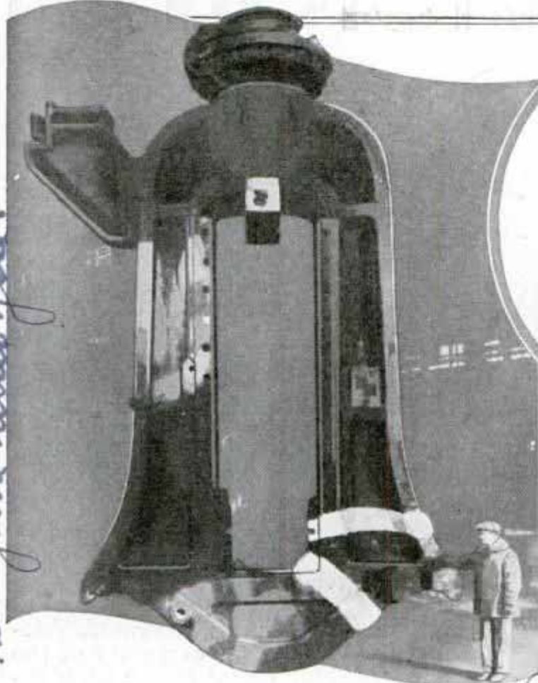
Above, Molten Steel Pouring from Crucible into Mold around End of Rails, Thermit-Welding Them into Solid Ribbon of Steel; Left, Thermit Weld Was Used to Repair Breaks in This: Huge Casting, Twenty-Two Feet High and Fifteen Feet Wide
