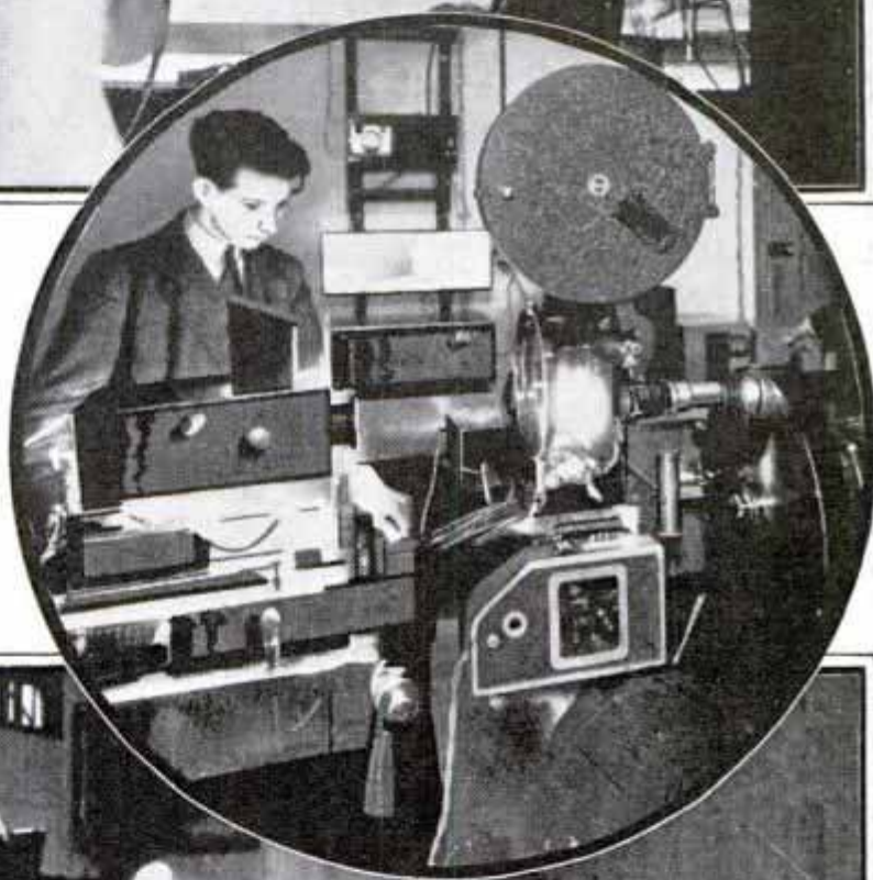
Above, Scene Being Transmitted from Crystal Palace by Intermediate Film Process; Right, Telecine Apparatus for Transmitting Talking Pictures; Below, Preparing to Transmit a Boxing Exhibition by Radio
