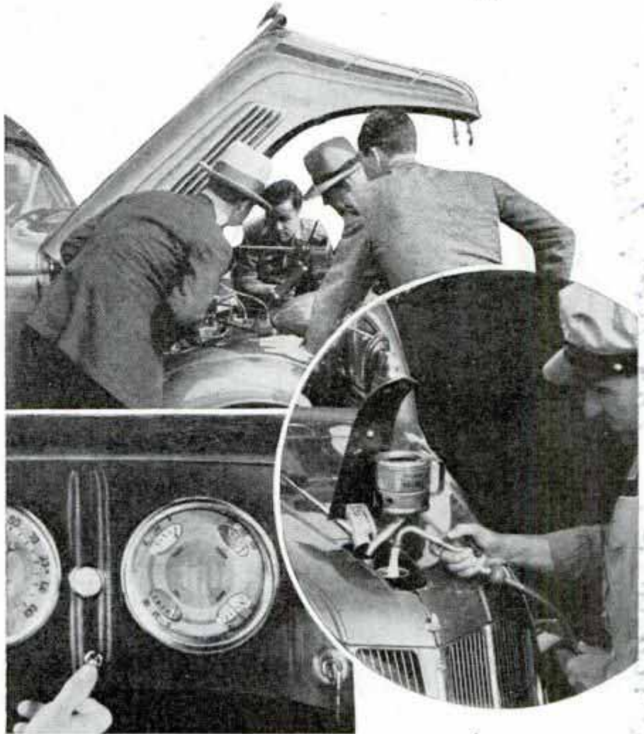
Top, Hood and Grille Lift as Unit; Left, Fuel Gauge Tells Oil Level on Pressing Button; Right, Door in Hood for Water and Oil
