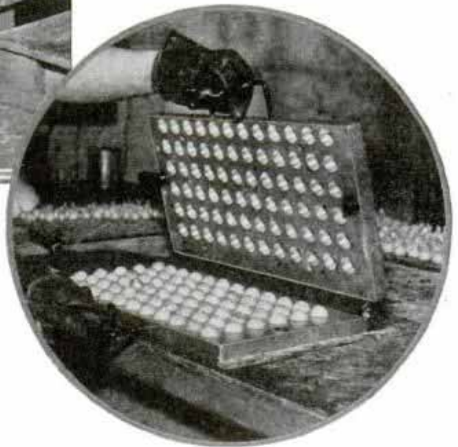
Top, Testing Resiliency under Pressure; Below, Centers Frozen in Molds to Insure Roundness
