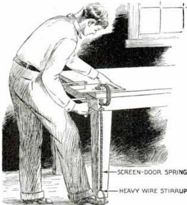
Spring and Stirrup Enable You to Tighten or Release C-Clamp Quickly When Doing Scroll-Saw Work
