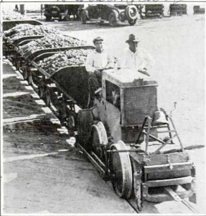
Locomotive Powered with a Gasoline Engine Hauling Cars of Grapes over Narrow-Gauge Railroad from Vineyards to Crushers in California
