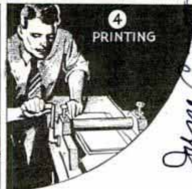
Inking the Thin Celluloid Plate before Transferring Impression to Paper, a Landscape Etching Made in Less Than Two Hours, and the Four Simple Steps in the Process
