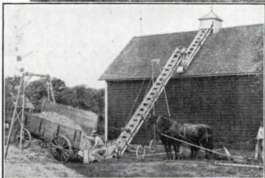
Top, Power Sheller Which Shells Two Tons of Corn in a Forenoon; Below, Power Hoist Saves Farmer's Back
