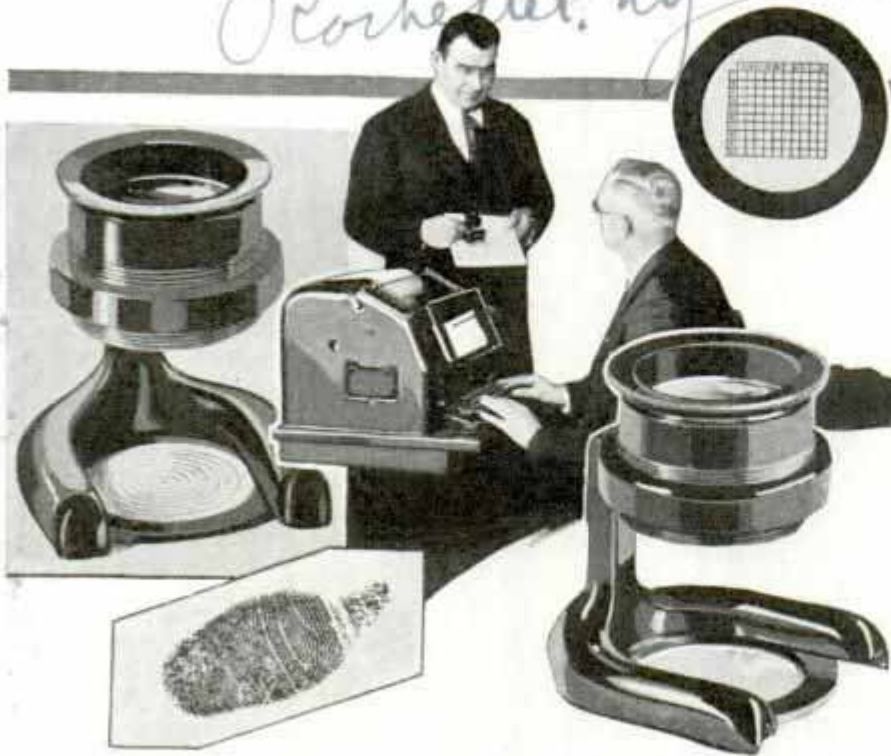
Apparatus for Sending Fingerprints by Wire; Note Equipment for Quick Comparison of Prints Received by the New System
