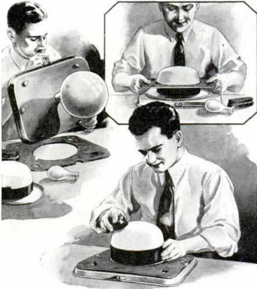
Left, Balloon Is Inflated; Right, Hat Is Placed over Balloon and Card-board Laid on Brim; Below, Hat Ready for Cleaning and Blocking
