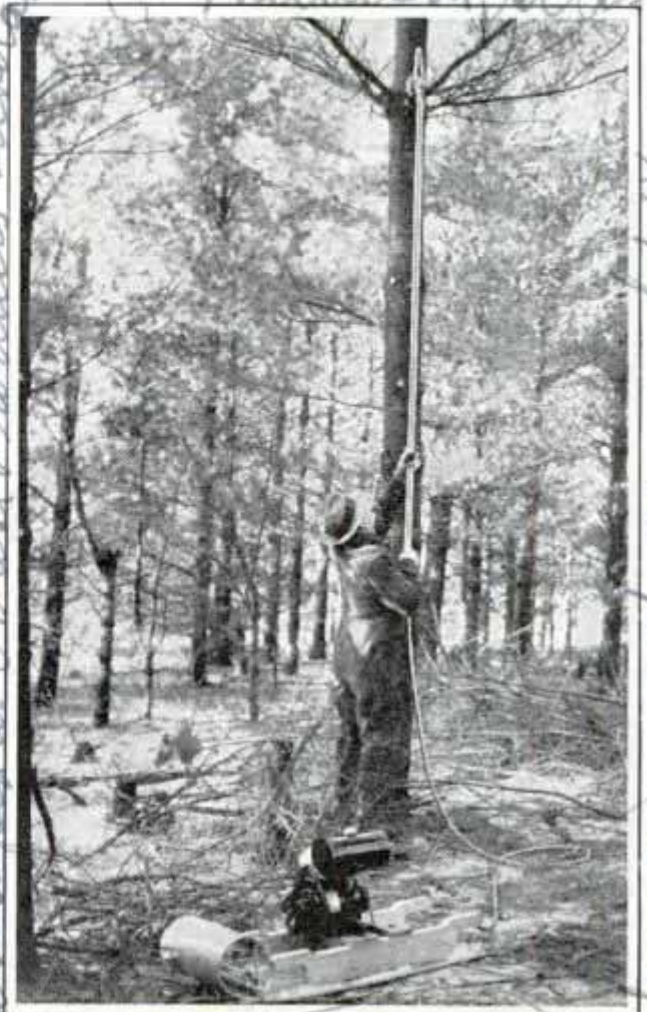
Forester Prunes Low Branches with Circular Saw Atop Pole, Driven by Engine Hauled on Toboggan
