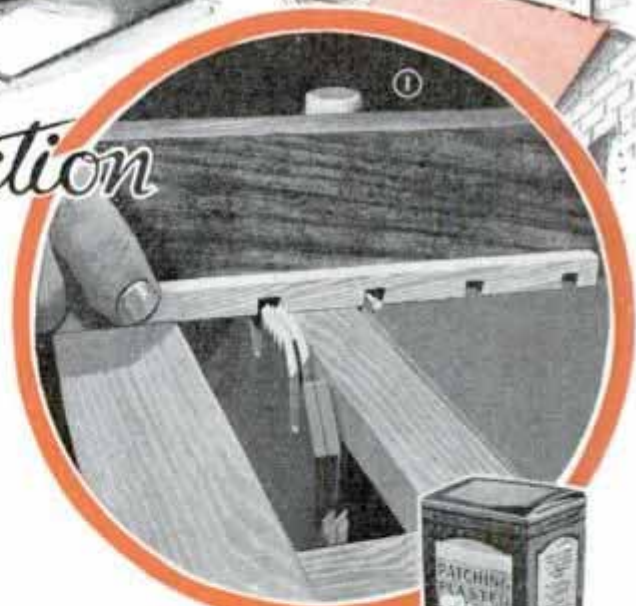
Notched Strips of Hardwood Assembled to Form a Grille in Which the Small Blocks Are Cast
