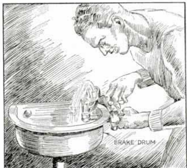
Old Car Brake Drum Mounted on Pipe Standard Serves as Bowl of Drinking Fountain
