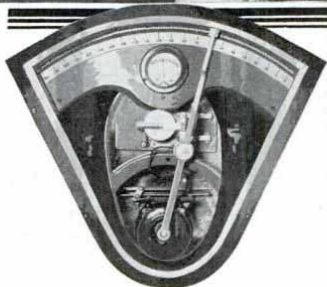
Top, Spitz Flight Recorder with Inventor at Voice Transmitting Microphone; Below, Divergence Wave Meter Which Shows Distance of Radio Signal from the Flight Recorder's Location
