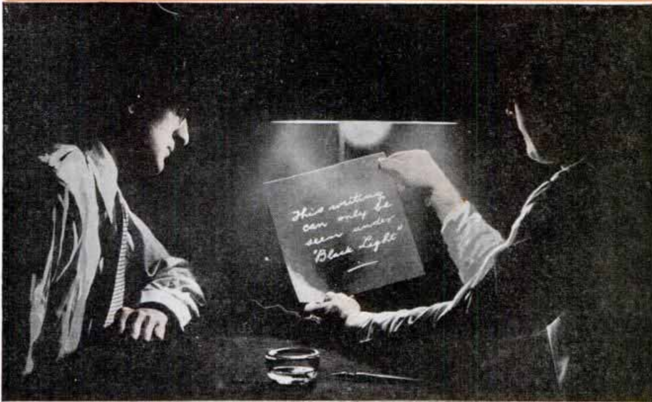
Invisible Inks, Made by Dissolving Quinine in Solution of Water and Alcohol, Lemon Juice or Aspirin Tablets in Water, Stand Out as if Luminescent Ink Had Been Used, When Viewed under the Dim Blue Glow of a Black-Light Bulb
