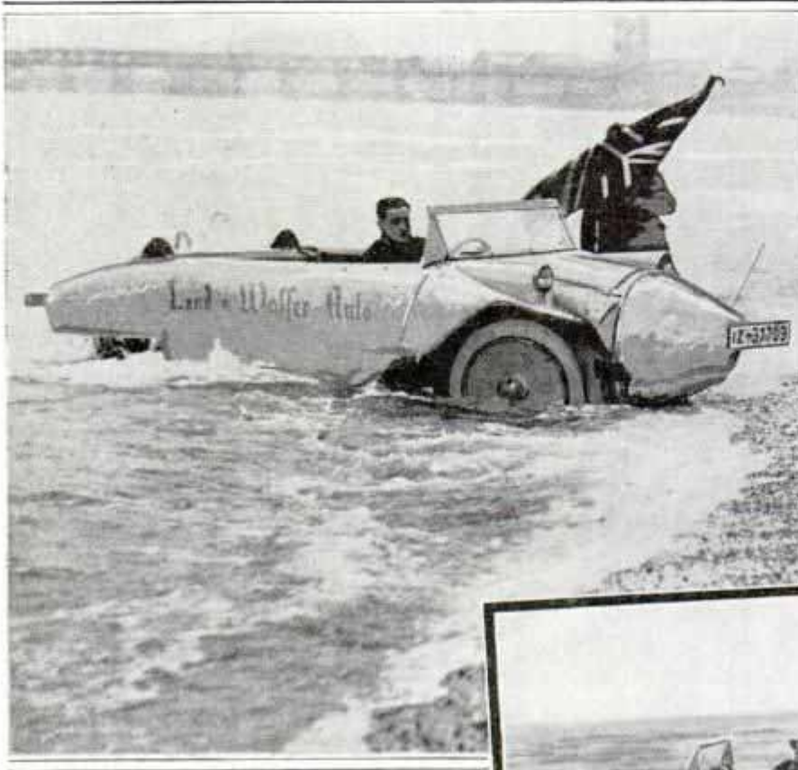
Top, Amphibian Automobile Landing on English Shore; Right, Cruising across British Channel; It Can Travel Twenty Miles an Hour on Road and Paddle Five Miles an Hour on Sea
