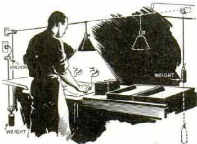
Darkroom Safelight Suspended between Pulleys above Workbench Is Moved Easily to Any Position
