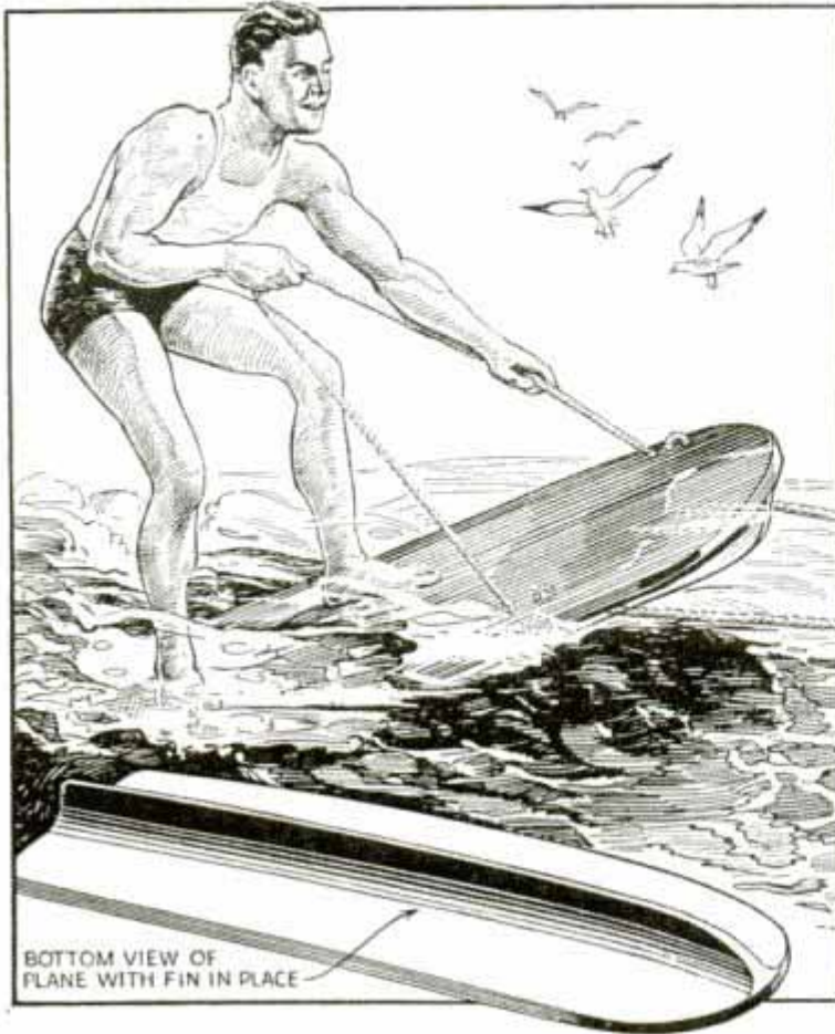
Tapered Hardwood Fin Screwed to Bottom of Aquaplane Makes It Easy to Handle
