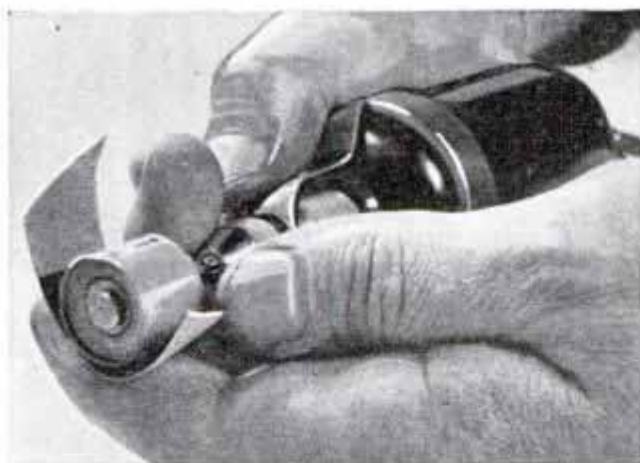
Abrasive Wheels Wrapped with Sandpaper Convert Small Hand Grinder into Sander for Intricate Work
