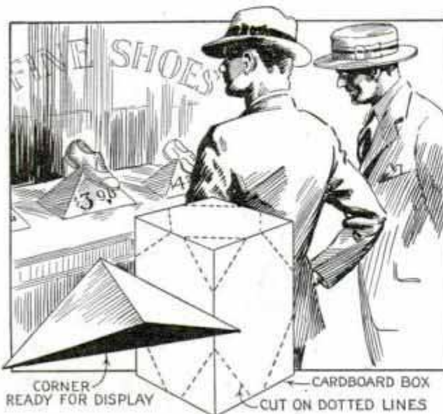
Corners Cut from Cardboard Boxes Used as Stands to Display Shoes in Show Windows
