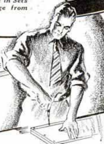
Chassis Construction for Experimenters Not Equipped to Bend Sheet Metal; Thin Copper May Be Laid over Wood Base for Shielding
