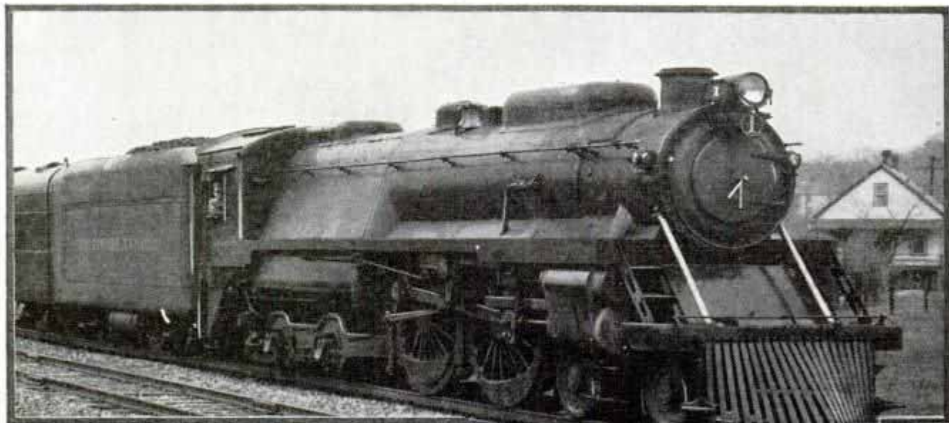
One Foot Lower than Ordinary Locomotives, This Baltimore and Ohio Coal-Burner with Seven-Foot Drive Wheels Can Haul Chicago-St. Louis Passenger Trains 100 Miles an Hour; Train Weighs Half the Usual Type
