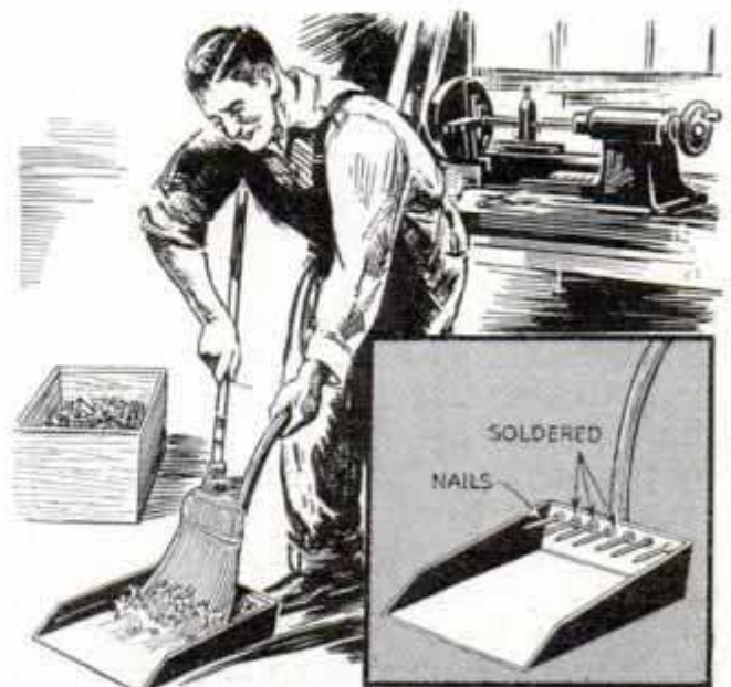
Broom Pulled over Row of Nails Soldered to Dustpan to Remove Metal Shavings
