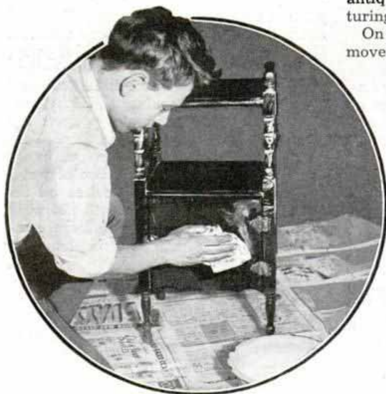
To Remove Surfaces for Painting, First Wash Them Thoroughly to Remove All Traces of Dirt, Greasy Film and Wax
