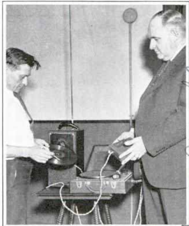
Pressing the Button Held by Man at Right Starts Phonograph Record and Broadcasts Alarm
