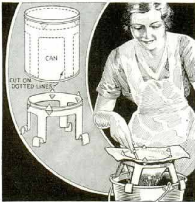
Simple Jig Cut from Tin Can Holds Cloth above Kettle for Straining Fruit Juices
