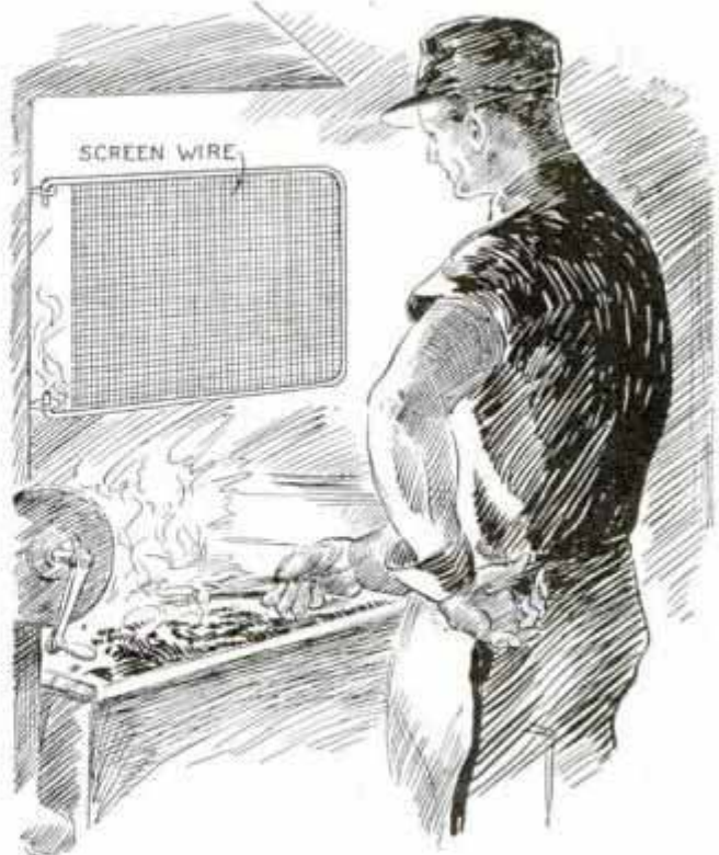
Screen-Wire Shield Helps to Protect Workman's Face from Heat of Forge
