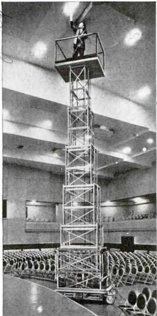
Extension Platform in Raised Position for Servicing Electric Lamps on Ceiling
