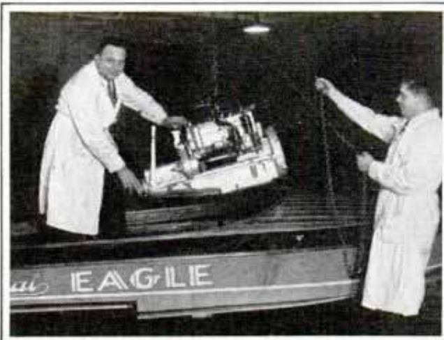
Four-Cylinder Engine Being Installed in Small Speed Boat Can Drive It Sixty Miles per Hour
