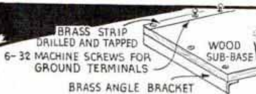
Chassis Construction for Experimenters Not Equipped to Bend Sheet Metal; Thin Copper May Be Laid over Wood Base for Shielding
