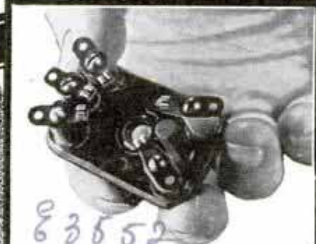
Socket for Acorn-Type Tube Has Flat Mounting Surface Which Aids in Holding Down Plates of Specified By-Pass Condensers
