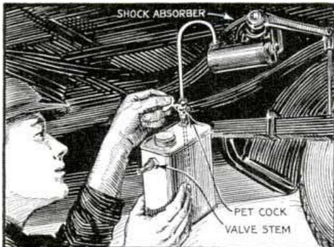
Difficulty in Filling Shock Absorbers Is Eliminated with This Homemade Pressure Can
