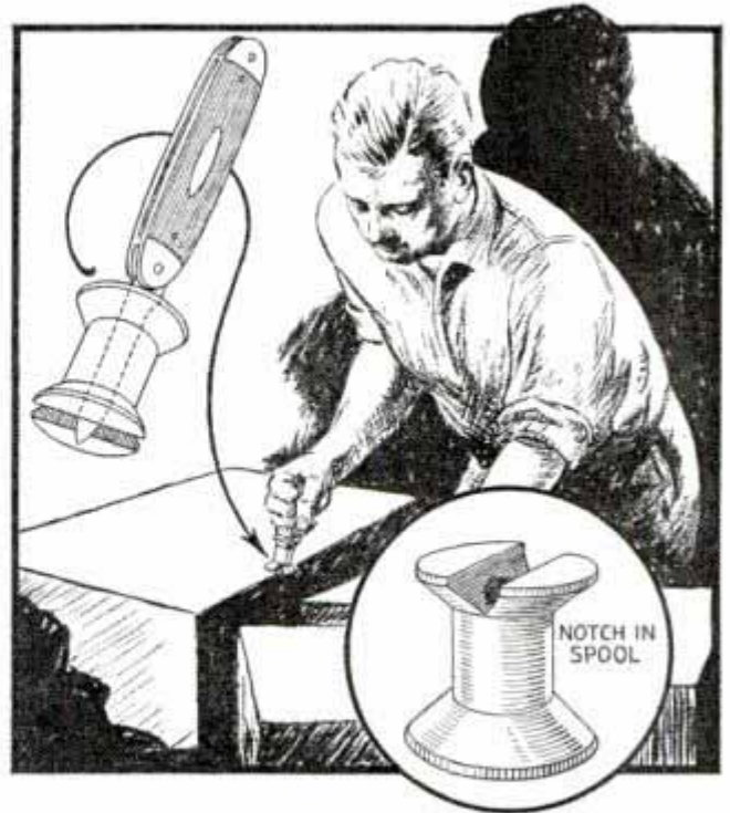
Spool Notched at One End Serves as a Depth Gauge on Knife When Opening Cardboard Boxes
