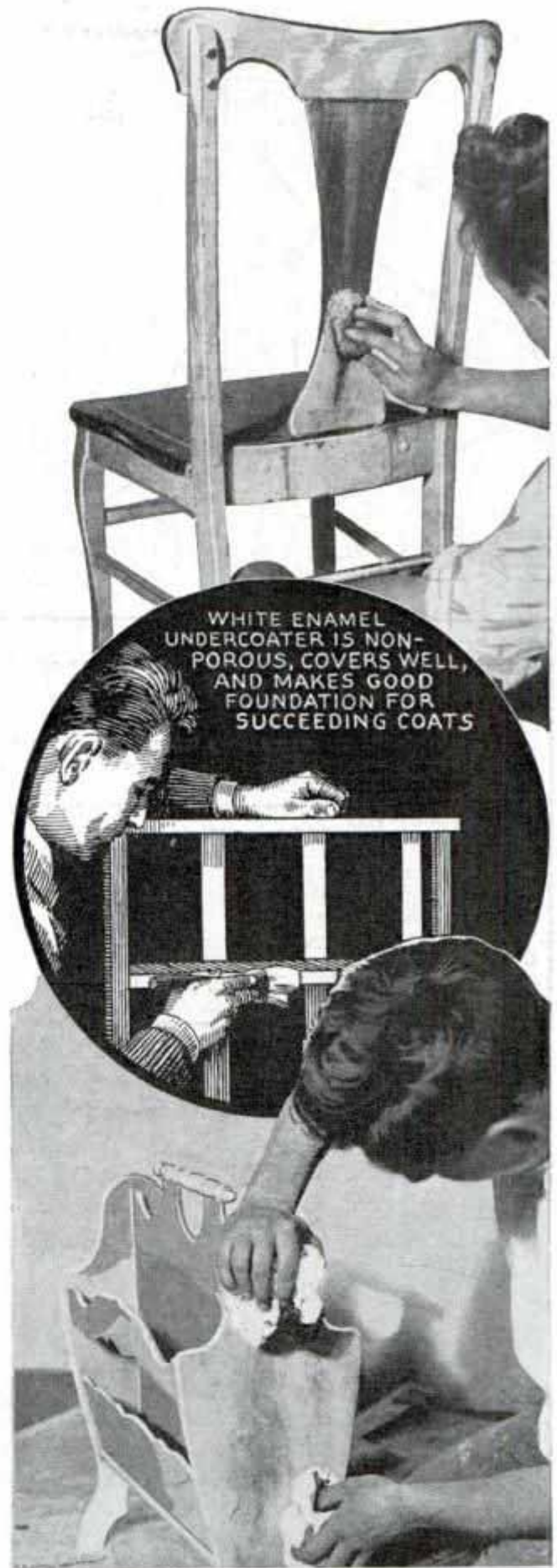
Above, Removing the Old Varnish from a Chair with Strong Solution of Floor Cleaner and Steel Wool; Below, Tinted Glazing Compound Brushed on in Streaks with a Cloth over Entire Surface
