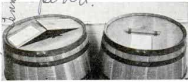
Left, Barrel Head Springs Up with Slat Removed; Right, Slat Screwed at Center Locks Head Tight
