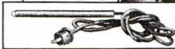
Homemade Probing Light for Working in Dark Corners; Construction Details for Two Varieties Are Given Above; the Multiple Plug Permits Operation of Set and Light from the Same Wall Socket
