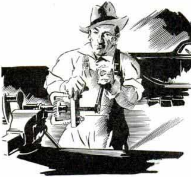
Made from Two Pipe-Wrench Jaws, This Puller Is Adjusted Quickly to Fit Various Gears
