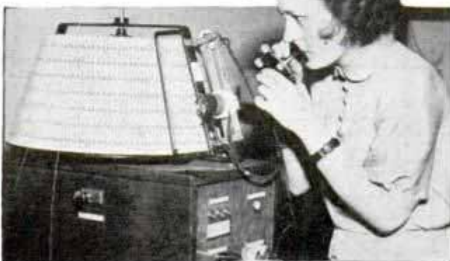
Jonascope As Girl Speaks, Voice Waves and Light Are Synchronized and Tone Is Read on Whirling Record
