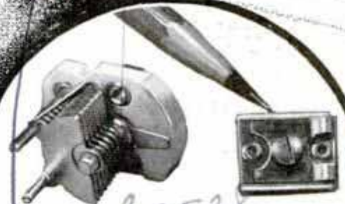
Midget Low-Loss Padding and Trimming Condensers; the Air-Tuned Type at Left Maintains Constant Capacity for Fixed Tuning in Plug-In Coils for Short-Wave Receivers
