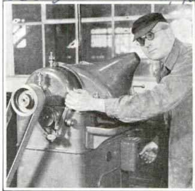
Working Brake Lever with Left Hand, Operator Listens for Note Indicating Defect
