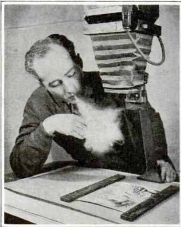
Smoke Blown between Lens and Printing Paper Gives Delicate Diffusion for Enlarging Photos
