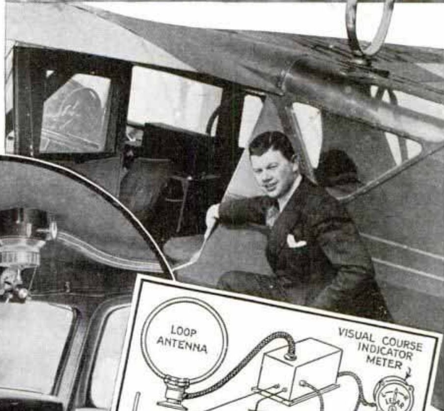
Top, Flying by Course Indicator; Center, Plane with Direction Finder's Loop Antenna; Bottom, Left, Device in Auto; Right, Sketch of the System
