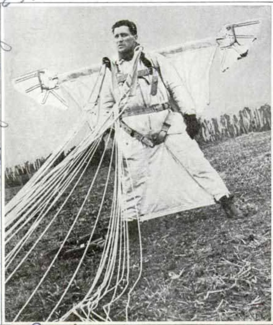
Acme L. A. Schmidt Parachute Jumper Equipped with Wings Which Enable Him to Glide as He Descends; He Opens the Parachute as He Nears the Ground
