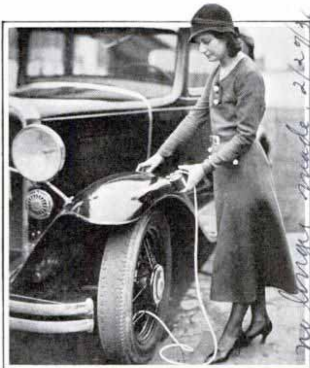
Spraying Fender with Paint Gun Operated by Air Taken from Tire, as Shown in Picture
