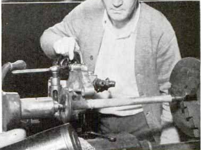
Top, Worn Machine Part Being Grooved or Threaded; Second from Top, Spraying Metal Particles at Rifle Bullet Speed into the Grooves; Third, Preparing to Smooth Off and Polish Rebuilt Section; Bottom (Left), Sample of Rebuilt Part after Completion of Polishing; Its Strength Is Said to Be as Great as When the Part Was New
