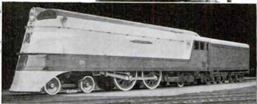
Trim Lines for Speed Feature the Medium-Weight Oil Burning Steam Locomotive of the Milwaukee Railroad's "Hiawatha"
