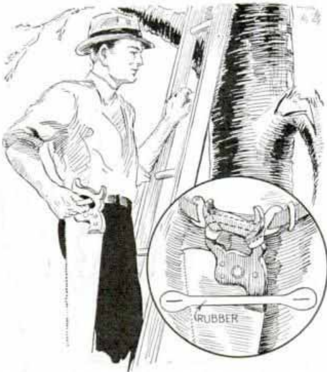
Holder for Handsaw Leaves Both Hands Free When Climbing or When Working on a Ladder
