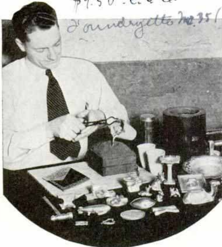
Making Castings with Small Foundry Outfit; This Photo Shows Metal Being Poured into the Casting Mold
