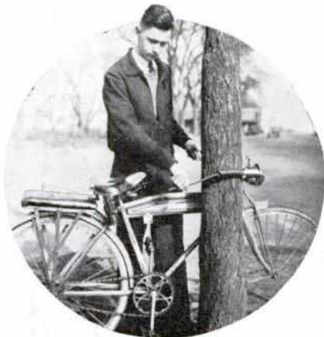
Locking Cable for Bicycle Which Is Concealed Inside the Handlebars When Not in Use
