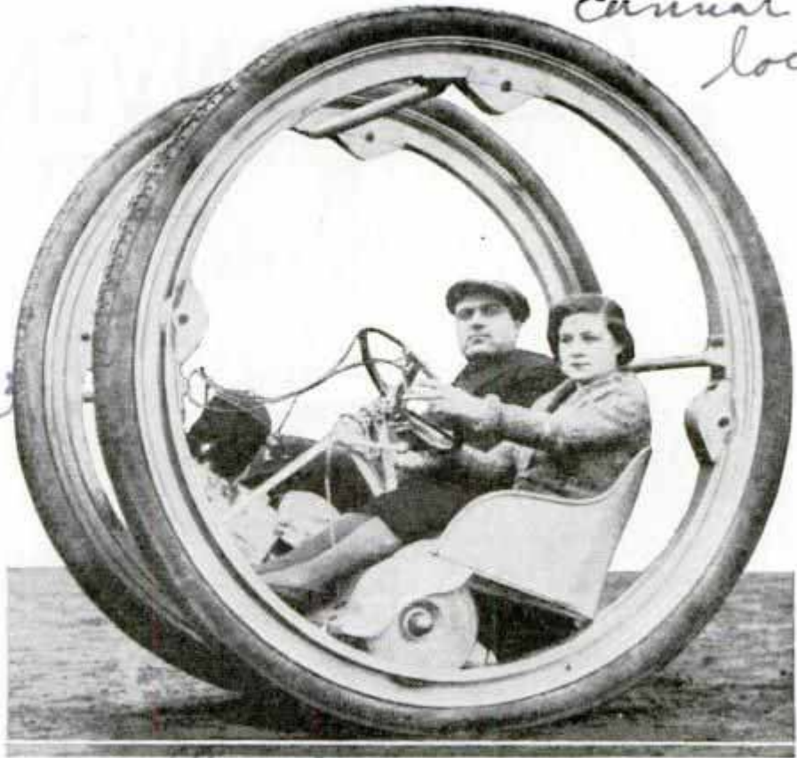
© Planet News Acme Ready for a Spin in This Giant Two-Wheeled Car; a Small Motor Propels the Odd-Looking Vehicle at High Speed
