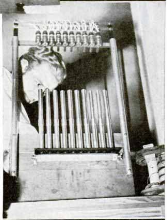
Above, Checking Instruments with Radio Time Signals at Earthquake Station; Below, Machine for Making Physical "Spectrum" of Earth Shocks
