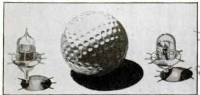
Small Vacuum Tubes Designed for Ultra-Short Waves, Compared in Size with a Golf Ball
