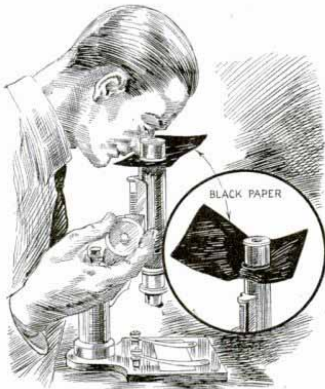
Black Paper over Barrel of Microscope Enables Amateur Microscopist to Keep Both Eyes Open
