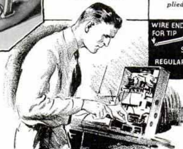
Strip of Insulating Material Provides Easy Method for Fastening Coil Ends Instead of Drilling Holes
