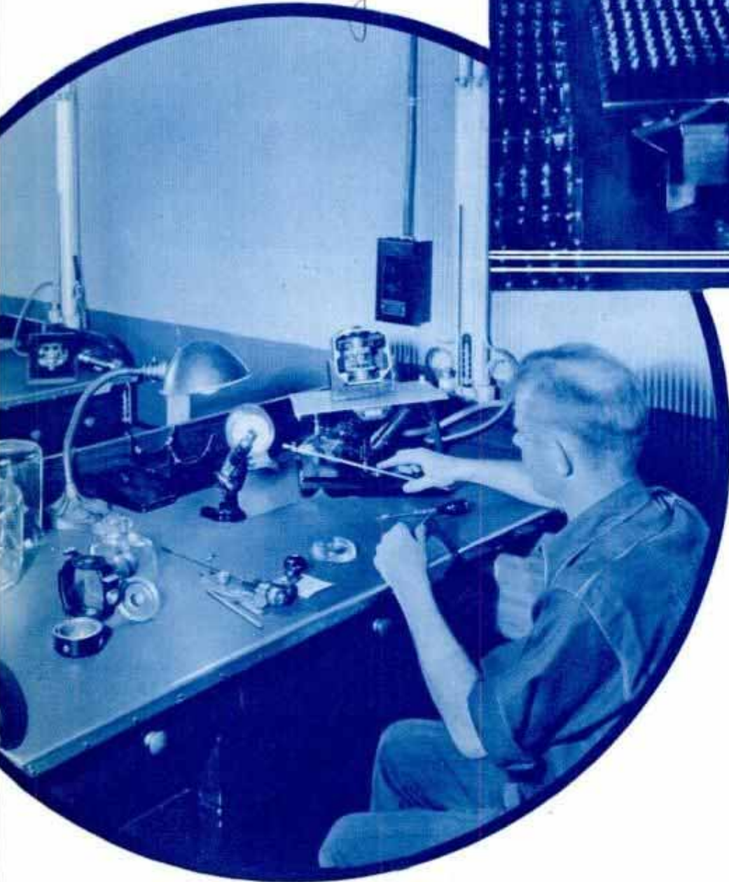
SERVICING and testing the hundreds of spark plugs at the air transport "round house" at Cheyenne, one of the many operations involved in overhauling and repairing the transport planes. Left, testing a directional gyro which has been removed from one of the transports for inspection and service.
