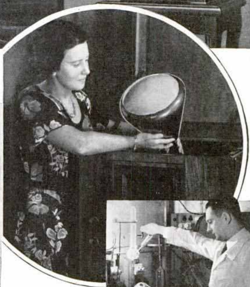
Cathode-Ray Tubes Now Bring Television Right into the Parlor of German Homes; on the Face of the Tube, Framed by a Cabinet, Appear the Pictorial Programs Being Broadcast Regularly in Berlin; at the Left Is the Antenna Mast from Which the State Broadcasting Company Sends Pictures on Ultra-Short Waves; Right, a Cathode-Ray Tube Is Being Evacuated, and Below It a Receiving Set Is Shown Assembled, Ready for Its Cabinet
