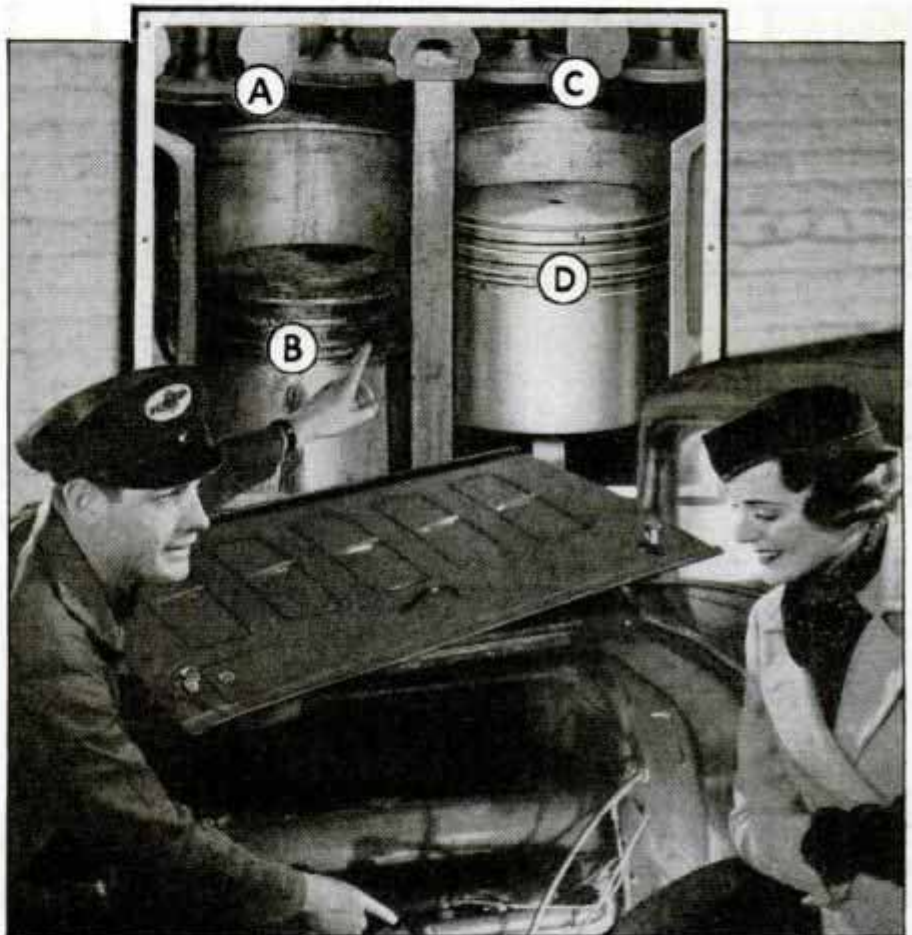
Note sludgy deposits from plain oil on (A) valves (B) piston rings, causing them to stick and leak. Compare with clean valves (C) and clean piston rings (D) lubricated with New Pennzoil
