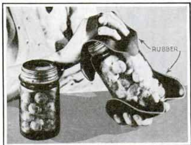
Mitts Cut from Inner Tube Save Time and Protect the Hands When Sealing Fruit Jars
