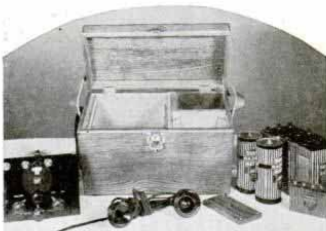
Portable Transceiver Assembly; All Parts, Including Handset and Batteries, Are Housed in Wood Case Provided with Carrying Strap
