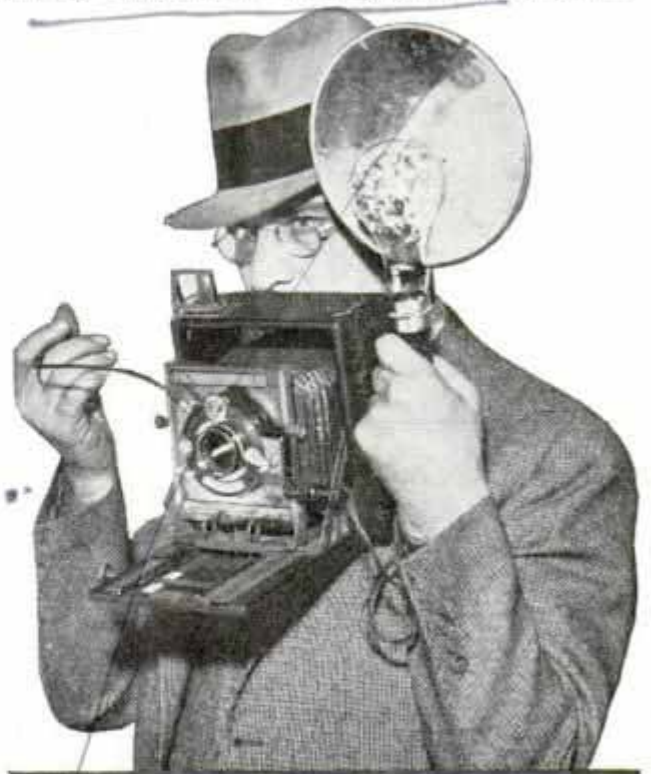
Ready to Snap a Picture; When Shutter Opens to Widest Point, It Sets Off Flash Bulb
