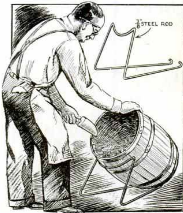
Kegs Supported by Brackets Take Place of Bins Ordinarily Used in Dispensing Nails in Stores
