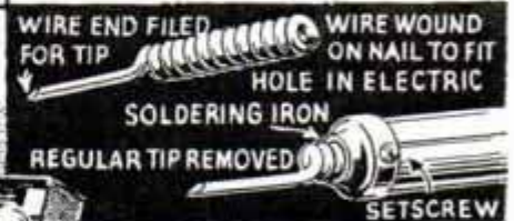
Small Homemade Emergency Tip for Electric Soldering Iron Simplifies Operation in Awkward Chassis Locations; Close-Wound No. 10 Copper Wire Is Substituted for Regular Tip
