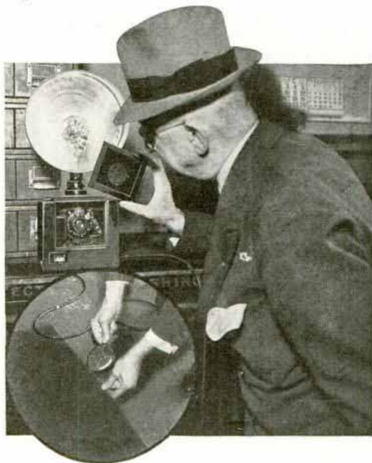
Preparing the Camera with Its Flash; Inset, Hiding the Disk That Would Make Burglar Take His Own Picture
