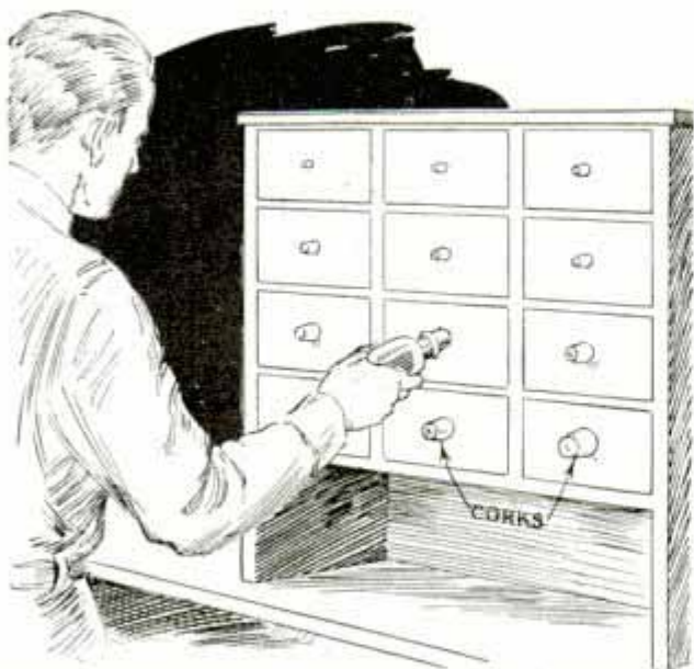
Druggist Saves Time in Fitting Bottles with Corks by Using Latter as Drawer Pulls
