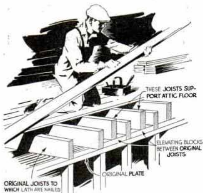
False Joists Support Attic Floor and Prevent Plaster on Ceiling from Being Cracked
