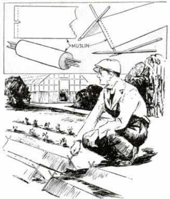
Strips of Muslin Stretched Tent-Fashion over Young Plants to Protect Them against Sun and Frost
