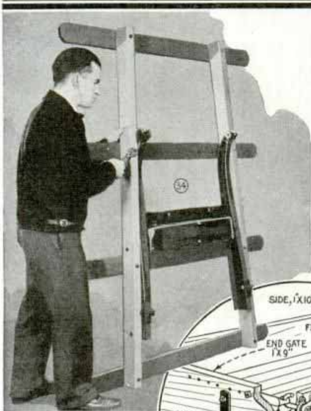
Above, a Simple Chassis Made by Bolting the Forward Frame Section of a Car to a Wood Frame; in Circle, Typical End Gate and Body Construction; Below, Two Boat Trailers from Ford Parts
