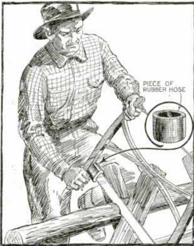
Piece of Rubber Hose Slipped over Heel of Bucksaw Blade Prevents Pinching Your Fingers
