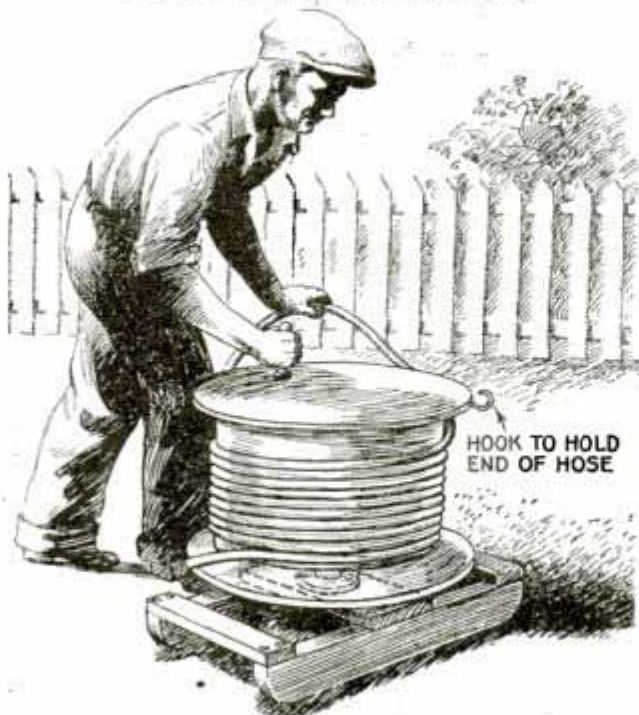
A Garden Hose Will Drain Thoroughly If Wound in One Layer on a Vertical Reel
