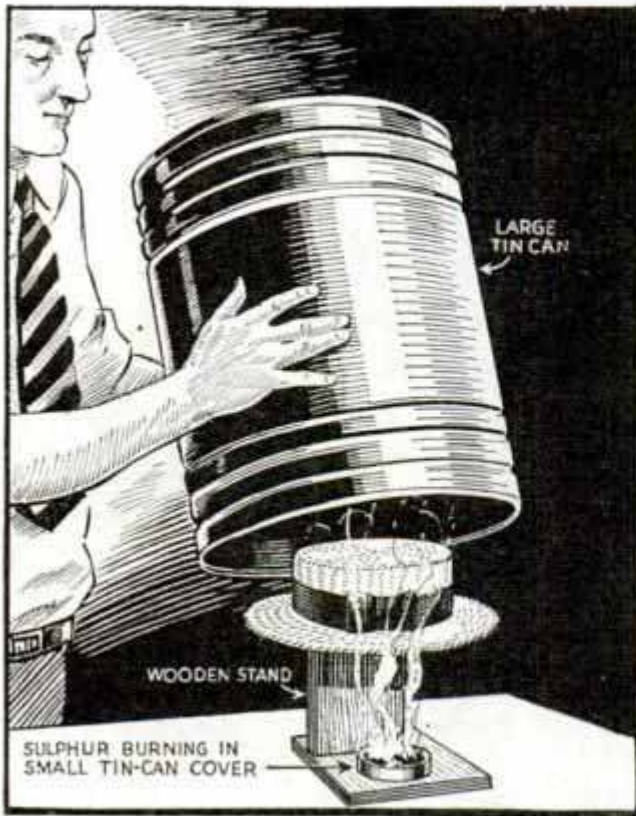
Discolored Straw Hat Bleached by Fumes from Flowers of Sulphur Confined under a Can
