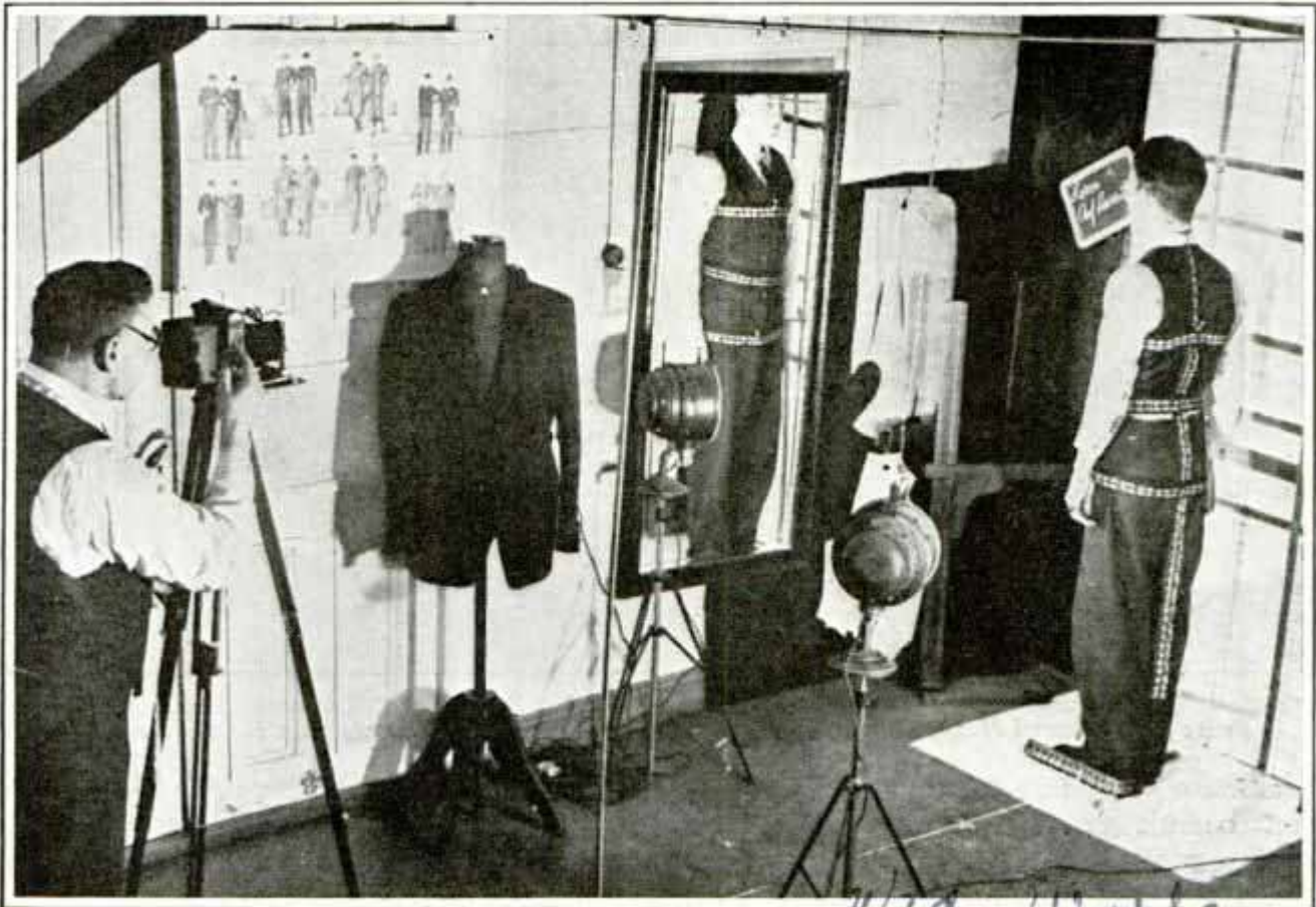
Wide World Taking Measurements for Suit Is Made Easy by Using Small Camera; Note Tapeline Attached to the Customer as He Stands Before Chart; Camera Records Measurements and Posture Quickly
