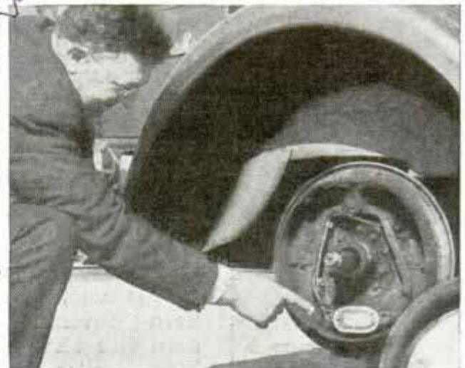
Pointing to Magnet Which Sets Brakes When Brake Pedal Releases Battery Current
