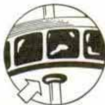
As nail punctures tube note how adhesive gum clings to nail, sealing puncture on inside.
