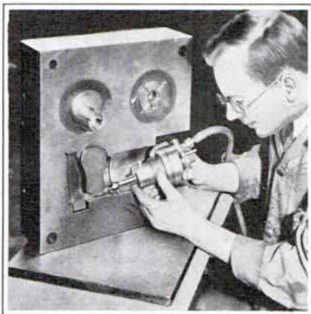
Lightweight Grinder in Use; Its High Speed Makes It Efficient on Many Jobs
