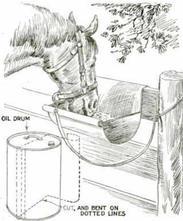
Feed Boxes That Can Be Moved Where Needed Are Made Easily from Small Oil Drums
