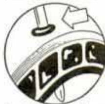
As nail is withdrawn note how gum clings to nail, sealing tube on outside.
