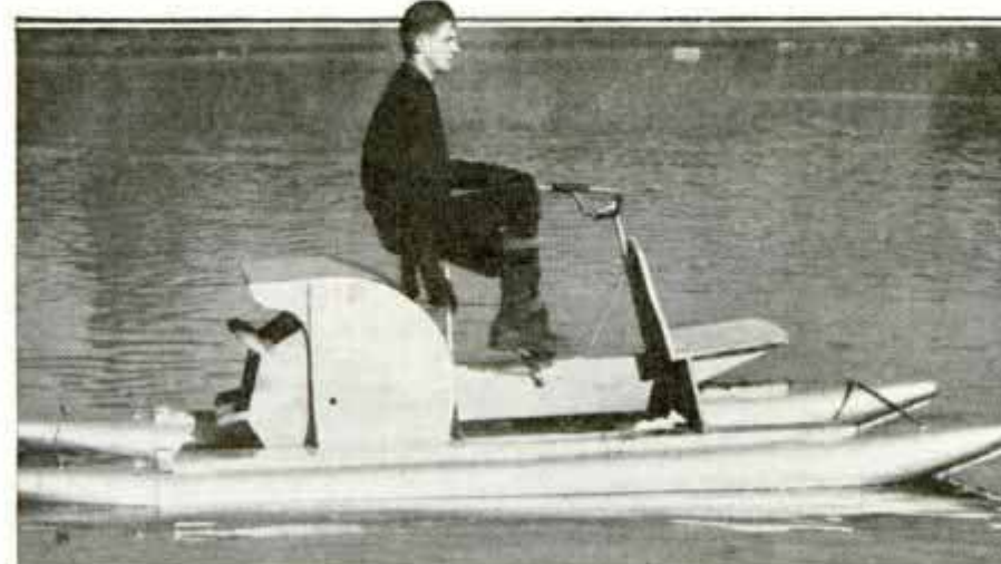
Pontoons Replace Wheels on This Water Cycle; a Speed of Ten Miles per Hour Is Possible by Pedaling the Craft Like a Bicycle
