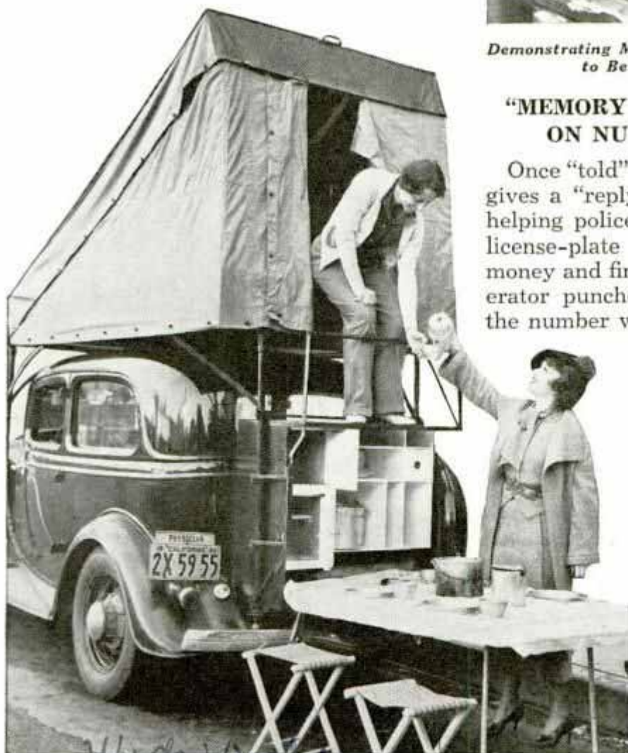
Camping Outfit for the Motorist Which Includes a Folding Tent, Carried on Top of the Car, and Collapsible Chairs and Table
