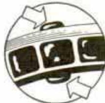
Puncture plugged with rubber rivet. Bulkhead holds plastic material in place... hole disappears.
