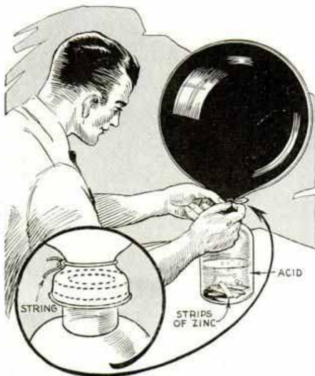
Toy Balloons Inflated with Hydrogen Gas Generated by Dropping Strips of Zinc into Muriatic Acid
