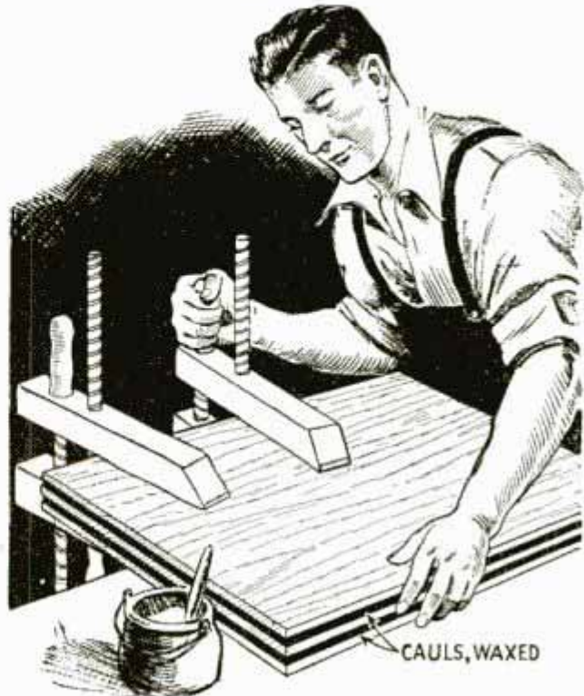
Cauls Impregnated with Wax Are Handy When Clamping Up Several Pieces of Veneer Work
