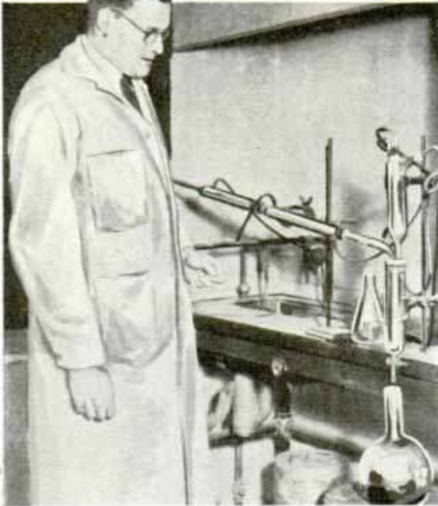
Apparatus Used for Distilling Sagebrush; the Weed Yields Valuable Products
