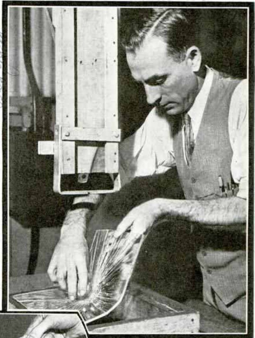
Clearste Demonstration of New Safety Glass; Right, Showing Effect of Steel Ball Dropped on the Glass; Below, Sheet of Glass under Load Has Appearance of a Net
