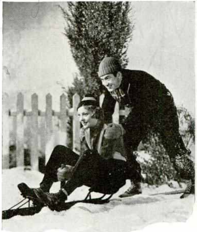
Snowplane Consisting of Single Runner with Saddle and Handle Bars; It Is Steered by Bending Body
