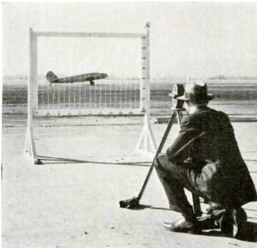
Using Movie Camera to Take Pictures through Grid of Landing Airplane, the Photographs Aiding in Computing the Plane's Speed
