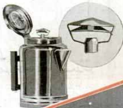
Below, Attachment for Coffee Percolator Protects Glass Top by Deflecting the Hot Liquid Downward; the Device Also Spreads the Water Evenly over Coffee to Speed Up Percolation
