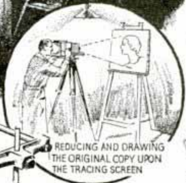
Sketches Show How Projector-Camera Is Used for Enlarging Photographs or Drawings
