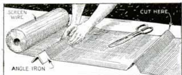
Screen Wire Creased over Edge of Angle Iron Is Cut Readily without Waste
