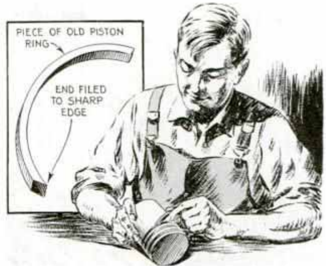
Broken Ring Beveled at One End Provides Scraper for Cleaning Ring Grooves in Piston
