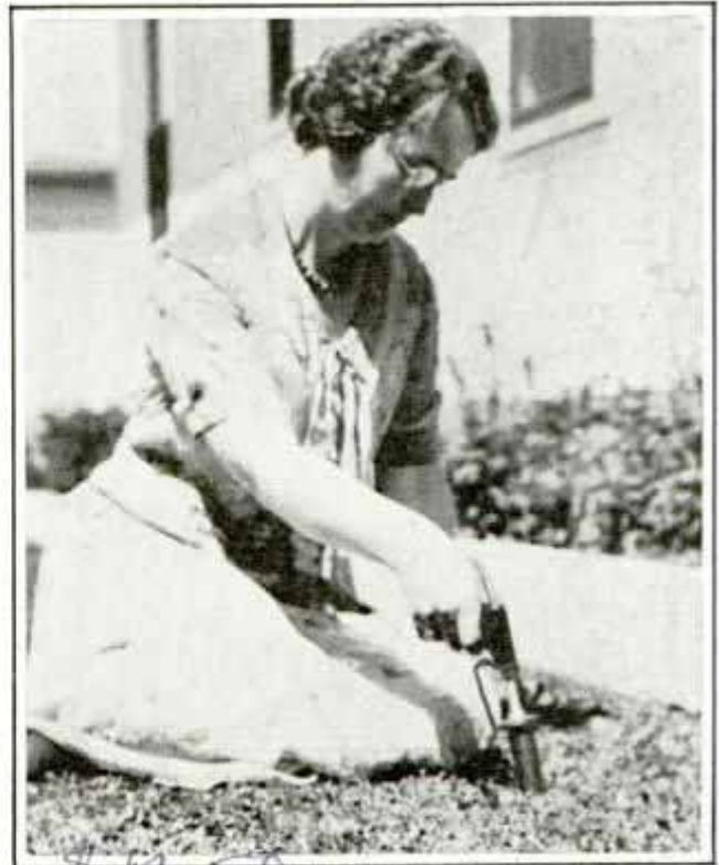
Operating an Electric Pistol Which Burns Heart of Weed When the Trigger Is Pressed the surrounding grass is not harmed when the weed in the lawn is killed.
