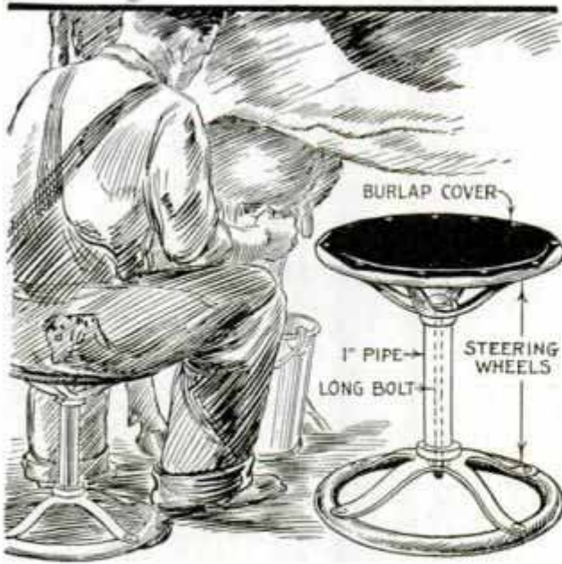
Fastened Together by a Bolt and Pipe Spacer, This Milk Stool Is Light and Rigid
