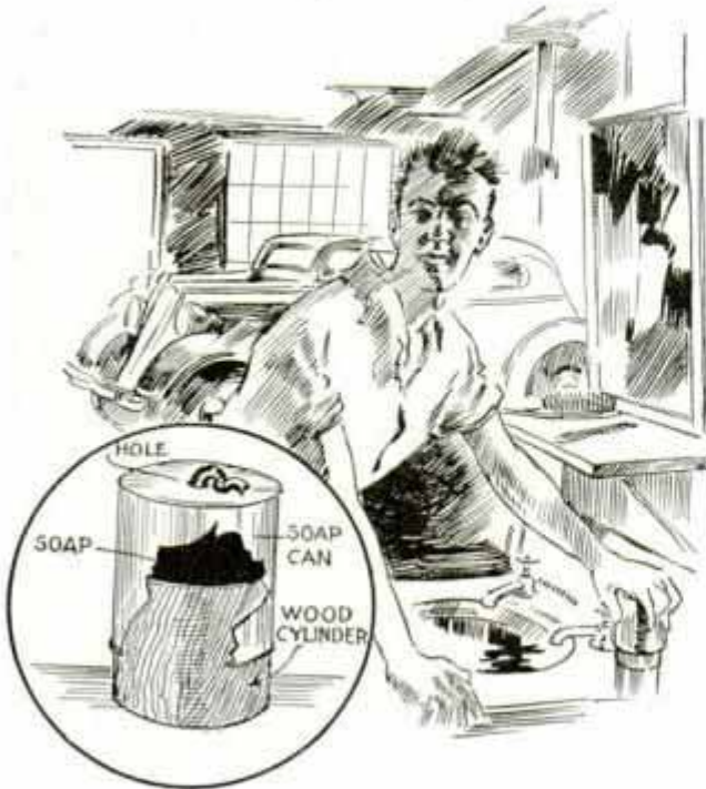
Mechanics' Paste Soap Dispenser Made by Fitting Wood Cylinder into Opened End of Can
