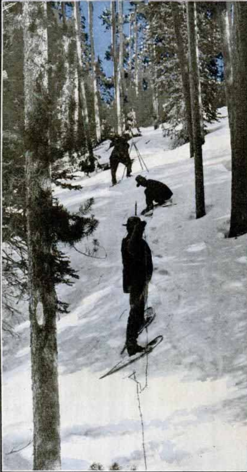
Running a Base Line in Connection with Snow-Measurement Work in National Forest in Colorado
