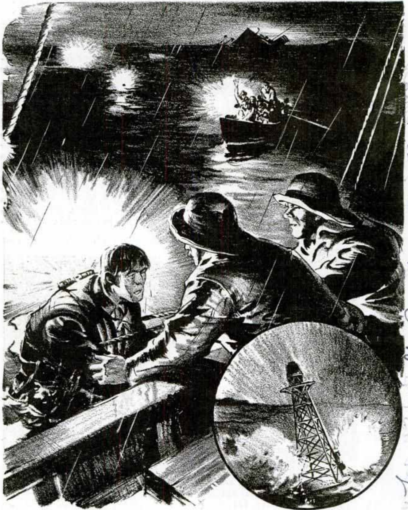
Night Rescues at Sea May Be Facilitated with the Aid of an Automatic Light Recently Designed for Life Jackets, Buoys and Lifeboats; This Light Flares Up as Soon as It Comes in Contact with the Water, Marking the Location of Survivors in the Confusion of Shipwrecks at Night; the Light Is Operated by Electrolysis, the Water Serving as an Activating Agent to Generate a Current from the Electrical Potentials of Separated Bars of Carbon and Zinc in the Light; Small Lights Are Used for Life Jackets, and Larger Ones for Buoys and Boats
