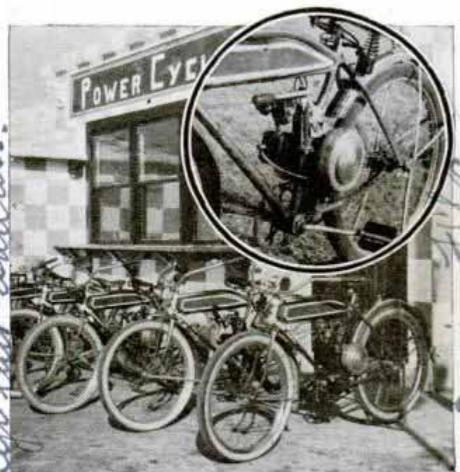
Bicycles with Motors Parked in Front of Rental Business; Inset, Location of Motor
