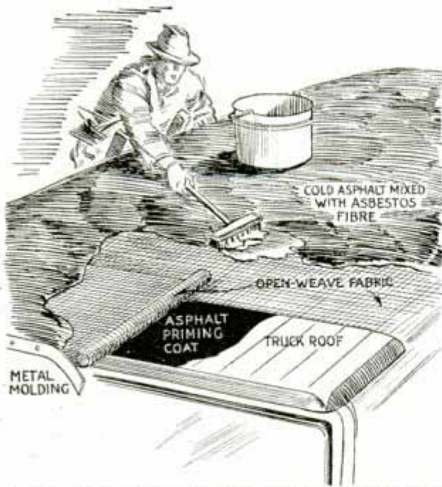
Layers of Asphalt and Fabric Make a Truck Roof That Is Flexible and Waterproof
