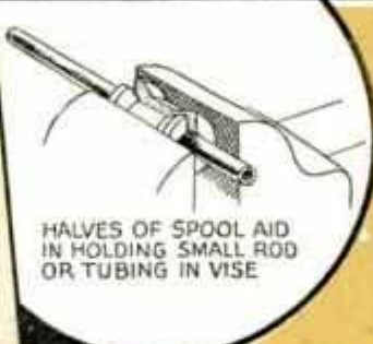
SMALL SPOOLS DIPPED IN GLUE AND COATED WITH ABRASIVE CAN BE USED FOR SANDING DELICATE SCROLL WORK
