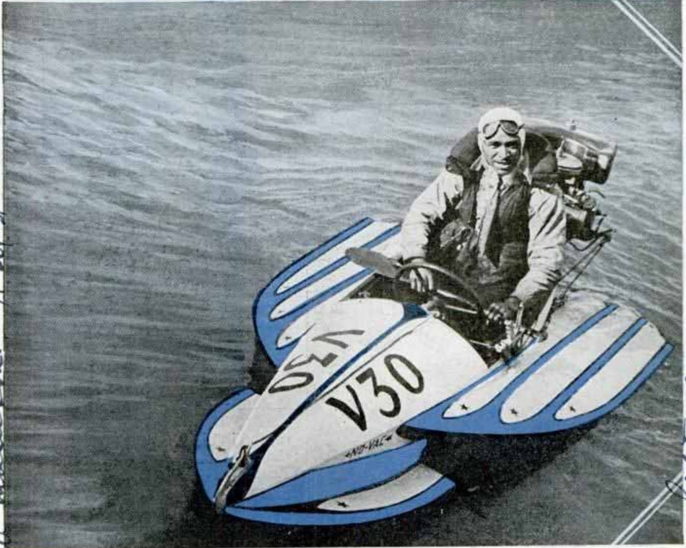
This View of the "No-Vac" Shows How Thoroughly It Has Been Streamlined; Note How the Planing Surfaces Have Been Designed to Resemble an Airplane Wing Section
