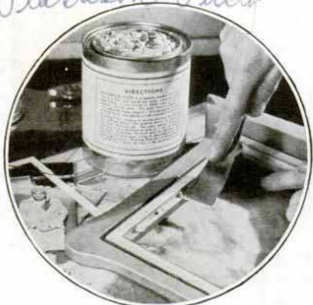
Illustrating the Ease with Which Rubber Putty Can Be Applied; It Forms Perfect Seal
