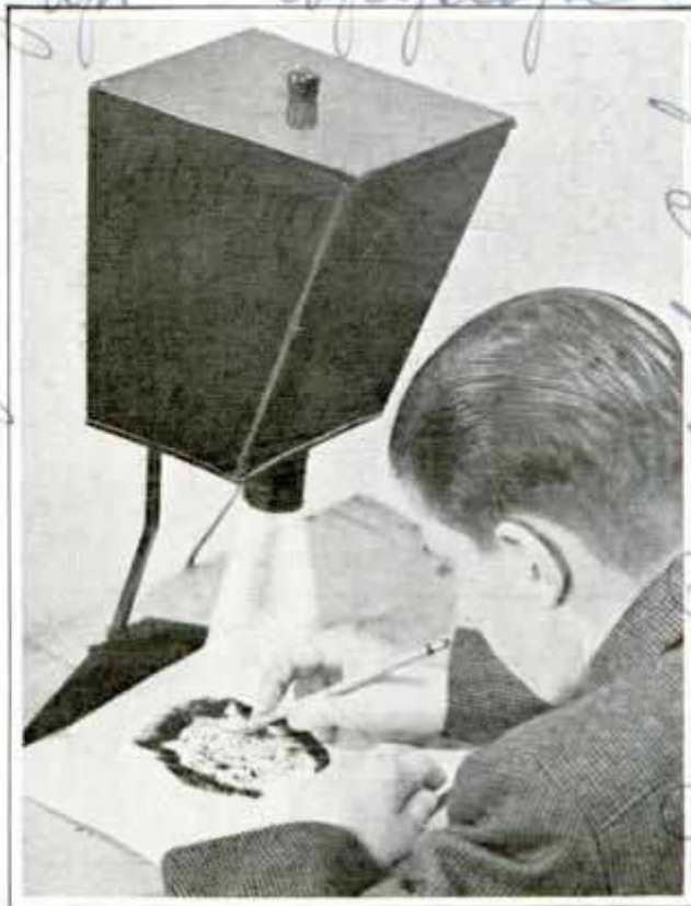
Tracing a Picture Projected on Paper by the Inexpensive Reflector Machine
