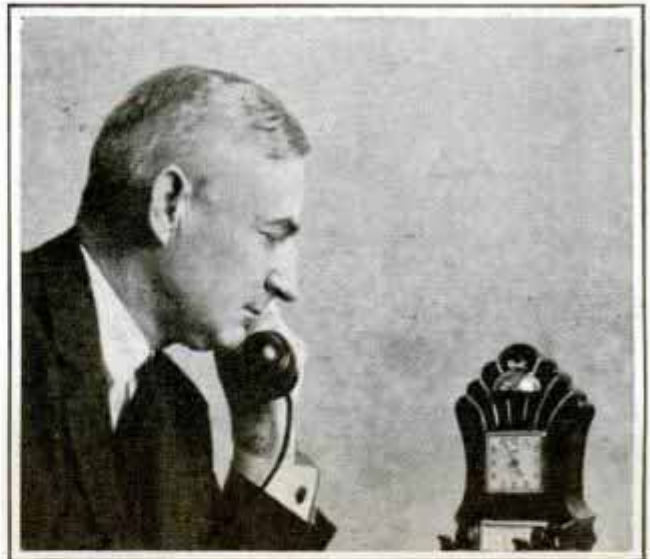
Telephone Holder Equipped with an Electric Light, an Electric Clock and a Calendar
