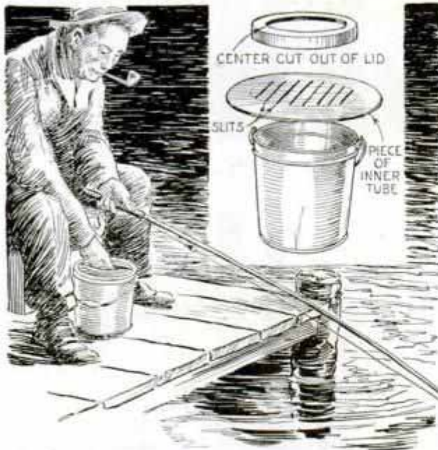
Rubber Cover on Minnow Pail Shades the Bait and Permits the Hand to Be Inserted Readily
