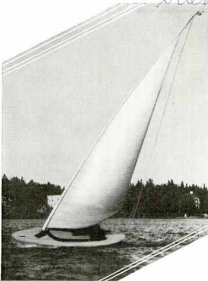
Two Views of Revolving Mast Boat; Odd Design of Sail Eliminates Boom and Stays; Sail Area Is Twice That of Conventional Sail, Resulting in a Considerable Increase in Speed
