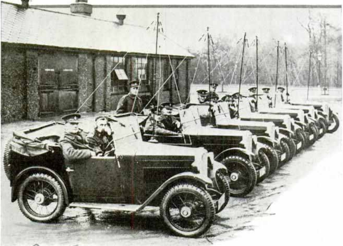
Radio Cars Equipped with High Aerial Masts Which Were Used to Maintain Communication between Various Military Units Policing the Saar During the Recent Plebiscite
