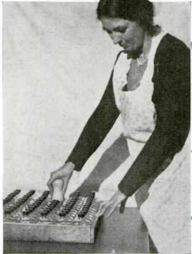
Wooden Handle with Composition Band in Hole in End Used for Tightening Screw Caps
