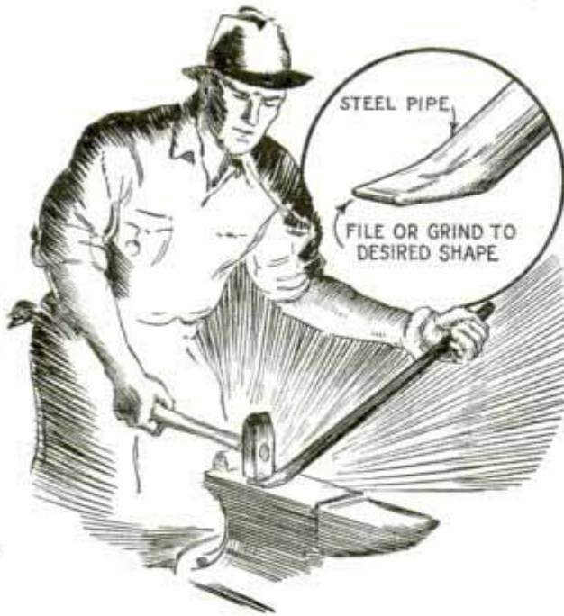
End of Steel Pipe Heated and Flattened to Make Lightweight Crowbar
