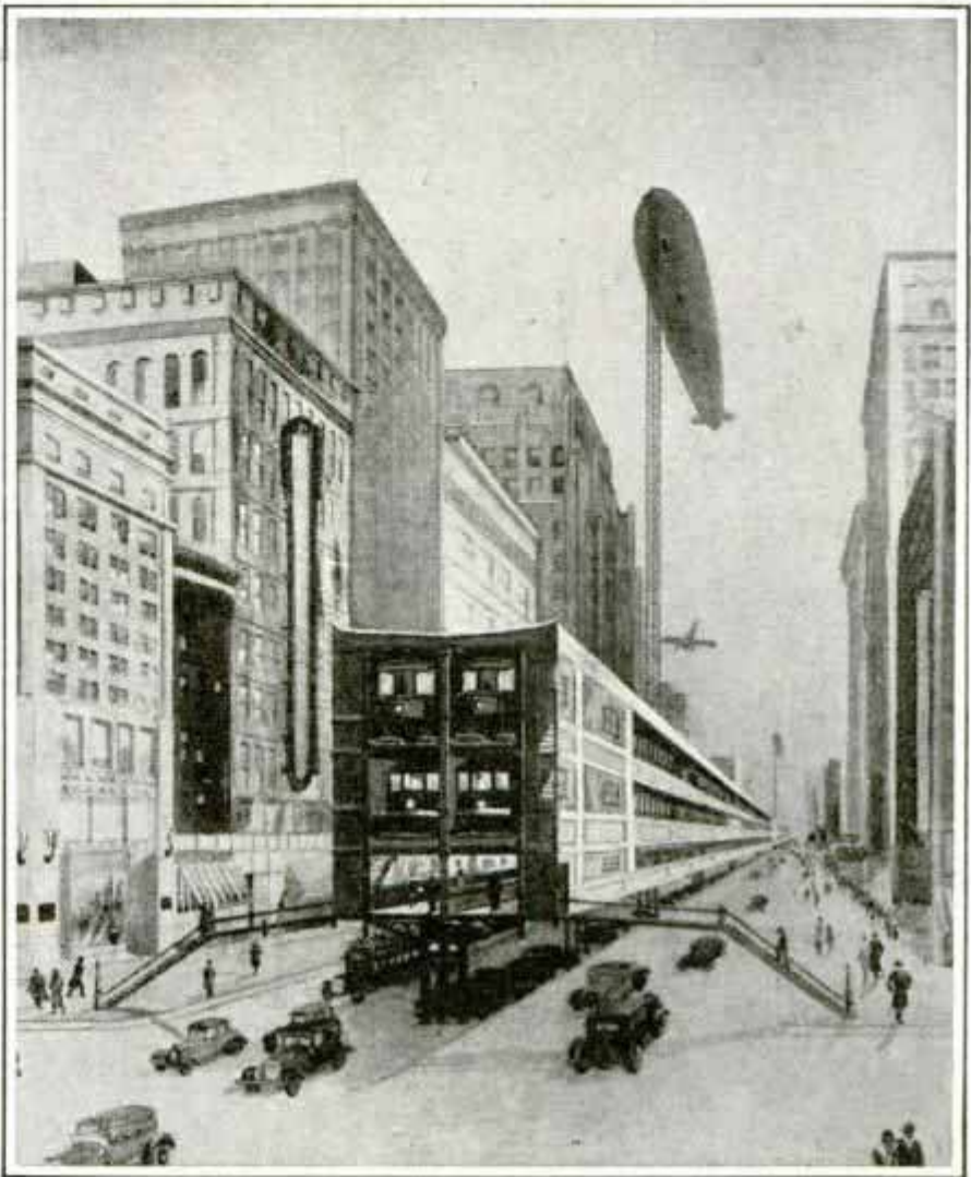
Sketch of Four-Deck Roadway as It Might Appear in City Street; Note Ramps Leading from Sidewalk to the Pedestrian Level
