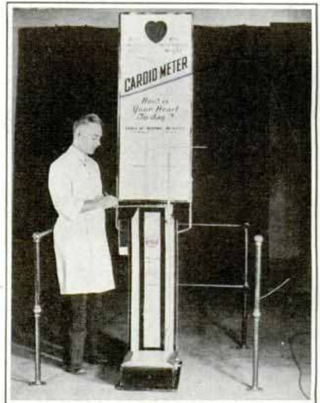
Scale Which Indicates Rate and Intensity of Heart Beats at Same Time It Registers Weight
