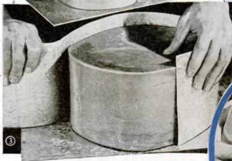
Above, after the molding compound has cooled to a stiff, jellylike consistency, the sheet-metal wall is removed. Right, when removing an intricate model from a mold, it is sometimes necessary to cut the mold with a knife, at points where the cut will meet the corners of the model
