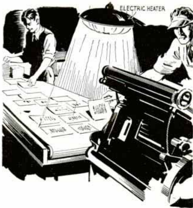
Ink on Printed Matter Quickly Dried by Passing It under Electric Heater
