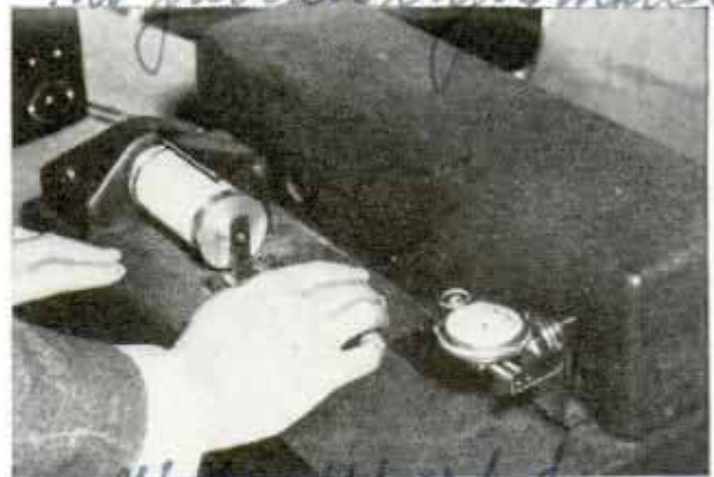
Testing Watch on Latest Machine; Dots on Cylinder at Left Show Whether It Is Accurate
