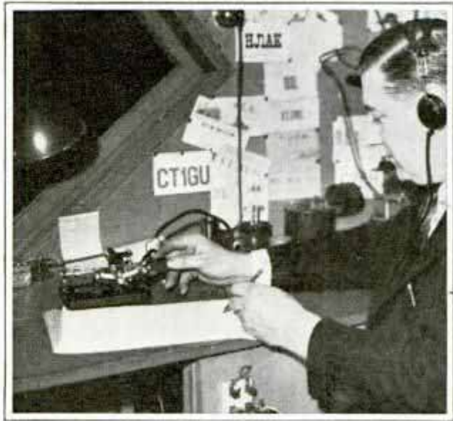
High-Speed Key Designed to Increase Rate of Transmission of Radio Code
