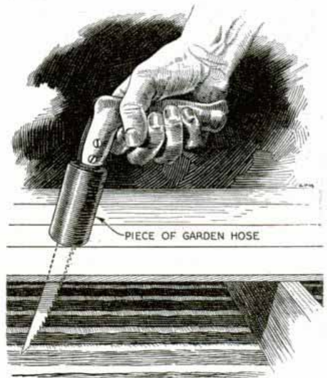
Piece of Garden Hose Slipped over Blade of Keyhole Saw Serves as Stop to Limit Stroke
