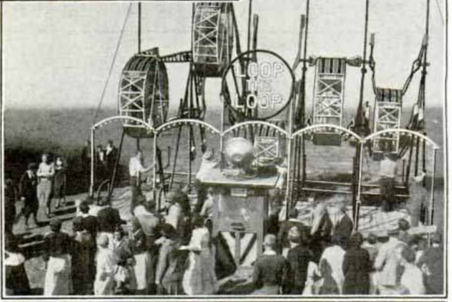
Top and Right, Latest Amusement Ride; Cages Remain Upright Even While Looping-the-Loop under Momentum Provided by Rider
