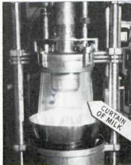
Above, Apparatus Used to Revive Frozen Limbs by Alternating a Vacuum and Normal Pressure; Below, Irradiating Milk; Note Gas-Tight Film of Water between Carbon Arc and Milk
