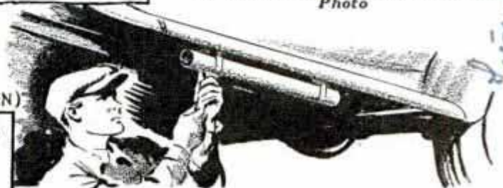
Capacity-Type Auto Antenna Made from Copper Drain Pipe, or Similar Material, May Be Easily Mounted on Stand-Off Insulators under Car
