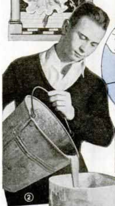
The model is placed on a sheet of tin and a tin retaining wall holds the melted molding compound, which is poured over the model
