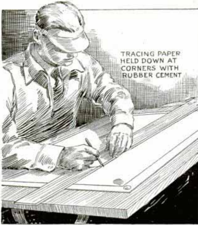
Tracing Paper Fastened over Drawing with Rubber Cement Instead of Thumb Tacks
