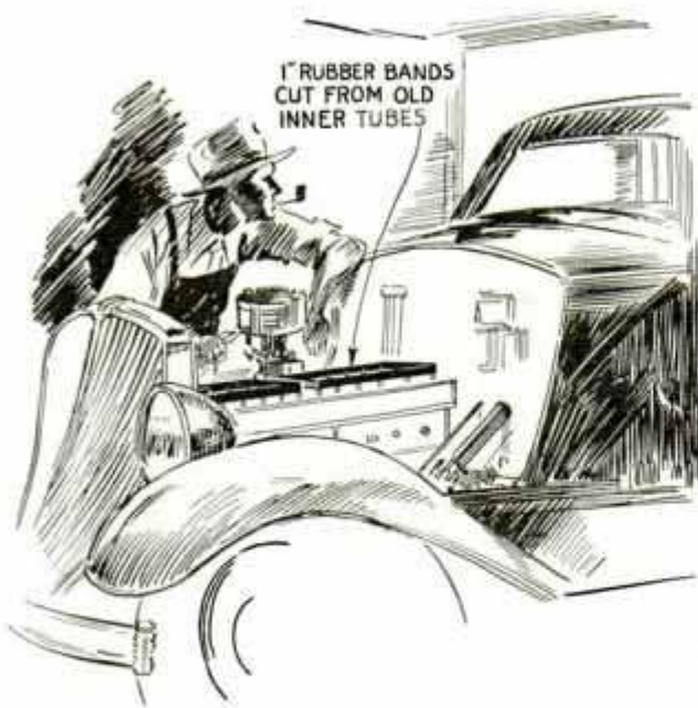
Wide Rubber Bands Stretched over Cylinder-Head Bolts Protect Hands When Working on Motor
