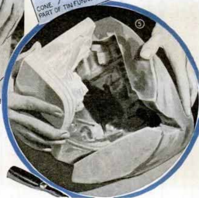
Above, after the molding compound has cooled to a stiff, jellylike consistency, the sheet-metal wall is removed. Right, when removing an intricate model from a mold, it is sometimes necessary to cut the mold with a knife, at points where the cut will meet the corners of the model
