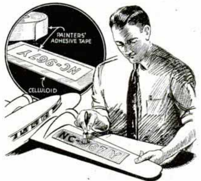
Stencil Made of Masking Tape Aids in Painting Letters or Figures on Models
