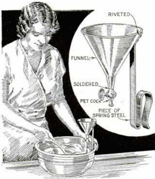
Clamped to a Mixing Bowl, This Device Adds Liquids to Mixtures a Drop at a Time
