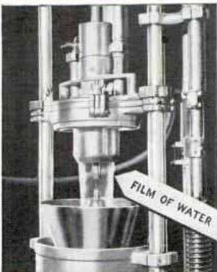
Above, Apparatus Used to Revive Frozen Limbs by Alternating a Vacuum and Normal Pressure; Below, Irradiating Milk; Note Gas-Tight Film of Water between Carbon Arc and Milk
