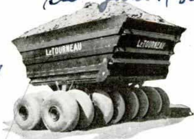
Sixteen Doughnut Tires Support This "Buggy" Which Has a Capacity of Thirty Cubic Yards
