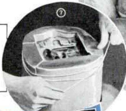
Greasing the inside surface of the mold with raw linseed oil to prevent plaster from sticking
