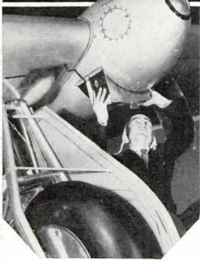
Top, Photo-Diagram of Camera Plane Showing Location of Camera in One Wing; Bottom, Installing Film Magazine in Camera Compartment Preparatory to Taking Aerial Pictures
