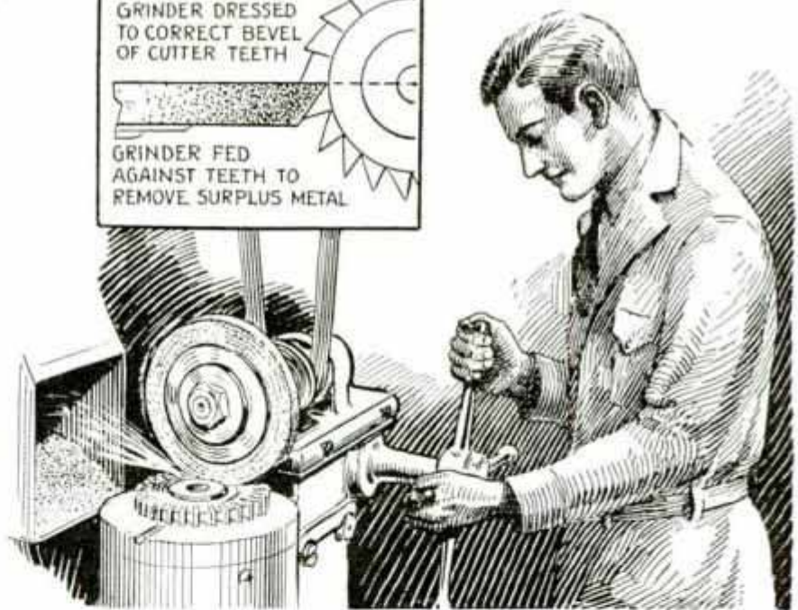
Grinding the necessary clearance on the cutter sides between the teeth and the center boss. This is done readily on a rotary-table surface grinder, which is fitted with a magnetic chuck
