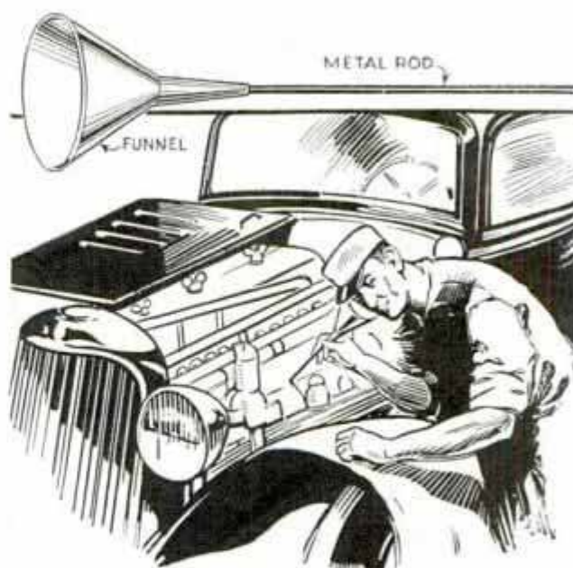
Motor-Knock Sounder Assists in Locating Knocks Made by Worn Bearings, Pistons, and Other Parts
