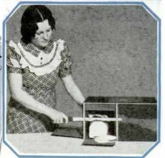
Above, Bread Box That Aids in Slicing; Loaf Is Pushed Against Adjustable Flange on Door and Knife Is Passed Through Guide Slots for Slicing; Meat or Cheese Also Can Be Sliced on This Handy Device
