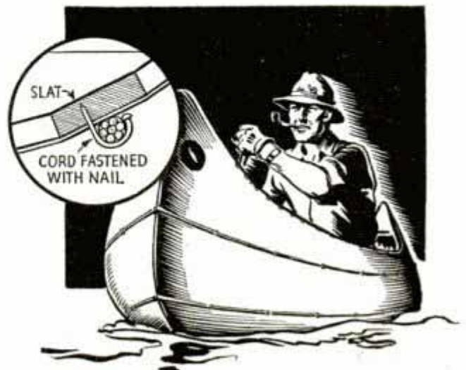
Sash Cord Attached to Sides and Bottom of Canoe Protects Canvas Covering against Wear
