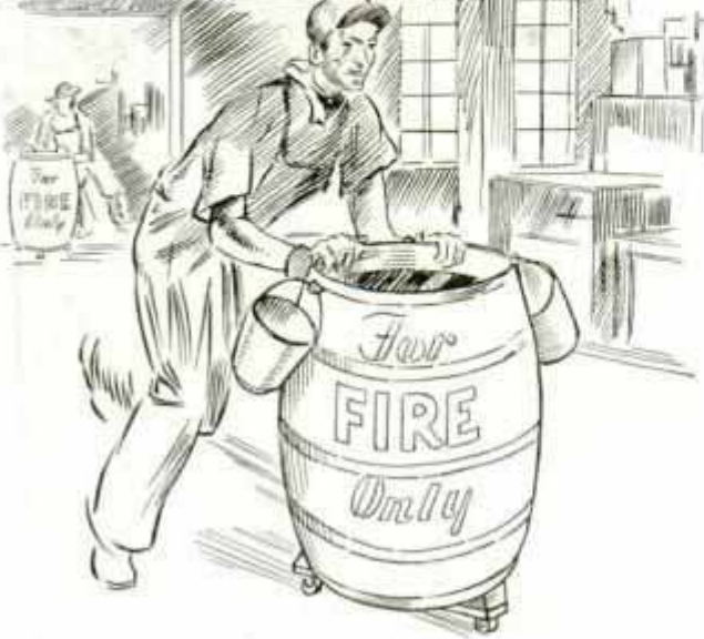
Set on a Frame Fitted with Casters, Fire Barrels Are Readily Pushed to Any Part of a Building
