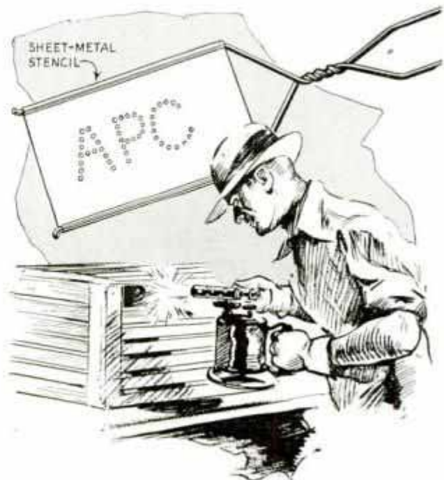
Owners' Initials Burned on Shipping Crates with Blowtorch and a Sheet-Metal Stencil
