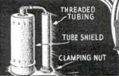
Above, Threaded Brass Tubing Makes Good Shield for Screen-Grid Tube Lead
