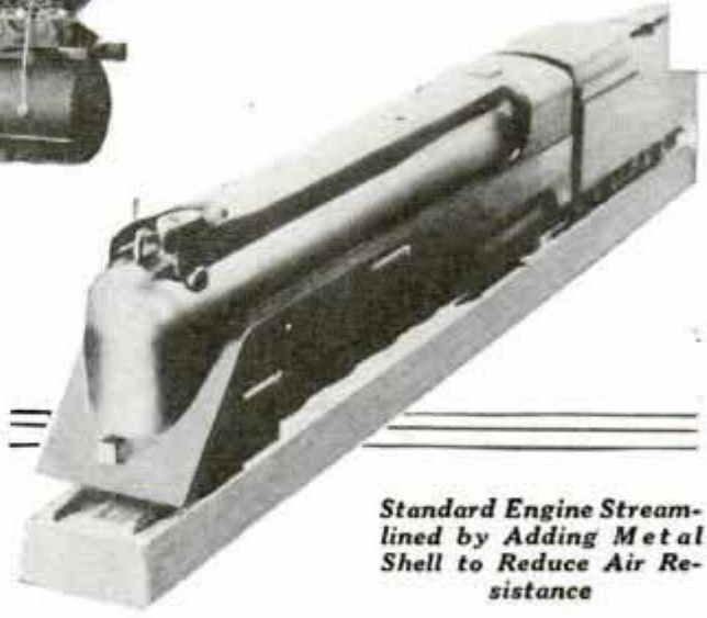
Model Locomotive and Its Upside Down "Mirror Image" Ready to Enter Wind Tunnel for Tests
