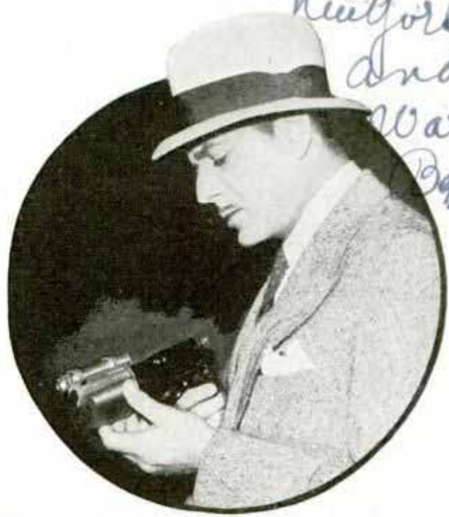
Gun with Spotlight Attached to Barrel to Illuminate Target When Shooting at Night
