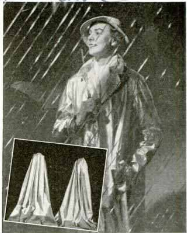
D1567 Raincoat and Samples of Fabric Treated with "Bakelite" Resinoid Material to Make Them Waterproof
