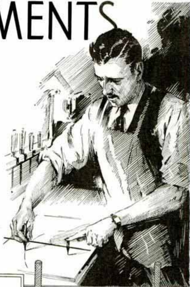
MACHINISTS' BEAM TRAMMEL USED IN SCRIBING CIRCLES, SEGMENTS AND IN TRANSFERRING MEASUREMENTS
