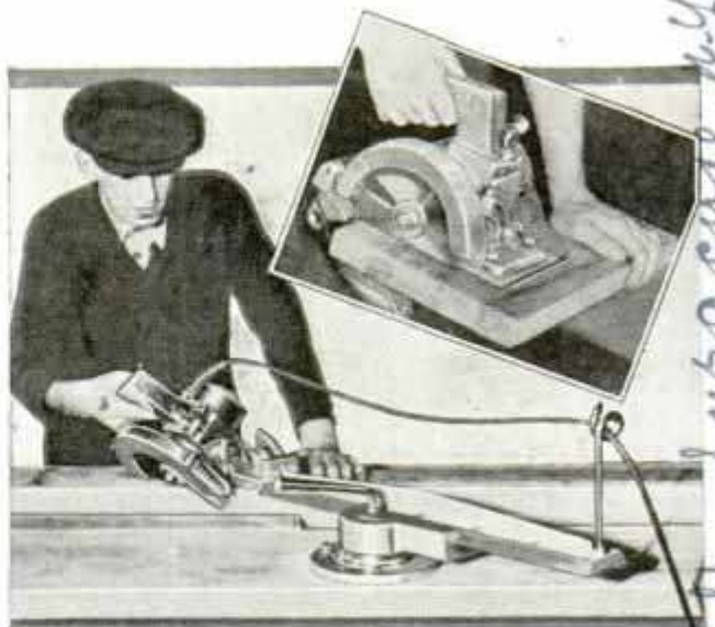
Portable Saw Being Used as Bench Tool by Addition of a Simple Table Attachment
