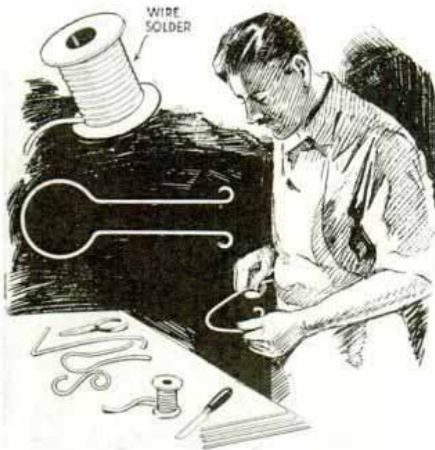
Patterns Made from Wire Solder Save Time When Bending Heavy Wire for Certain Jobs
