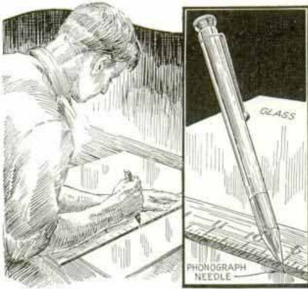
Steel Phonograph Needle Held in Automatic Pencil Serves as Emergency Glass Cutter
