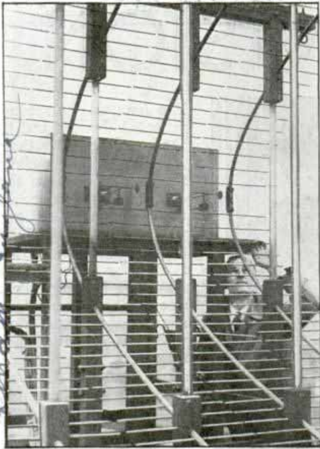
Marconi Micro-Wave Aerial System with Parabolic Reflectors; It Is Used in Experimental Work
