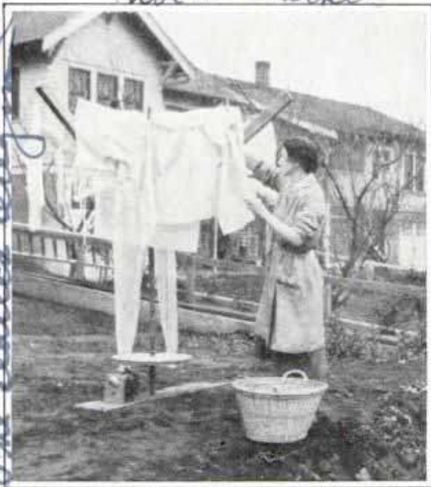
Clothesline Which Is Rotated by a Small Motor, the Motion Resulting in Rapid Drying
