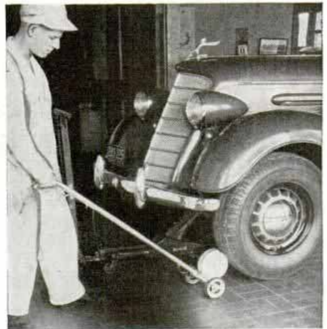
Testing Wheels for Shimmy and Wobble; Easily Operated Spinner Eliminates Road Test
