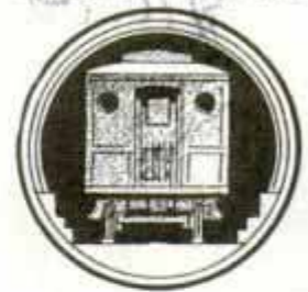
HUDSON AND MANHATTAN TUNNEL DIAMETER 16 FT. 7 INS.
