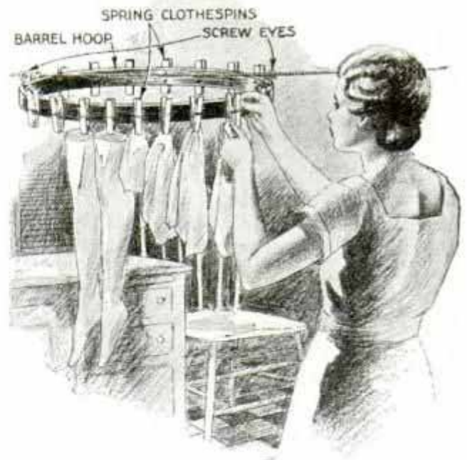
Reel Made from Barrel Hoop for Drying Clothes inside House Takes Very Little Space
