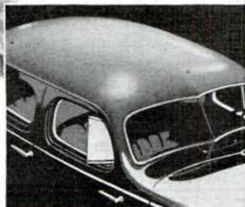
This is the way the new Fisher "Turret Top" looks—a single seamless sheet of tough drawn steel, steel reinforced with steel like a battleship turret
