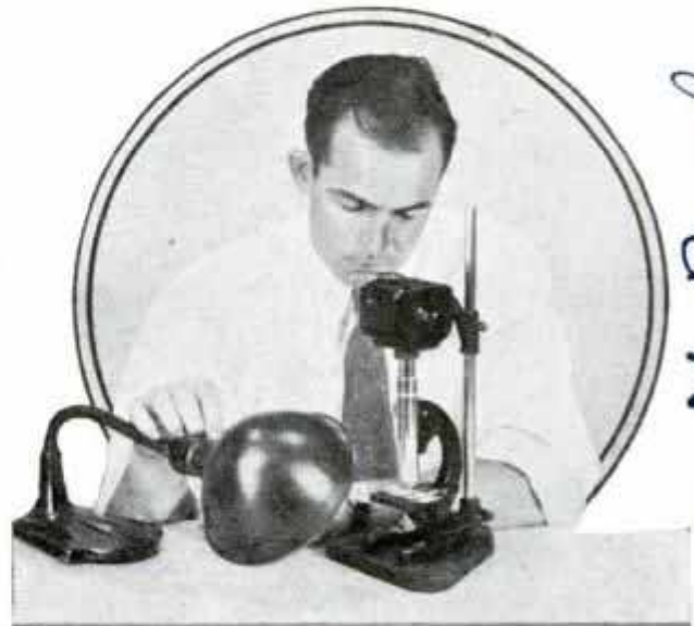
Equipment for Photographing Objects under Microscope; Its Operation Is Simple
