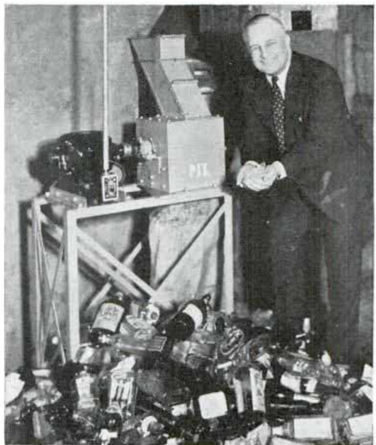
Bottle Breaker Which "Digests" Glass Containers, the Broken Glassware Finding a Ready Market
