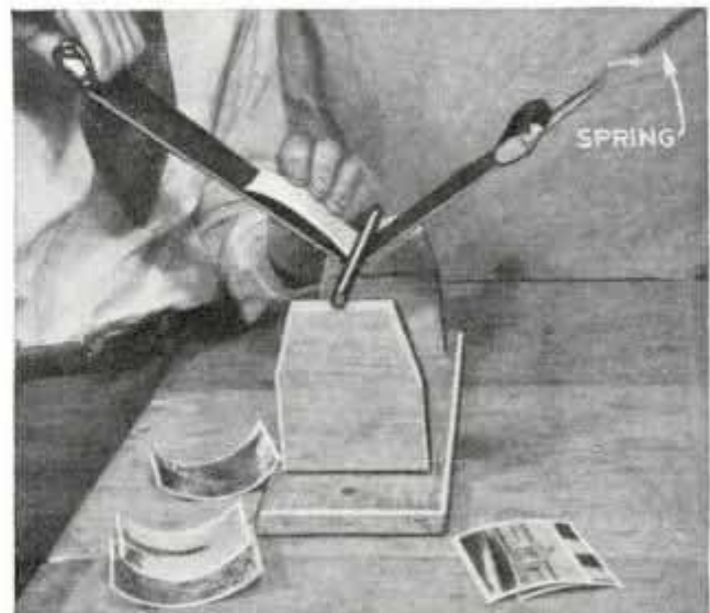
Photo Prints Straightened by Pulling Them under Rod with Strip of Soft Leather
