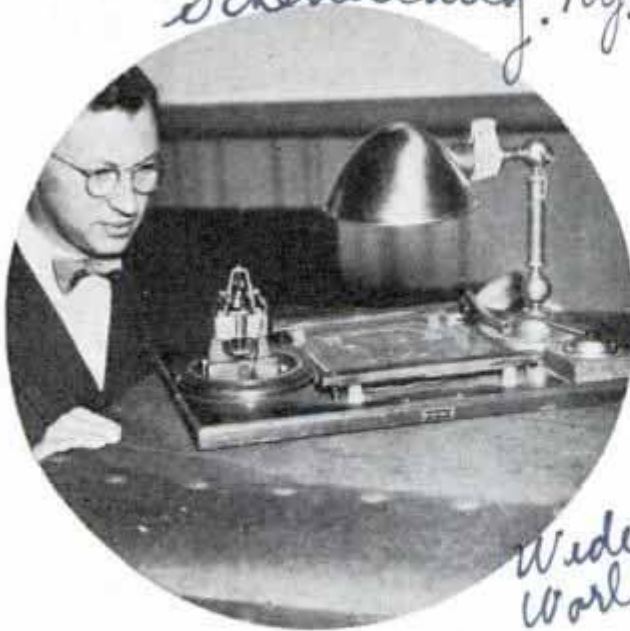
Small Motor at Left Is Driven by Energy Taken from Sunlight by Photo-Electric Cells
