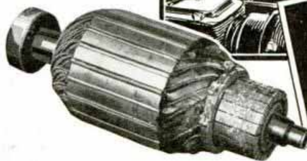
Corroded and frayed battery cables and terminal posts resist passage of current and may cause generator to burn out. Evidence of solder on the commutator indicates over-heating caused by resistance in charging circuit
