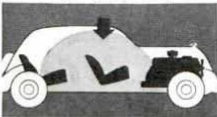
Engine is moved forward, as first introduced by famous "Airflow" cars.
