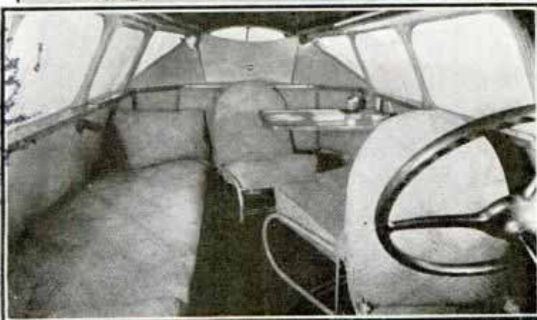
Bottom, Interior Which Has Five Inches More Headroom Than Conventional Car; Note Rear Seat Has Been Moved to Side and Extended for Sleeping, Making Day and Night Travel Easier
