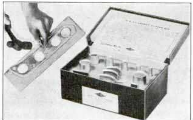
Handy Outfit for Cutting New Gaskets by Using the Old Gasket as a Pattern
