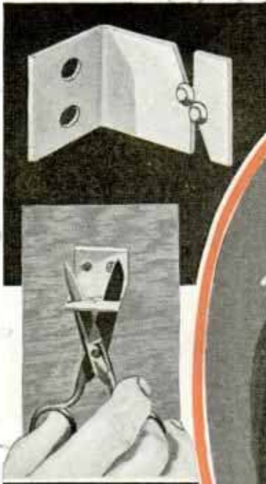
Above, Double-Acting Scissors Sharpener Designed to Eliminate Sharpening One Blade at a Time; Wall Holder Has Two Sets of Revolvable Steel Wheels; by Working the Scissors Up and Down in Holder, the Wheels Dress Each Blade Uniformly
