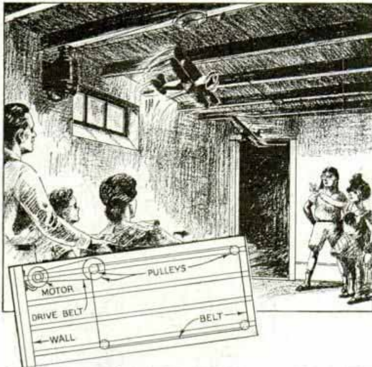
Small Model Airplanes Give Realistic Imitation of Flying When Suspended from Traveling Belt Driven by Motor
