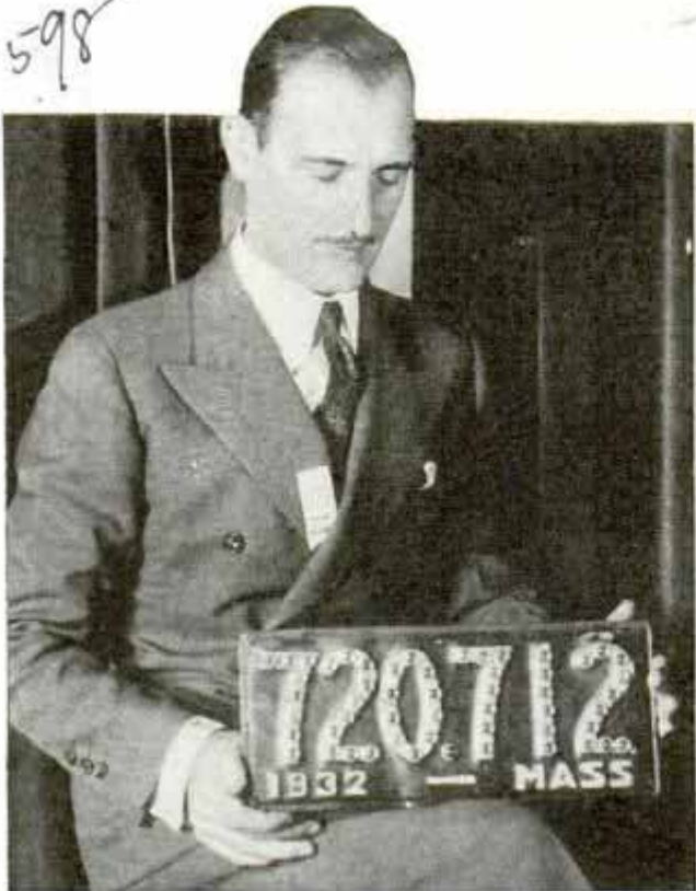
License Plate with Reflectors Set in the Numbers, Making It Easy to Read at Night
