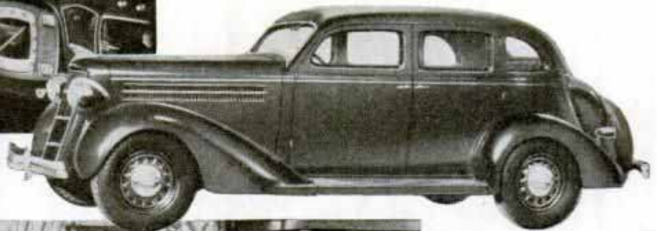
Above, the Dodge Sedan, Which Improves Riding Qualities with New Front-End Suspension and Redistribution of Weight; Left, Latest Oldsmobile, Which Has All-Steel Body, Hydraulic Brakes and Oil-Distributing System with Drilled Passages That Replace Oil Pipes; Oil System Is Cast with Cylinder Block, and Water Passage Is Cast Integral with the Block
