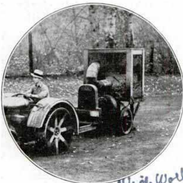
Outdoor "Vacuum Cleaner" Shown Collecting Leaves from Golf Course; It Is Tractor-Towed
