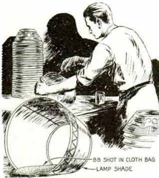
Cloth Bag Filled with Shot Holds Edges of Parchment on Lamp Shade until Glue Dries
