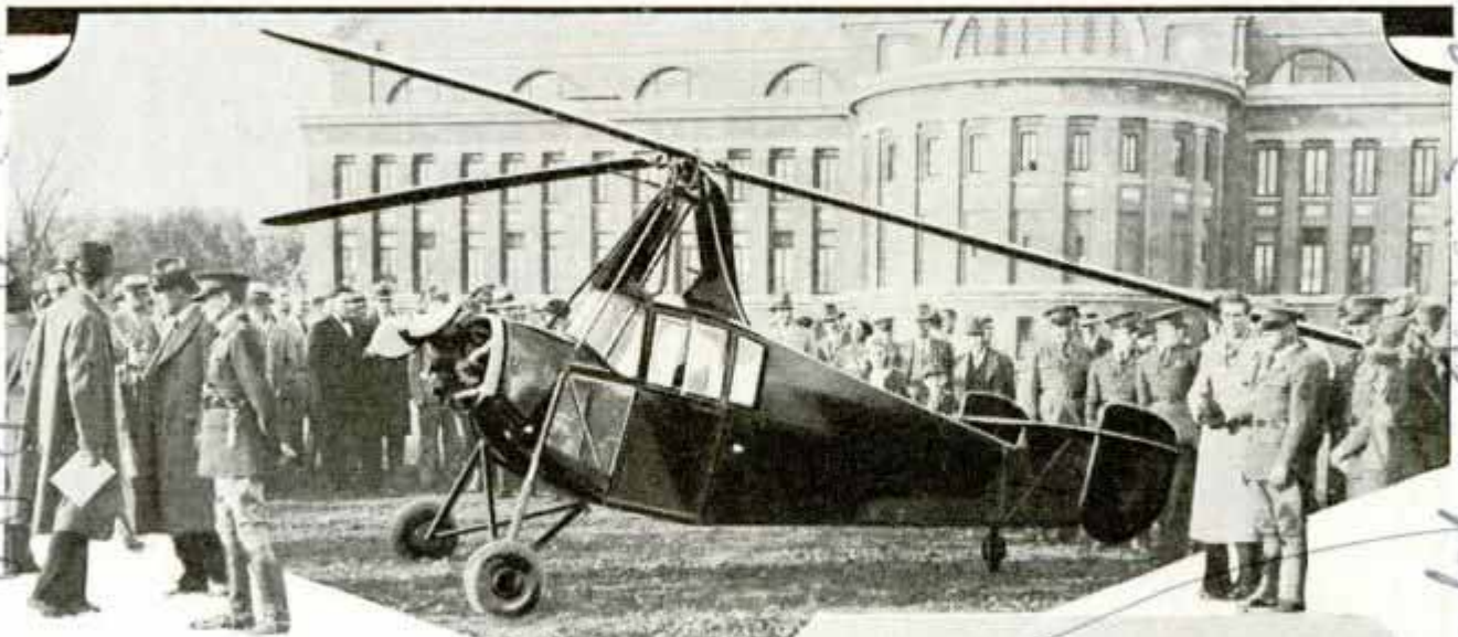
Wingless Autogiro Which Rises and Lands Almost Vertically and Can Be Parked Like a Car
