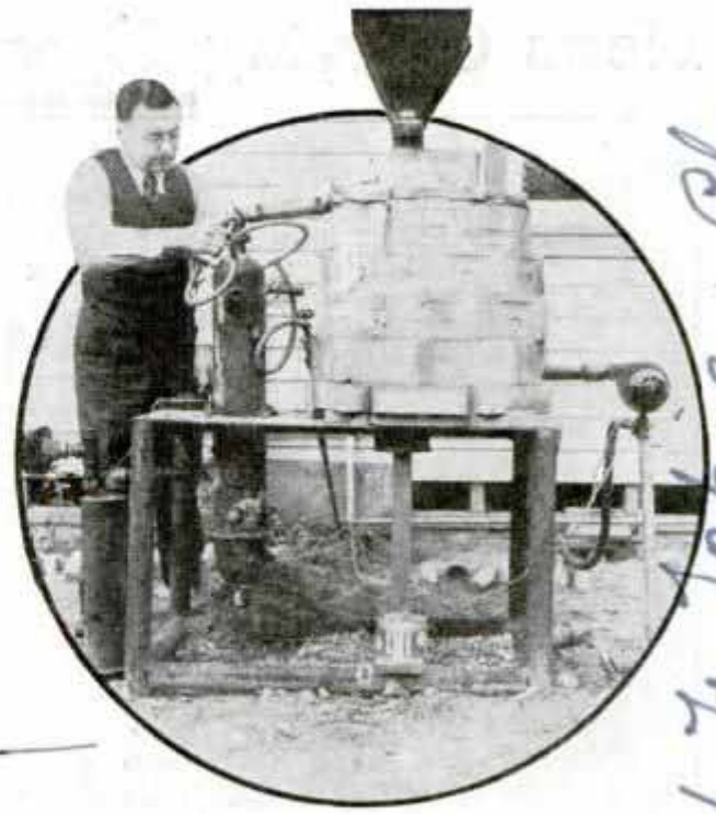
Small-Scale Plant for Taking Mercury from Ore; Its Efficiency Is Said to Be High
