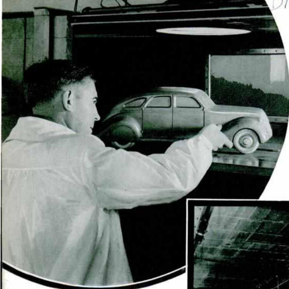
LEFT , here we see the automobile in miniature as designers and engineers seek to determine the effect of air currents on its shape; the model is shown in a wind tunnel through which the air is forced at high speed.—Courtesy DeSoto Motor Corporation.
