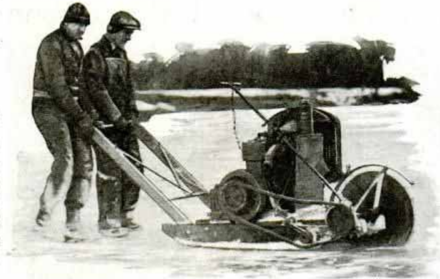
Made from an Old Wood Saw, This Ice Saw Is Mounted on Runners and Is Pushed by Two Men
