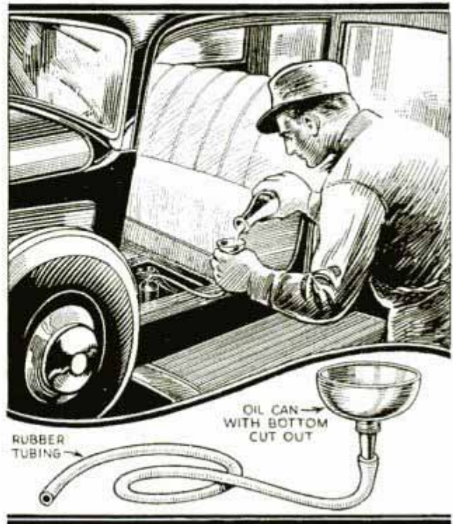
Master Cylinder of Hydraulic-Brake System Filled by Means of Rubber Tube and Funnel
