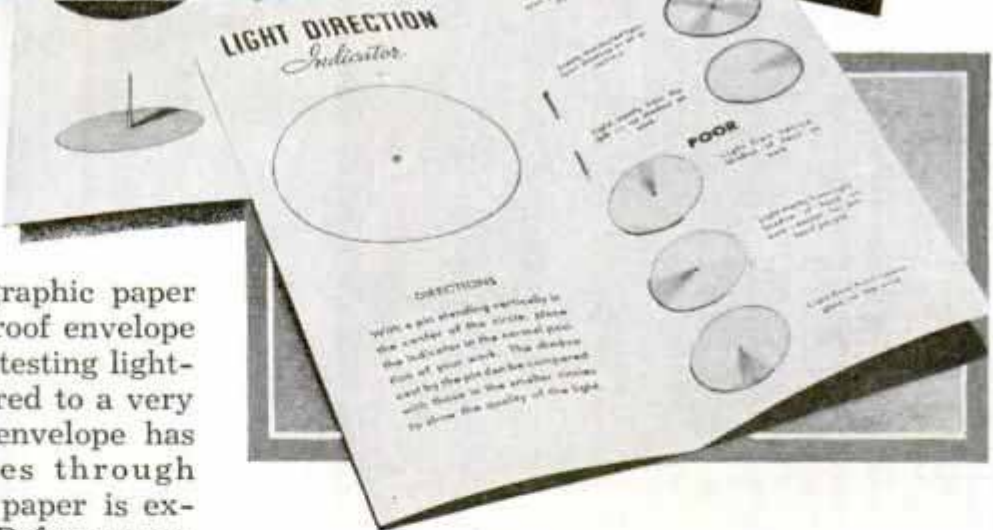
Left, Testing Intensity of Light with Sensitive Paper; Right, the Indicator; Below, Another Paper Indicator That Shows If Light Is Coming from Right Direction
