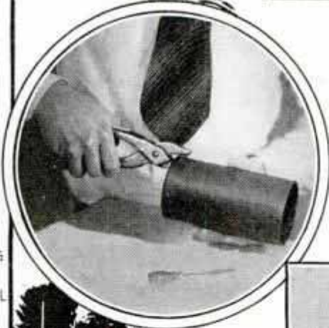
An Easily Made Mounting for Insulating Grounded-Condenser, or Resistor-Unit Shafts
