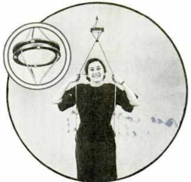
The Two Glass Disks Supporting the Girl Are Held Together by Molecular Attraction
