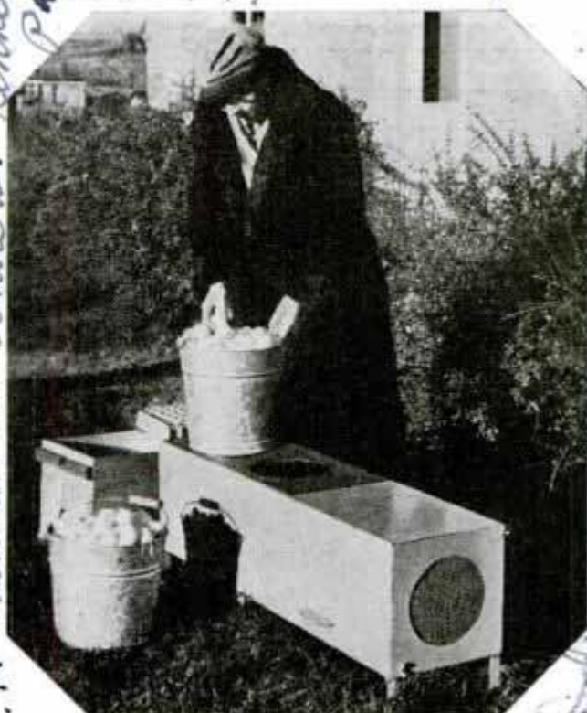
Electric Cooler Which Blows Air around Eggs in Buckets Equipped with Screened Bottoms
