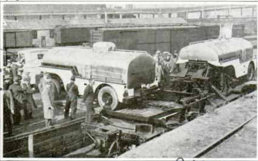
Flat Car Containing Two Turntables, Each Accommodating a Semi-Trailer Milk Tank Which Can Be Attached to a Truck
