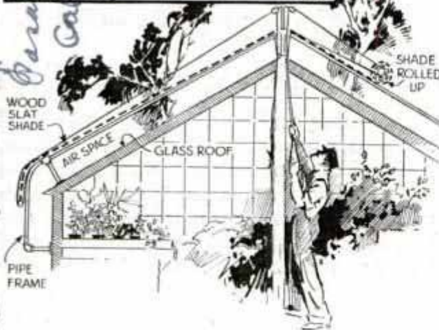
Rolling Shade Which Shelters Delicate Greenhouse Plants; Note the Pipe Framework
