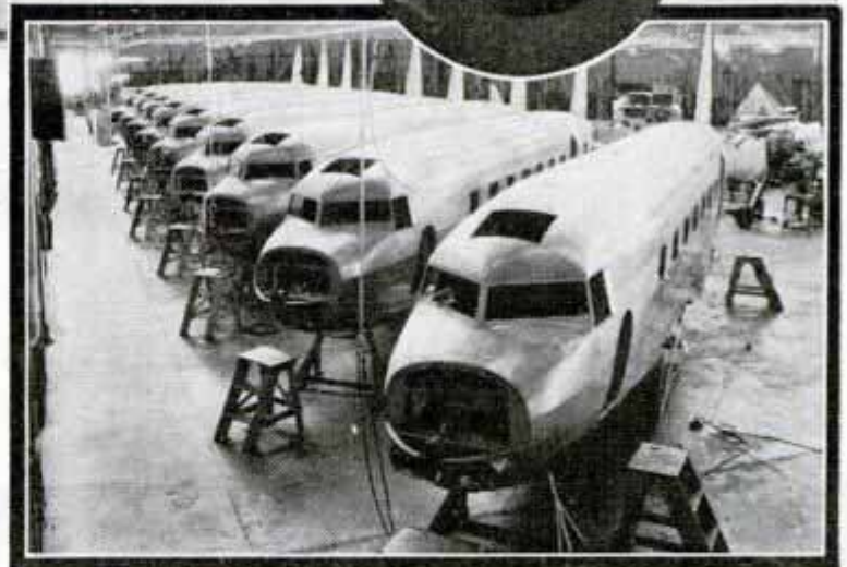
The Nose of a Douglas Transport, and Fuselage Assembly Room of Douglas Aircraft Company Factory
