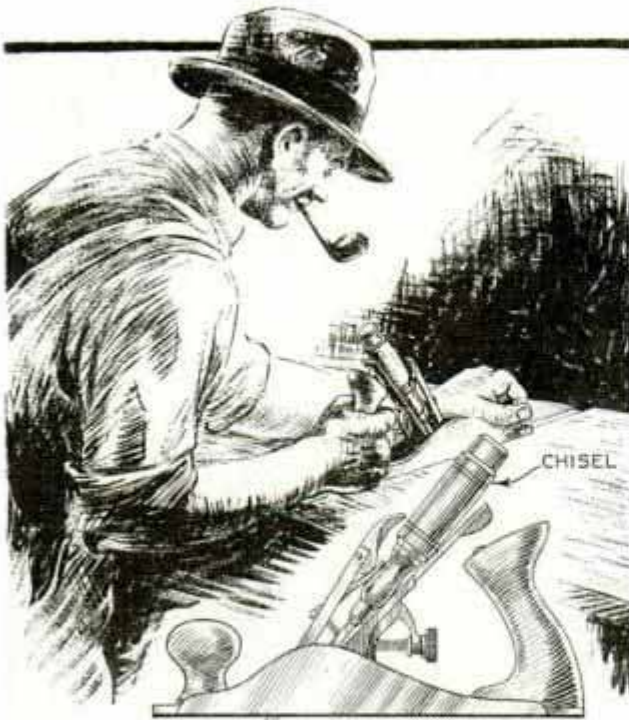
Grooves Cut with Plane in Which Wood Chisel Is Substituted for Plane Iron
