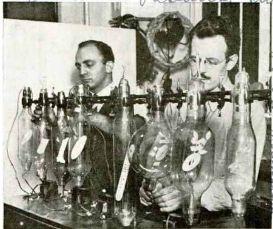
Cathode-Ray Tubes Built around Trade-Marks; Chemicals Are Used in Producing Brilliant Colors to Light the Advertising Emblems
