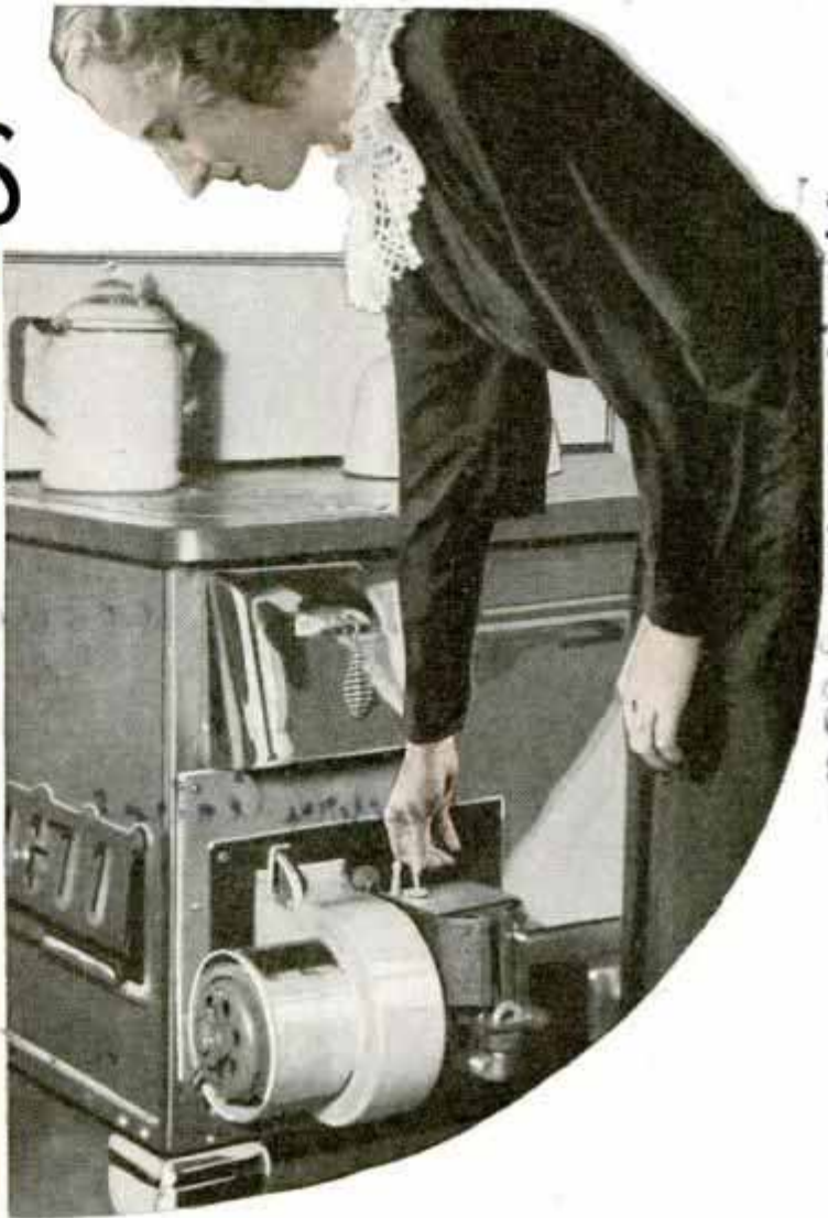
Above, Oil Burner Which Can Be Attached to Ordinary Coal Range; It Consists of a Compact Burner and a Blower Operated by a Small Electric Motor
