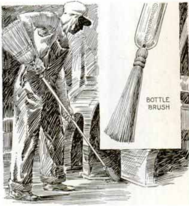
Corners and Other Tight Places Are Cleaned Quickly with Brush in End of Broom Handle
