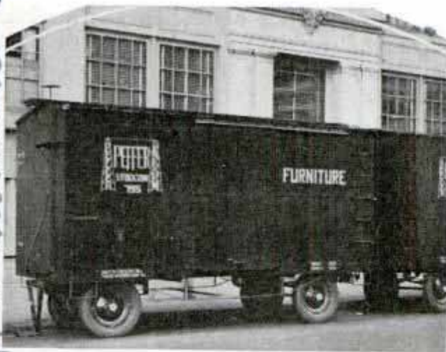
Truck Trailer Built to Resemble a Box Car and Used to Haul Furniture on Pacific Coast
