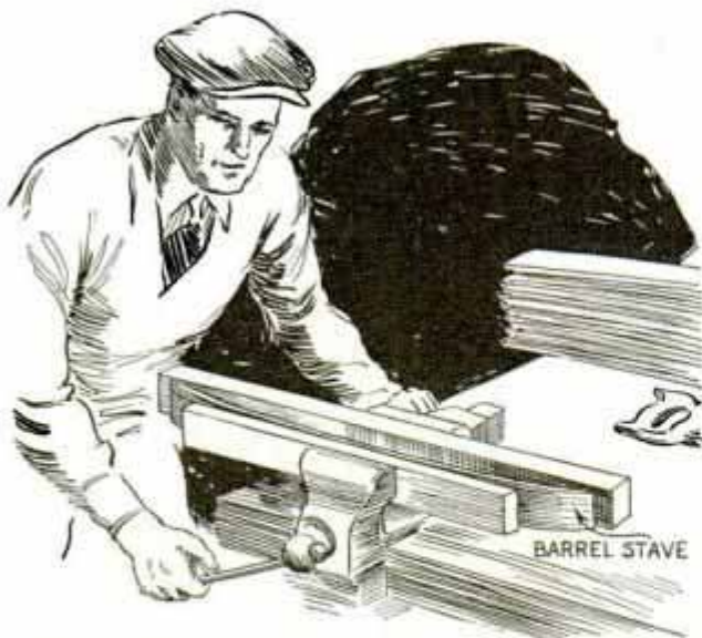
Barrel Staves Soaked in Water and Then Clamped in Vise to Dry Straight Make Good Boat Frames
