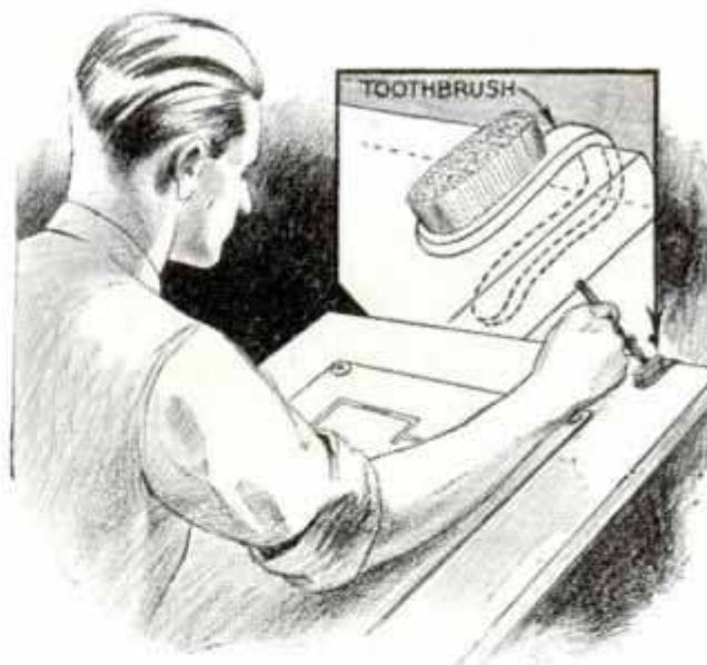
Old Toothbrush Bent to Clamp over Drawing Board Serves as Pen Cleaner
