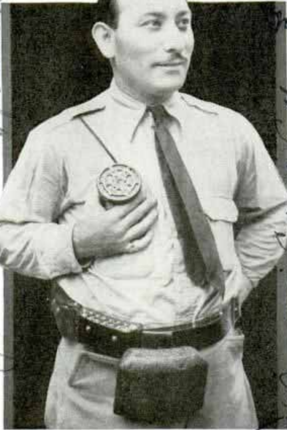
Radio Set for the Man on Foot; the Receiver and Batteries Are Attached to the Belt
