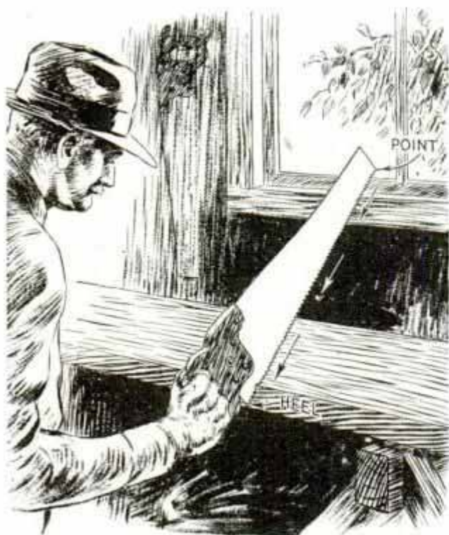
Pulling Newly Filed Saw over Edge of a Scrap Board to Remove Burrs from Teeth
