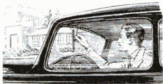
Condensed Moisture on Inside Surface of Windshield Cleaned Off with Hand-Operated Wiper
