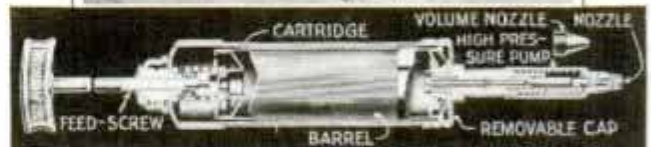
Top, Inserting Grease Cartridge; Bottom, Cutaway Showing Parts of Grease Gun
