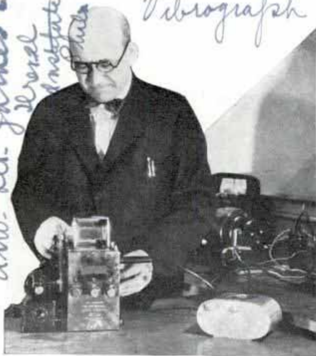
Using an Apparatus Like a Seismograph Which Records Engine Vibrations in Three Dimensions
