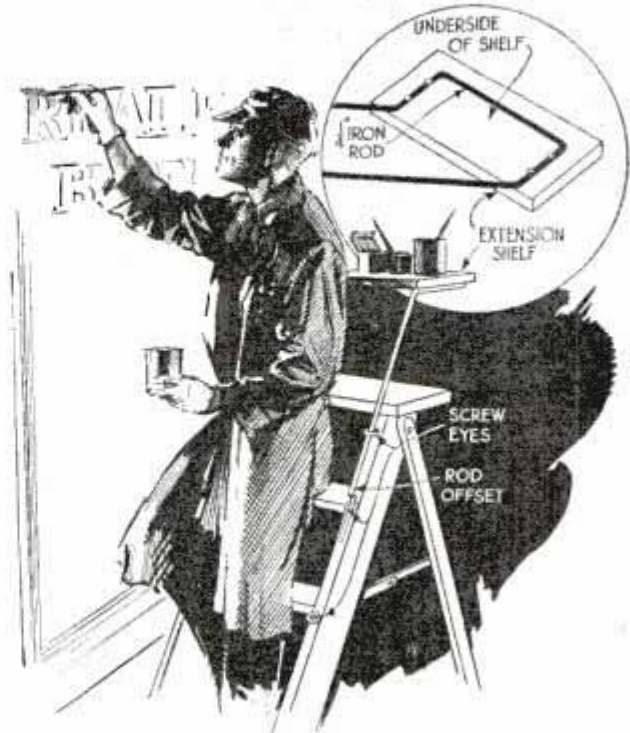
Supported on Screw Eyes, This Extension Shelf for Small Stepladders Keeps Tools within Reach
