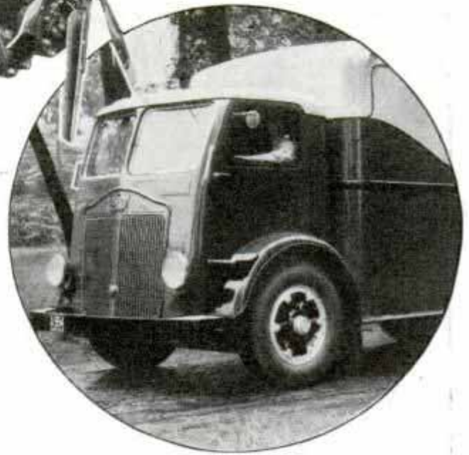
Top, Horizontal or "Pancake" Motor Used in New Truck; Right, Short Front of Truck Designed to Decrease Wind Resistance; Note Driver's Position
