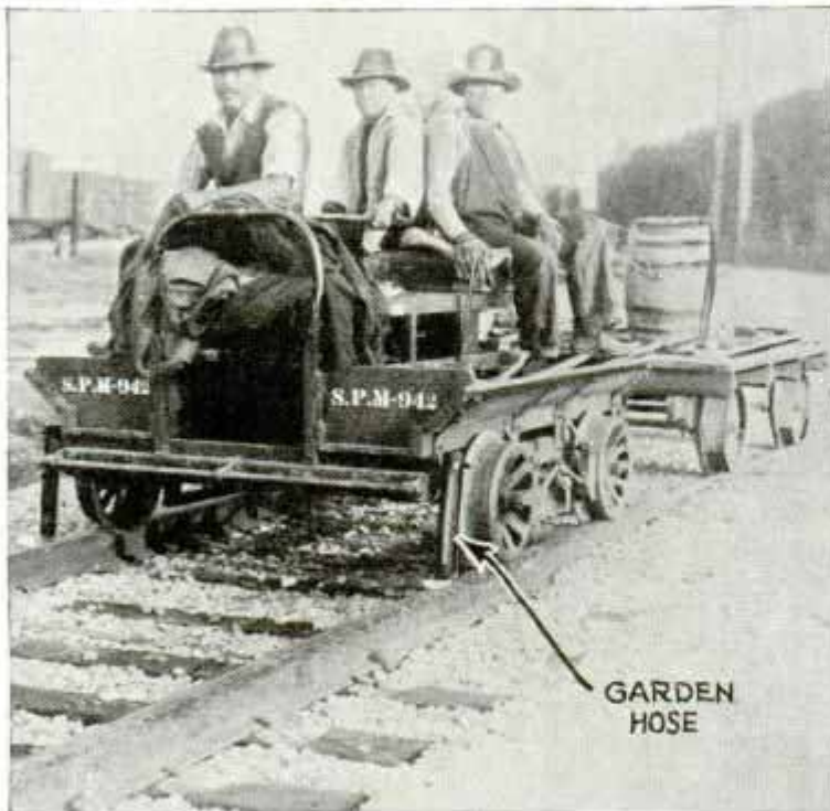
Short Pieces of Hose on Motor Section Car Sweep Small Rocks Off Rails
