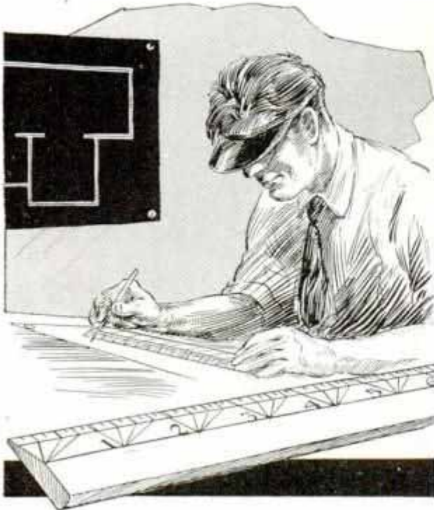
Lines Scratched in Surface of Rule to Indicate Division Marks, Aid in Making Line Drawings
