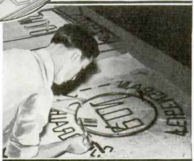
Above, Transferring Diagram to Asbestos Pattern and, Below, Glass Bender Shaping Tubing to Conform with Pattern
