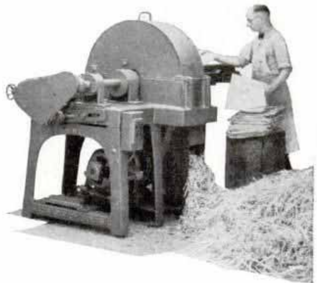
Shredding Machine Which Converts Old Newspapers and Magazines into Excelsior
