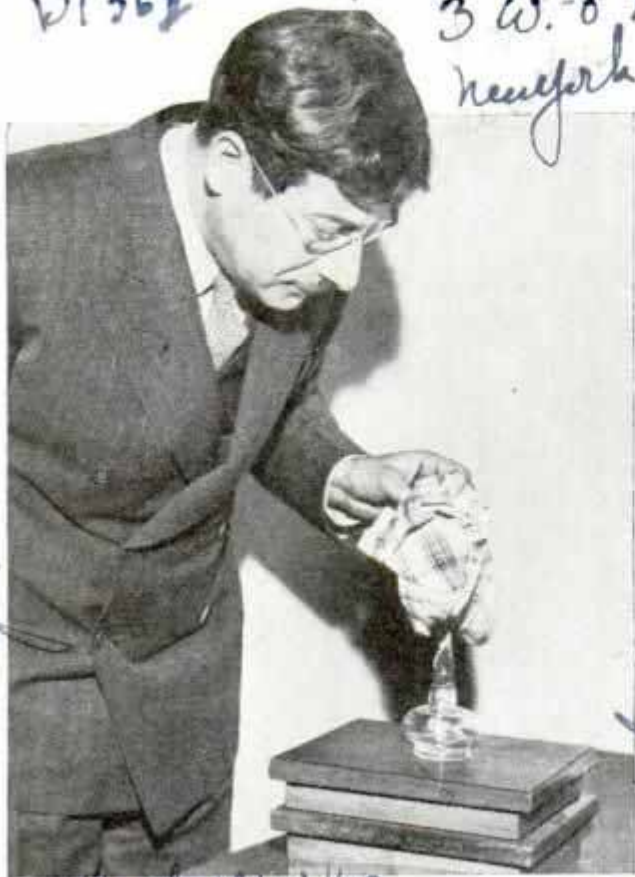
This Piece of Cloth Which Has Been Fireproofed Is Being Tested by Placing It in Flame
