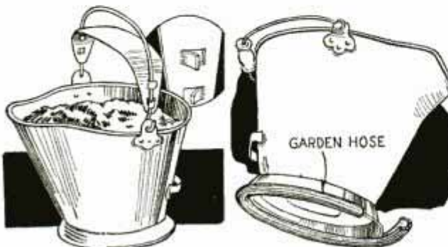
Hose Prevents Coal Hod Marring Floors, and Shield on Bail Protects Hand from Hot Ashes
