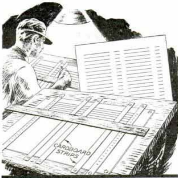
When Duplicate Forms Are Needed, Cardboard Spacing Strips Help to Do the Ruling Quickly
