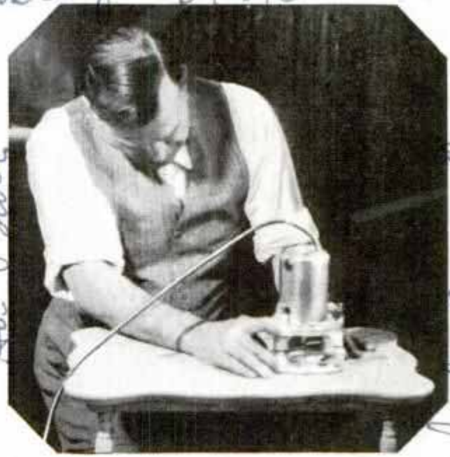
Electric Router That Runs at High Speed May Serve Many Purposes of the Craftsman
