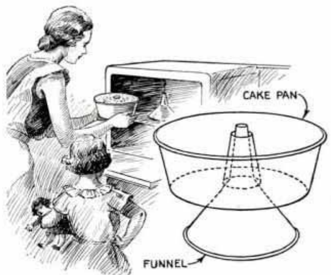
Pan Set on Funnel in Oven to Get Uniform Temperature When Baking Angel-Food Cake
