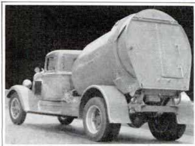
Refuse Collection Truck Equipped with Rotating Tank Which Aids in Loading and Dumping
