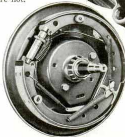
Above, Give Your Thermostatically Controlled Shock Absorbers Time to Adjust Themselves to New Kind of Road; Left, the Internal Expanding Brake Does Not Burn and Seize When Over-Used on Long Grade; It Simply "Fades" and Fails to Stop Car Efficiently
