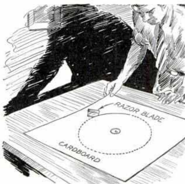
Cardboard Disks of Any Diameter Are Cut Easily with Aid of Thumb Tack and Razor Blade
