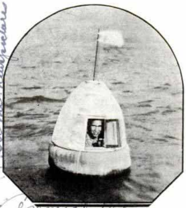
Inflated Rubber Life Preserver with an Upper Section to Protect the Face and Head
