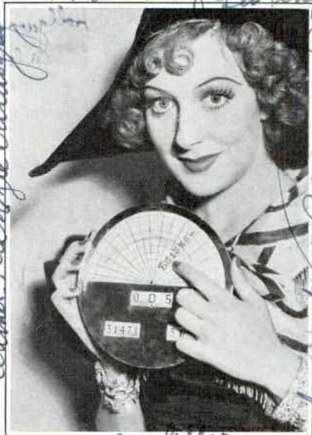
© Paramount Productions, Inc. This Speedometer Keeps a Chart Record of the Miles per Hour Traveled during a Trip
