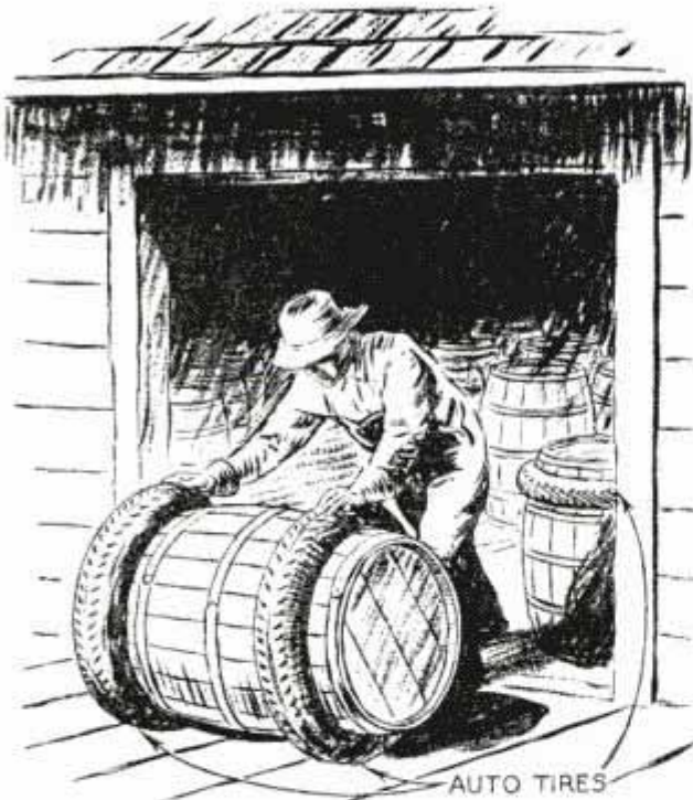
Old Auto Tires Useful in Avoiding Breakage When Handling Heavy Barrels in the Warehouse
